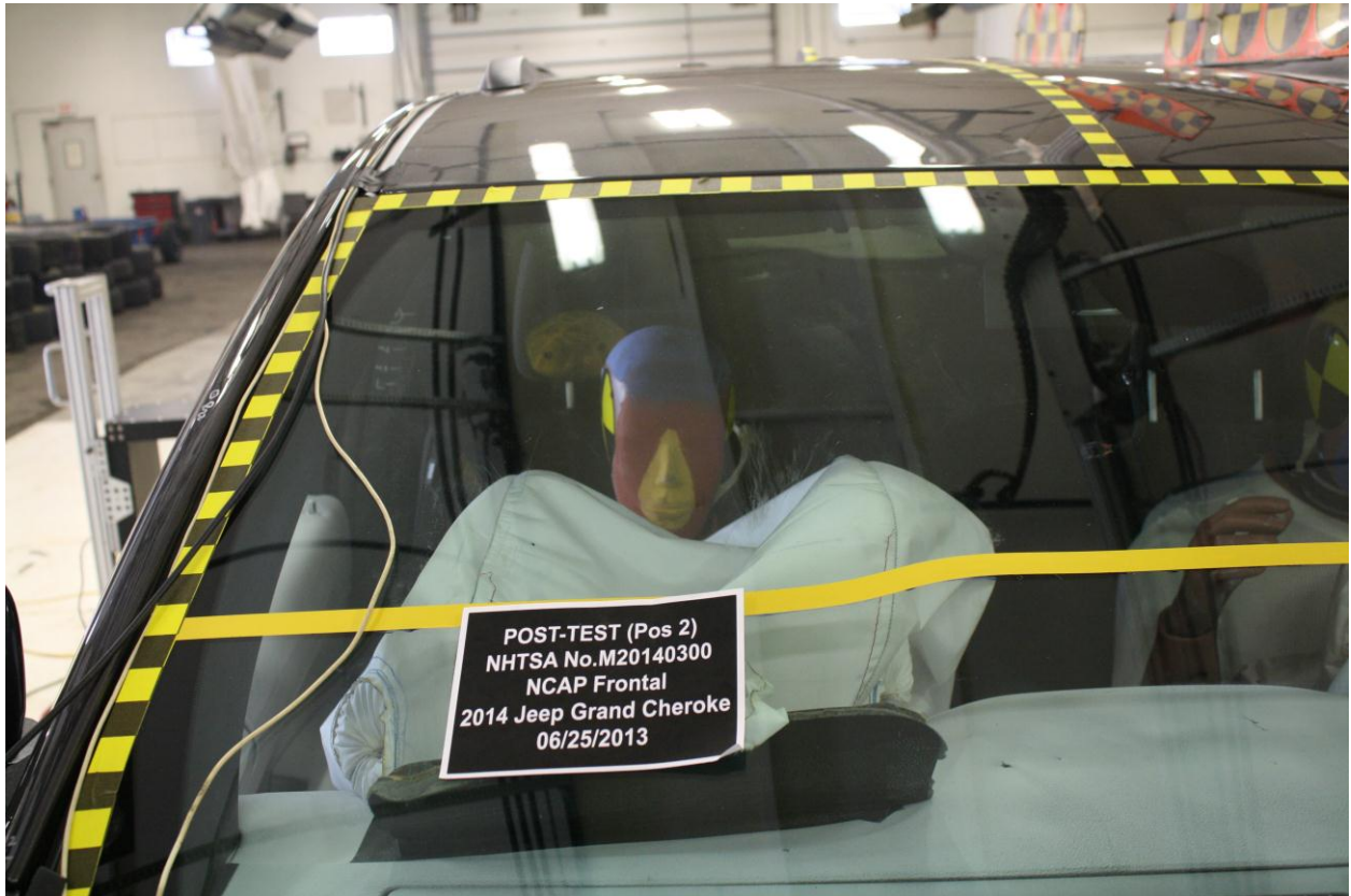
Figure A-51: Post-Test Passenger Dummy Front View
