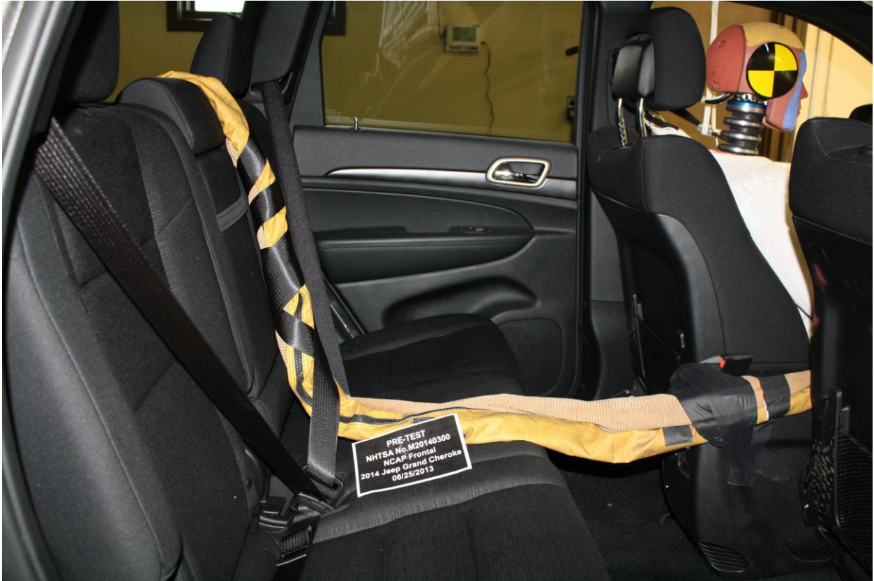
Figure A-27: Pre-Test Dummy Cable Routing
