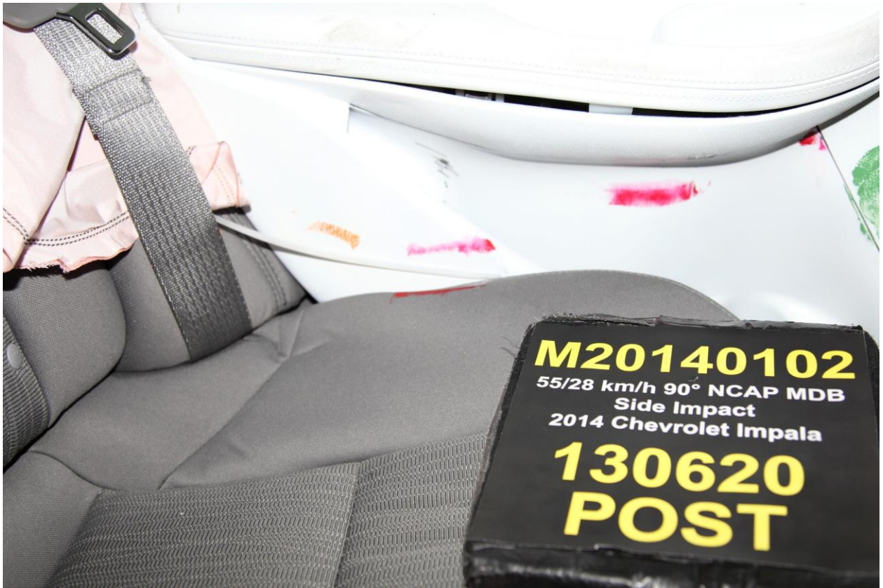
080 Post-Test Rear Passenger Dummy Close-Up Pelvis Contact with Side Airbag View
