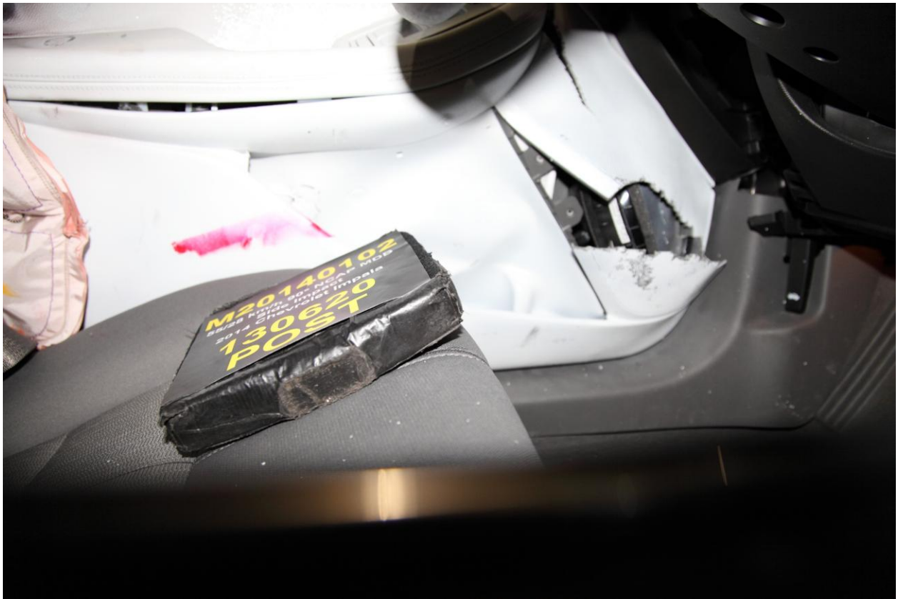
054 Post-Test Driver Dummy Close-Up Knee Contact View
