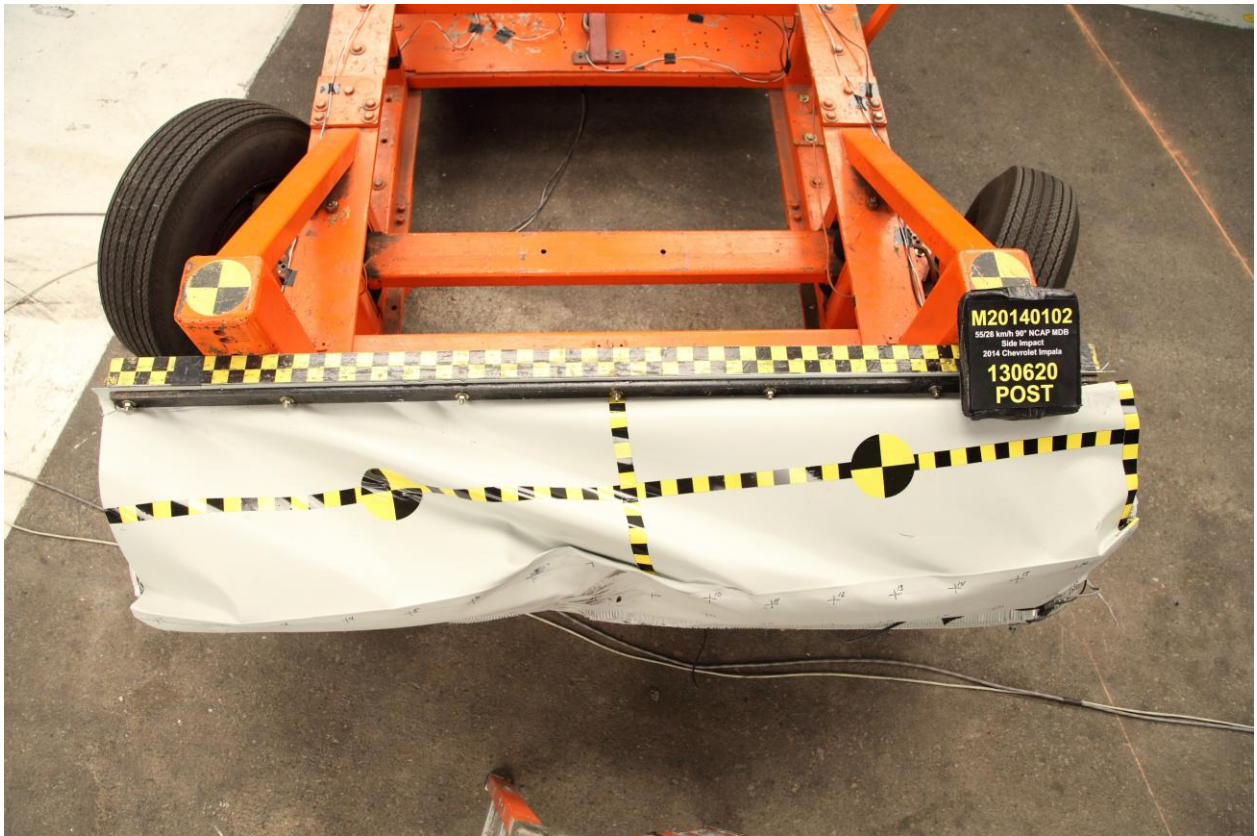
087 Post-Test Top View of MDB Impactor Face
