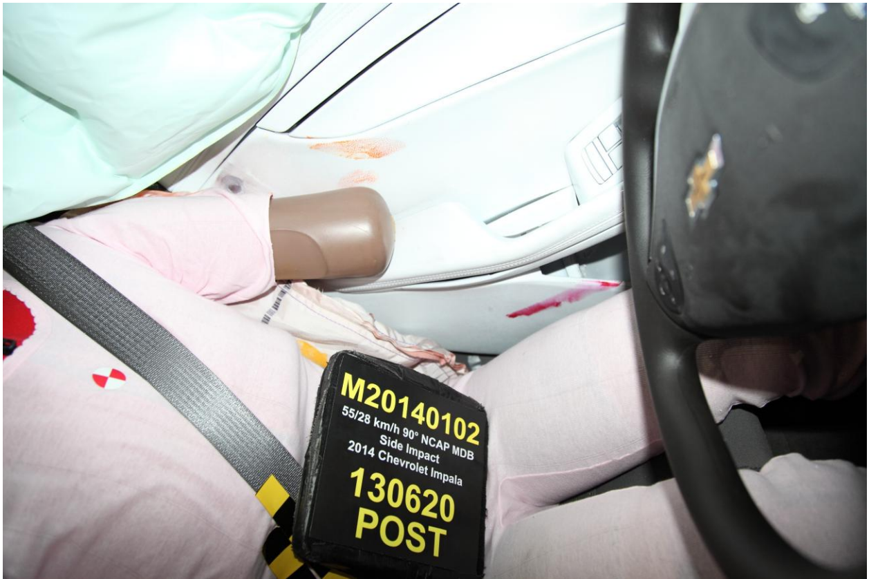
043 Post-Test Driver Dummy and Door Clearance View
