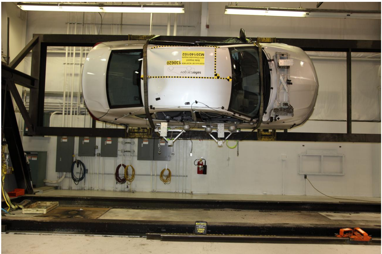
097 FMVSS No. 301 Static Rollover 90 Degrees
