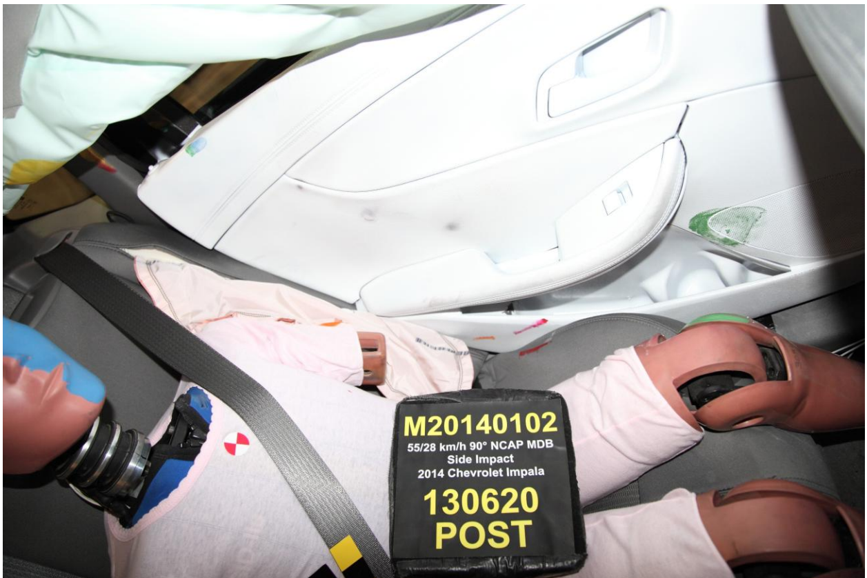
070 Post-Test Passenger Dummy and Door Clearance View
