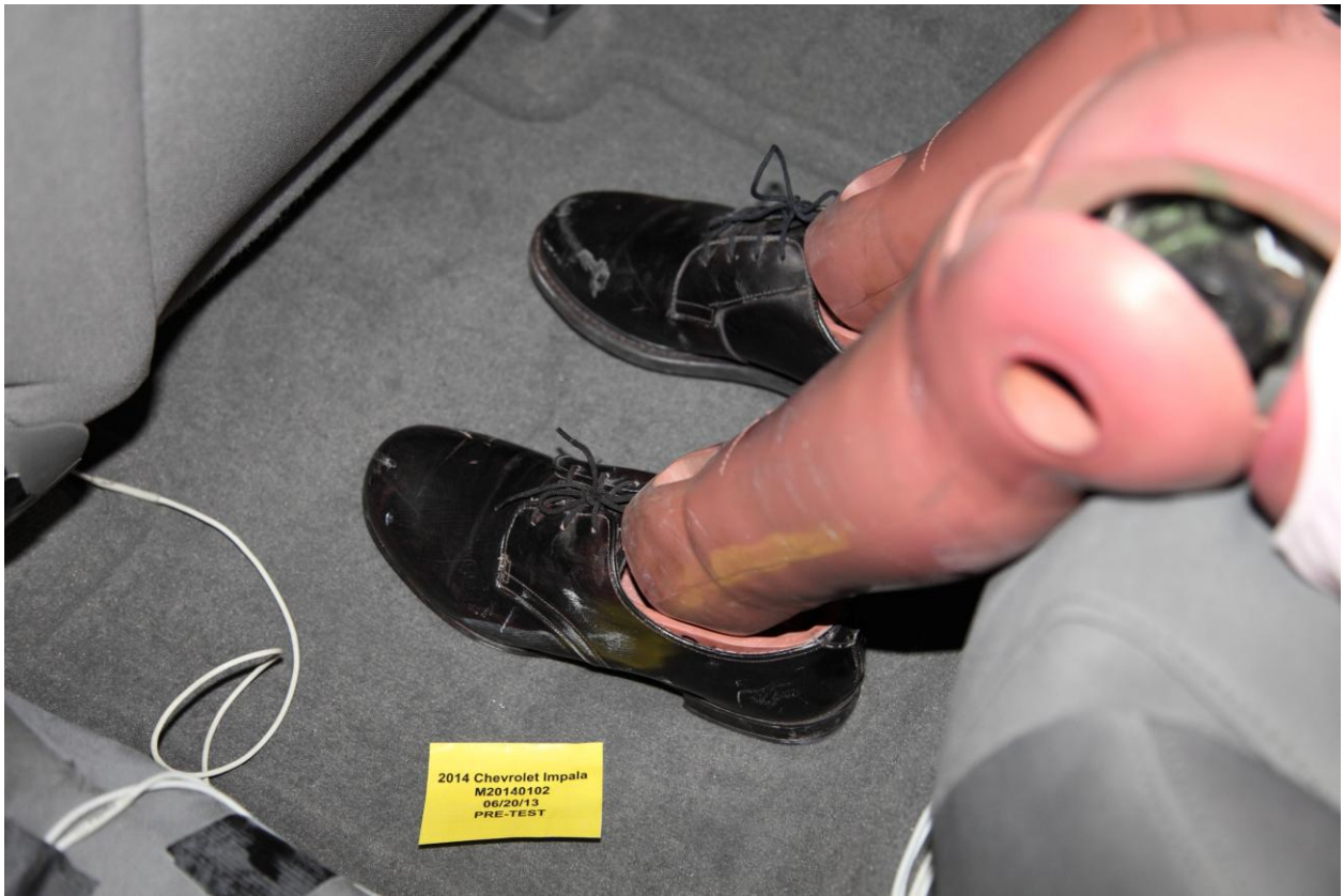
064 Pre-Test Placement of Rear Passenger Dummy Feet
