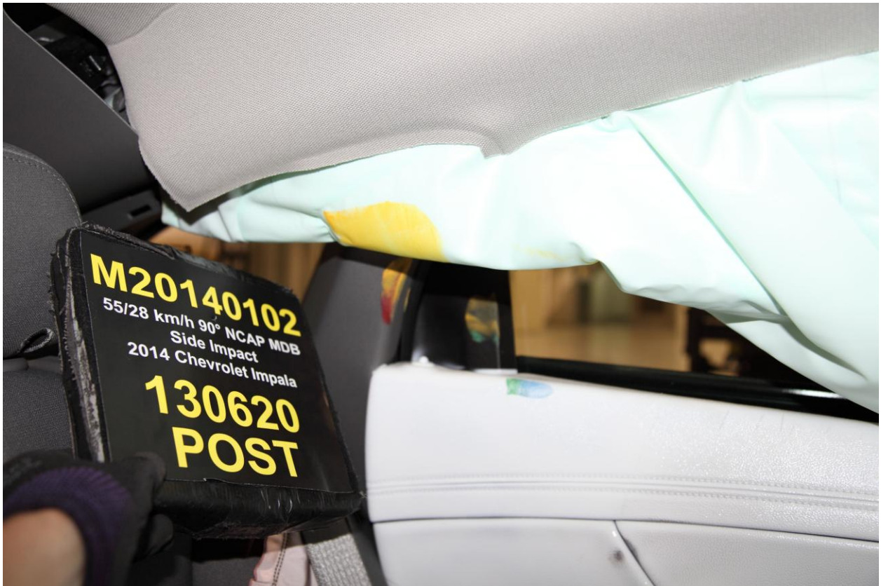
075a Post-Test Rear Passenger Dummy Close-Up Head Contact with Vehicle View
