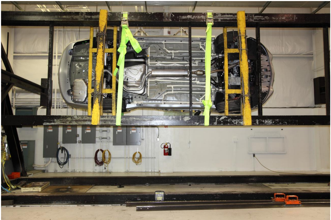
099 FMVSS No. 301 Static Rollover 270 Degrees
