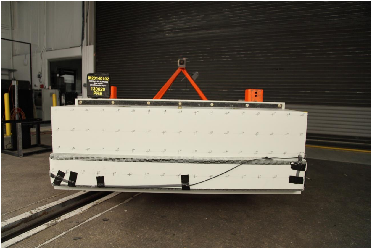
084 Pre-Test Front View of MDB Impactor Face
