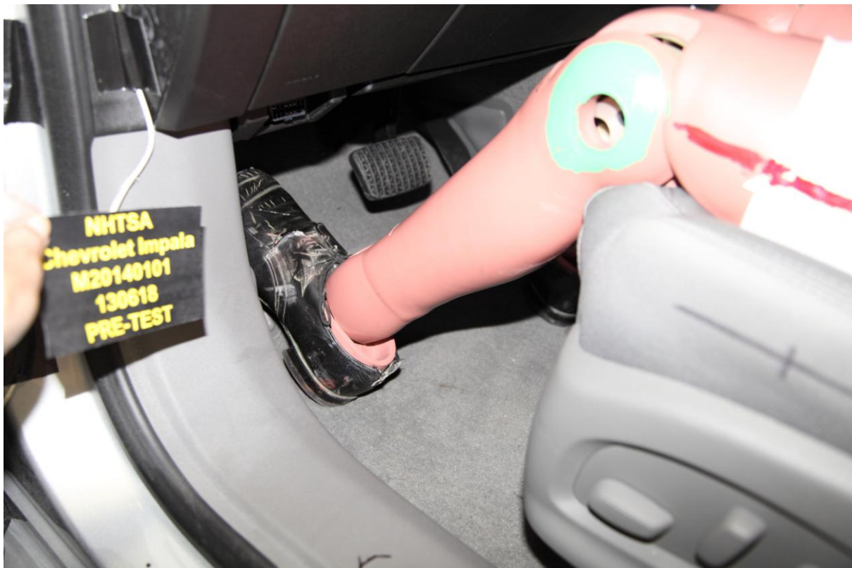
032 Pre-Test Placement of Dummy Feet
