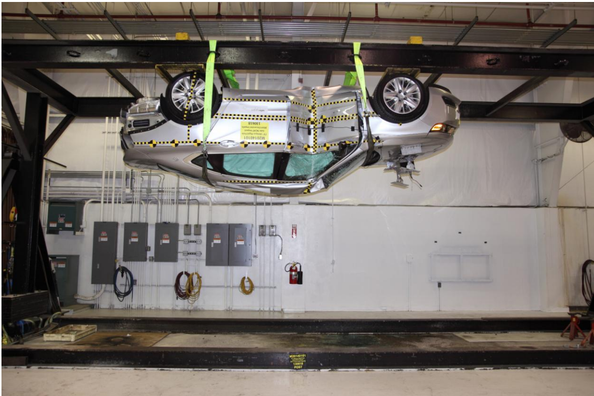
065 FMVSS No. 301 Static Rollover 180 Degrees
