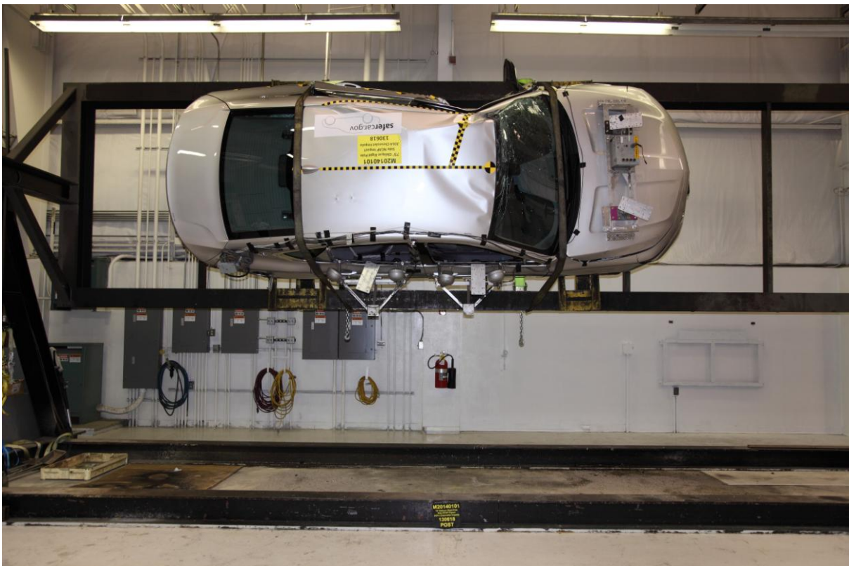
064 FMVSS No. 301 Static Rollover 90 Degrees
