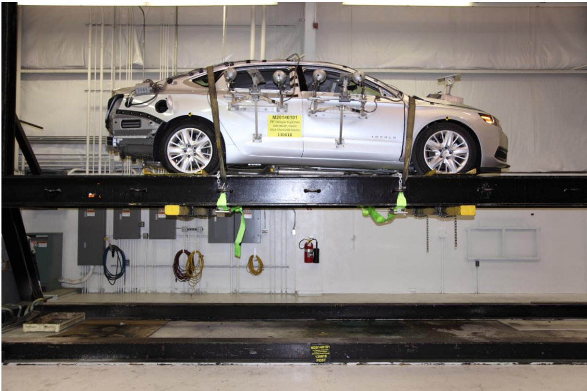
067 FMVSS No. 301 Static Rollover 360 Degrees
