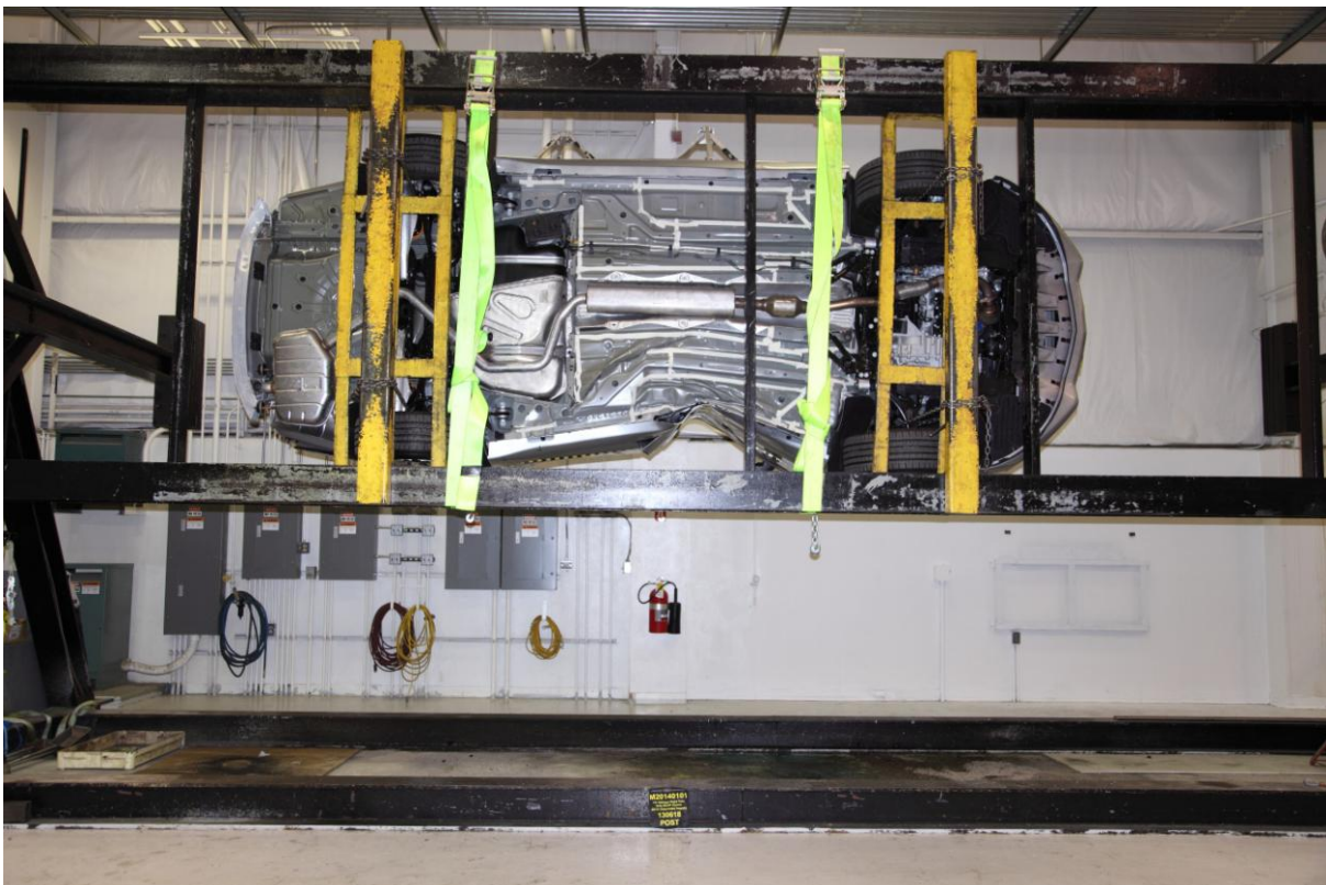
066 FMVSS No. 301 Static Rollover 270 Degrees
