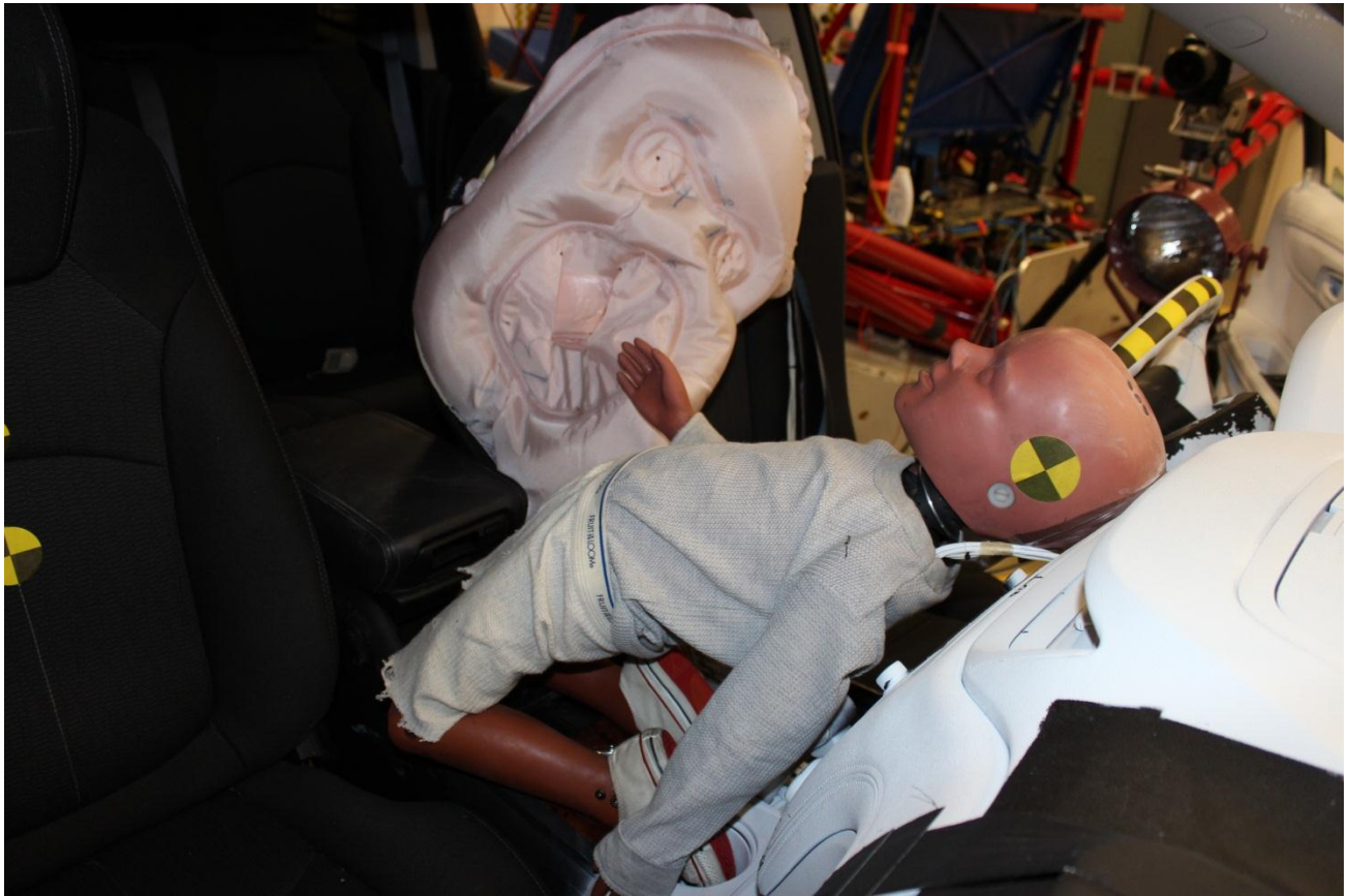
Figure A-17: Post-Test HIII 3 Year Old Dummy Right \frac{3}{4} Front View
