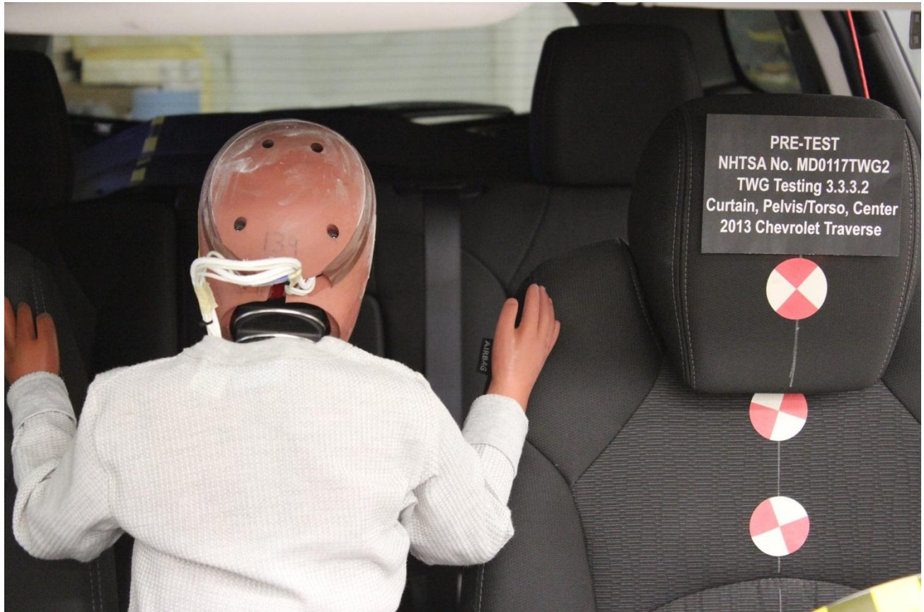
Figure A-15: Pre-Test HIII 3 Year Old Dummy Front Close-up View
