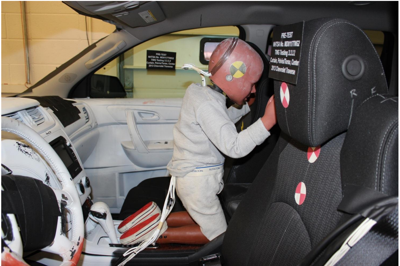
Figure A-5: Pre-Test HIII 3 Year Old Dummy Left Side View
