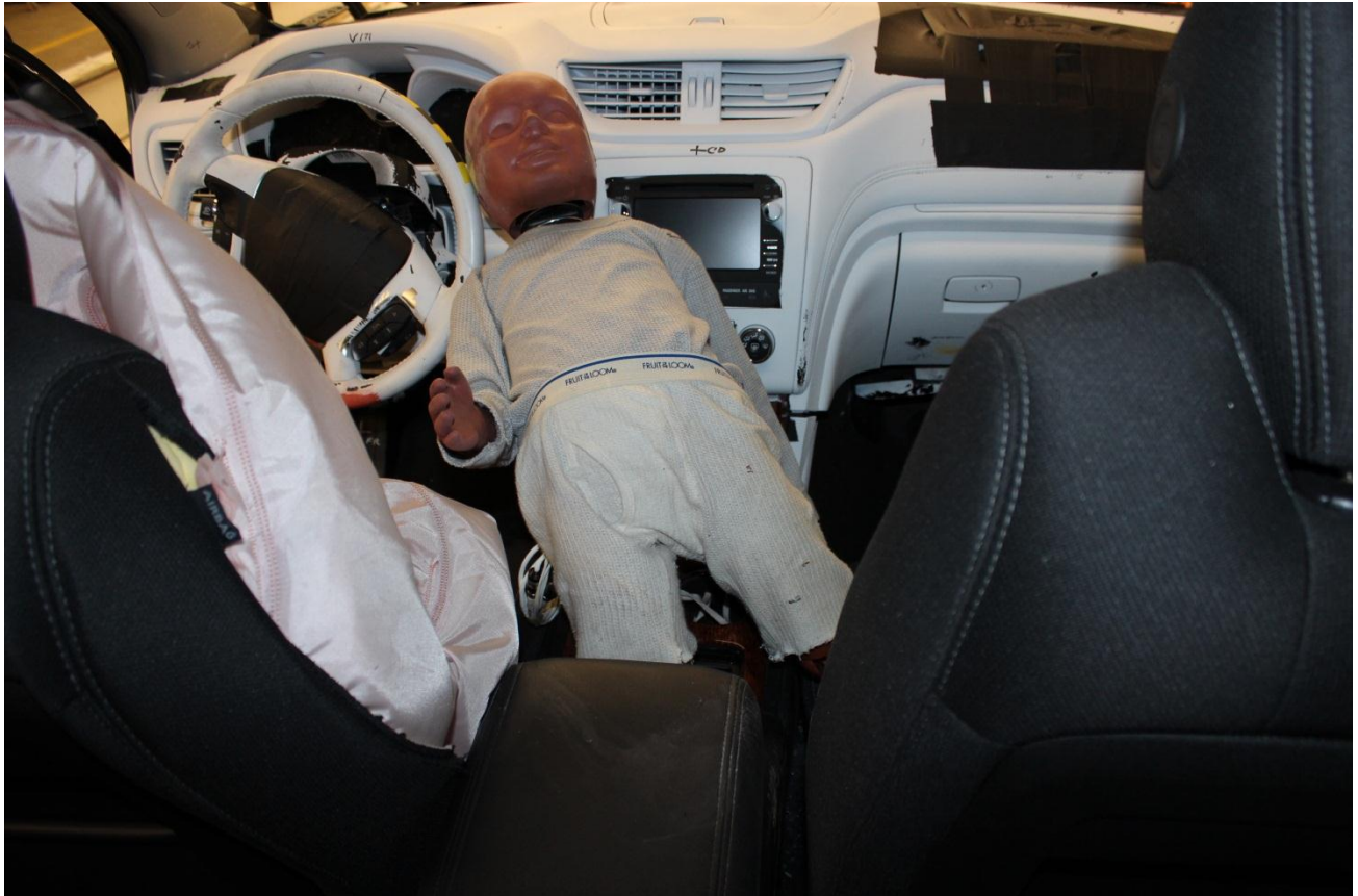
Figure A-22: Post-Test HIII 3 Year Old Dummy Rear View
