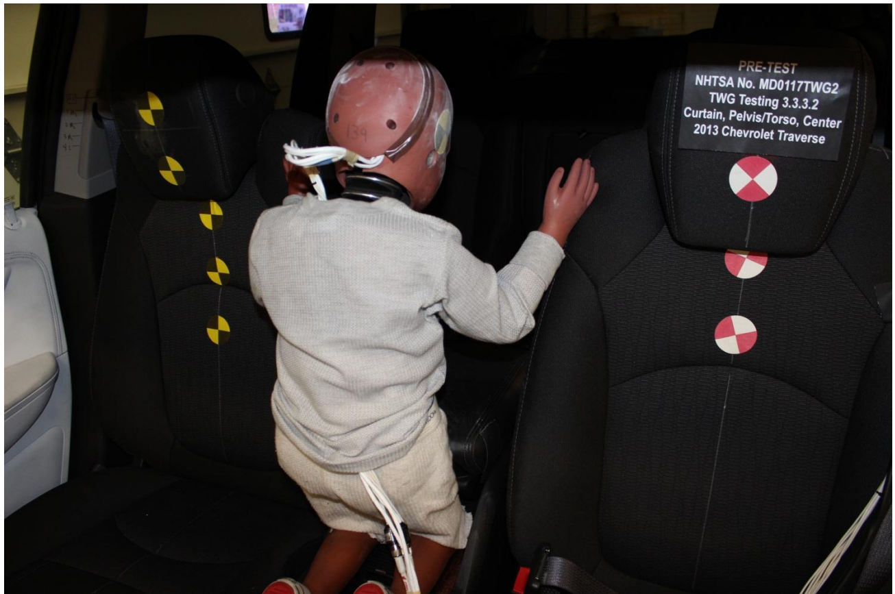
Figure A-9: Pre-Test HIII 3 Year Old Dummy Left \frac{3}{4} Front View
