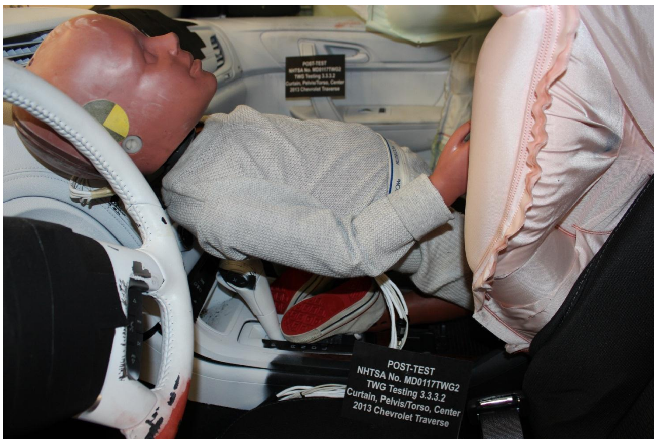
Figure A-8: Post-Test HIII 3 Year Old Dummy Left Side Close-up View
