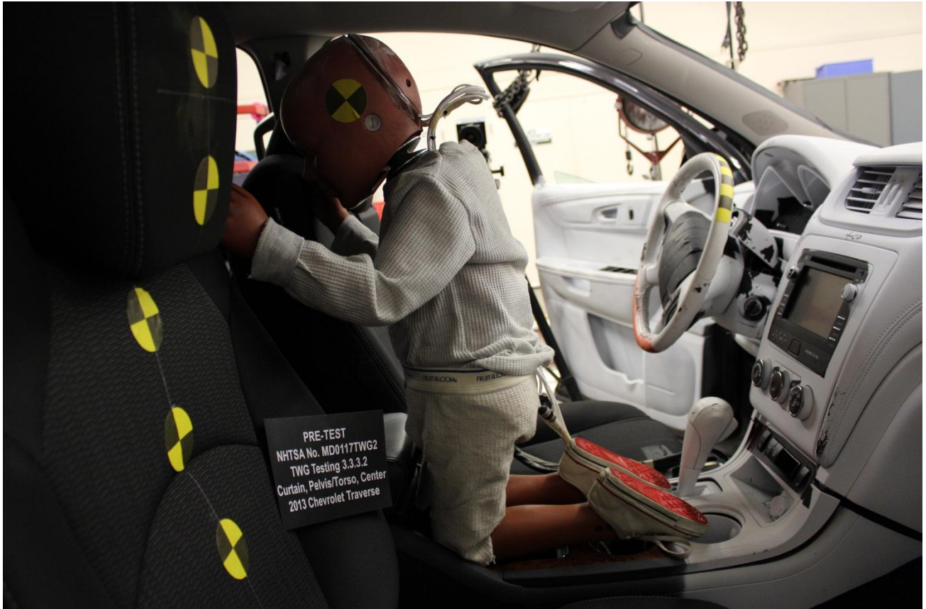
Figure A-18: Pre-Test HIII 3 Year Old Dummy Right Side View
