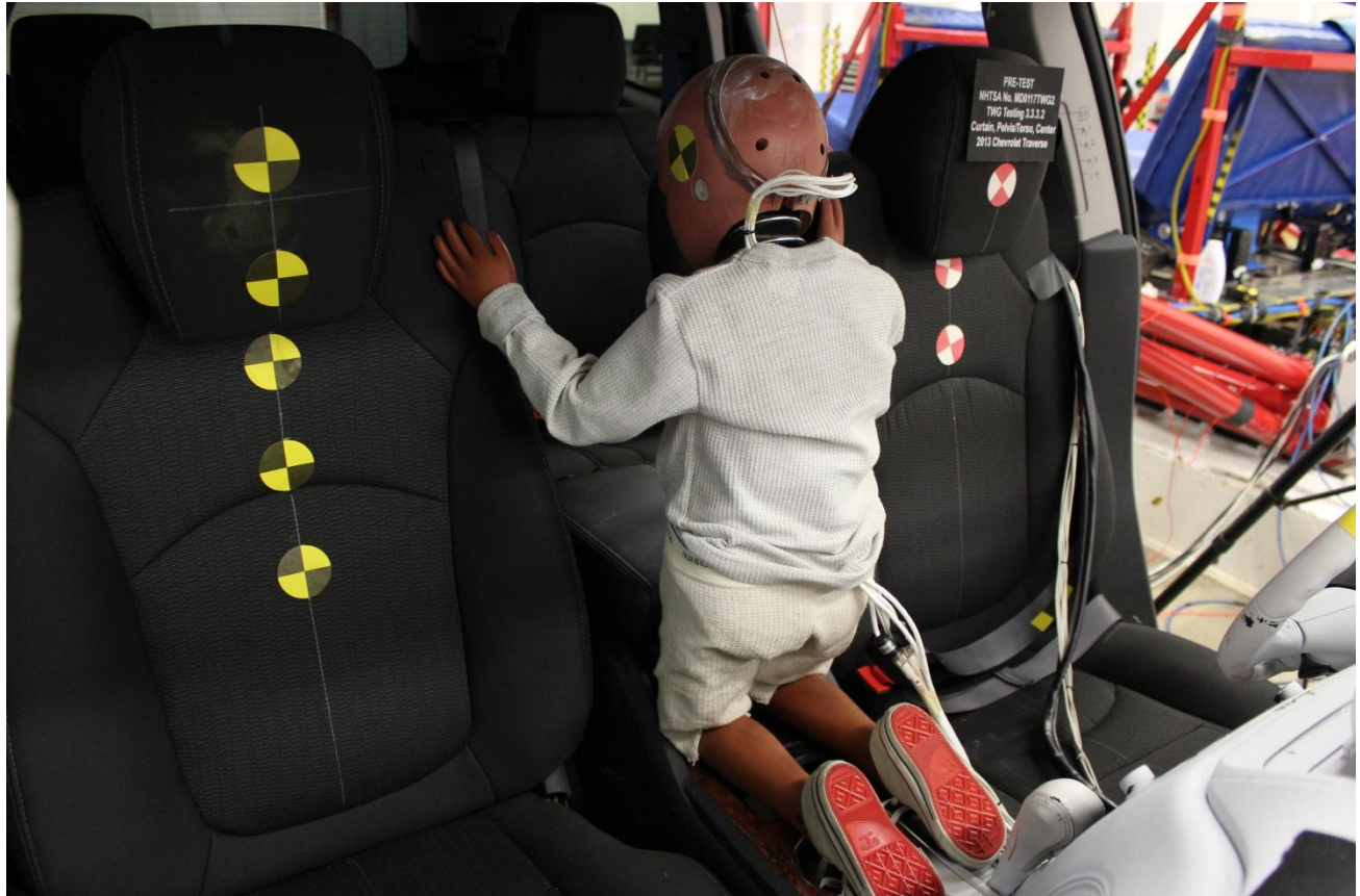
Figure A-16: Pre-Test HIII 3 Year Old Dummy Right \frac{3}{4} Front View
