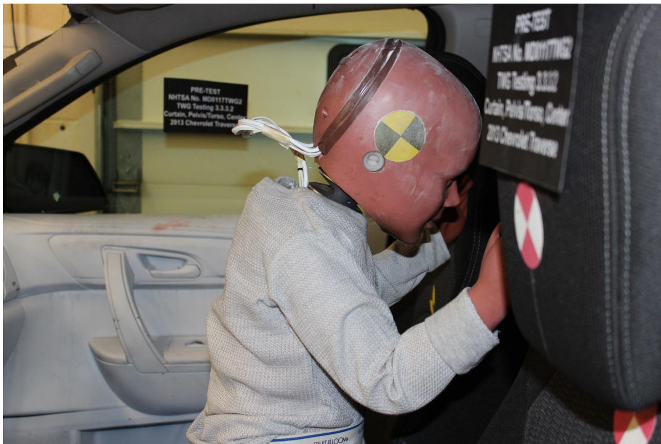
Figure A-7: Pre-Test HIII 3 Year Old Dummy Left Side Close-up View
