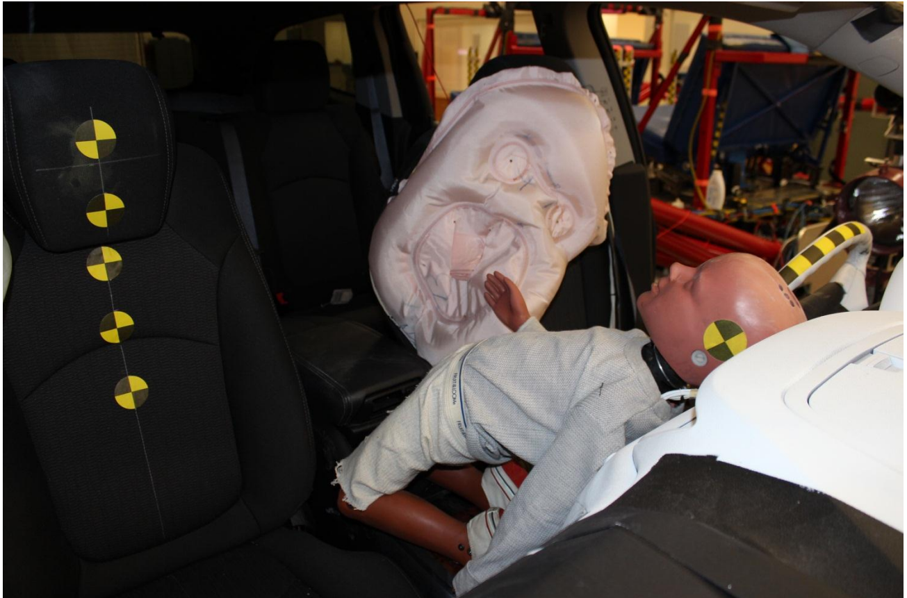
Figure A-24: Post-Test Center Airbag Right \frac{3}{4} Front View
