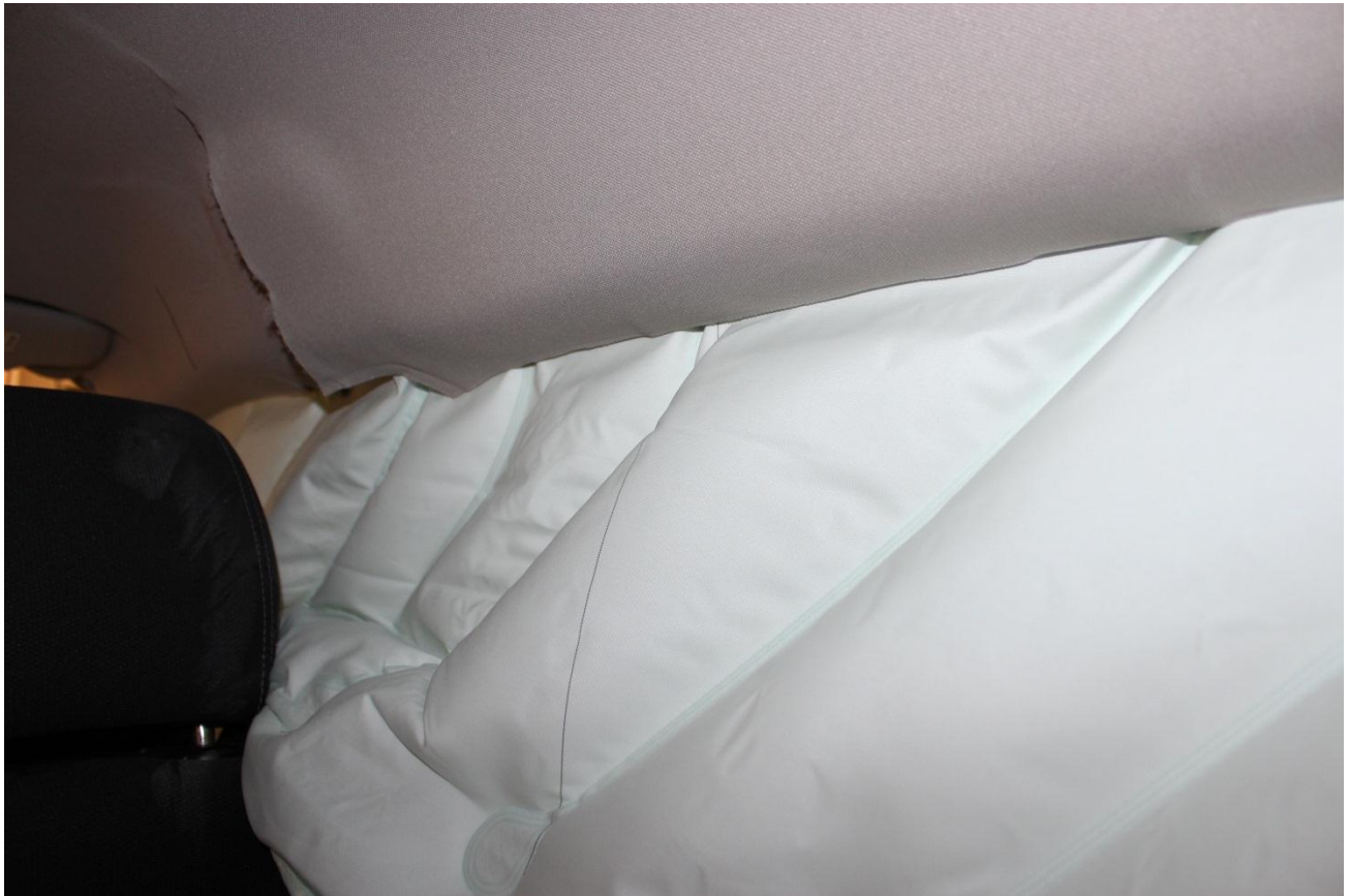
Figure A-23: Post-Test Curtain Airbag Right \frac{3}{4} Rear View
