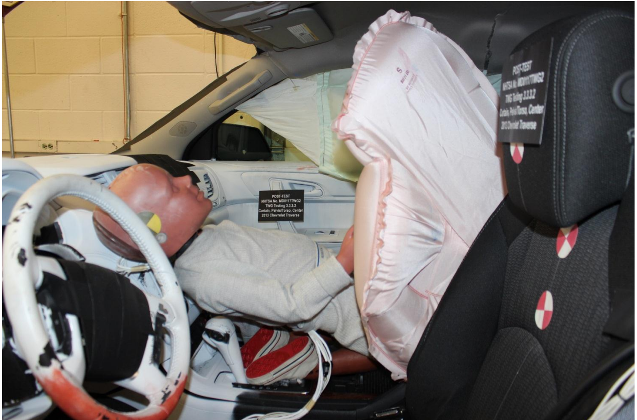
Figure A-6: Post-Test HIII 3 Year Old Dummy Left Side View
