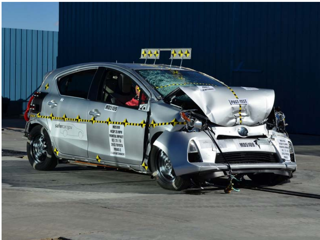
FIGURE 4. Post-Test Right Front ¼ View of NCAP Frontal Impact Test
