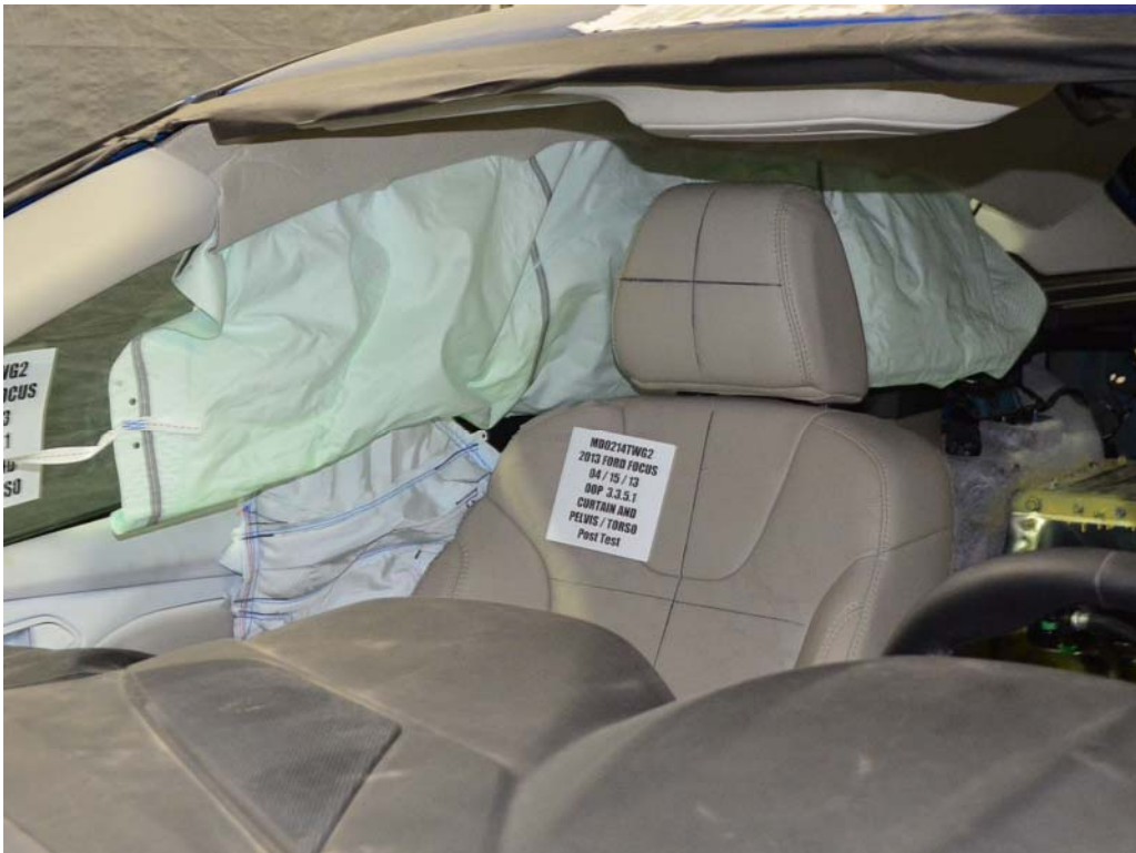
FIGURE 14. Post-Test Airbags, Left Front ¾ View
