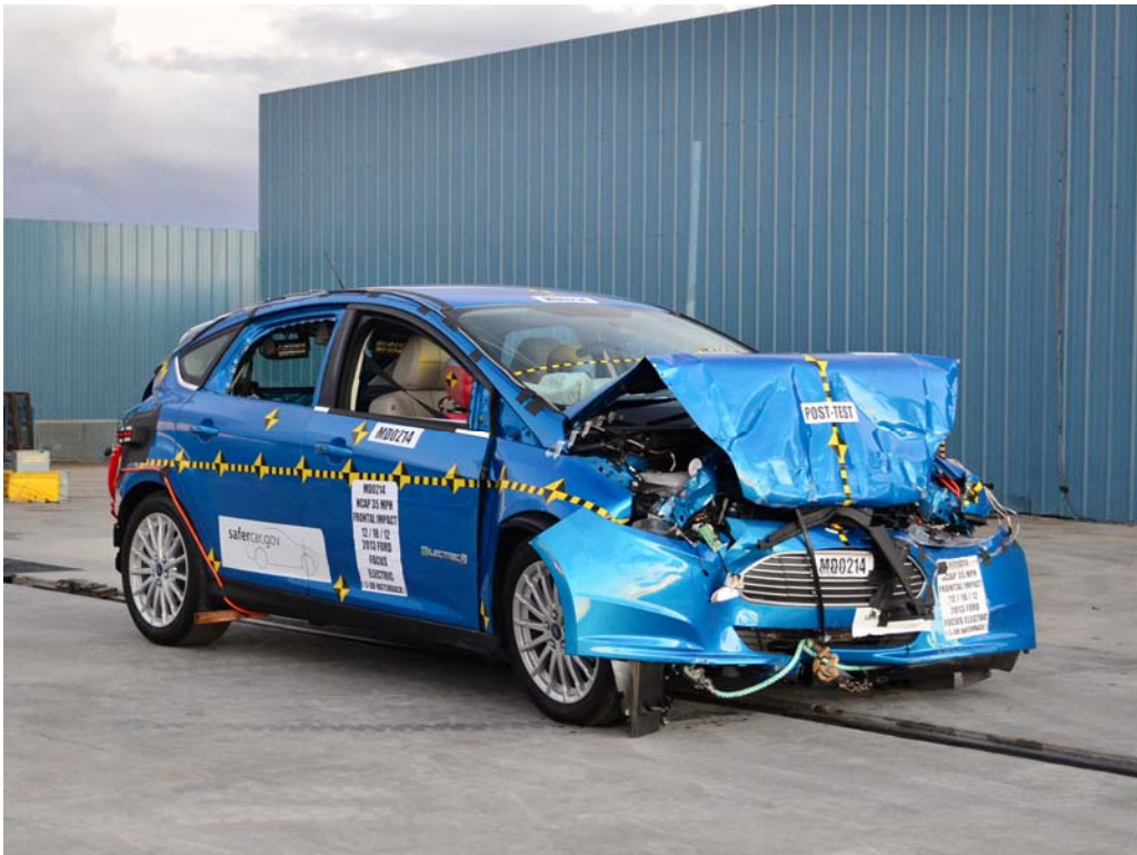
FIGURE 4. Post-Test Right Front 1/4 View of NCAP Frontal Impact Test
