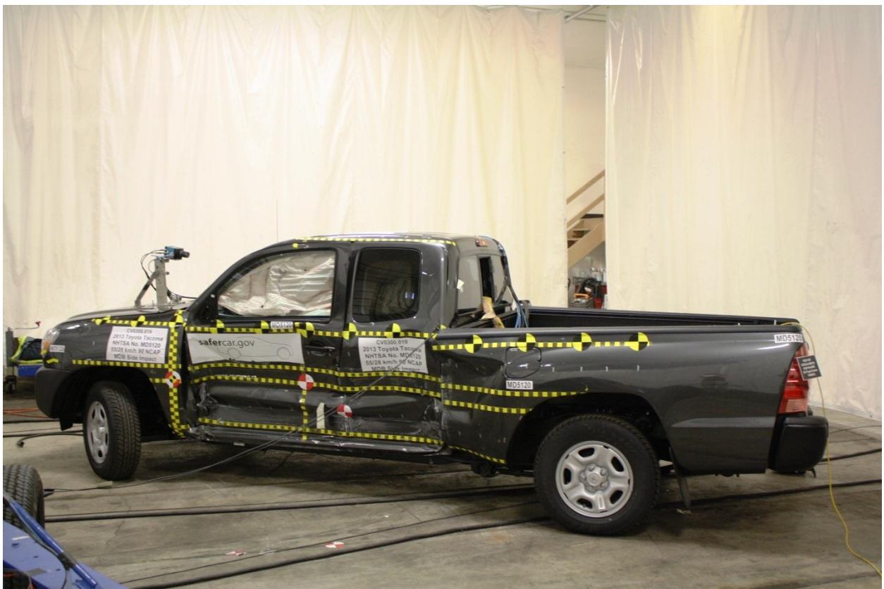
Figure A-24: Post NCAP Left Side View
