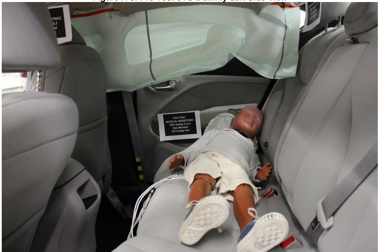
Figure A-6: Post-Test 3YO Dummy Left Side View
