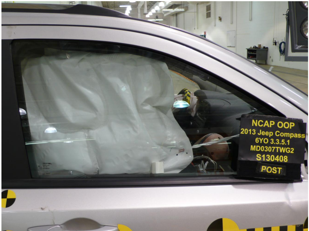
Figure A-15 Post-Test Front Passenger Door-Window
