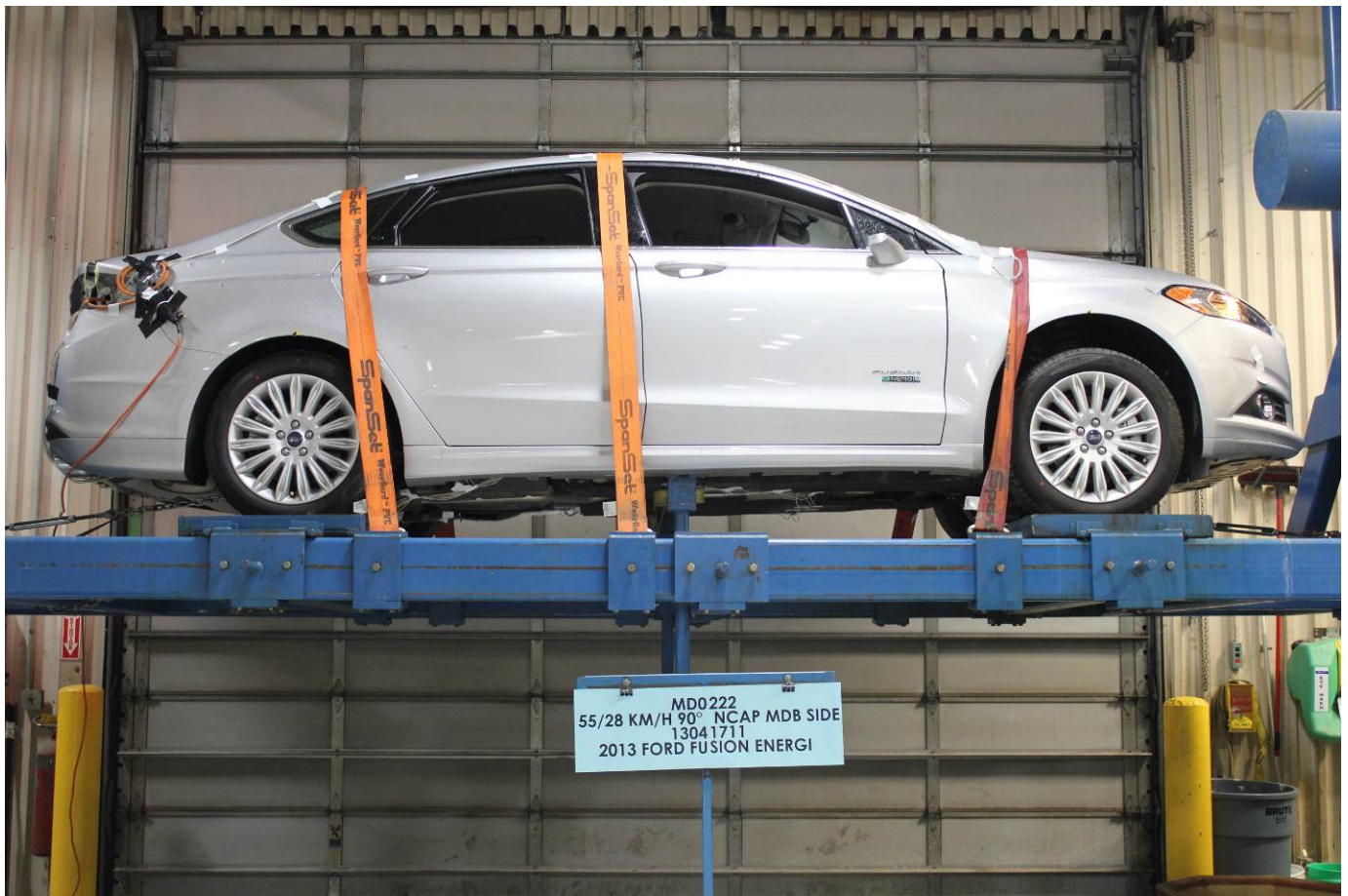
FMVSS No. 301 Static Rollover 0 Degrees
