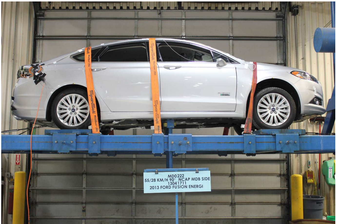
FMVSS No. 301 Static Rollover 360 Degrees
