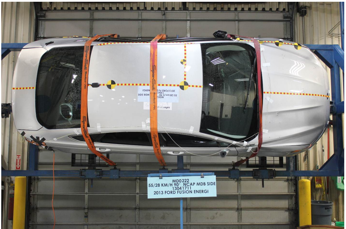
FMVSS No. 301 Static Rollover 270 Degrees
