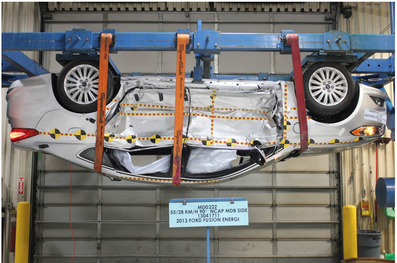
FMVSS No. 301 Static Rollover 180 Degrees
