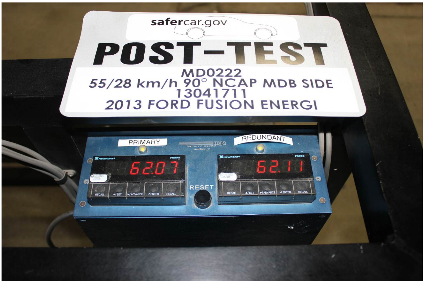
Post-Test Primary and Redundant Speed Trap Read-Out
