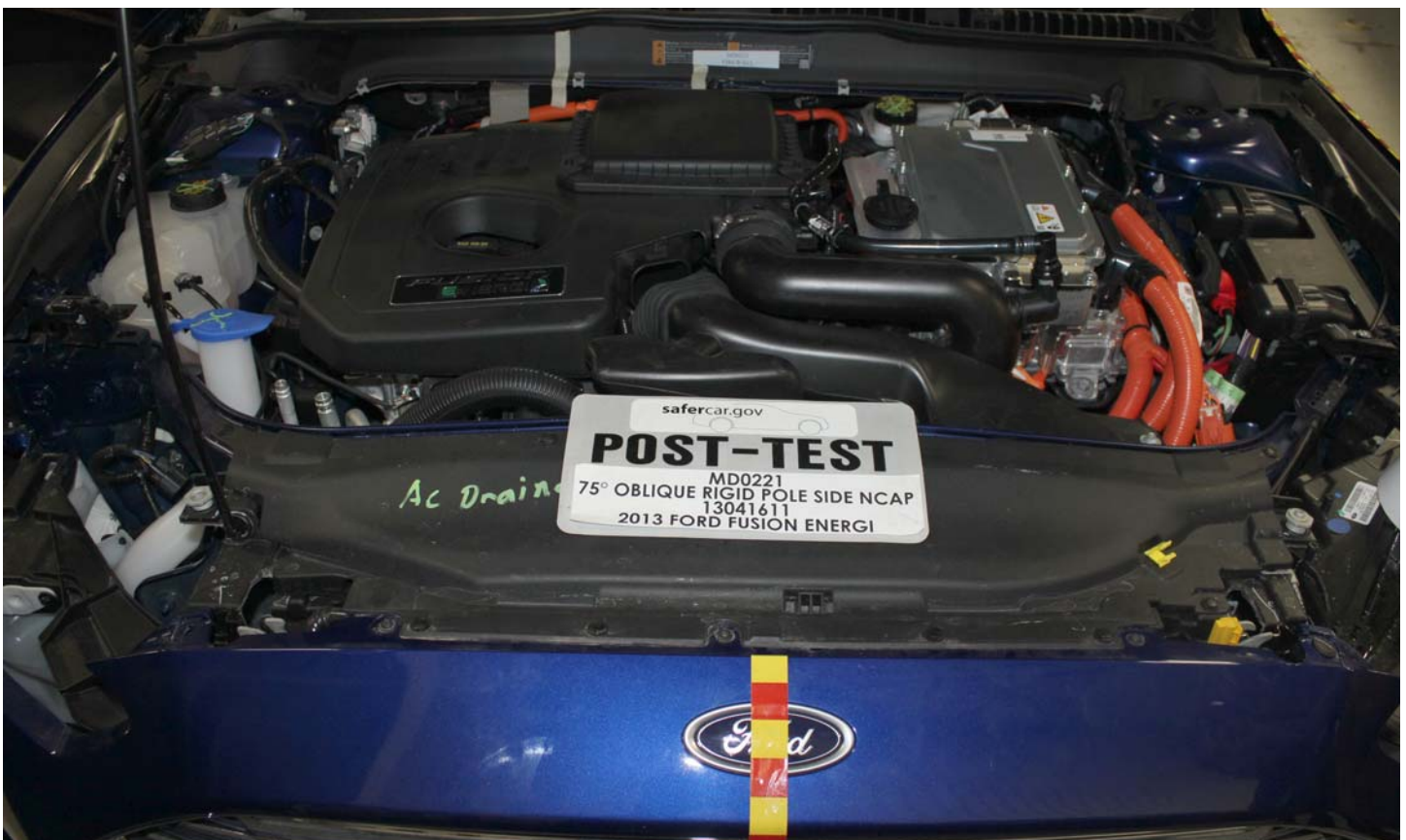
No. 017 Post-Impact View of Electric Propulsion Drive
