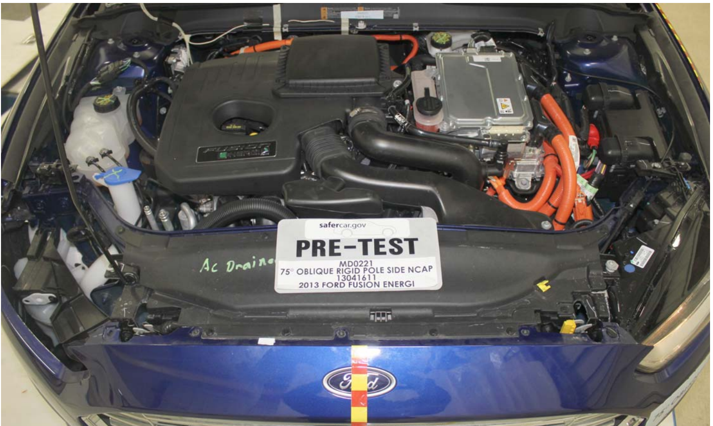
No. 016 Pre-Impact View of Electric Propulsion Drive
