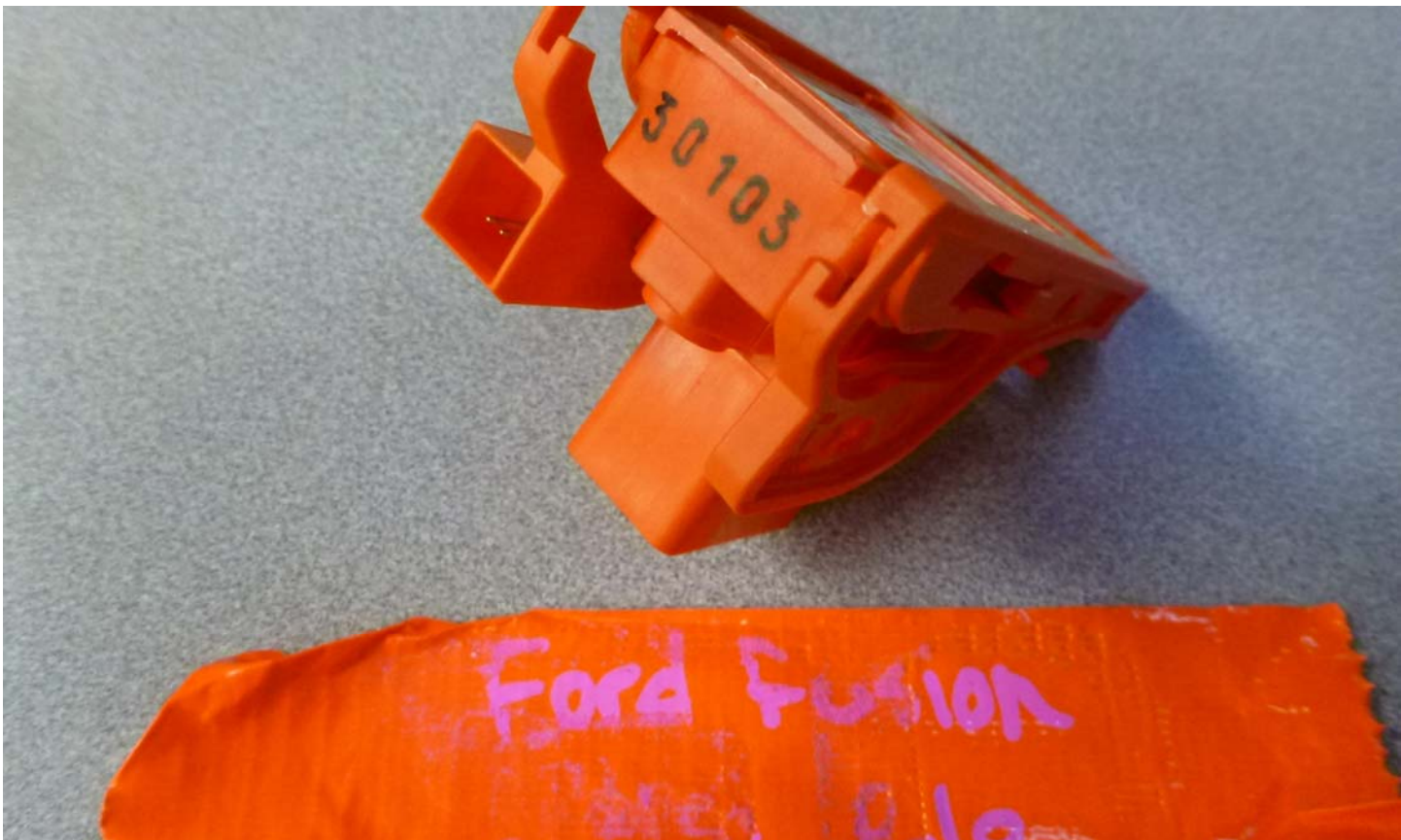
No. 008 Manual High Voltage Service Disconnect Removed
