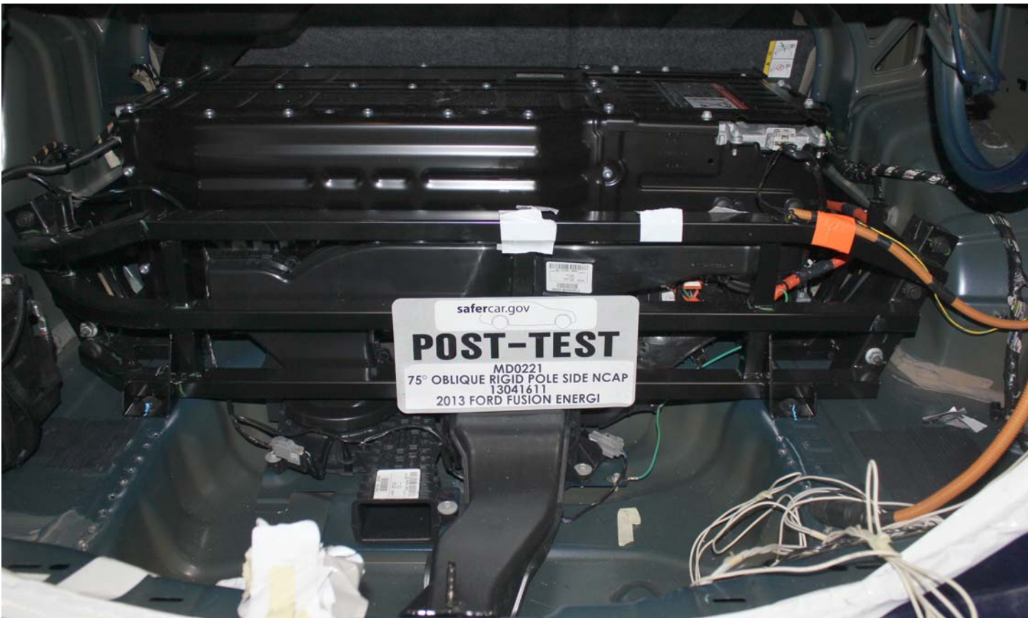
No. 011 Post-Impact Rear View of Propulsion Battery
