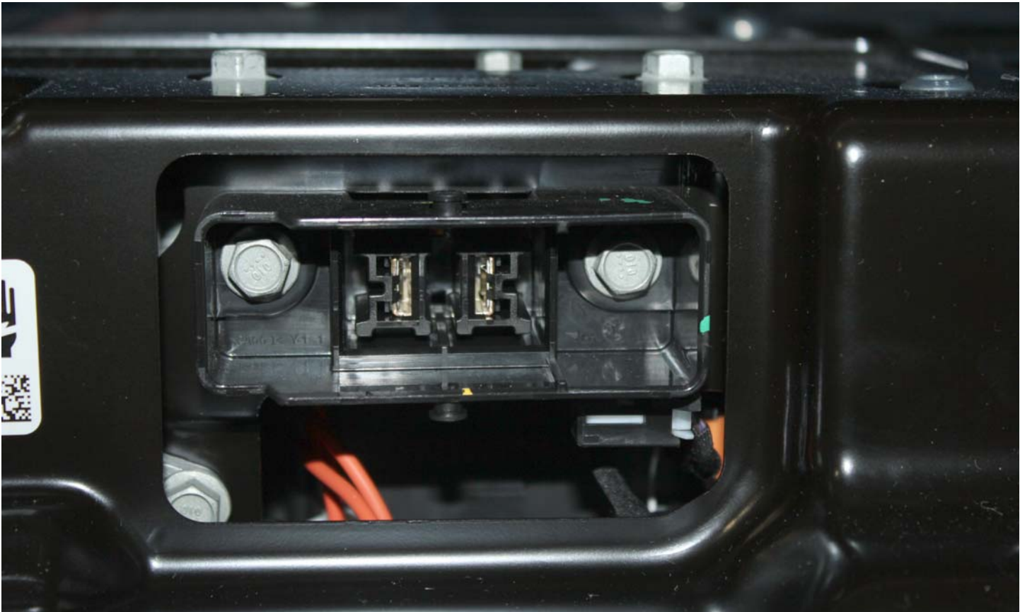
No. 007 Manual High Voltage Service Disconnect Removed
