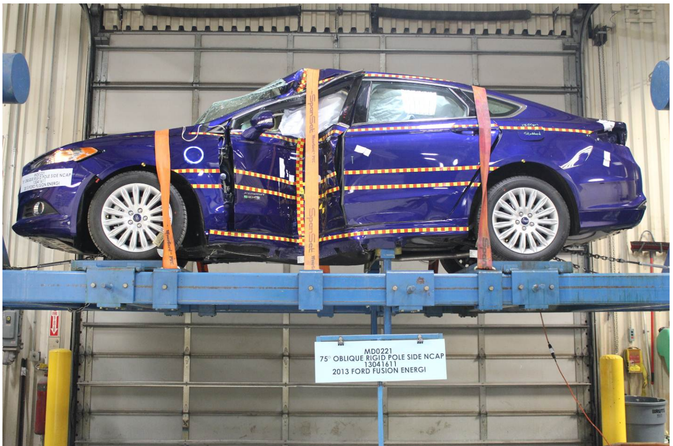
FMVSS No. 301 Static Rollover 360 Degrees
