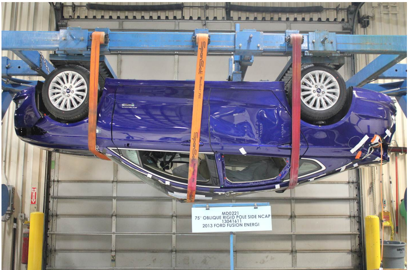
FMVSS No. 301 Static Rollover 180 Degrees
