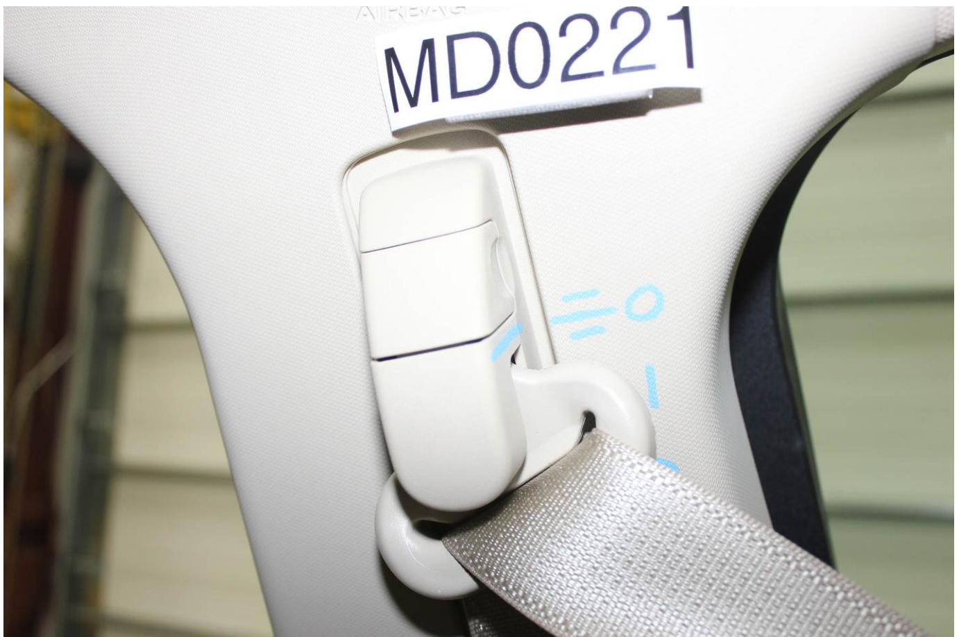
Pre-Test View of Belt Anchorage for Dummy
