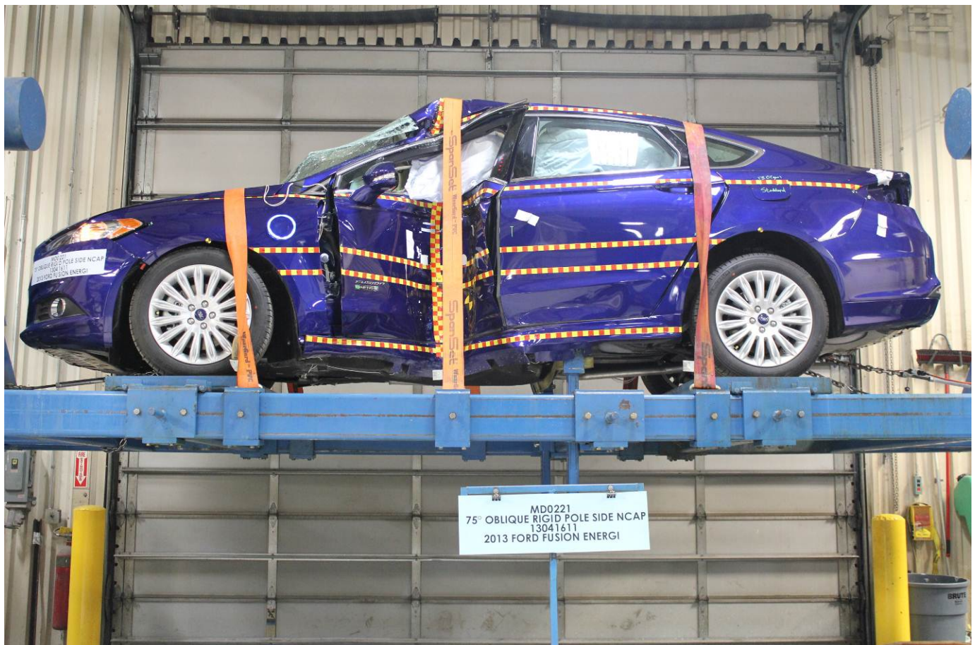
FMVSS No. 301 Static Rollover 0 Degrees
