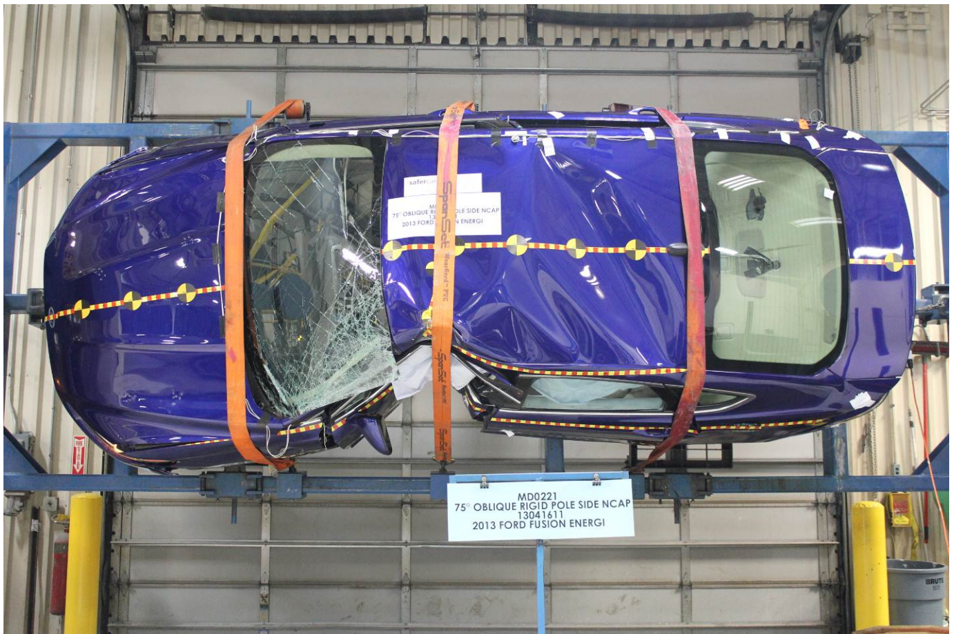
FMVSS No. 301 Static Rollover 90 Degrees
