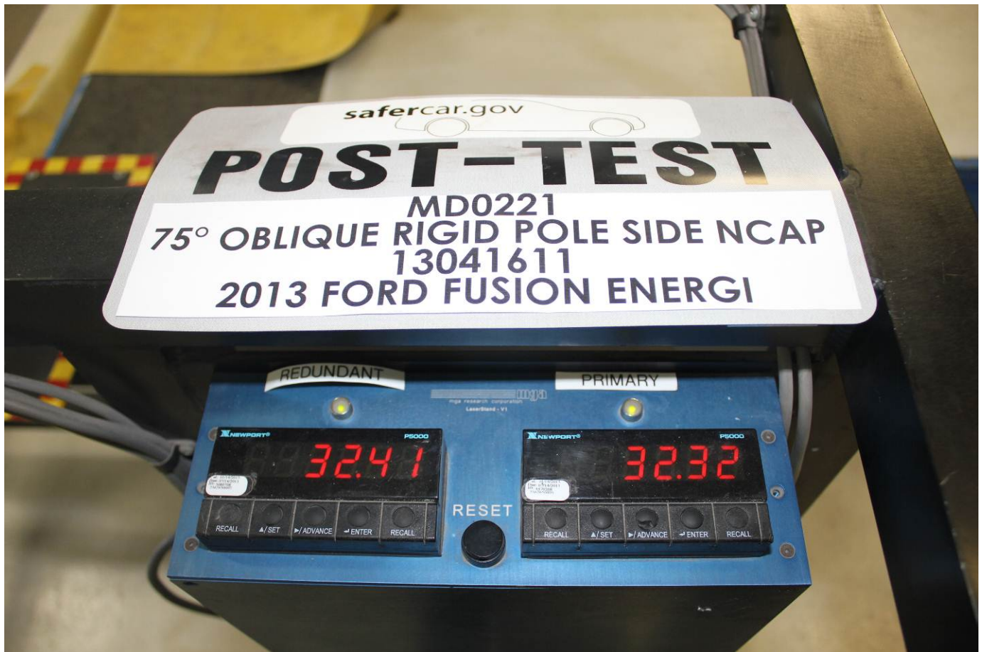
Post-Test Primary and Redundant Speed Trap Read-Out
