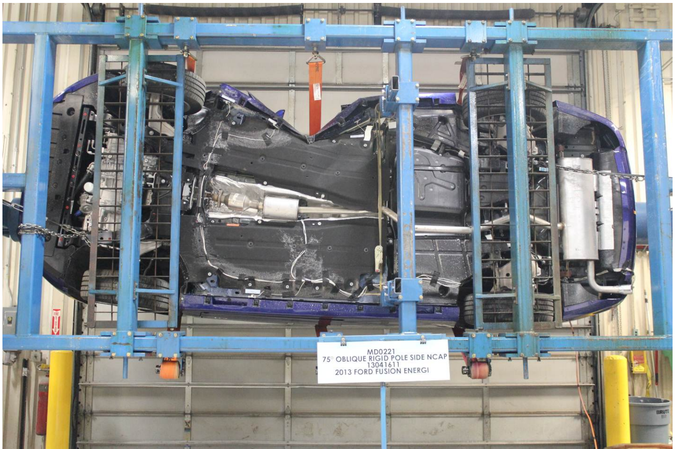
FMVSS No. 301 Static Rollover 270 Degrees
