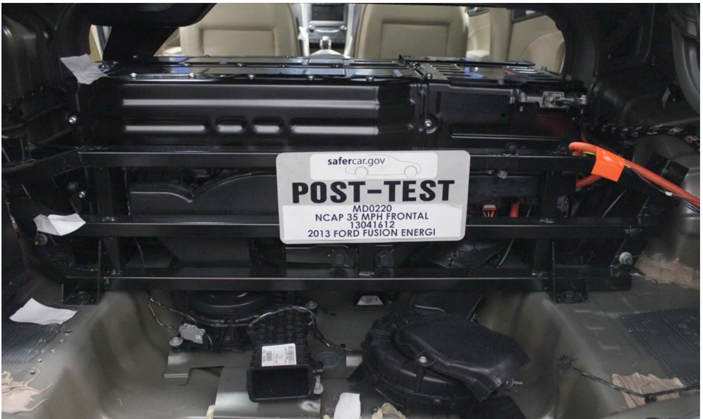
No. 011 Post-Impact Rear View of Propulsion Battery
