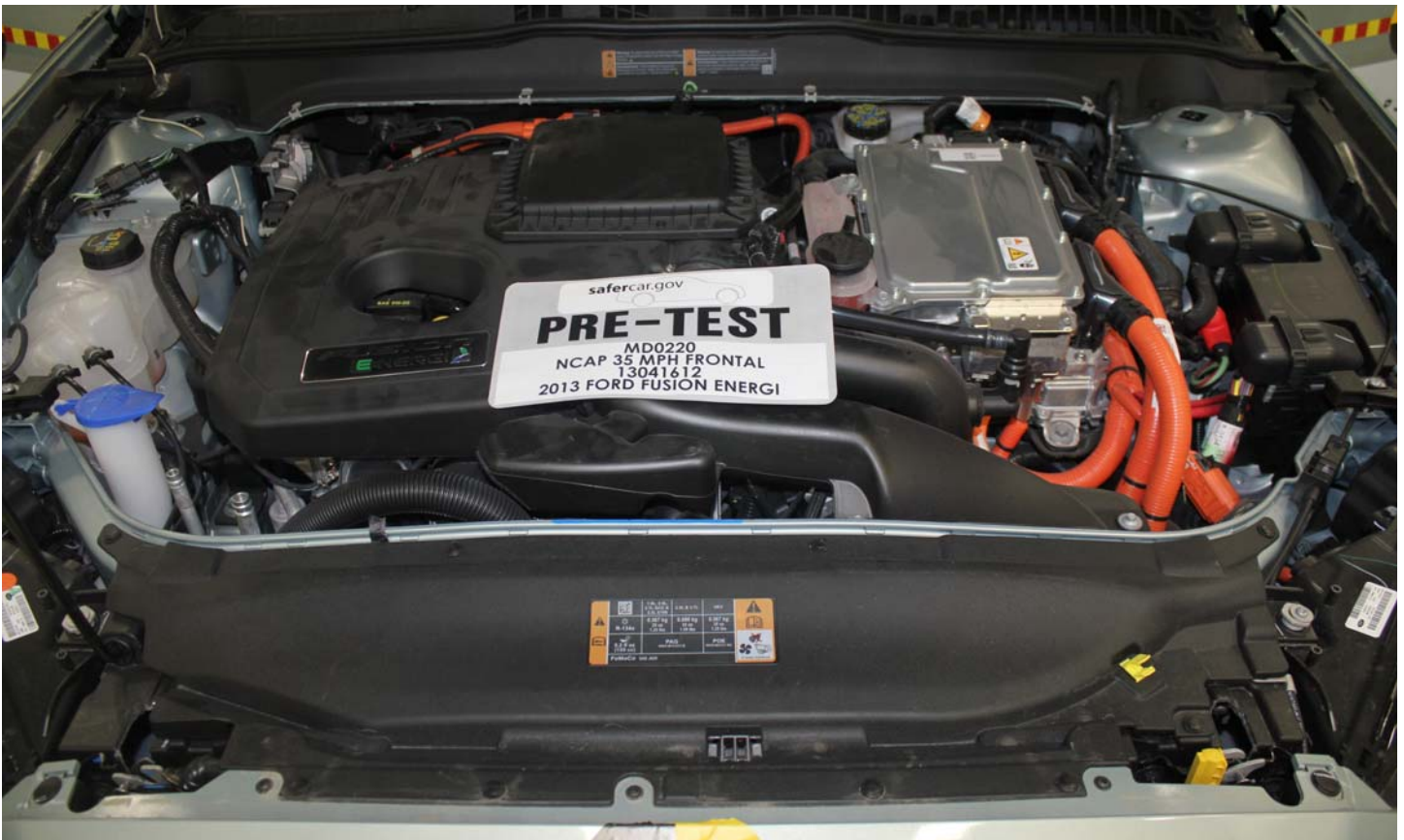
No. 016 Pre-Impact View of Electric Propulsion Drive
