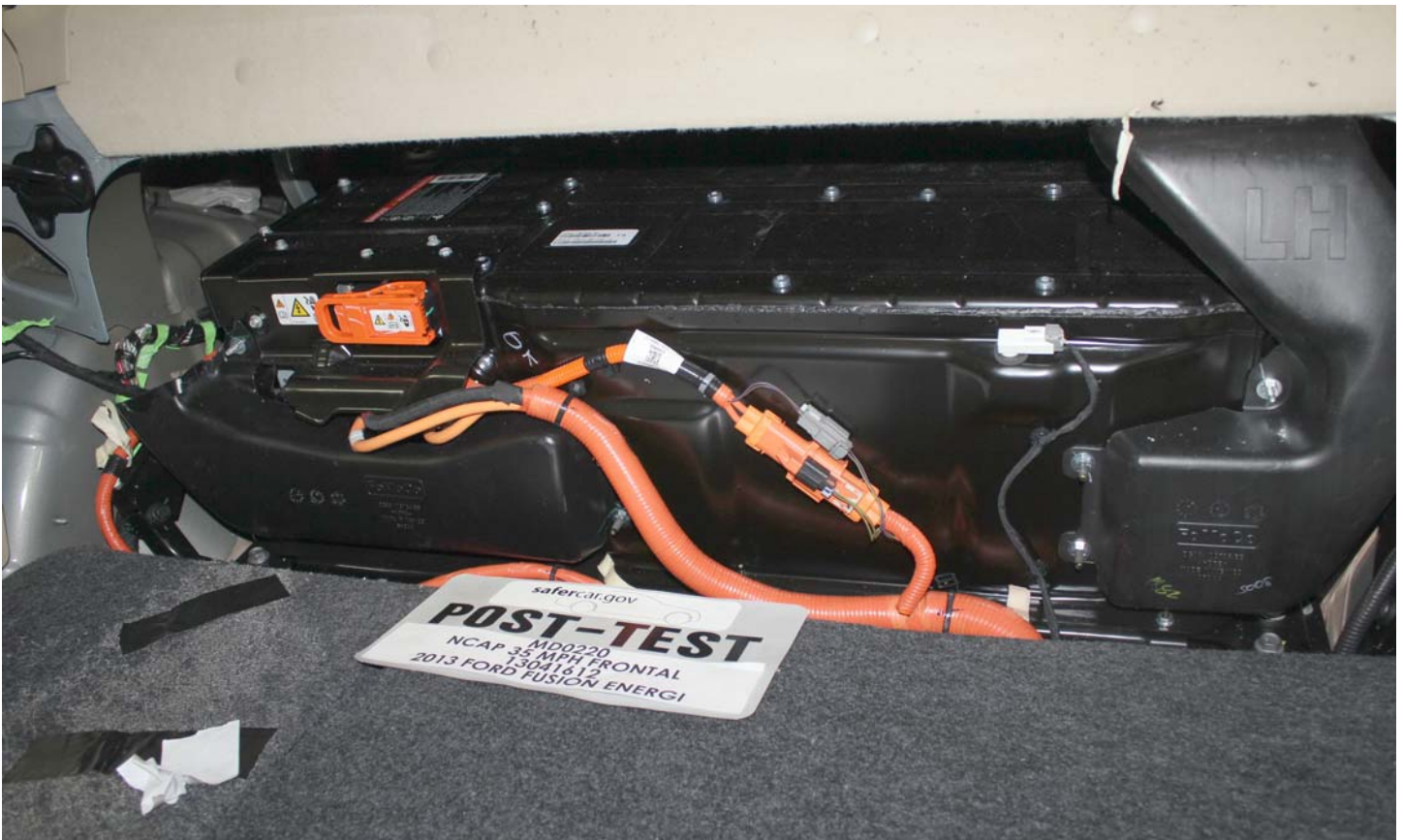
No. 010 Post-Impact Front View of Propulsion Battery
