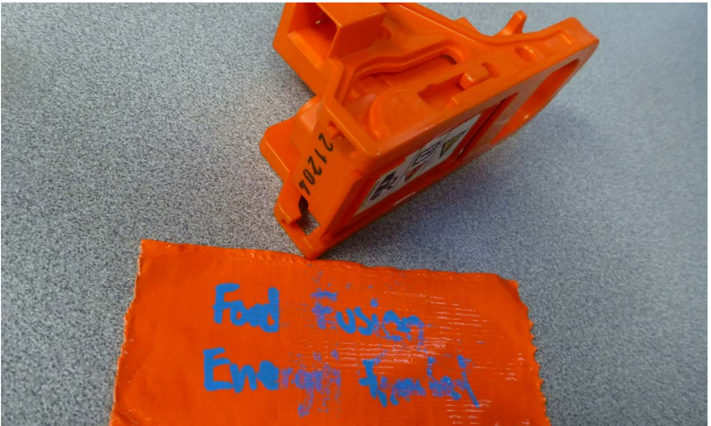
No. 008 Manual High Voltage Service Disconnect Removed
