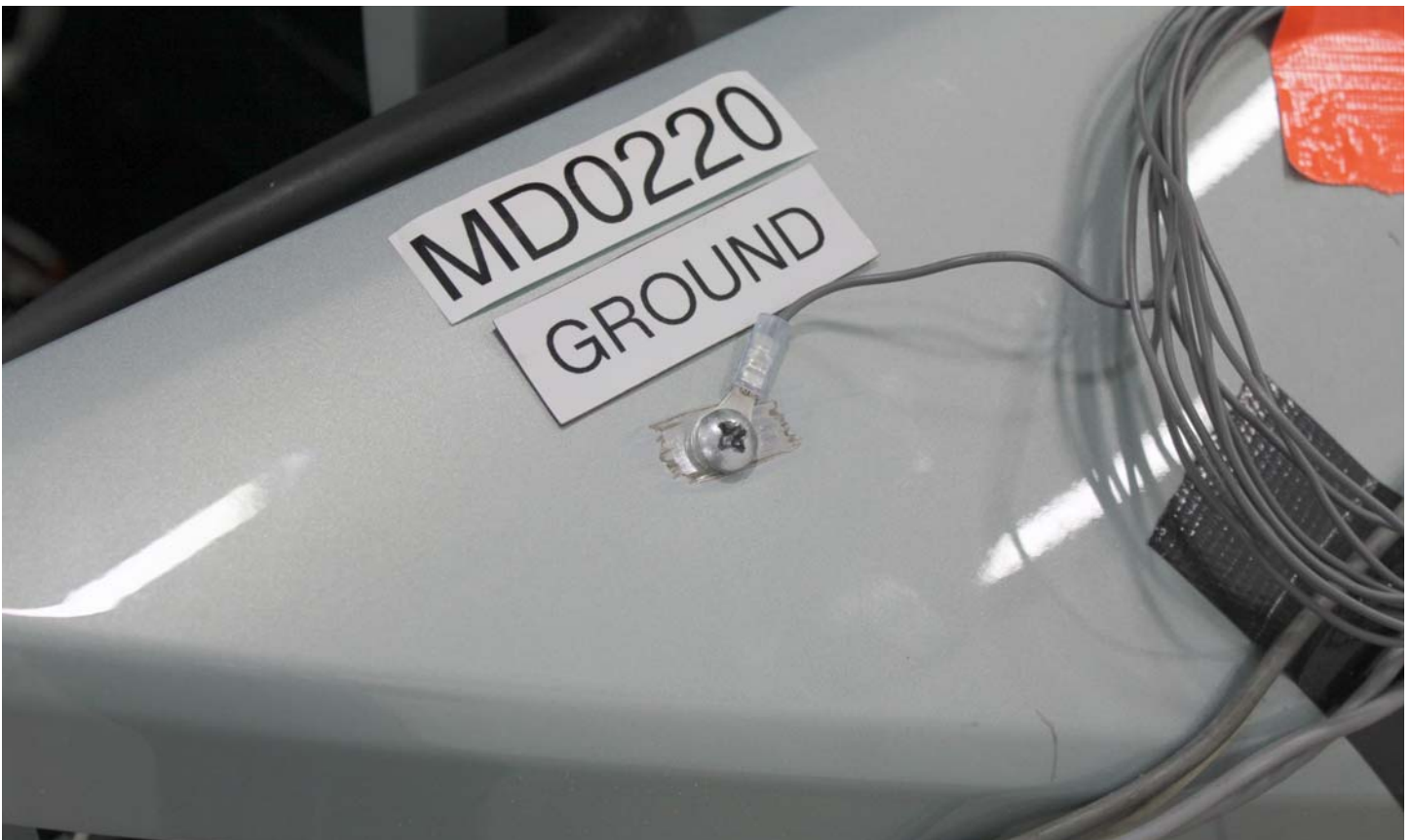
No. 021 Pre-Impact View of Ground Lead Attached
