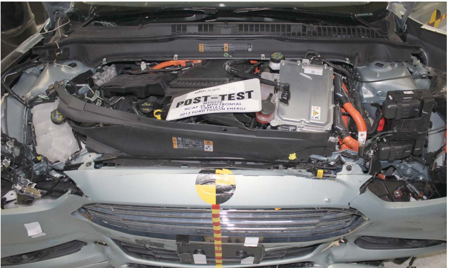
No. 017 Post-Impact View of Electric Propulsion Drive
