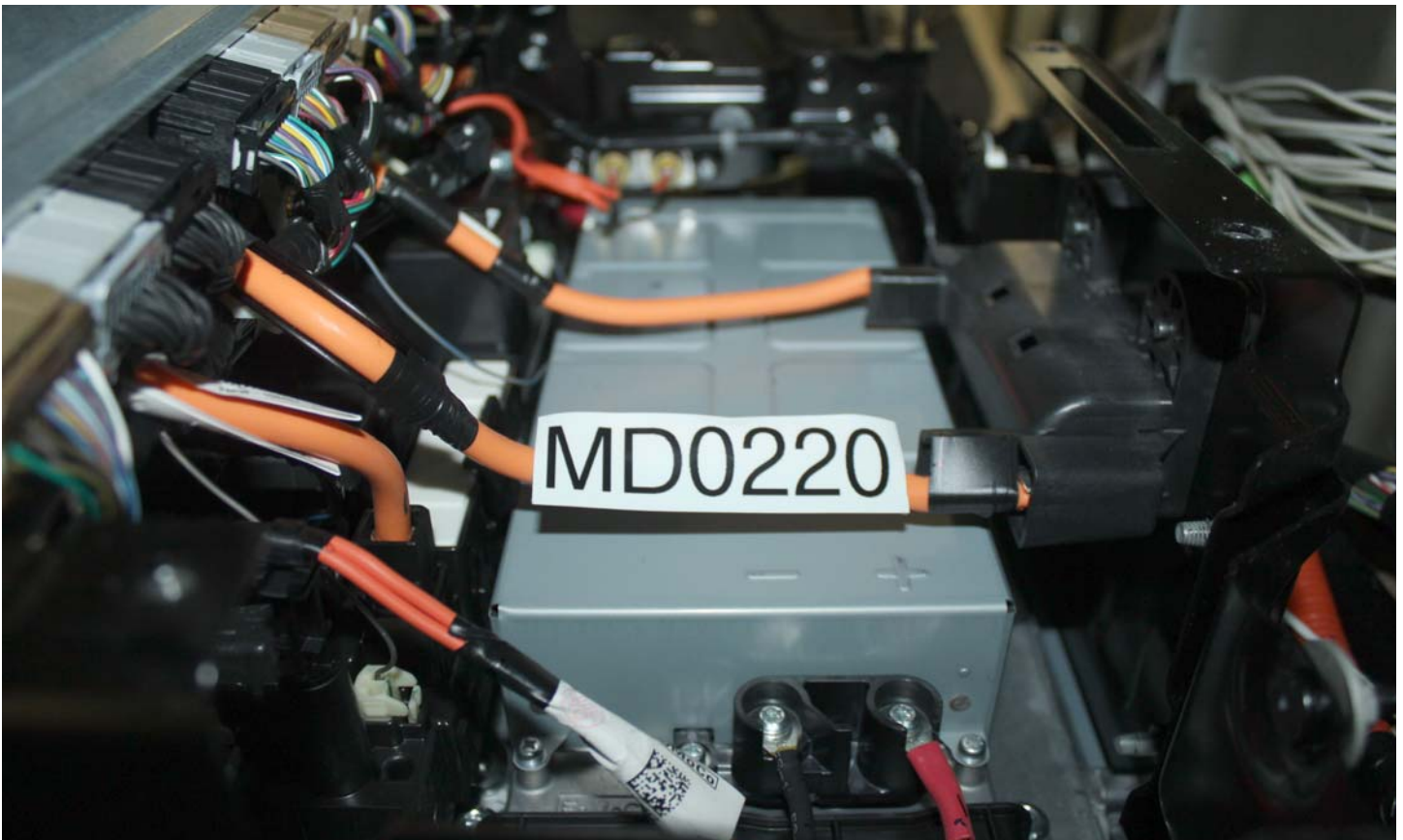
No. 018 Pre-Impact View of High Voltage Interconnect(s)
