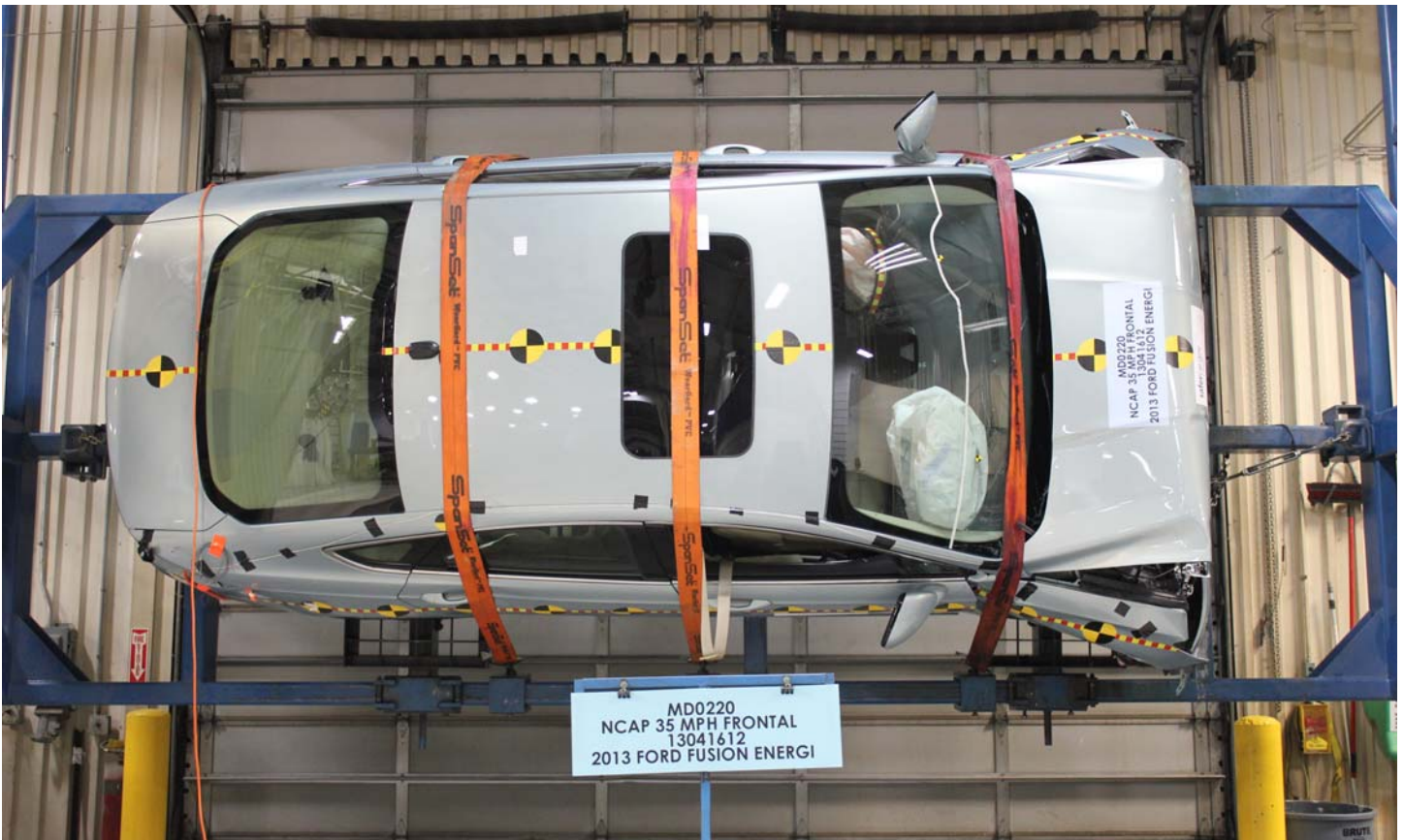
No. 030 FMVSS No. 305 Static Rollover at 270°
