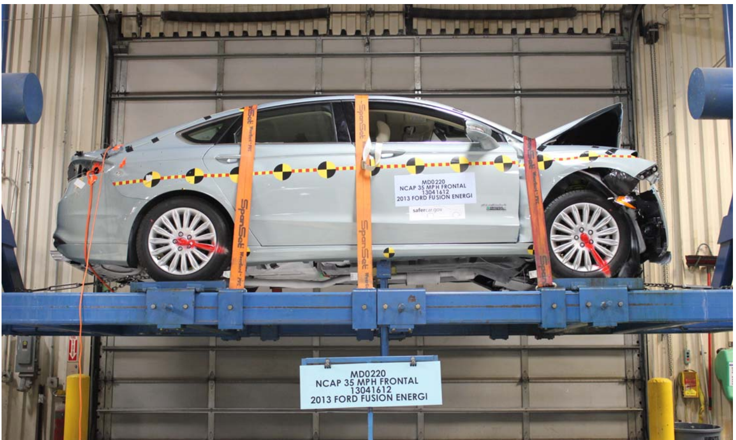
No. 031 FMVSS No. 305 Static Rollover at 360°
