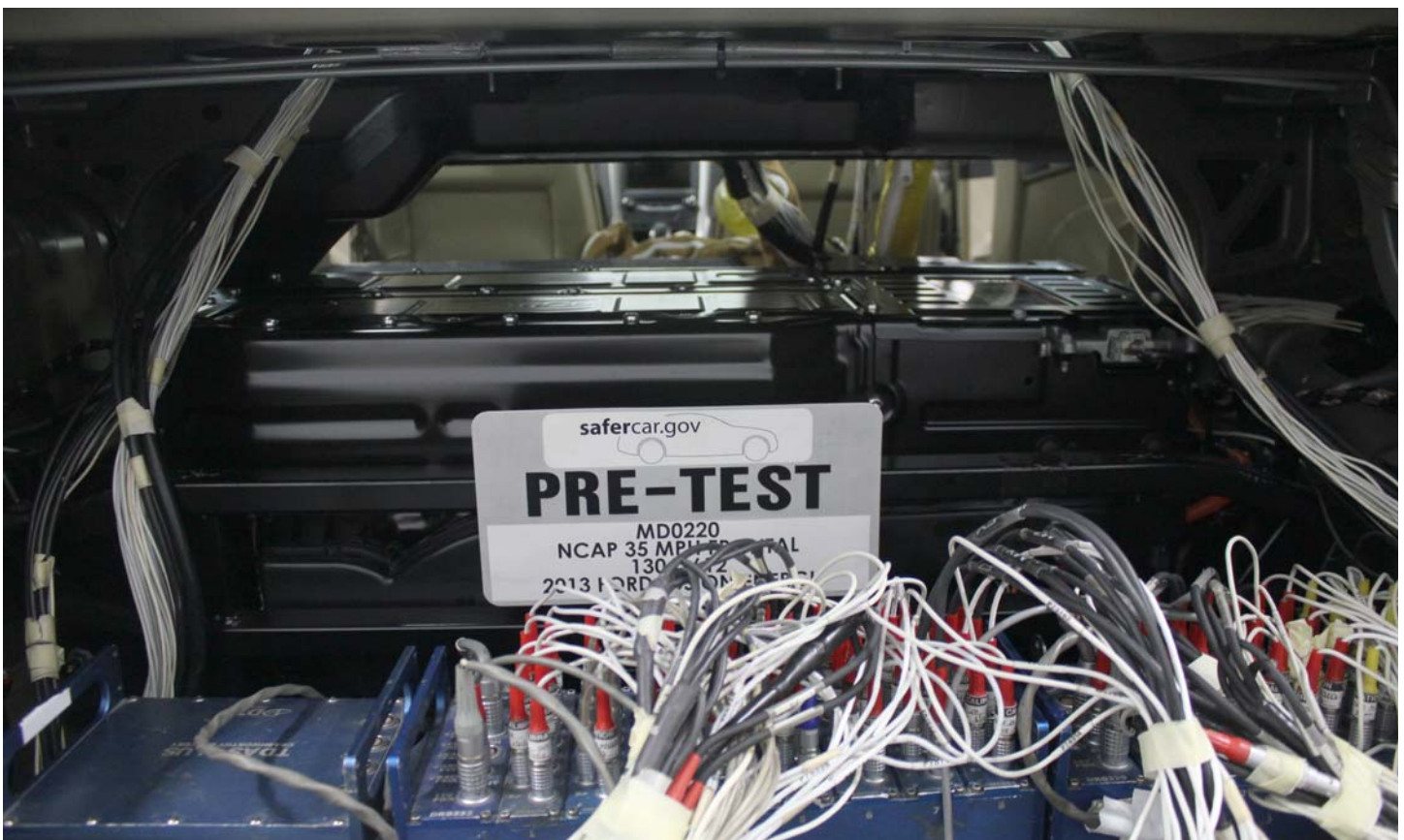
No. 009 Pre-Impact View of Propulsion Battery
