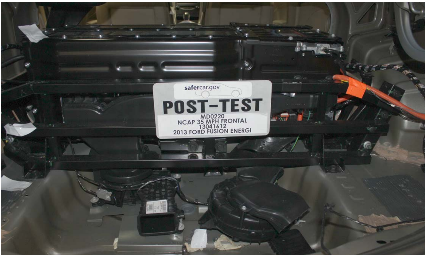
No. 013 Post-Impact View of Battery Box(s) or Container(s) Which Holds Individual Battery Modules
