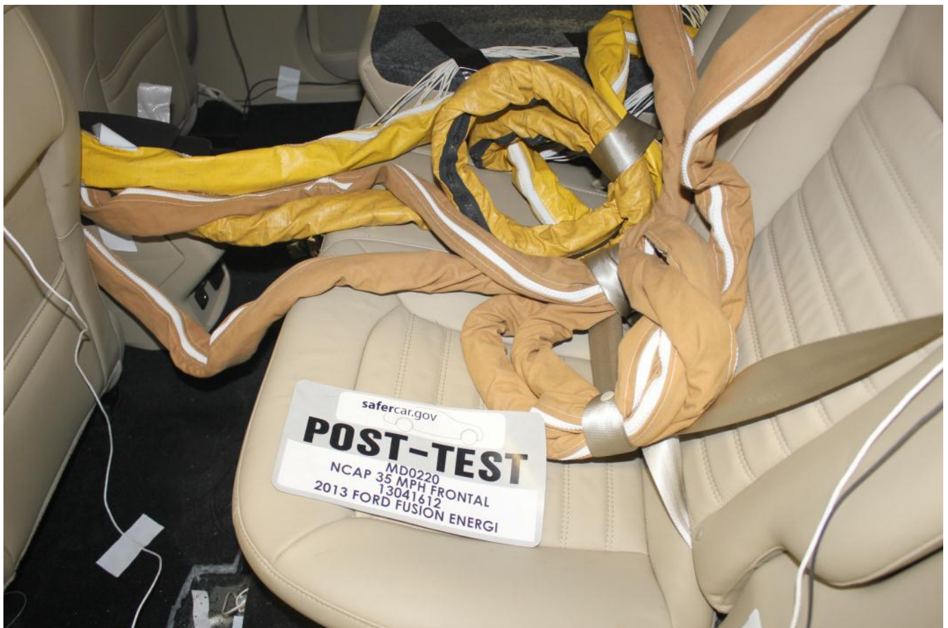
Post-Test Dummy Cable Routing
