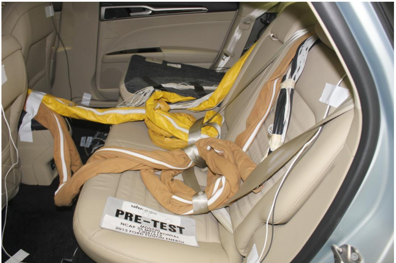
Pre-Test Dummy Cable Routing
