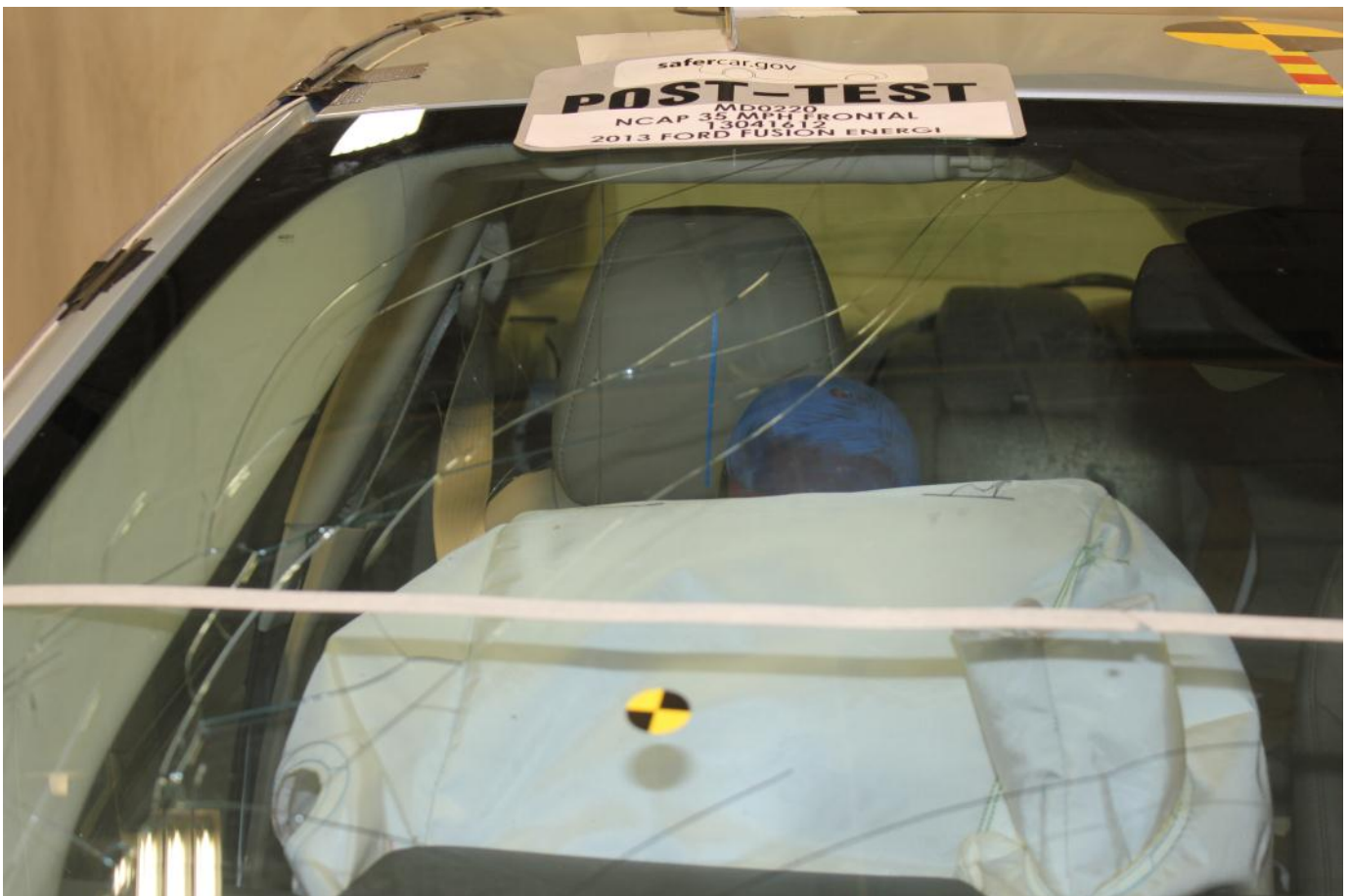
Post-Test Passenger Dummy Front View
