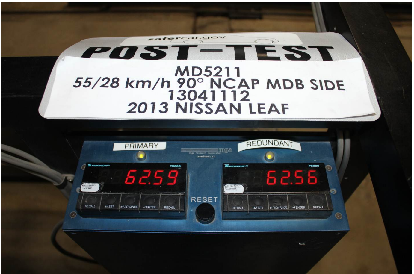
Post-Test Primary and Redundant Speed Trap Read-Out
