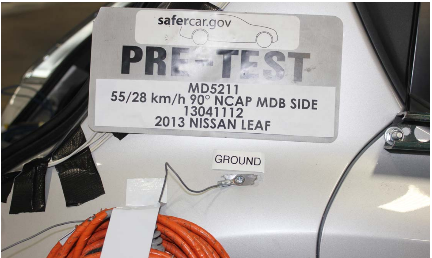
No. 021 Pre-Impact View of Ground Lead Attached
