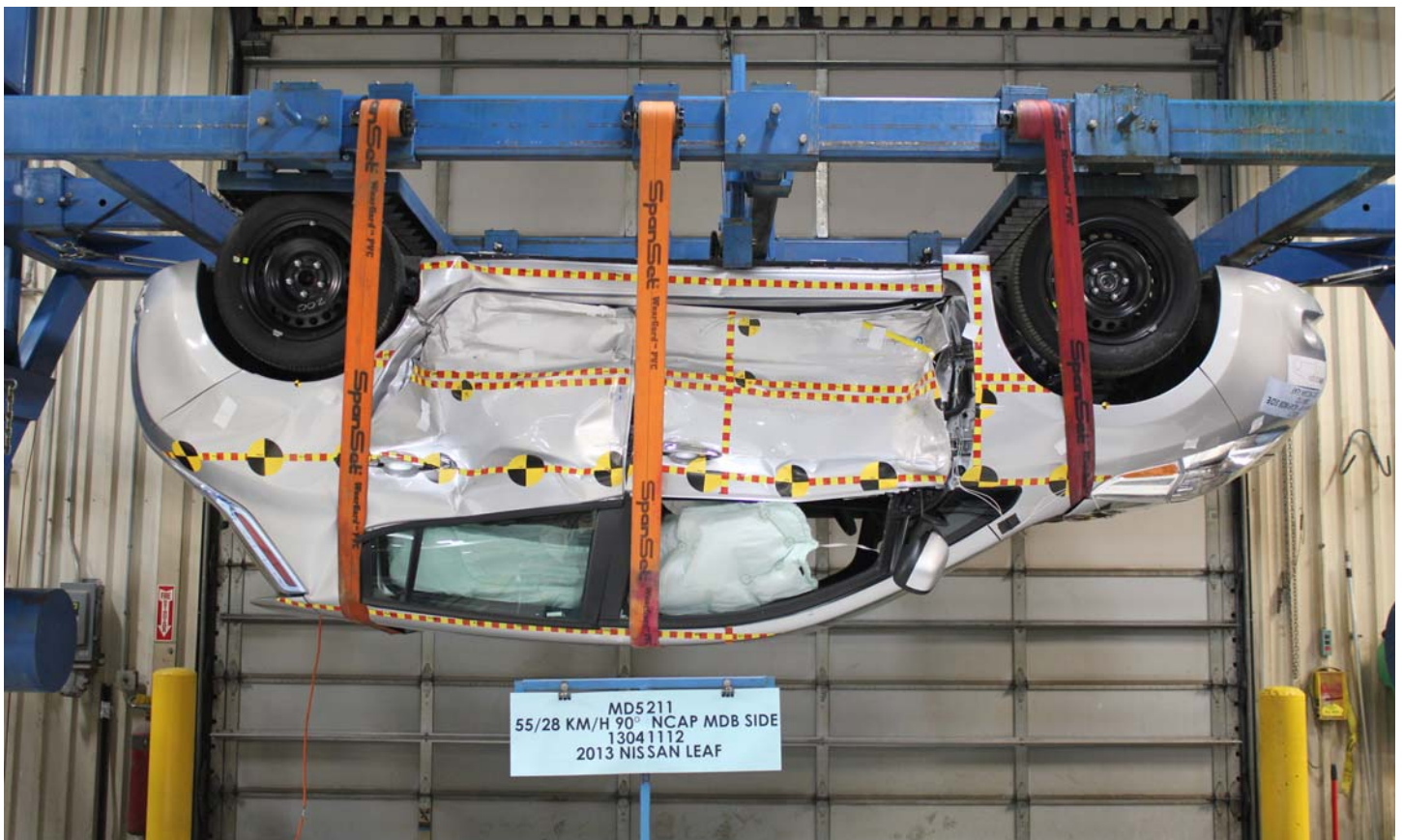
No. 029 FMVSS No. 305 Static Rollover at 180°
