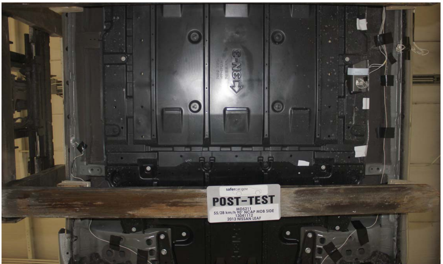
No. 010 Post-Impact Front View of Propulsion Battery
