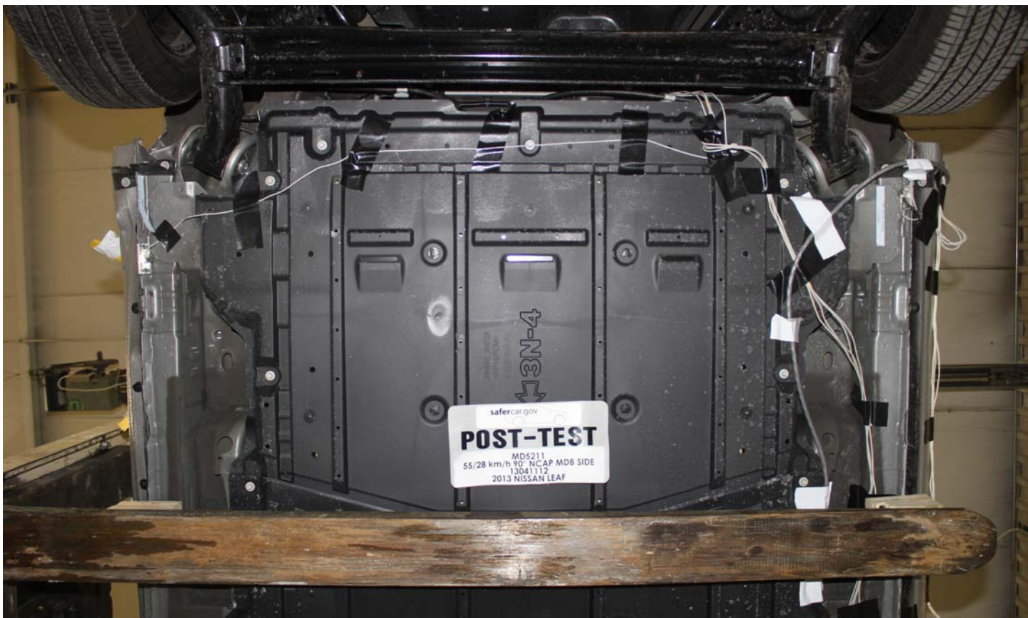
No. 011 Post-Impact Rear View of Propulsion Battery
