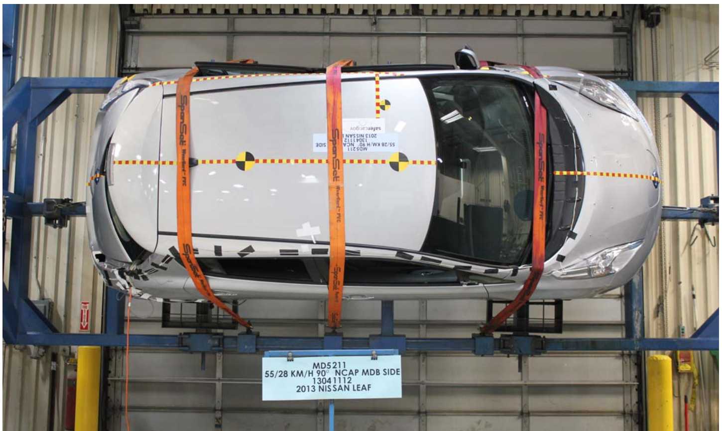
No. 030 FMVSS No. 305 Static Rollover at 270°
