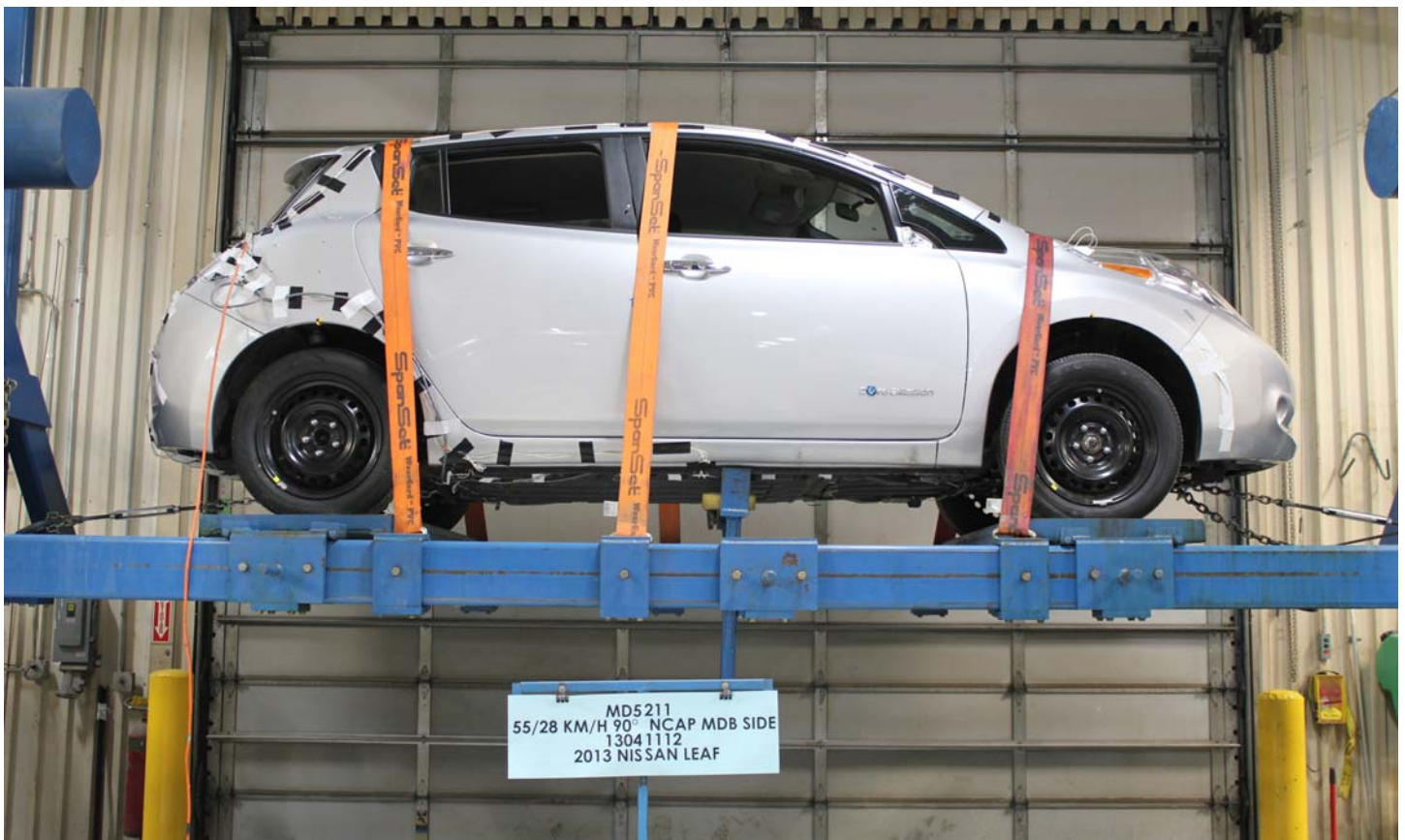
No. 031 FMVSS No. 305 Static Rollover at 360°
