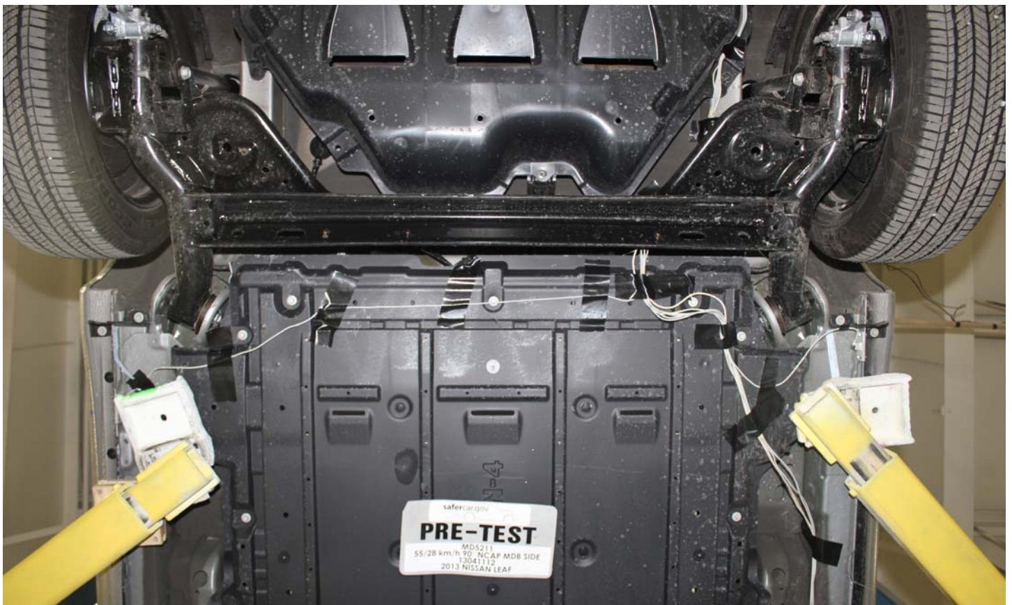
No. 009a Pre-Impact View of Propulsion Battery
