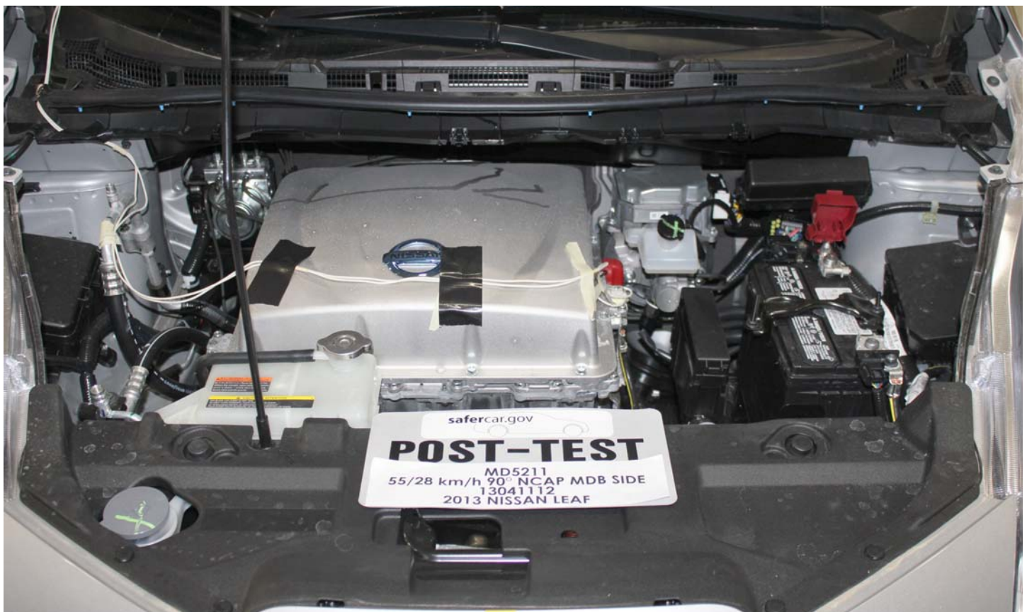
No. 017 Post-Impact View of Electric Propulsion Drive
