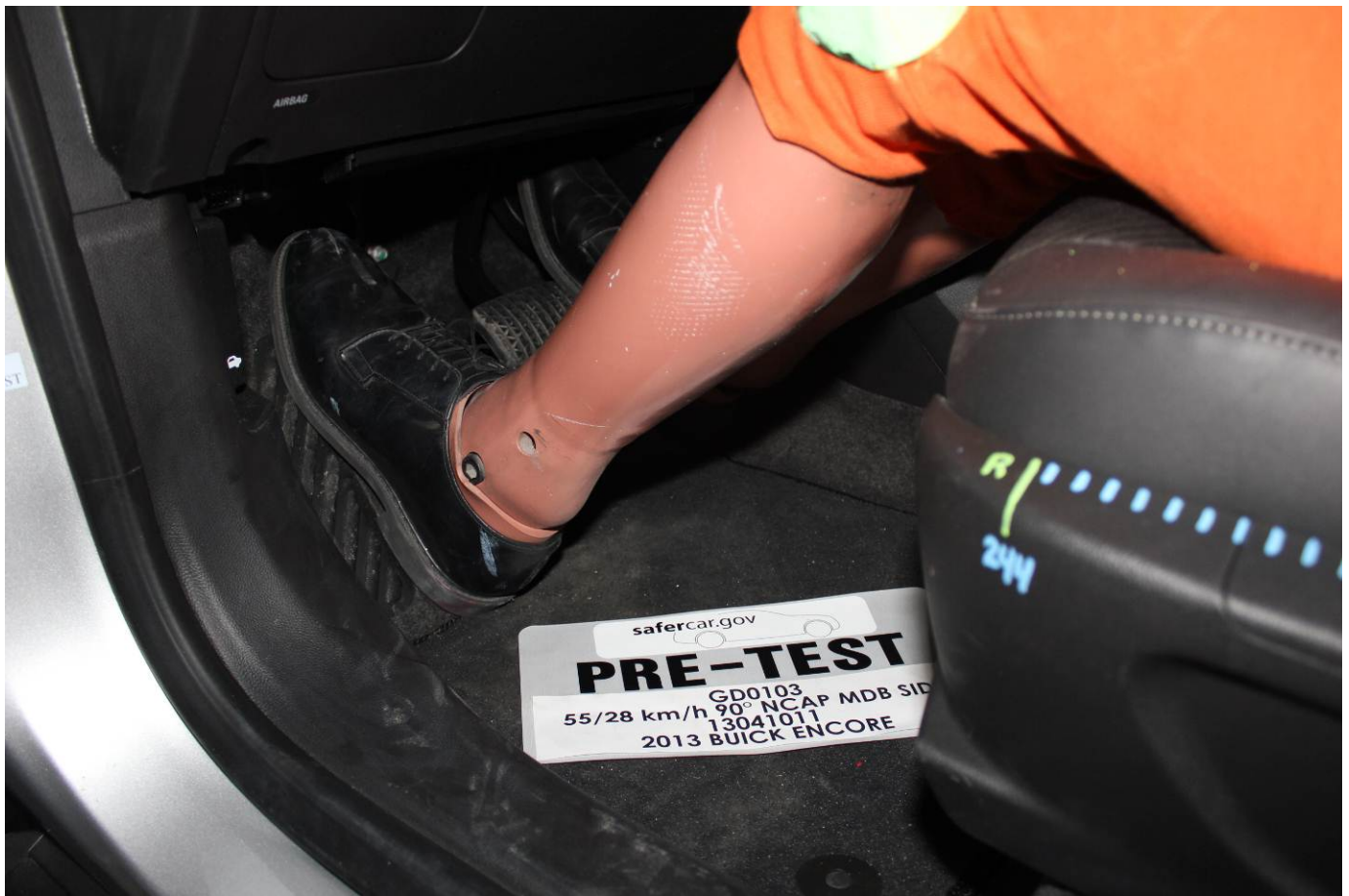
Pre-Test Placement of Driver Dummy's Feet
