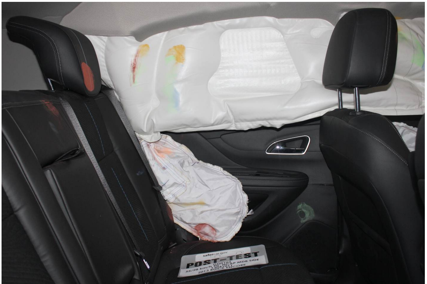
Post-Test Rear Passenger Inner Door Panel View
