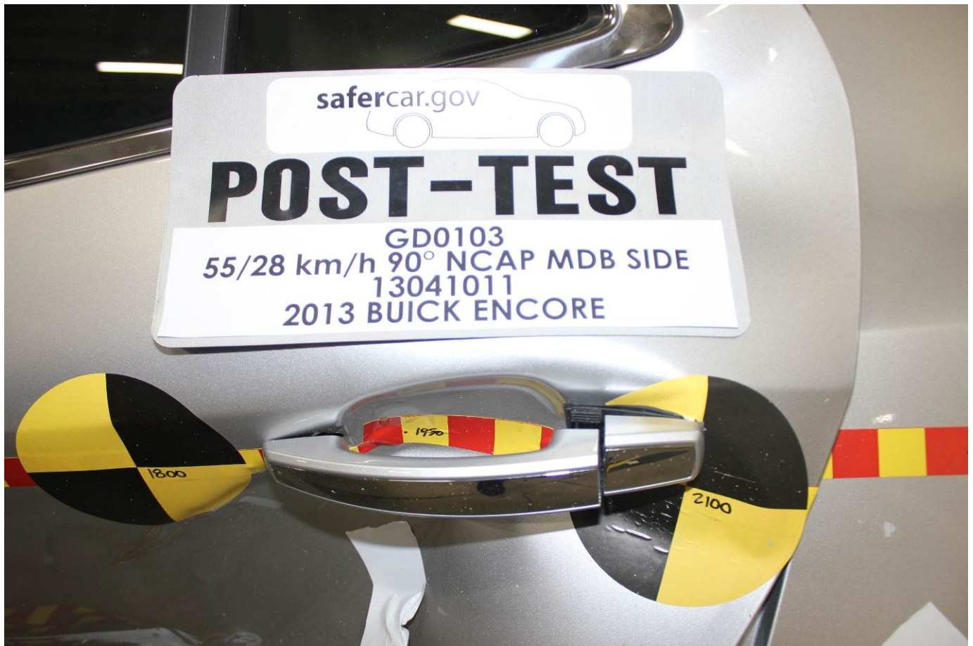
Post-Test Left Rear Door Latch Close-Up
