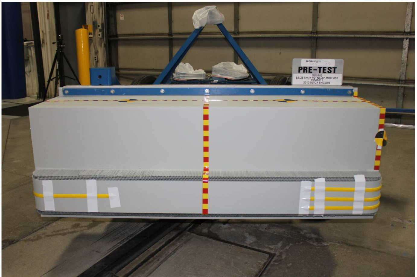
Pre-Test Front View of MDB Impactor Face
