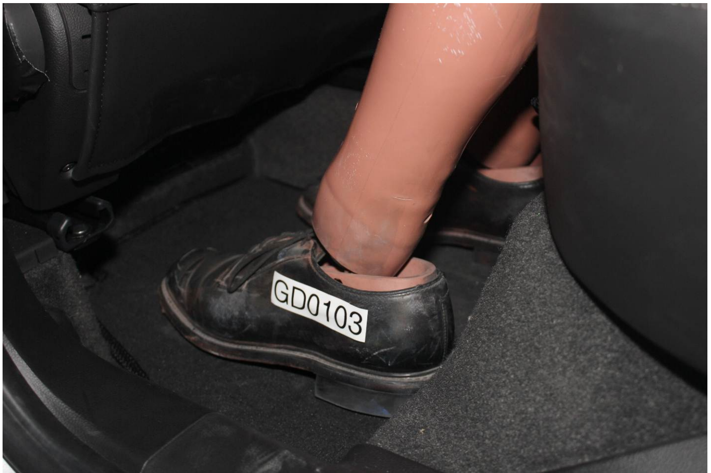
Pre-Test Placement of Rear Passenger Dummy's Feet
