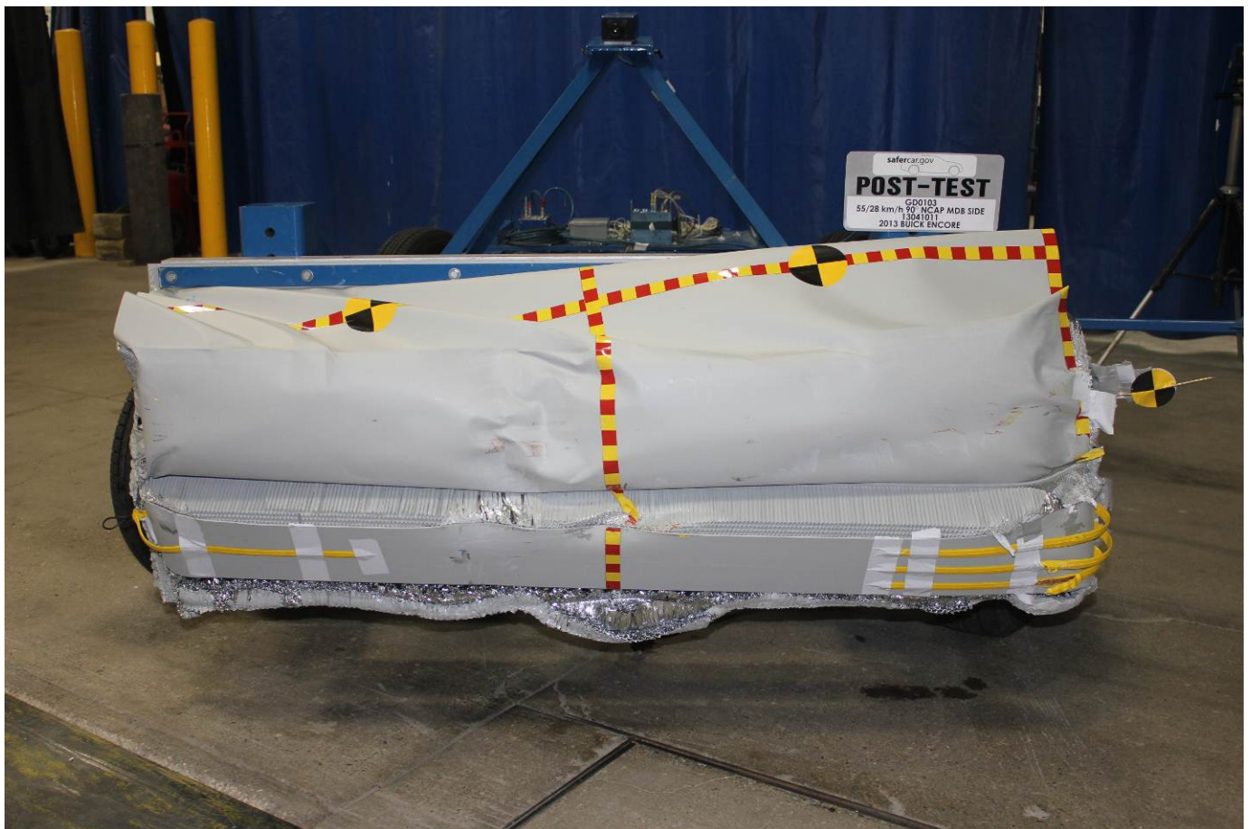
Post-Test Front View of MDB Impactor Face
