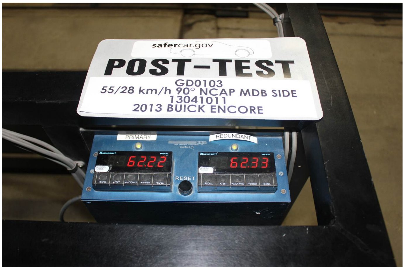
Post-Test Primary and Redundant Speed Trap Read-Out
