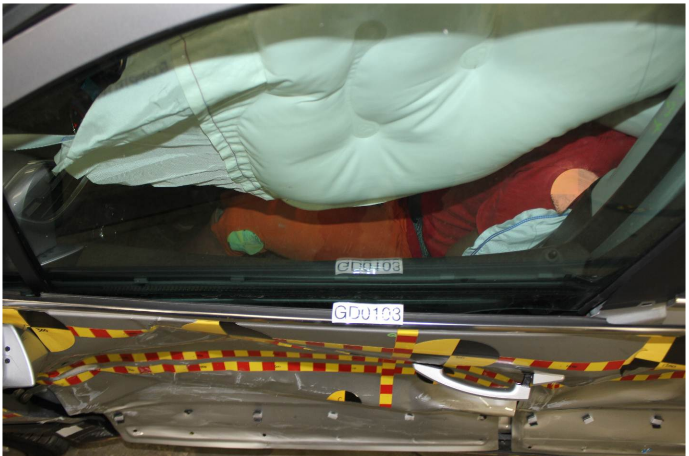
Post-Test Driver Dummy and Door Clearance View
