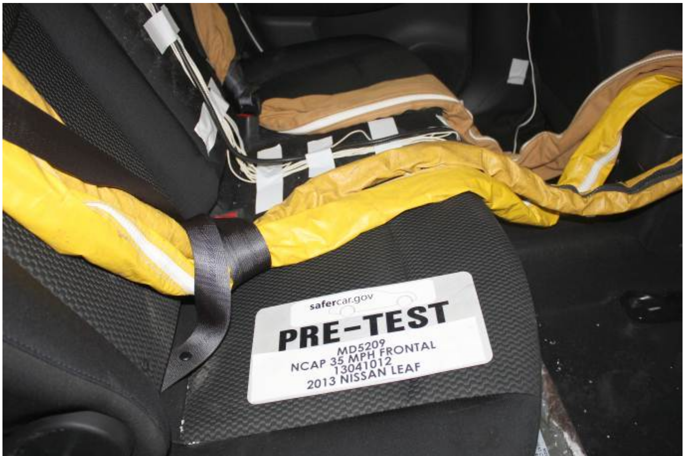
Pre-Test Dummy Cable Routing
