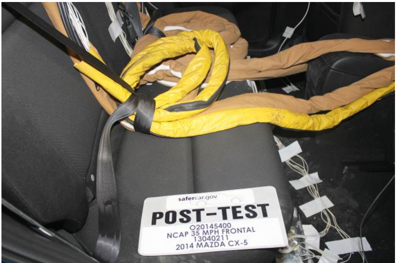
Post-Test Dummy Cable Routing
