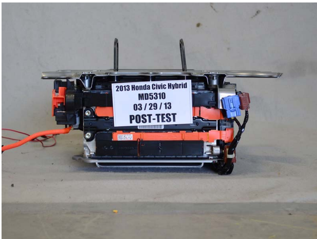
FIGURE 15b. Post-Impact View of Propulsion Battery Modules
