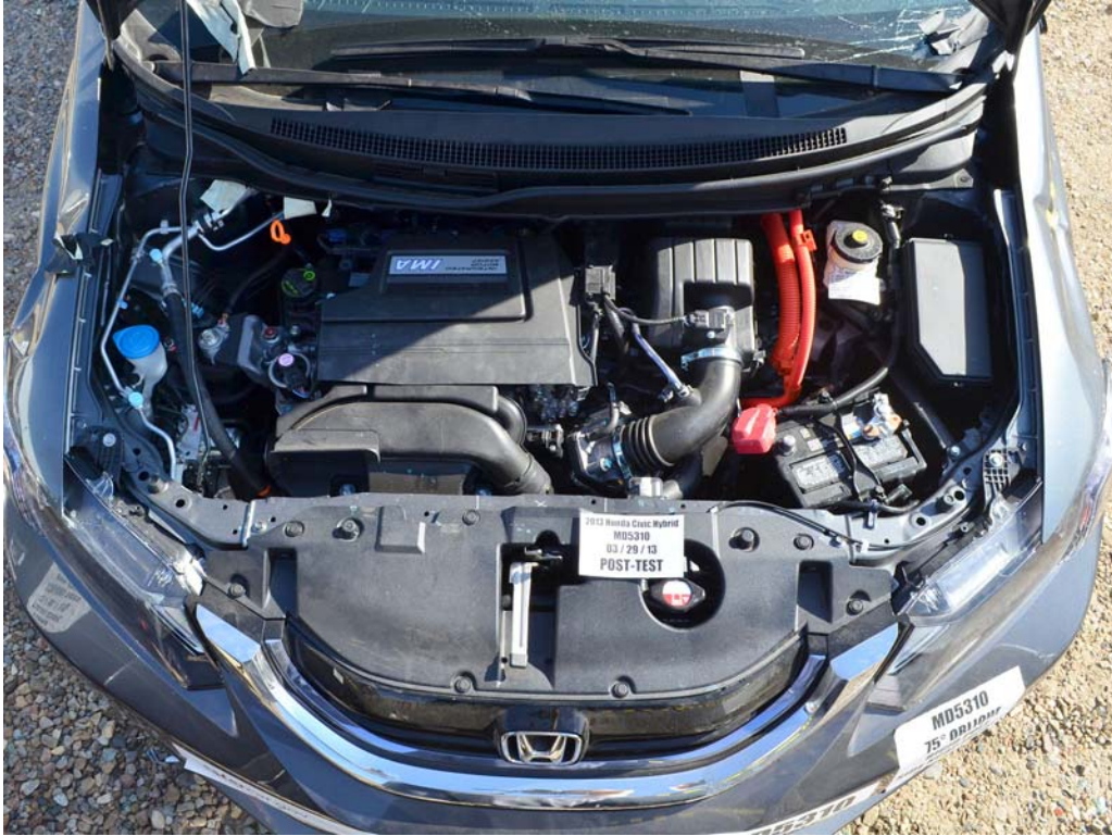
FIGURE 17. Post-Impact View of Electric Propulsion Drive
