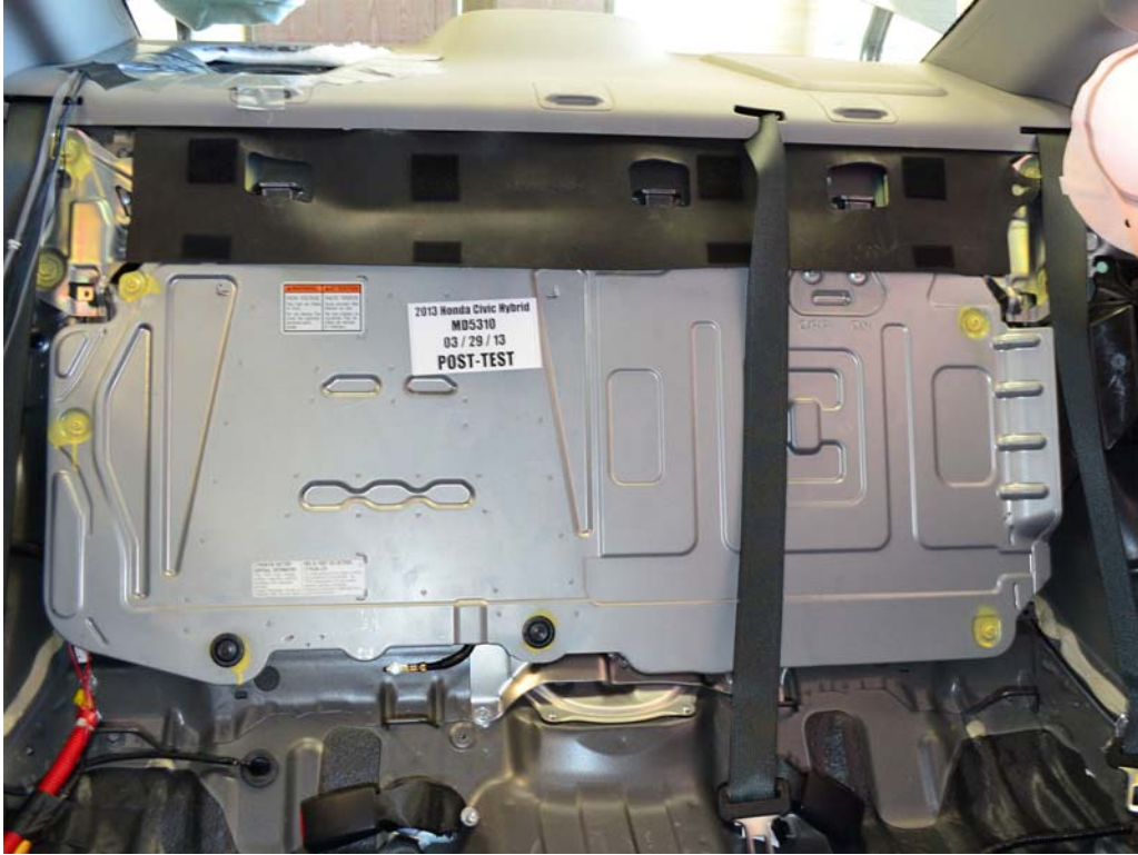
FIGURE 10. Post-Impact Front View of Propulsion Battery
