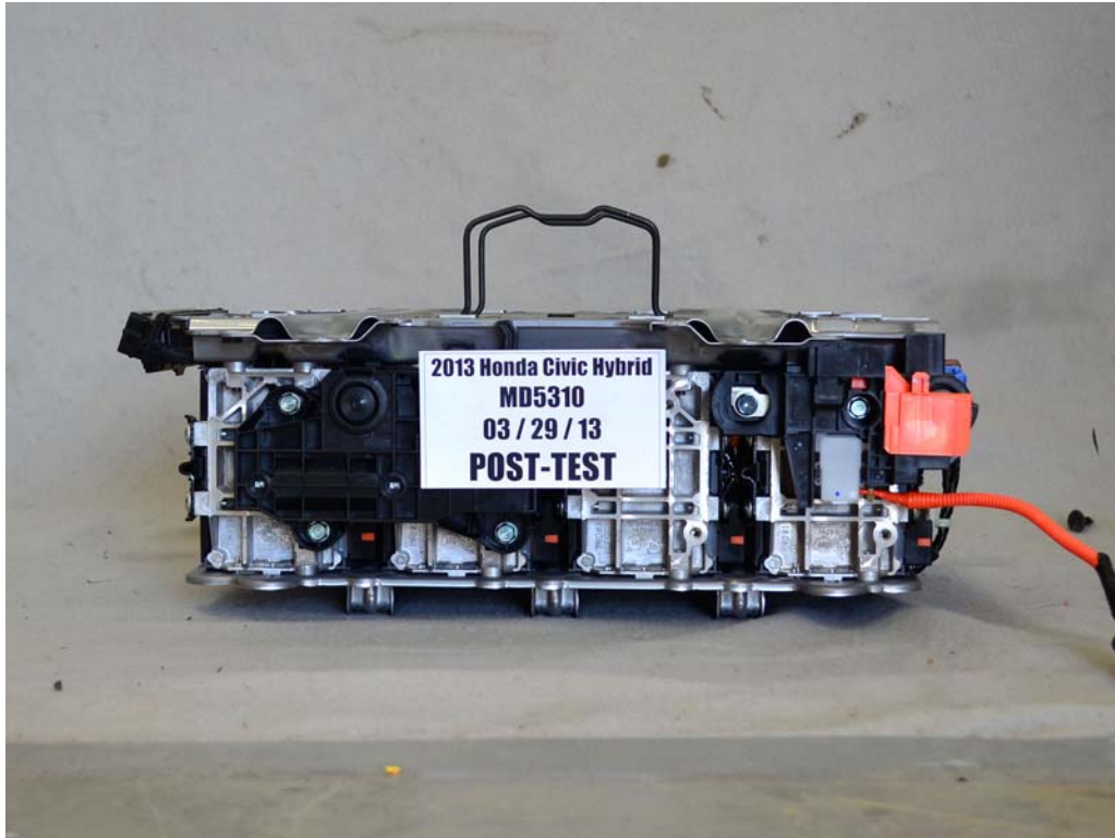
FIGURE 15c. Post-Impact View of Propulsion Battery Modules
