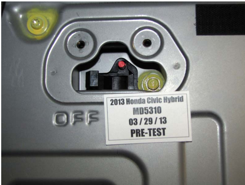
FIGURE 8. Manual High Voltage Service Disconnect Removed
