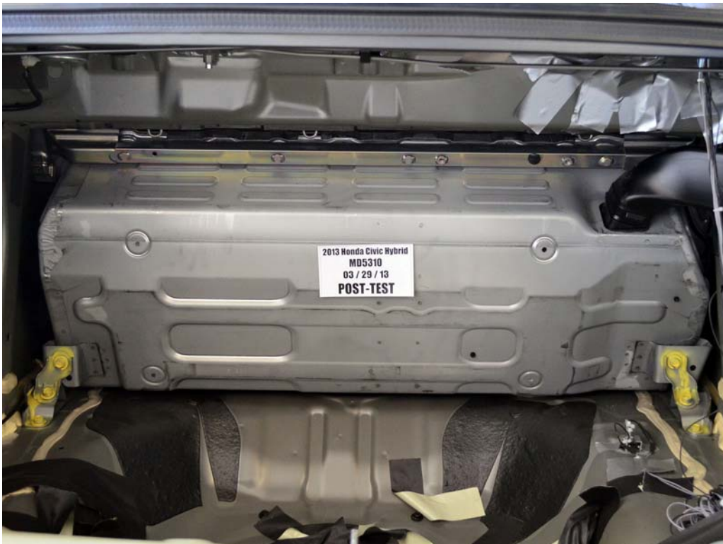
FIGURE 11. Post-Impact Rear View of Propulsion Battery
