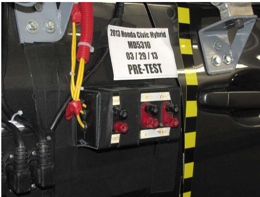
FIGURE 24. Pre-Impact View of Installed Test Interface Port
