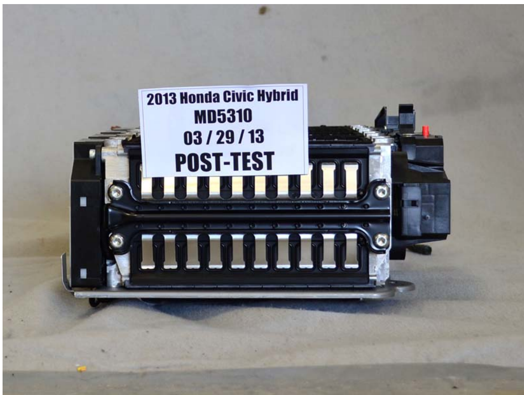
FIGURE 15d. Post-Impact View of Propulsion Battery Modules
