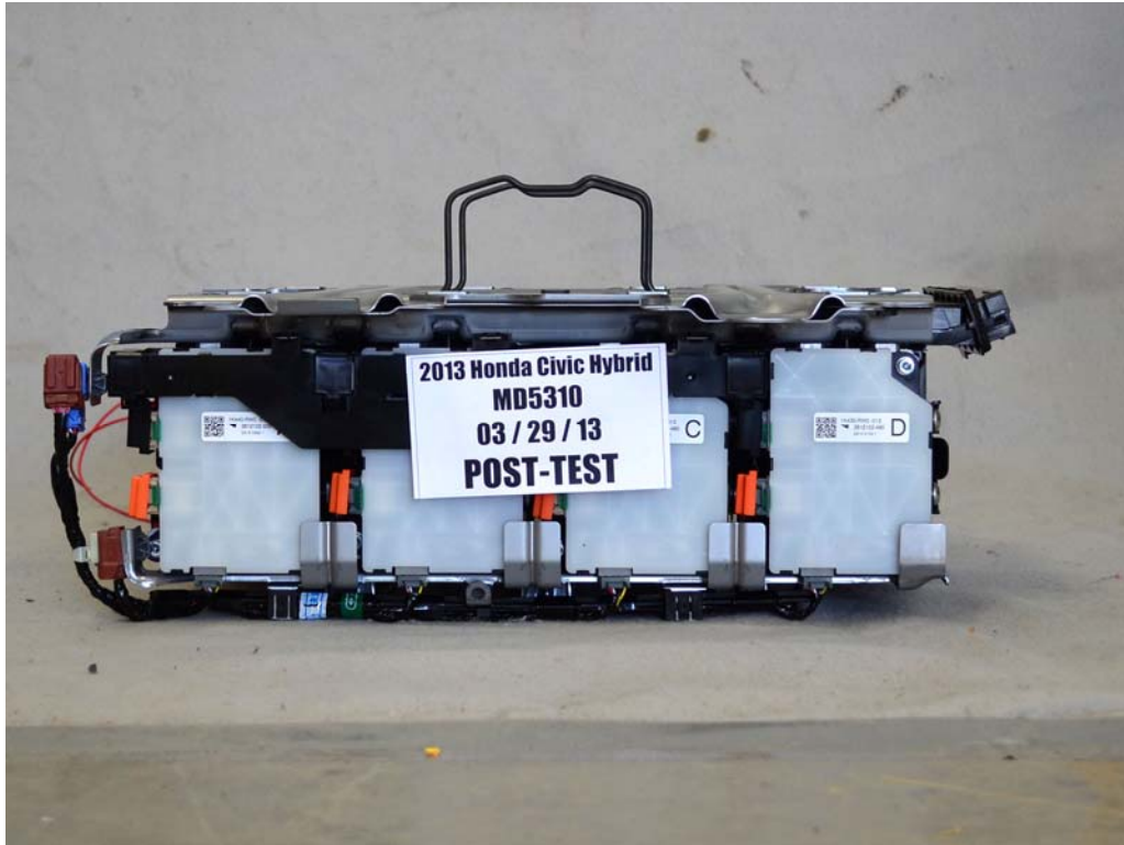
FIGURE 15a. Post-Impact View of Propulsion Battery Modules
