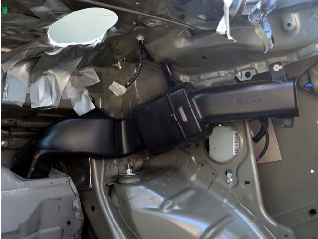
FIGURE 19b. Pre-Impact View of Propulsion Battery Venting System
