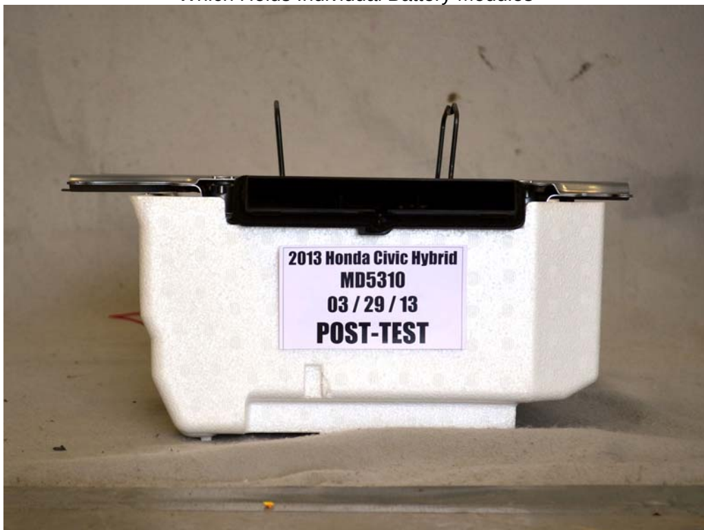
FIGURE 13e. Post-Impact View of Battery Box or Container Which Holds Individual Battery Modules
