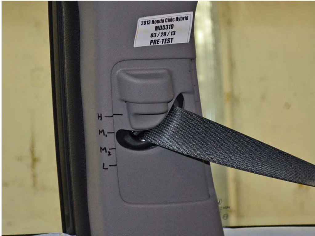
FIGURE 33. Pre-Test View of Belt Anchorage for Dummy
