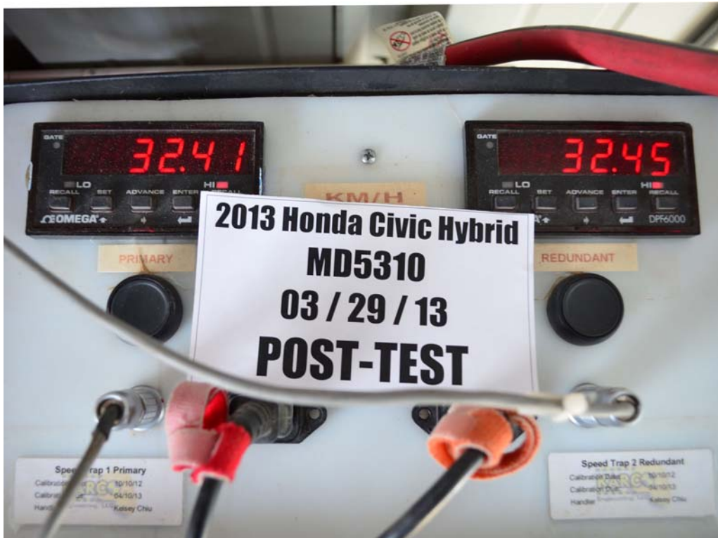
FIGURE 62. Post-Test Primary and Redundant Speed Trap Read-Out
