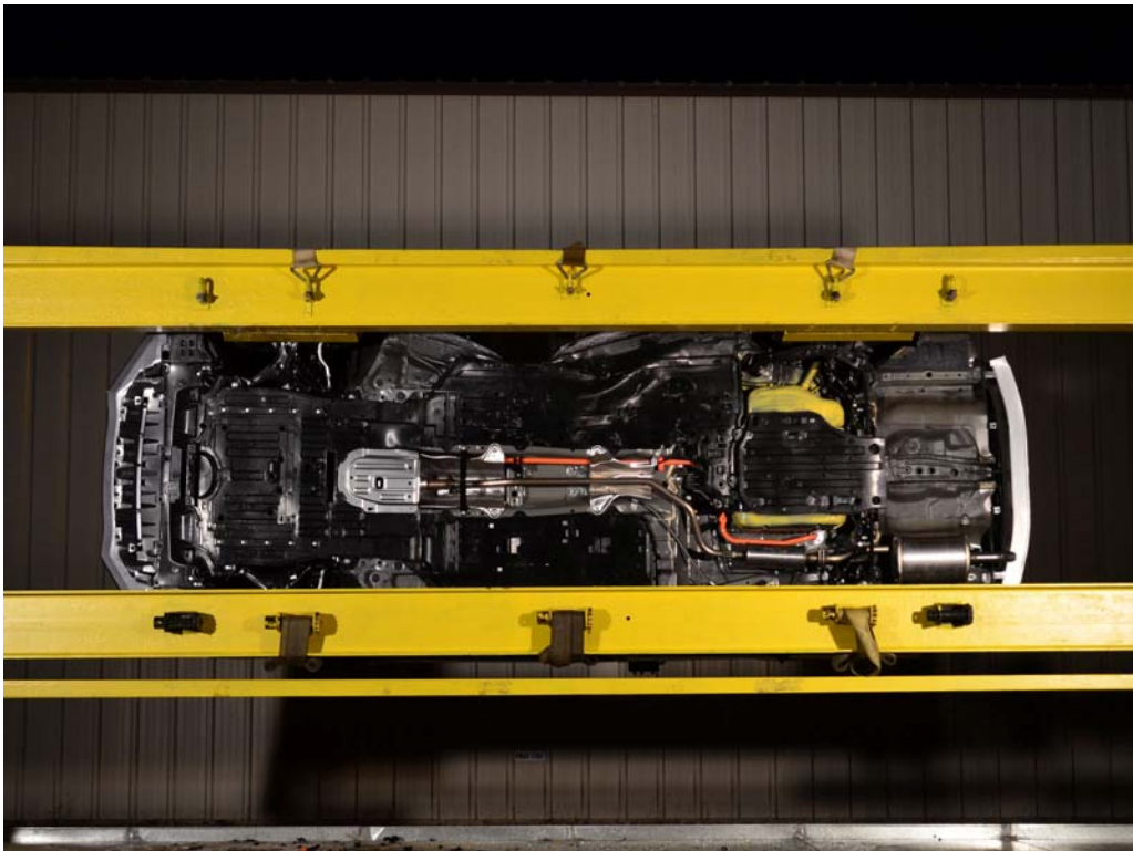
FIGURE 66. FMVSS No. 301 Static Rollover 270 Degrees
