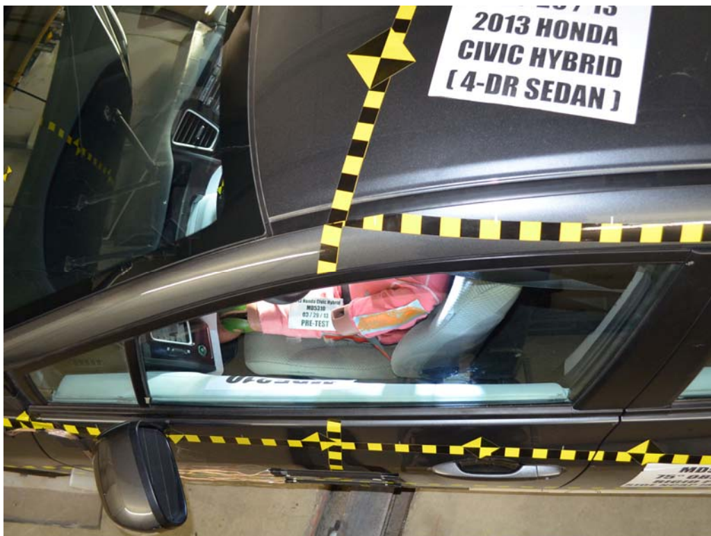
FIGURE 40. Pre-Test Dummy and Door Clearance
