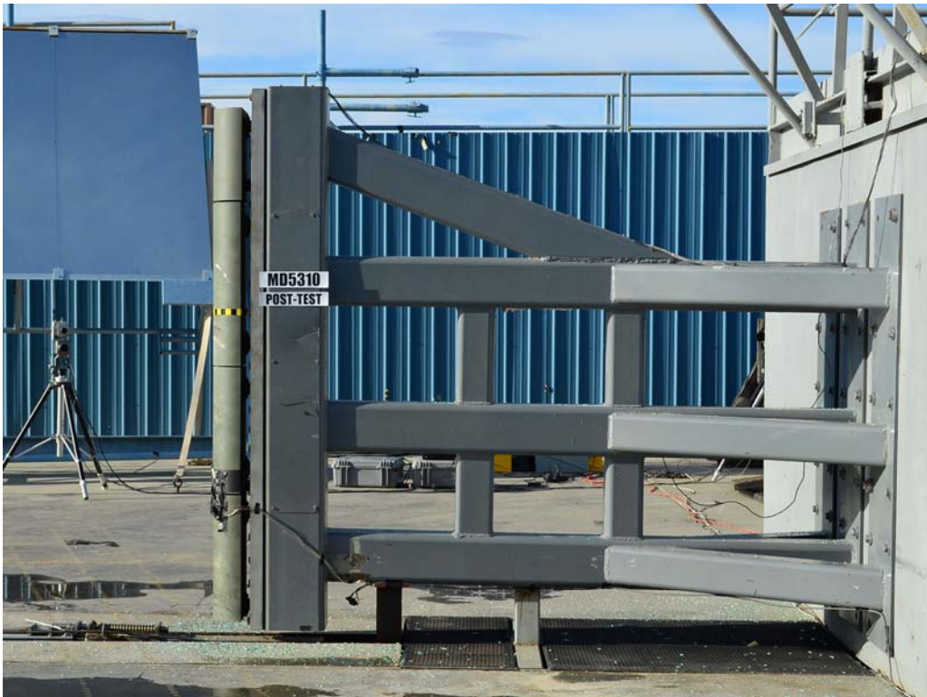
FIGURE 60. Post-Test Pole Barrier Side View
