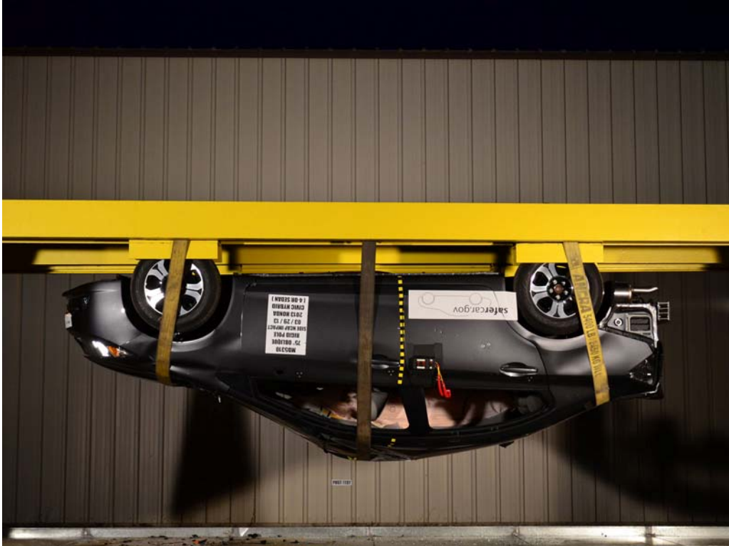
FIGURE 65. FMVSS No. 301 Static Rollover 180 Degrees
