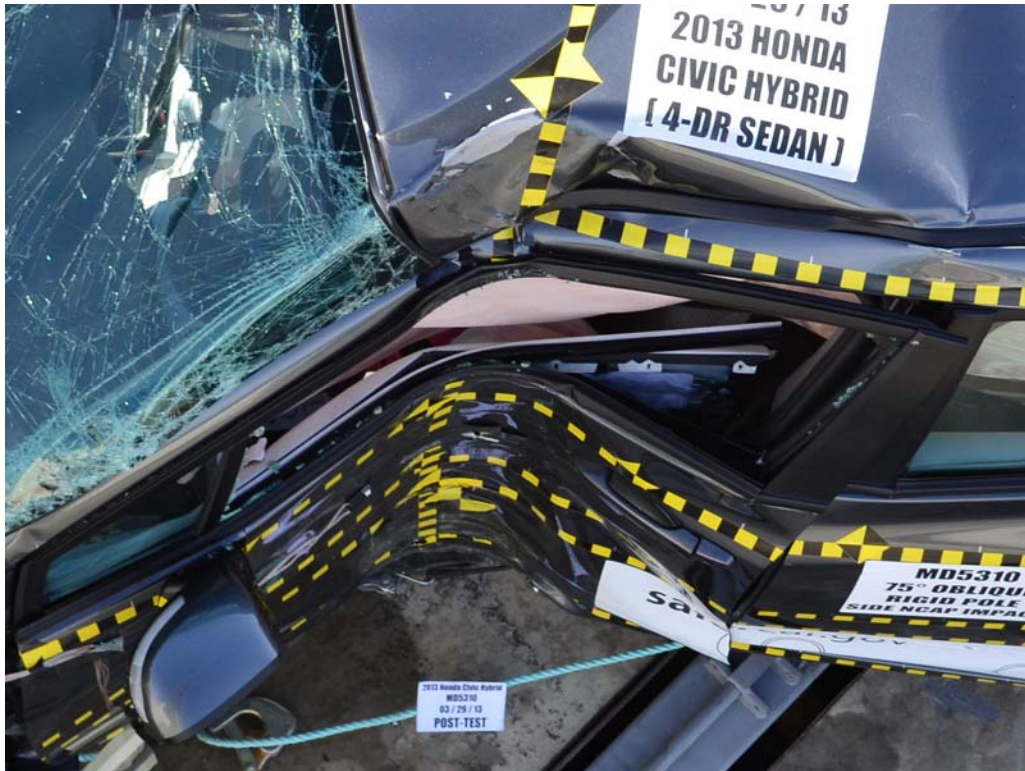
FIGURE 41. Post-Test Dummy and Door Clearance
