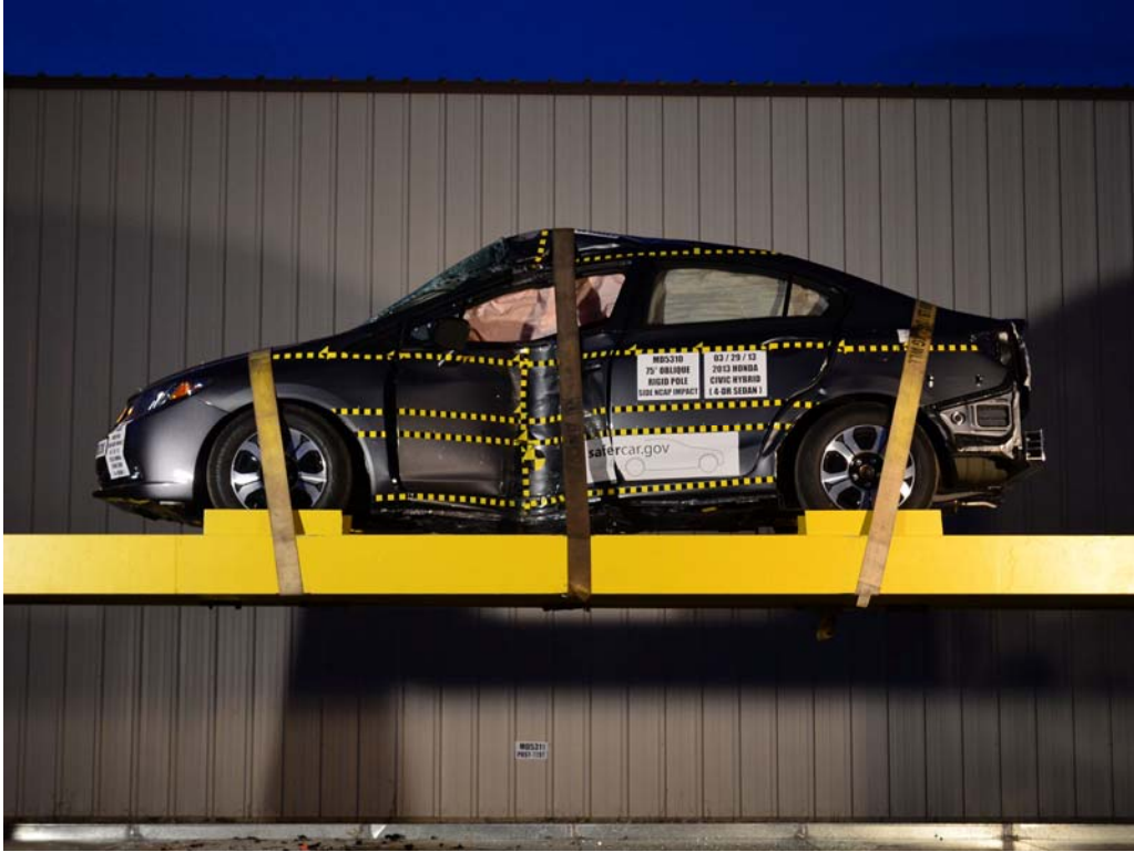
FIGURE 63. FMVSS No. 301 Static Rollover 0 Degrees
