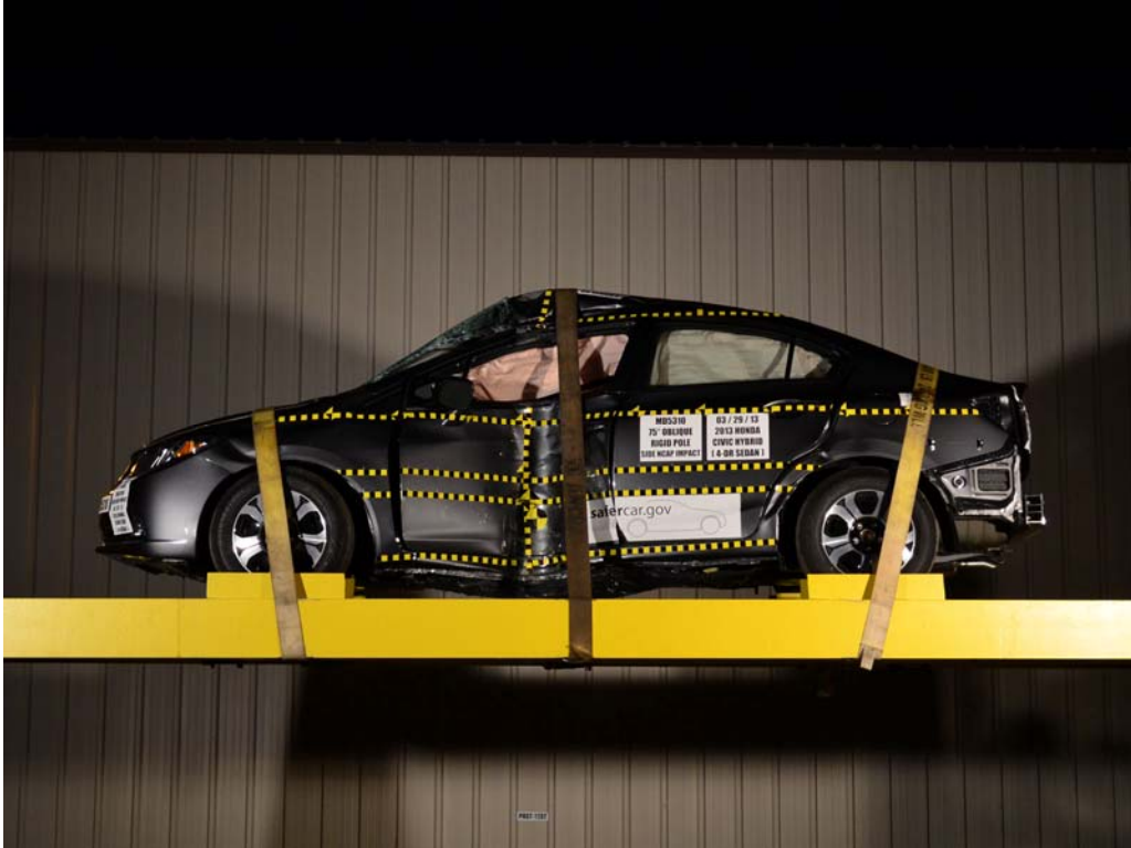
FIGURE 67. FMVSS No. 301 Static Rollover 360 Degrees
