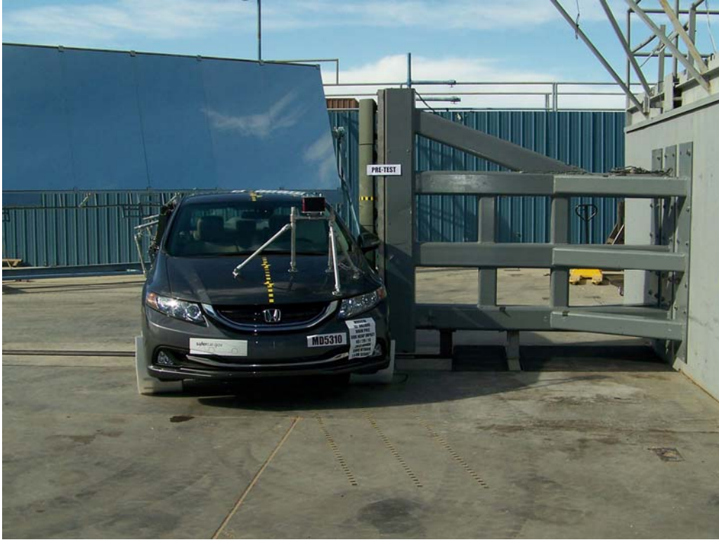
FIGURE 17. Pre-Test Left Side View of Pole Positioned Against Side of Test Vehicle
