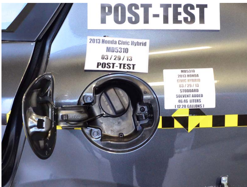
FIGURE 54. Post-Test View of Fuel Filler Cap or Fuel Filler Neck
