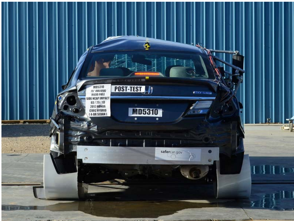
FIGURE 12. Post-Test Rear View of Test Vehicle
