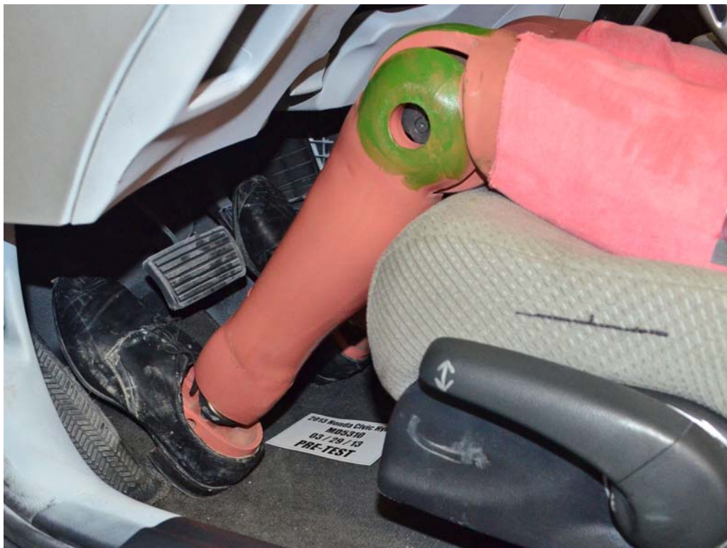
FIGURE 32. Pre-Test Placement of Dummy's Feet
