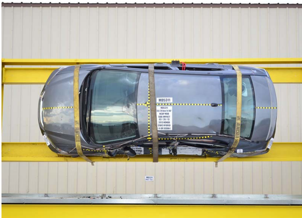
FIGURE 97. FMVSS No. 301 Static Rollover 90 Degrees
