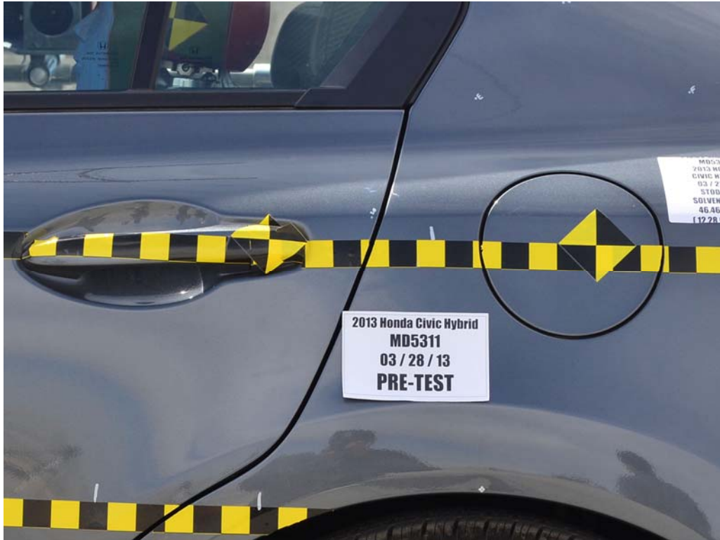
FIGURE 23. Pre-Test Left Rear Door Latch Close-Up
