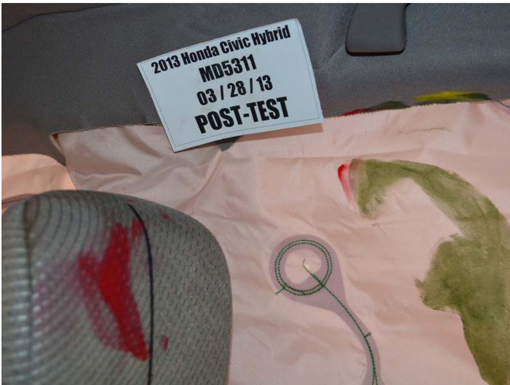
FIGURE 48. Post-Test Driver Dummy Close-Up Head Contact with Vehicle Interior View
