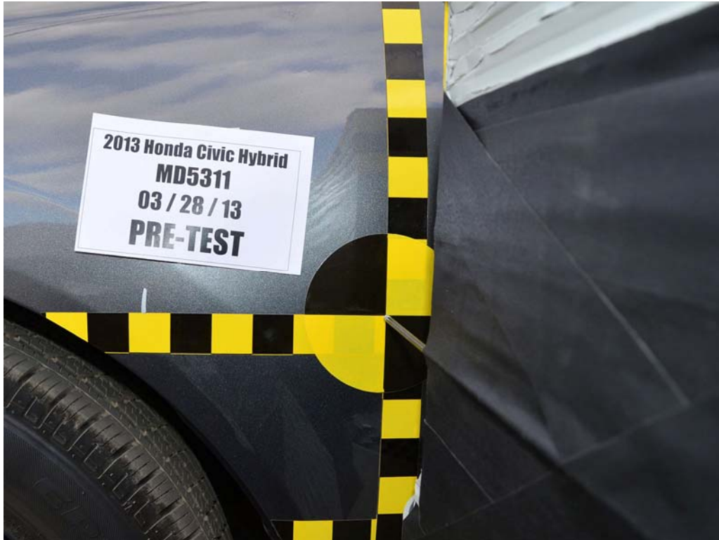
FIGURE 19. Pre-Test Close-Up View of Impact Point Target
