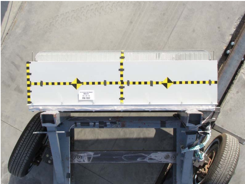
FIGURE 86. Pre-Test Top View of MDB Impactor Face
