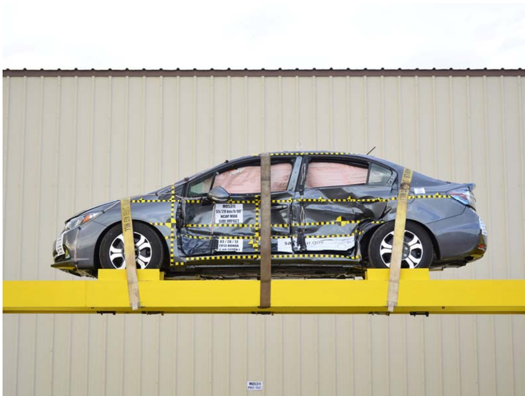
FIGURE 96. FMVSS No. 301 Static Rollover 0 Degrees
