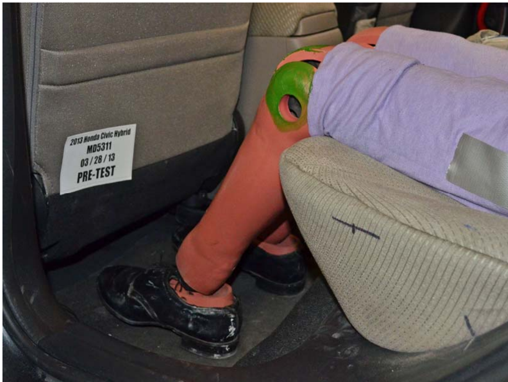
FIGURE 64. Pre-Test Placement of Rear Passenger Dummy's Feet
