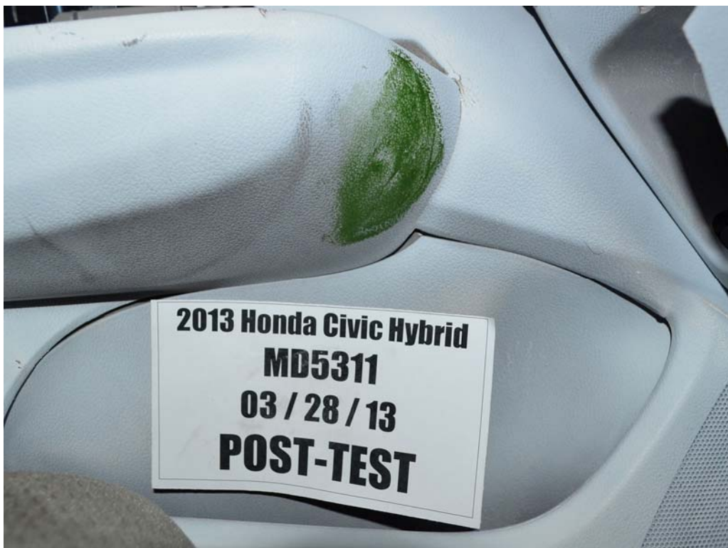
FIGURE 54. Post-Test Driver Dummy Close-Up Knee Contact View
