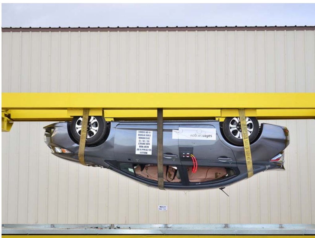
FIGURE 98. FMVSS No. 301 Static Rollover 180 Degrees
