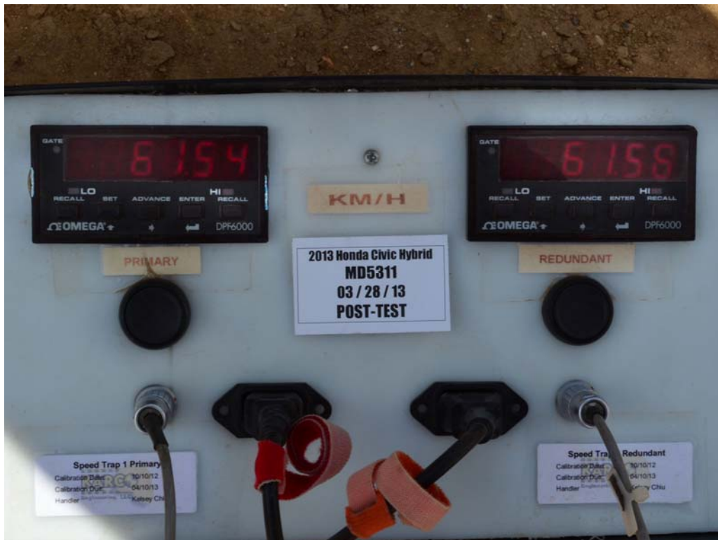
FIGURE 95. Post-Test Primary and Redundant Speed Trap Read-Out
