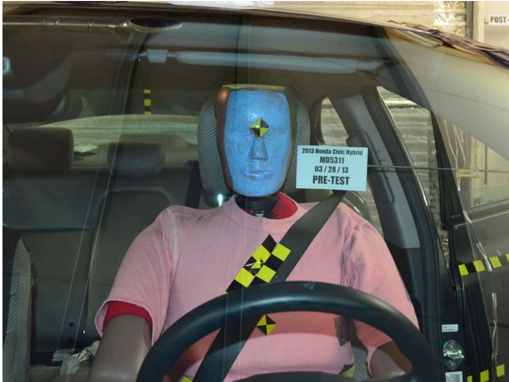
FIGURE 25. Pre-Test Front Close-Up View of Driver Dummy
