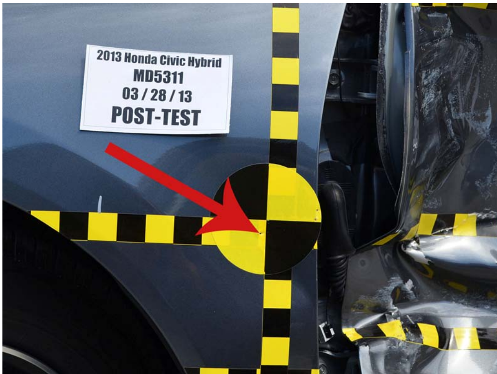
FIGURE 20. Post-Test Close-Up View of Impact Point Target
