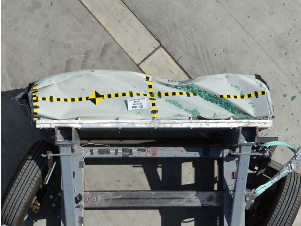
FIGURE 87. Post-Test Top View of MDB Impactor Face
