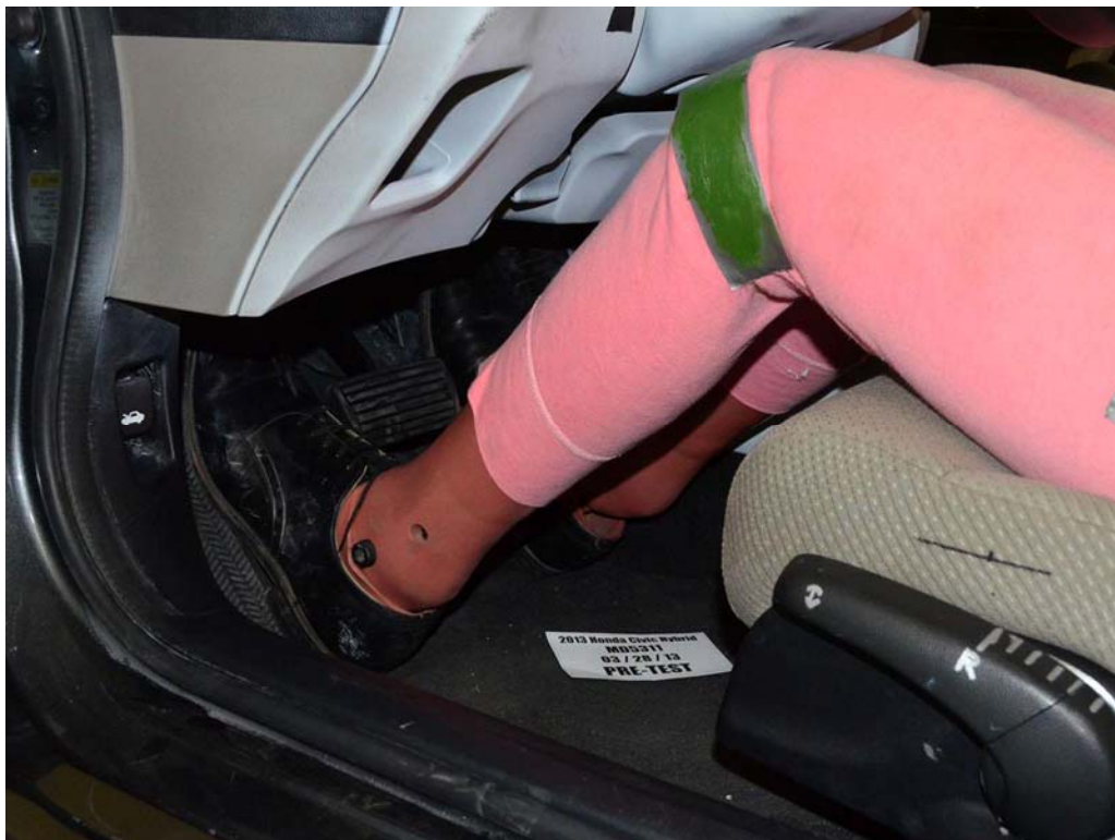
FIGURE 34. Pre-Test Placement of Driver Dummy's Feet
