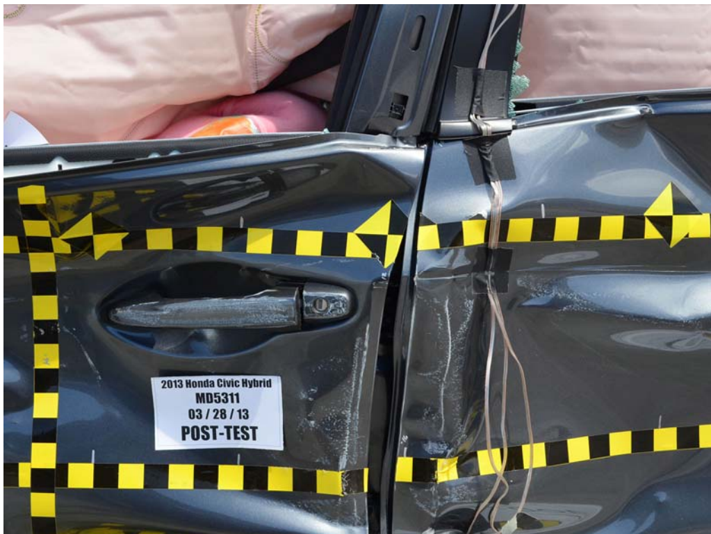
FIGURE 22. Post-Test Left Front Door Latch Close-Up
