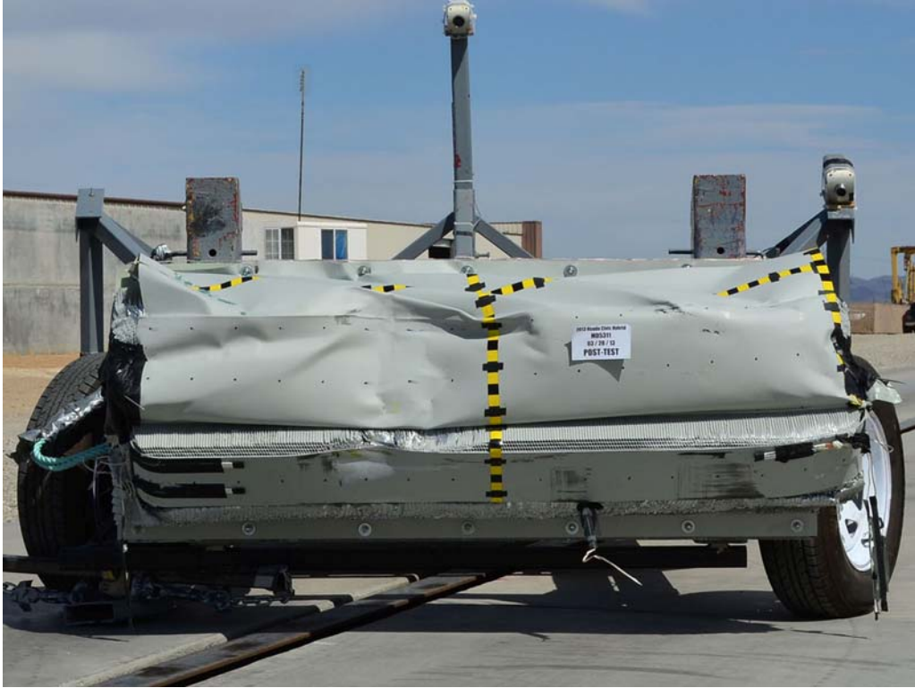
FIGURE 85. Post-Test Front View of MDB Impactor Face
