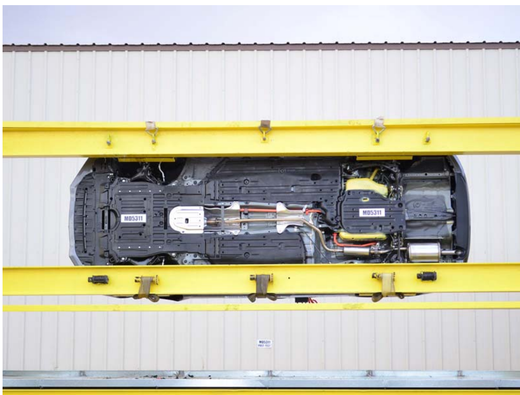
FIGURE 99. FMVSS No. 301 Static Rollover 270 Degrees
