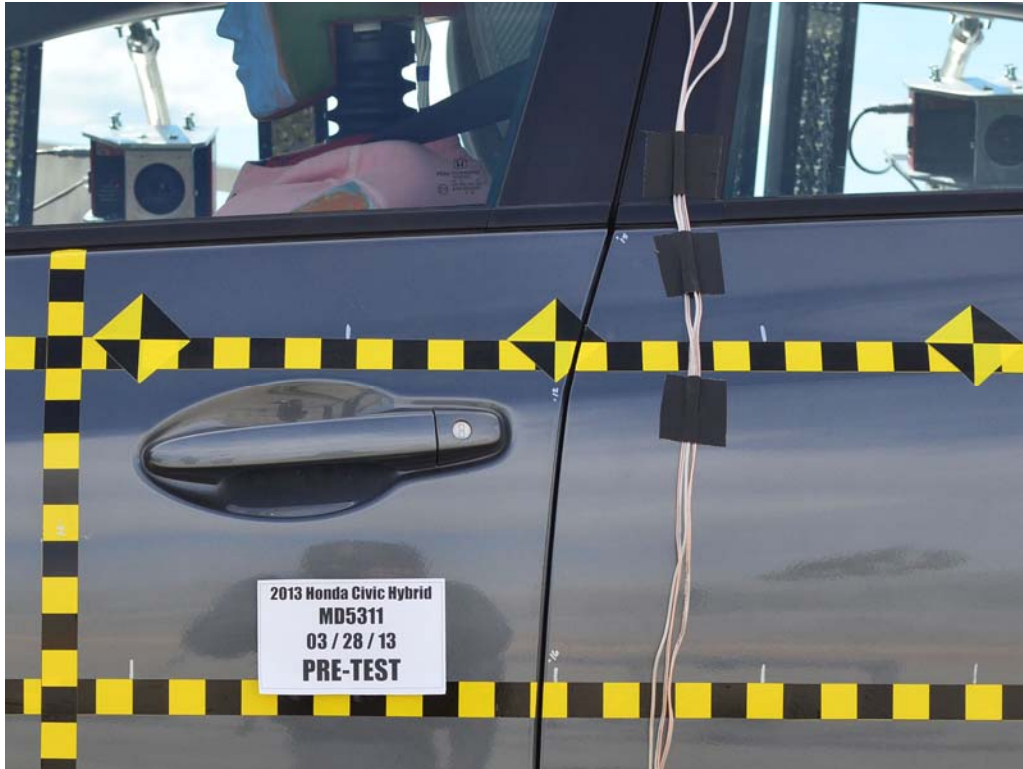
FIGURE 21. Pre-Test Left Front Door Latch Close-Up
