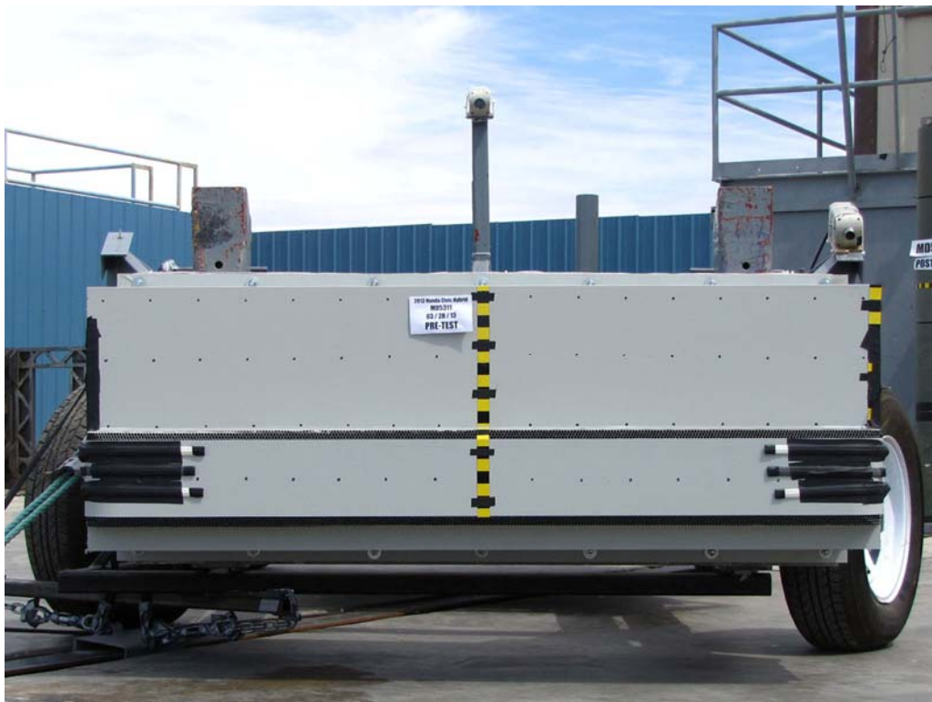
FIGURE 84. Pre-Test Front View of MDB Impactor Face
