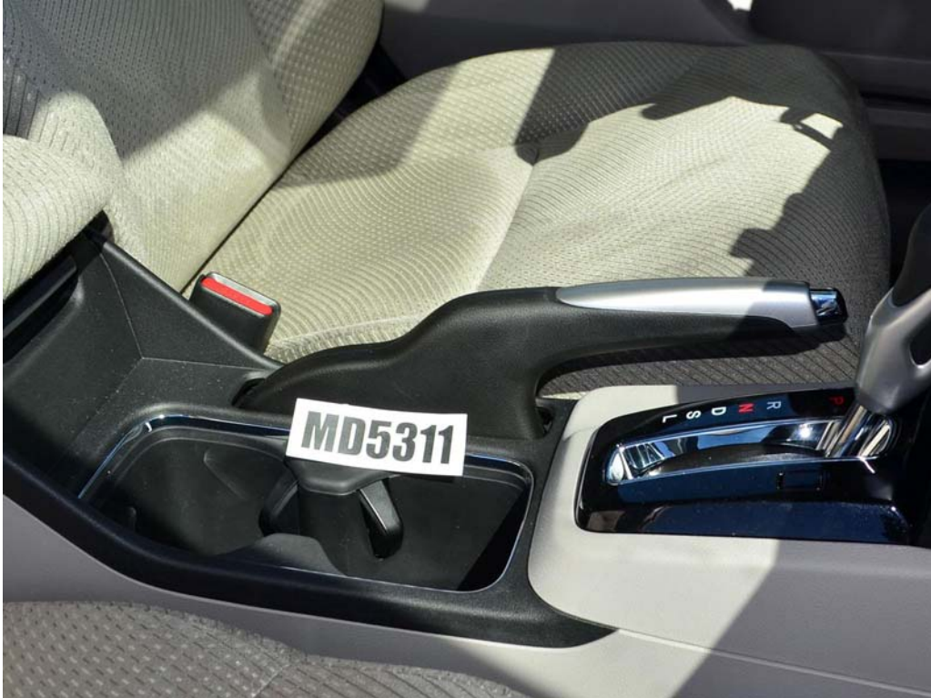
FIGURE 37. View of Disengaged Parking Brake
