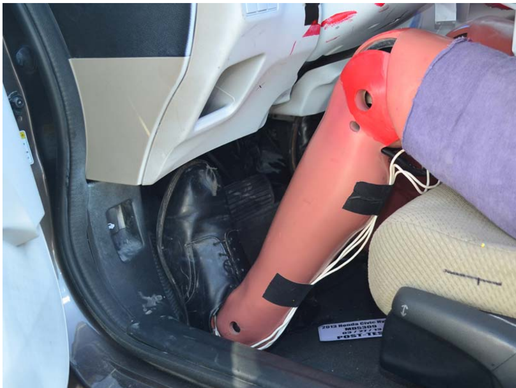
FIGURE 40. Post-Test Driver Dummy Feet
