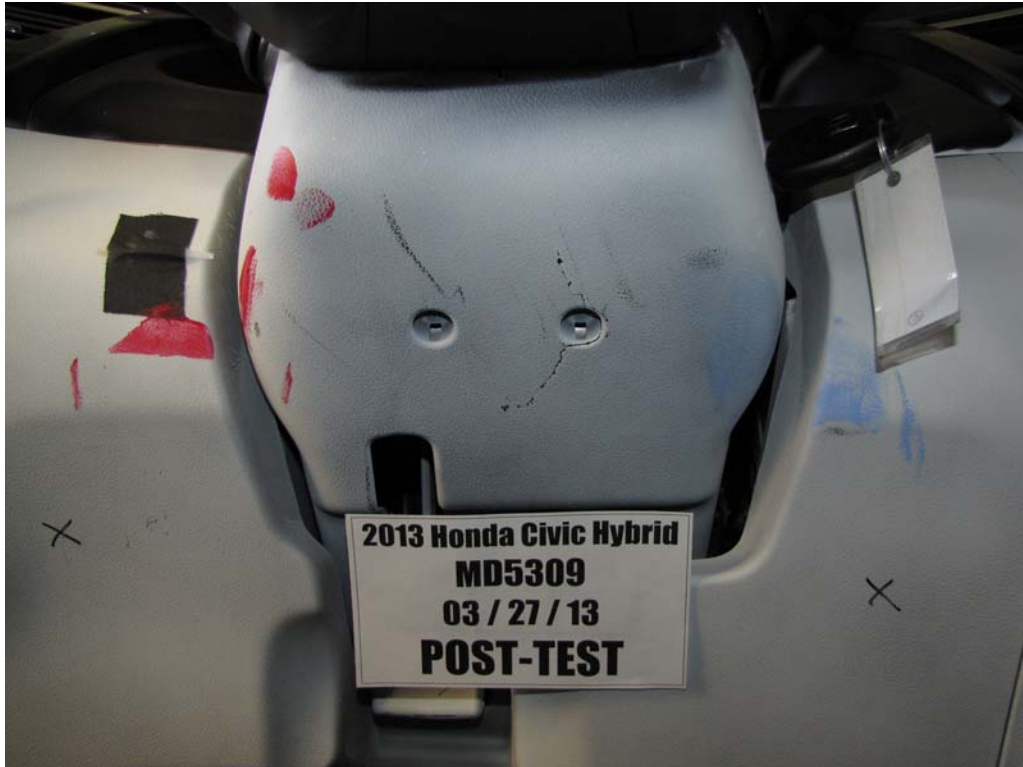
FIGURE 47b. Post-Test Driver Dummy Contact with Steering Column
