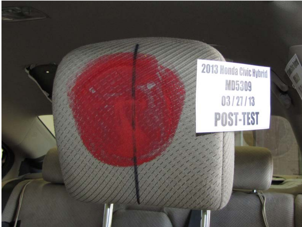
FIGURE 47. Post-Test Driver Dummy Contact with Headrest
