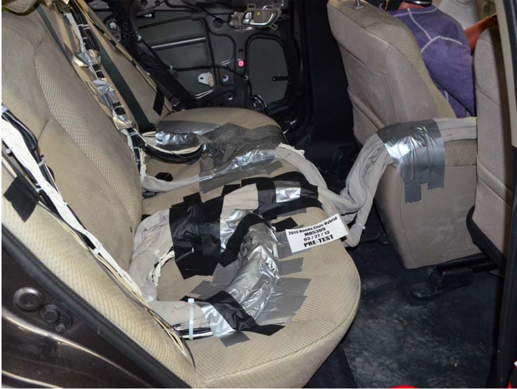
FIGURE 27. Pre-Test Dummy Cable Routing
