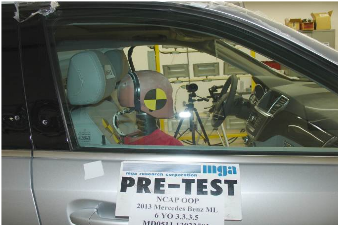
Pre-Test 6-Year-Old Child Dummy Right Side View
