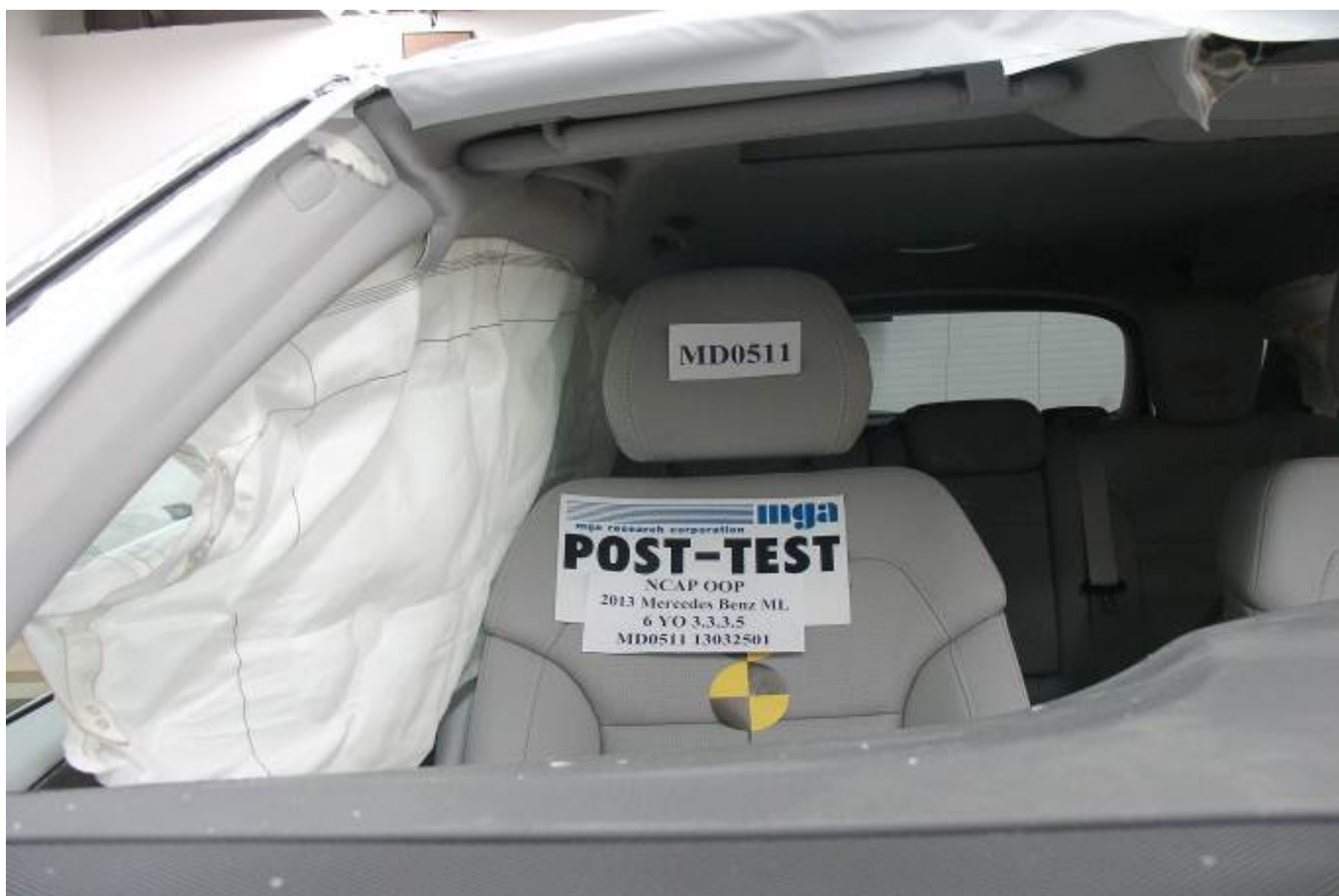
Post-Test Curtain Airbag Front View
