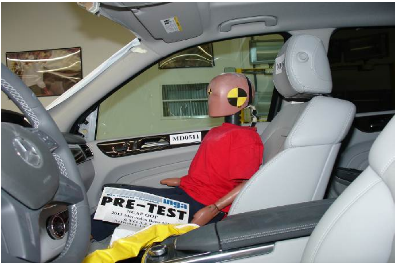
Pre-Test 6-Year-Old Child Dummy Left Side View
