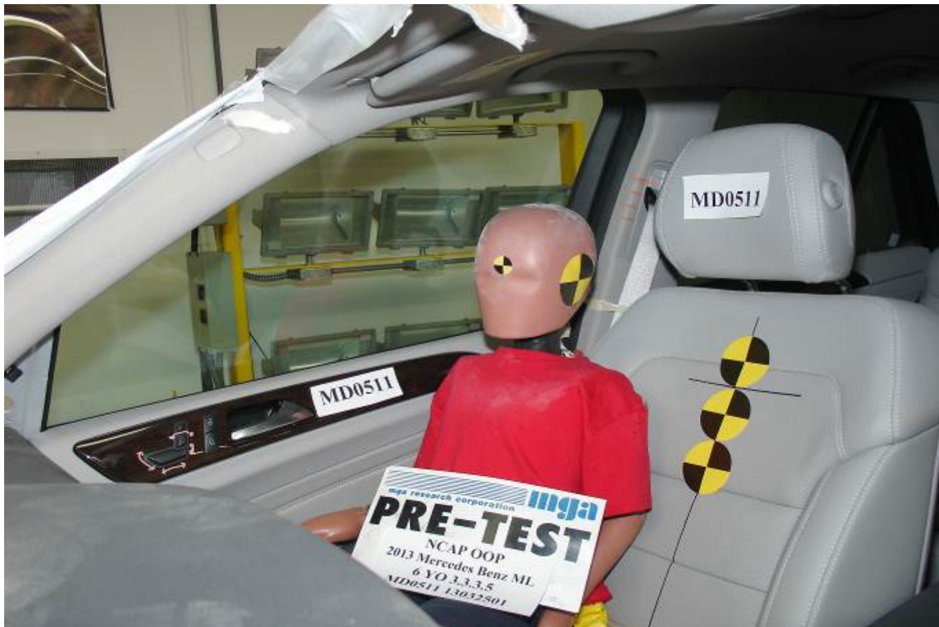
Pre-Test 6-Year-Old Child Dummy Left 3/4 Front View
