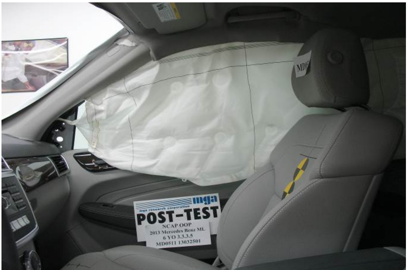
Post-Test Curtain Airbag Left Side View
