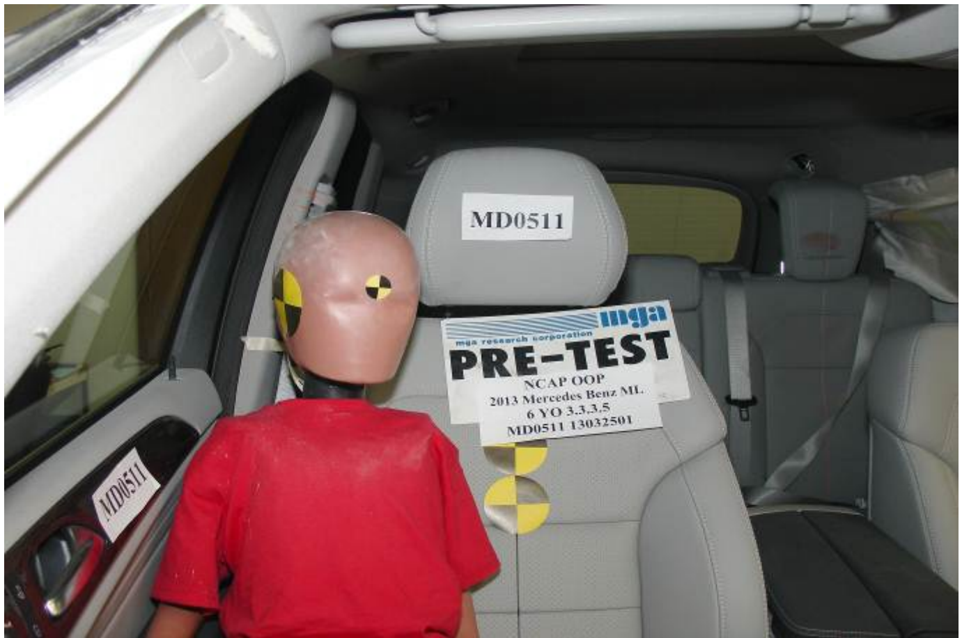
Pre-Test 6-Year-Old Child Dummy Front View
