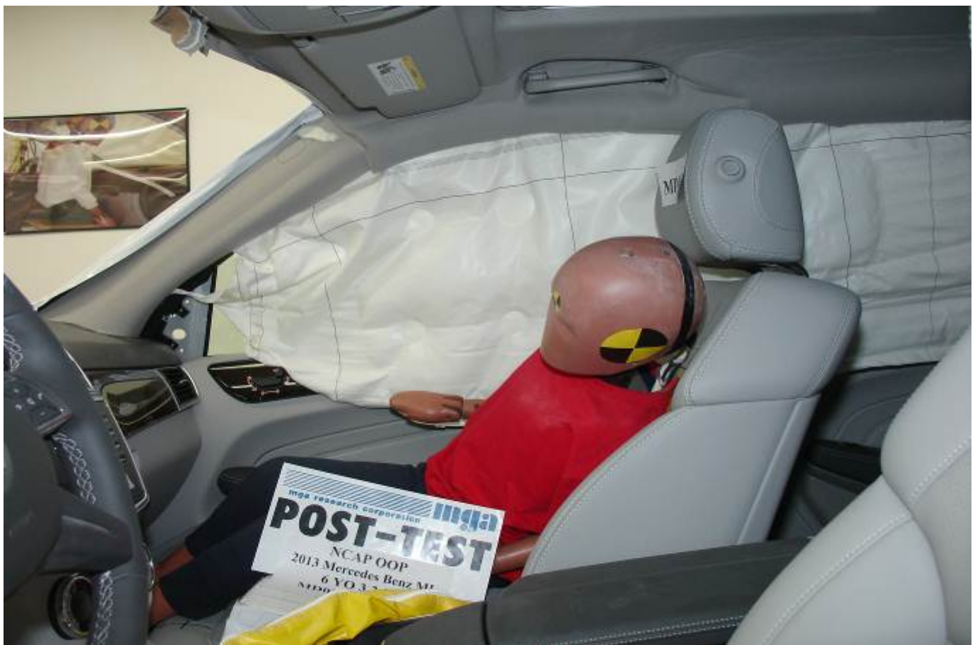
Post-Test 6-Year-Old Child Dummy Left Side View
