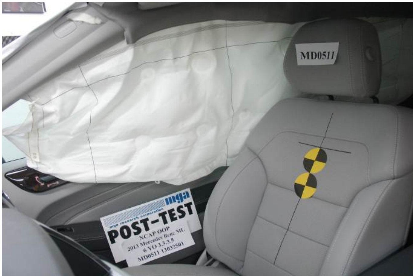
Post-Test Curtain Airbag Left 3/4 Front View
