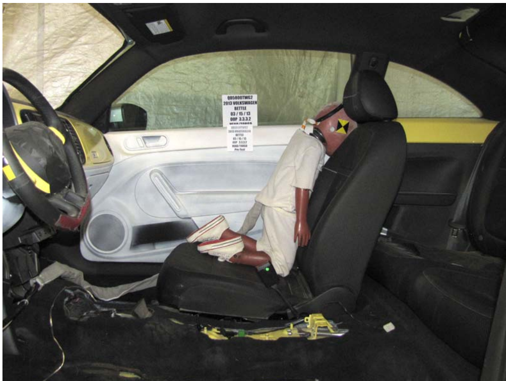
FIGURE 7. Pre-Test Dummy Position, Left Side View
