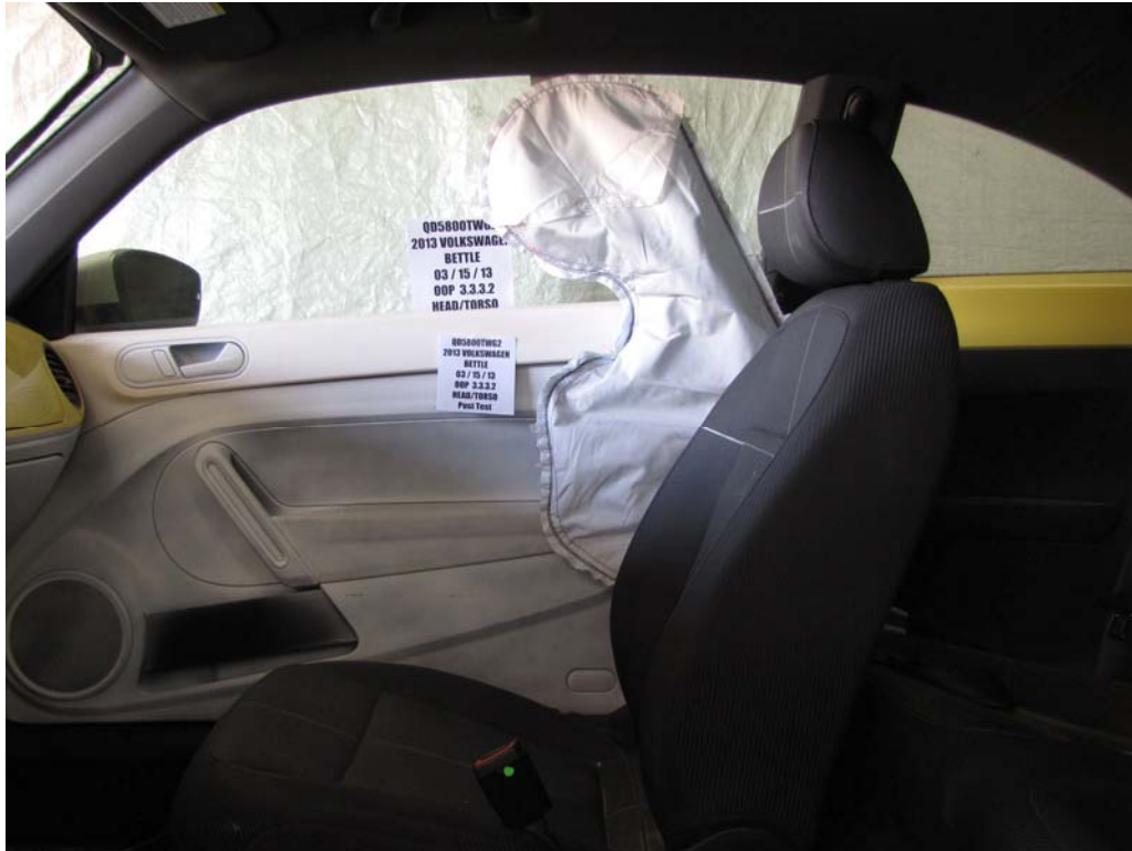
FIGURE 13. Post-Test Airbags, Left Side View
