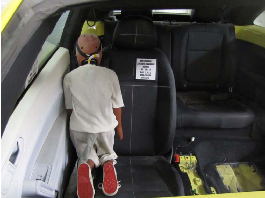
FIGURE 11. Pre-Test Dummy Position, Front View
