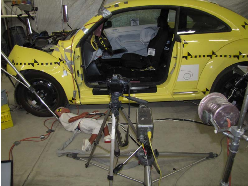
FIGURE 17. Post-Test, Dummy Final Resting Position
