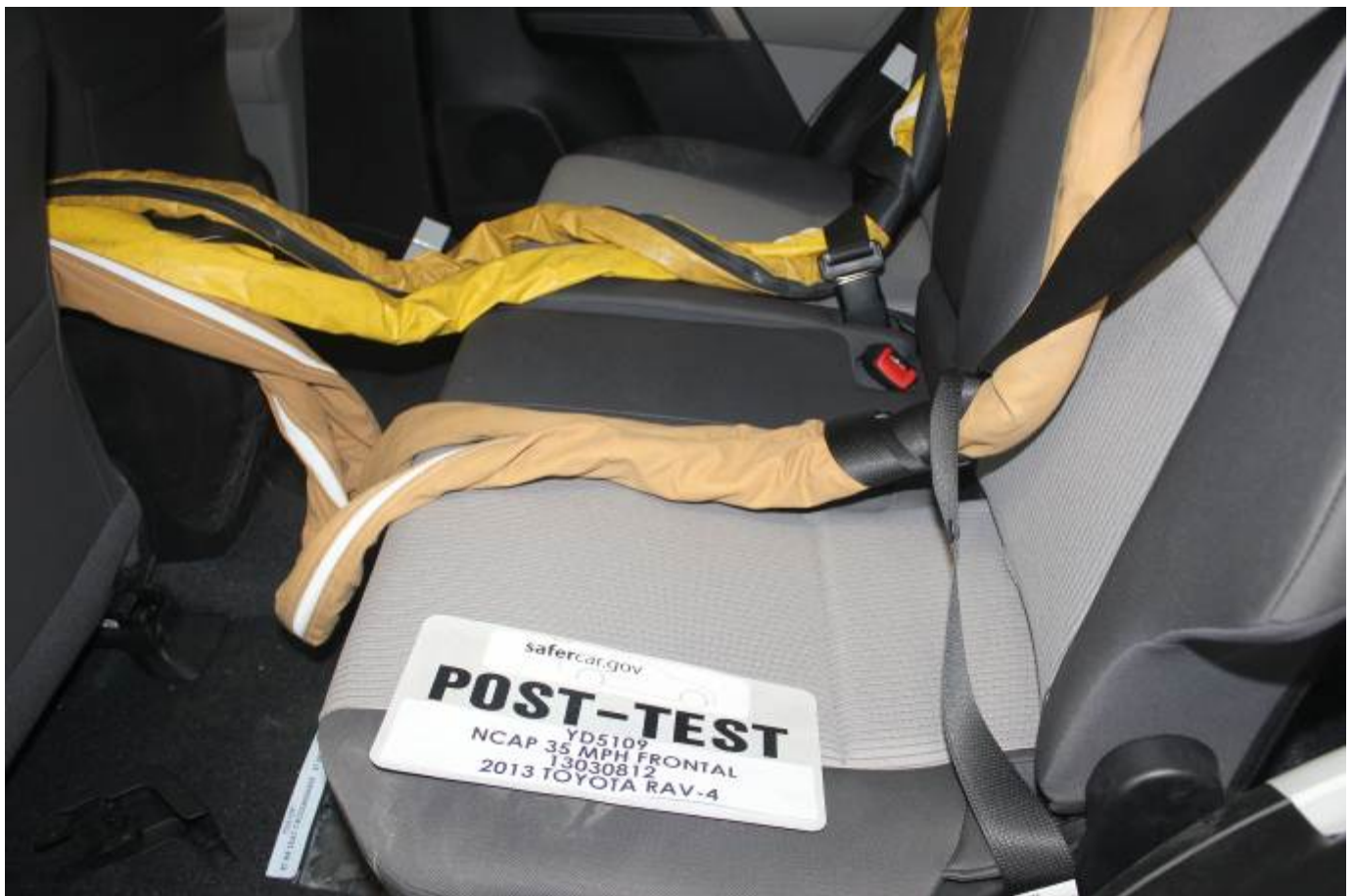
Post-Test Dummy Cable Routing
