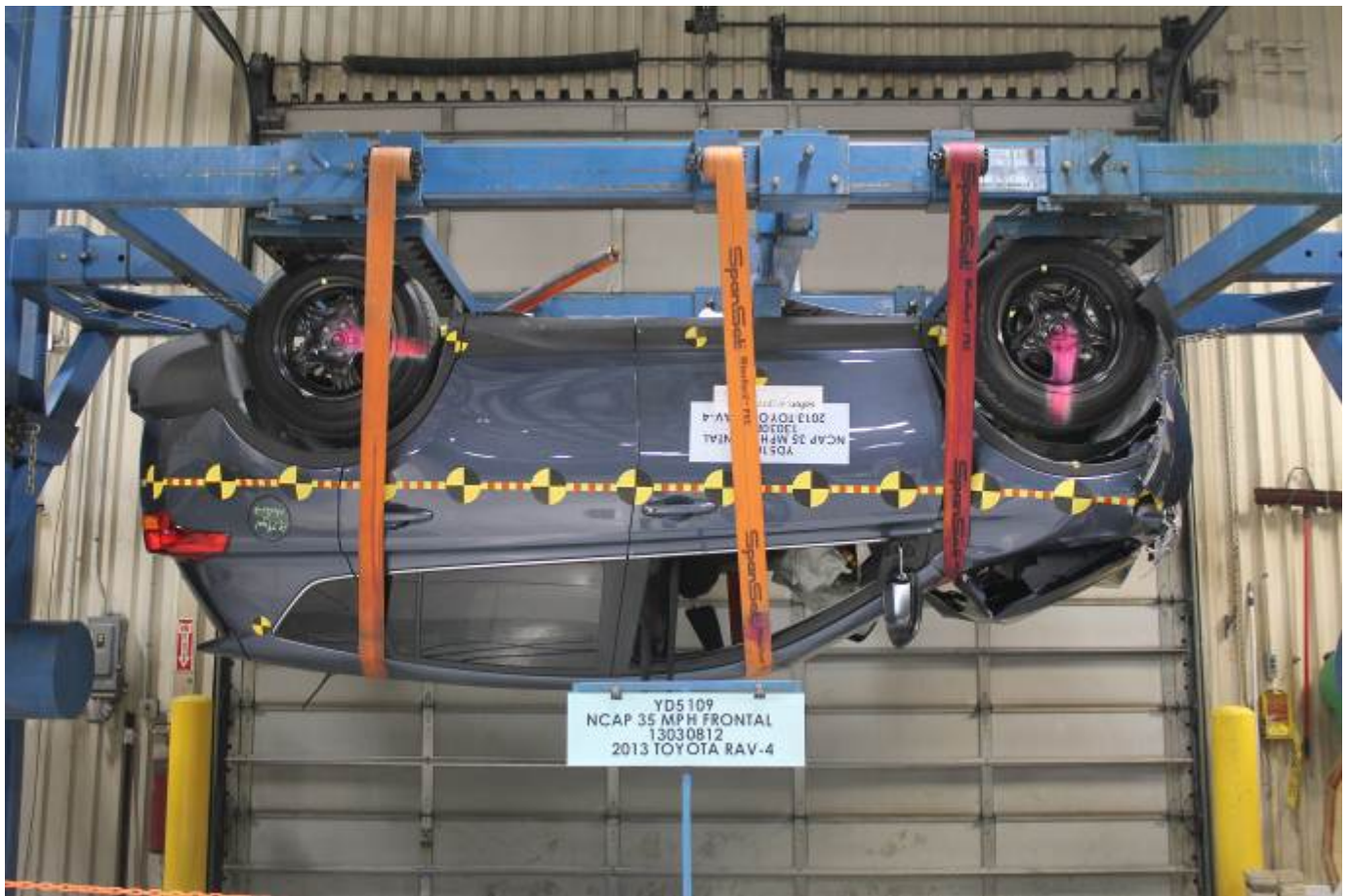
Vehicle at 180° on Static Rollover Device
