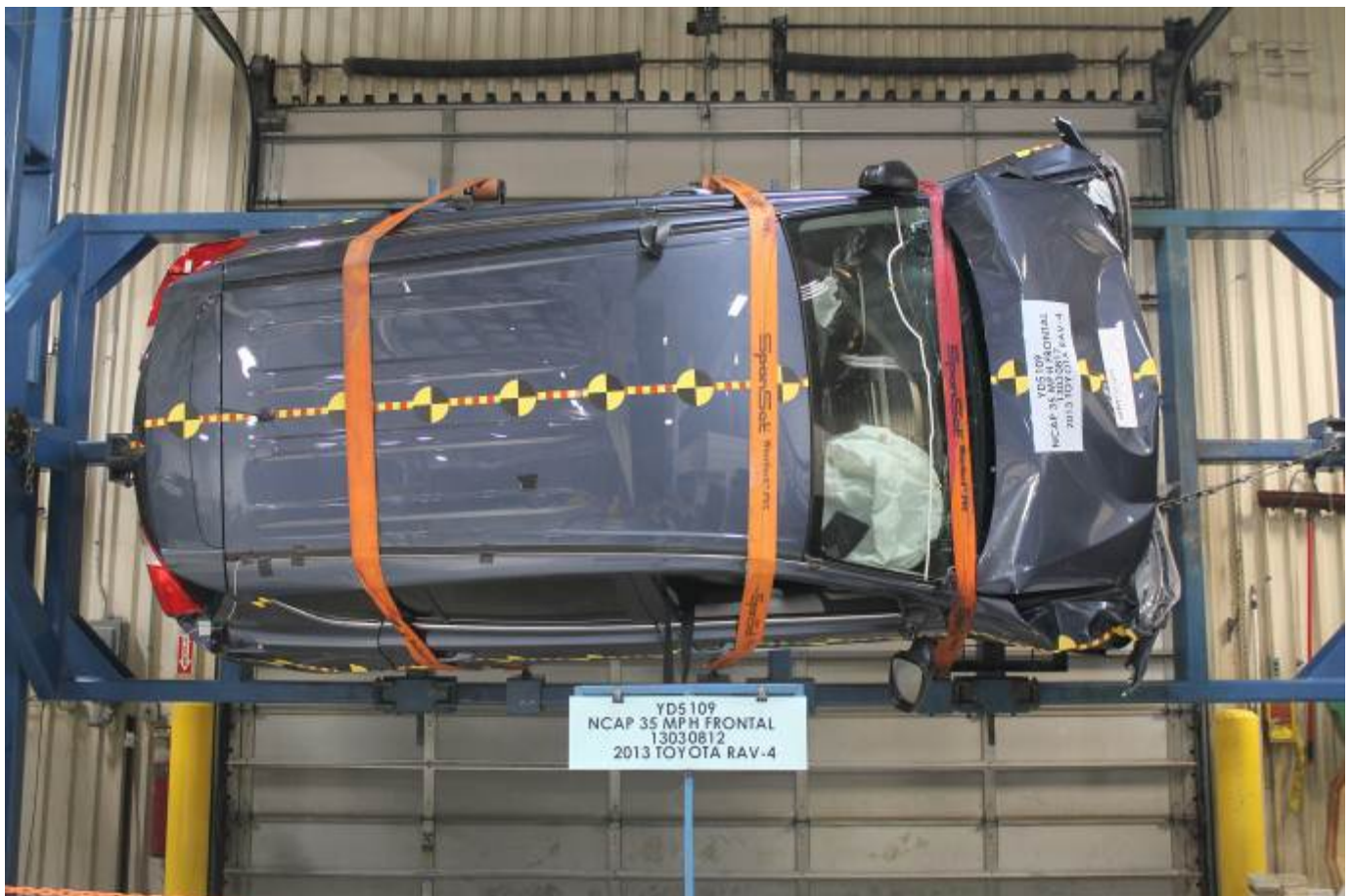
Vehicle at 270° on Static Rollover Device
