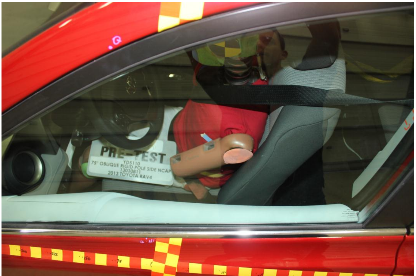
Pre-Test Dummy and Door Clearance View
