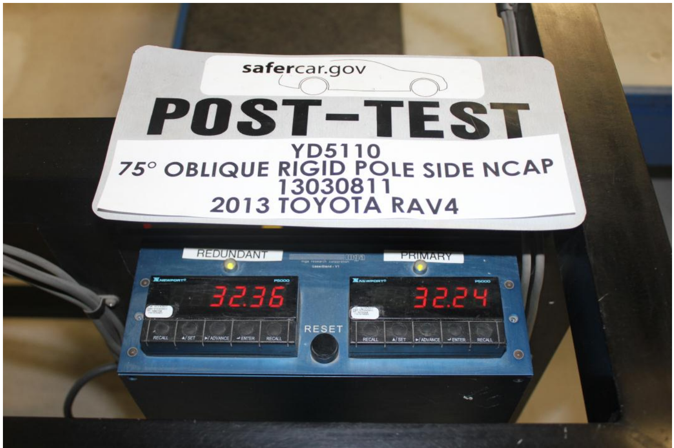
Post-Test Primary and Redundant Speed Trap Read-Out
