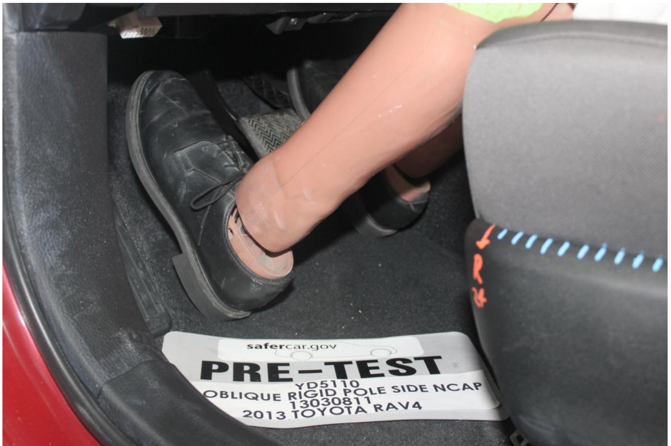
Pre-Test Placement of Dummy's Feet
