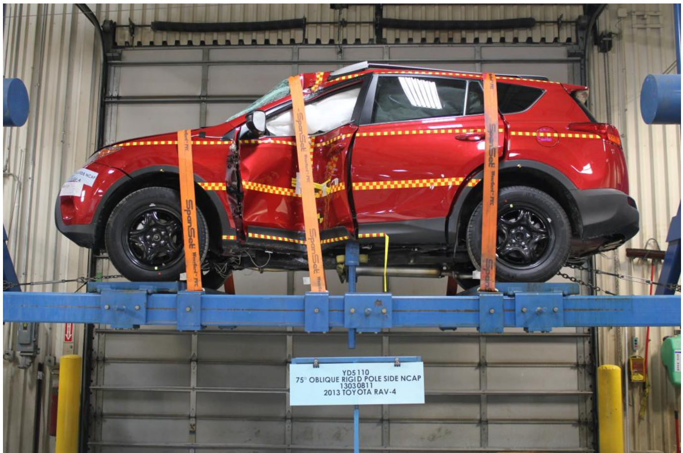
FMVSS No. 301 Static Rollover 0 Degrees
