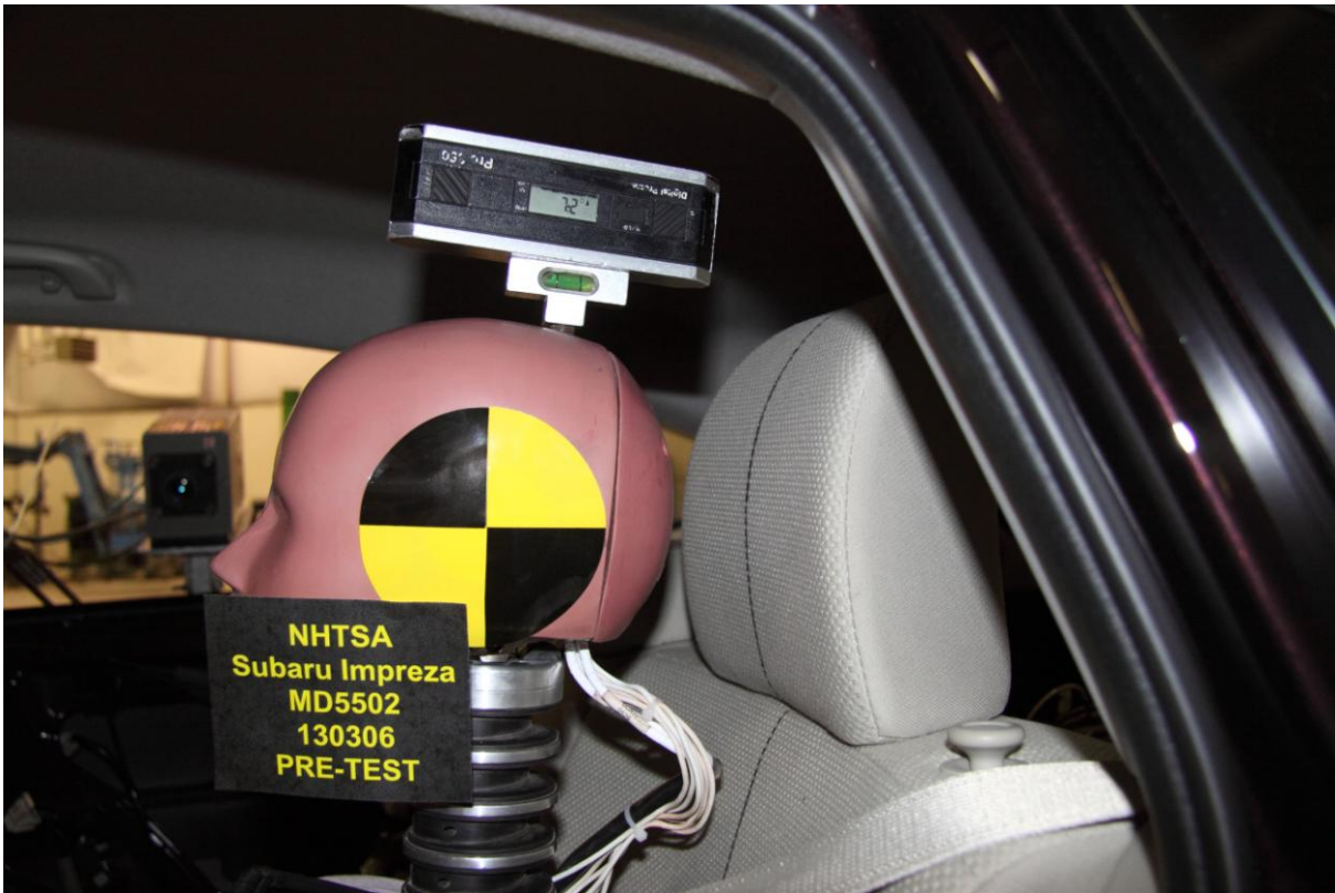
063 Pre-Test View of Rear Passenger Dummy Head Showing Dummy Head is Level
