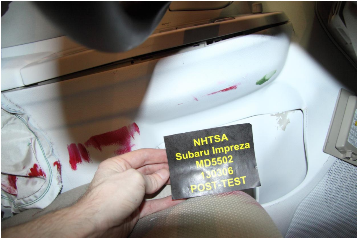
054 Post-Test Driver Dummy Close-Up Knee Contact View
