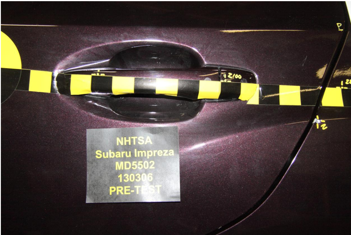
023 Pre-Test Left Rear Door Latch Close-up
