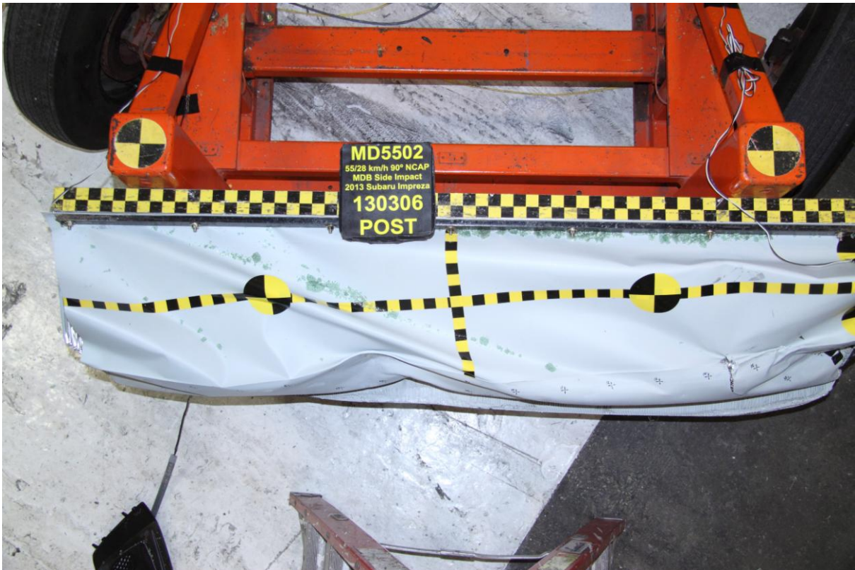
087 Post-Test Top View of MDB Impactor Face
