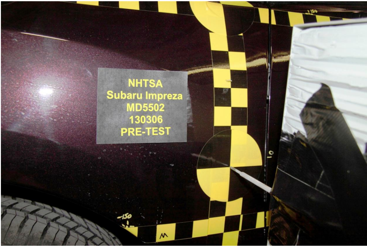
019 Pre-Test Close-up View of Impact Point Target
