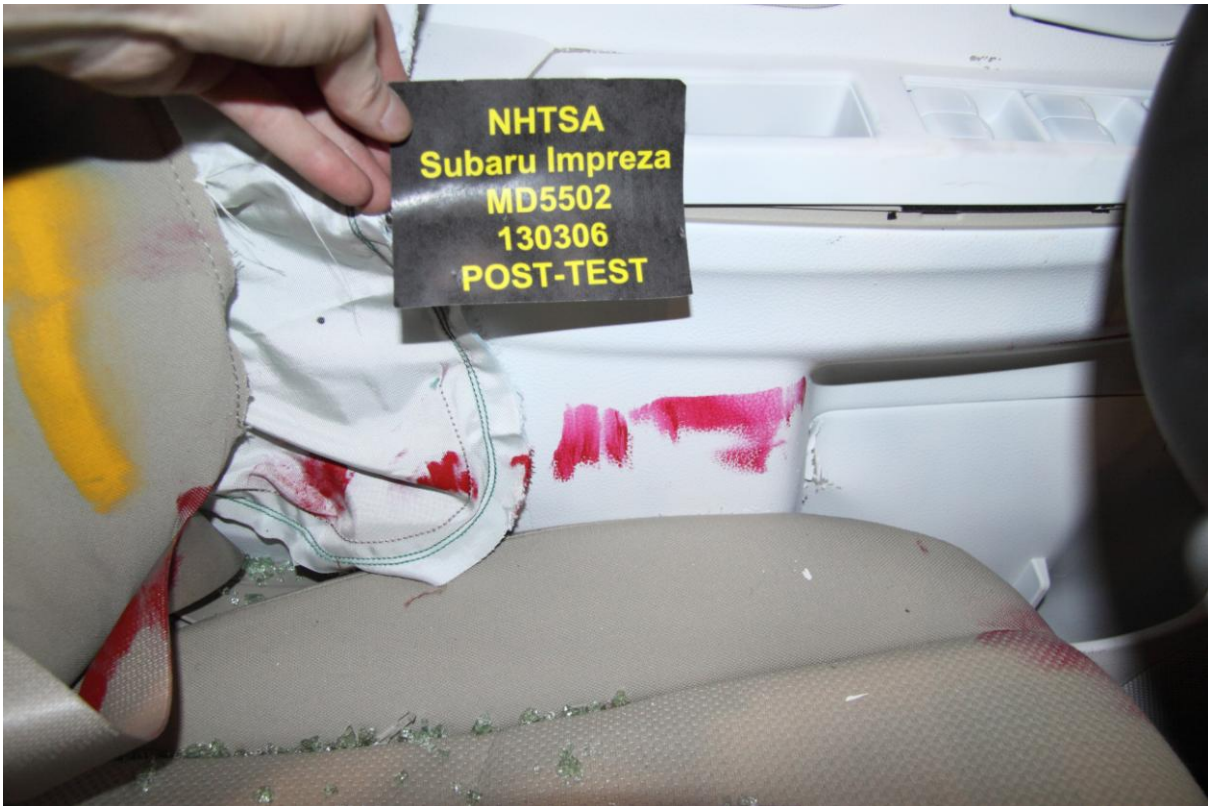
052 Post-Test Driver Dummy Close-Up Pelvis Contact View
