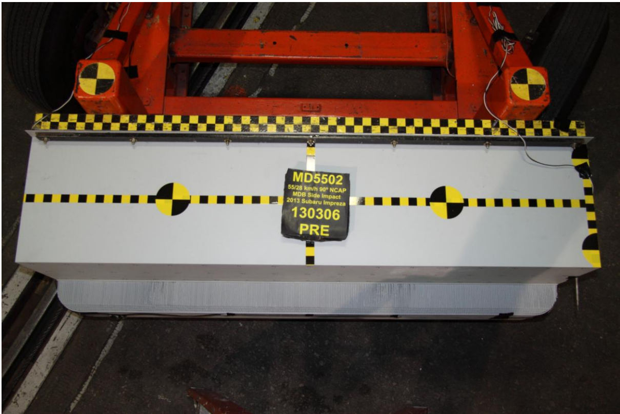
086 Pre-Test Top View of MDB Impactor Face
