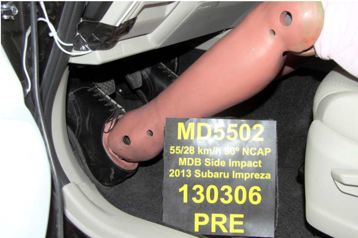
034 Pre-Test Placement of Driver Dummy Feet
