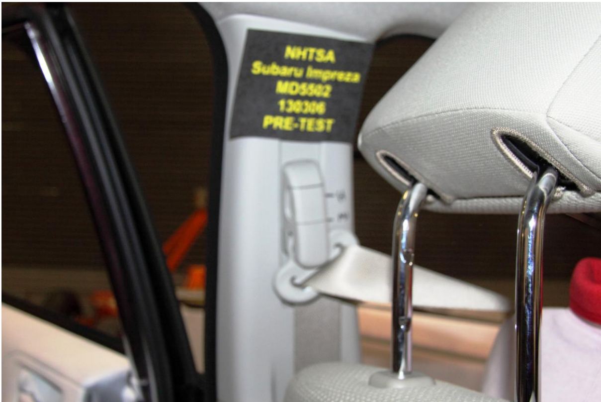
035 Pre-Test View of Belt Anchorage for Driver Dummy
