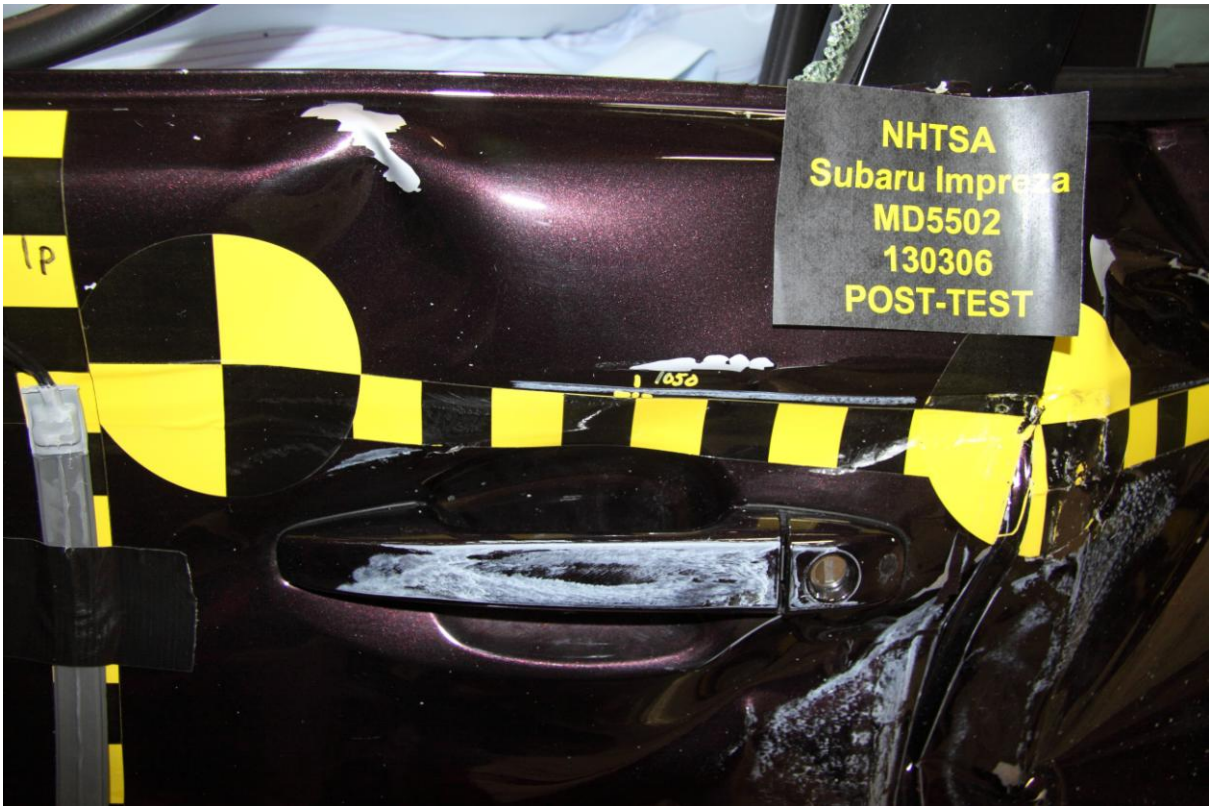
022 Post-Test Left Front Door Latch Close-up
