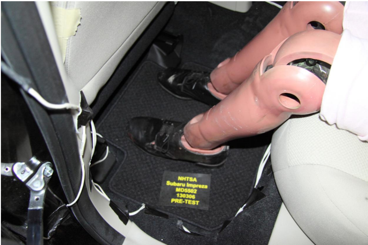
064 Pre-Test Placement of Rear Passenger Dummy Feet
