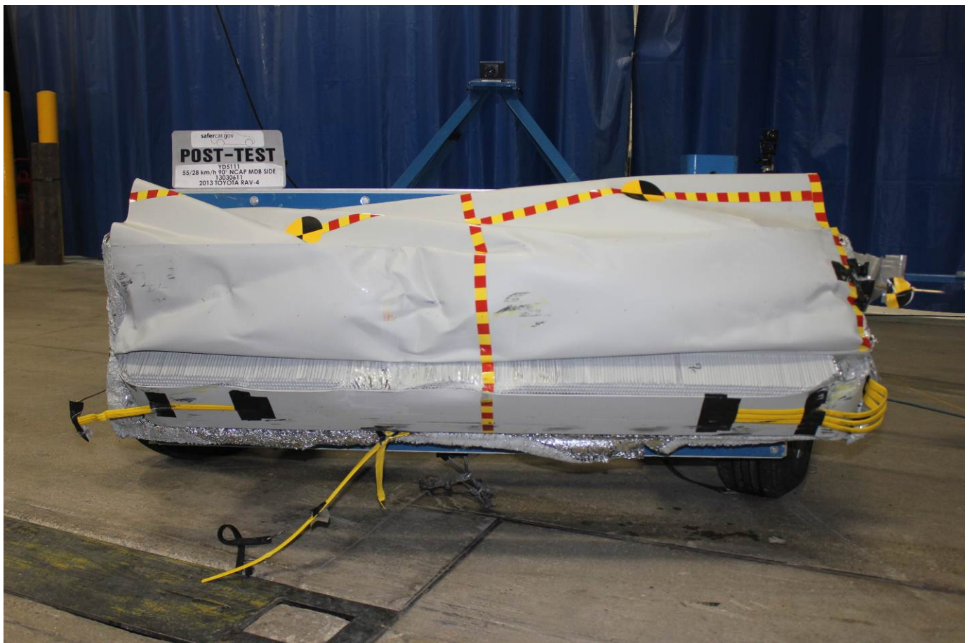
Post-Test Front View of MDB Impactor Face
