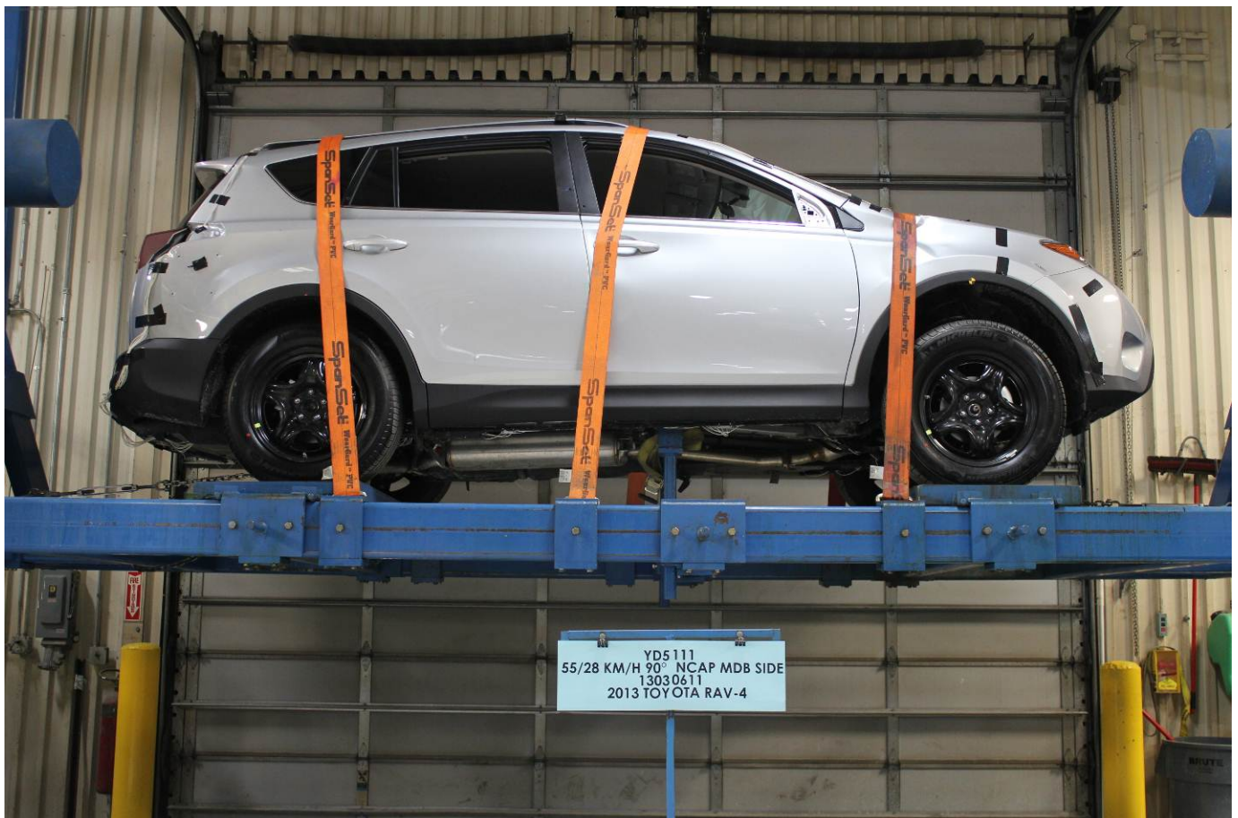
FMVSS No. 301 Static Rollover 360 Degrees
