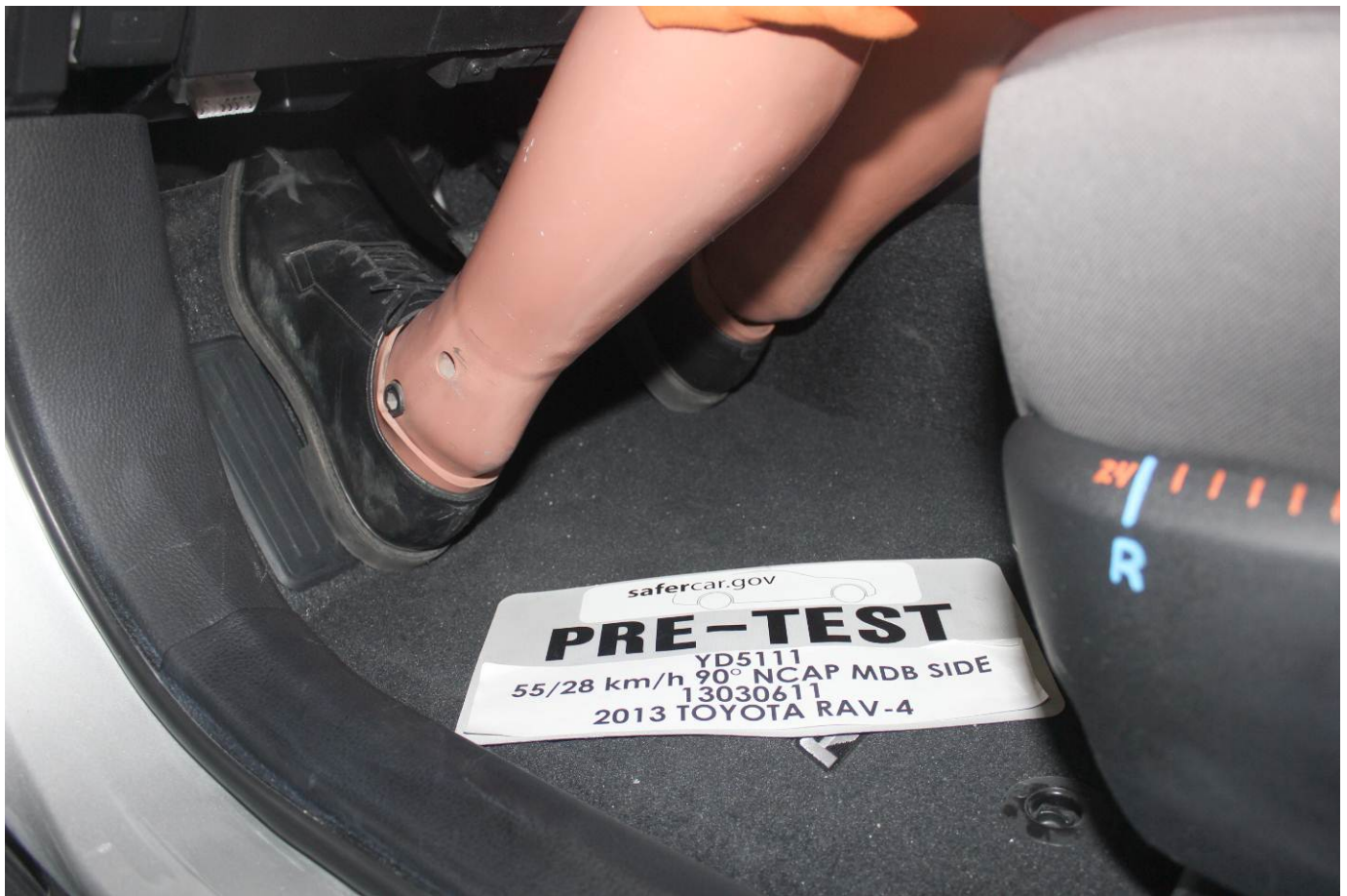
Pre-Test Placement of Driver Dummy's Feet
