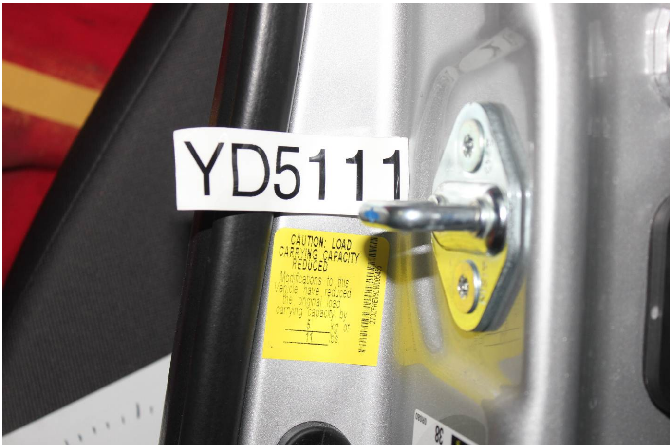
Close-Up View of Vehicle's Load Carrying Capacity Reduced Label
