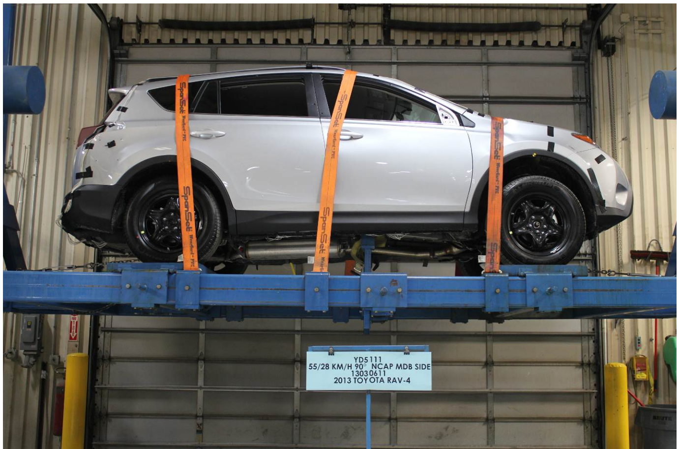
FMVSS No. 301 Static Rollover 0 Degrees
