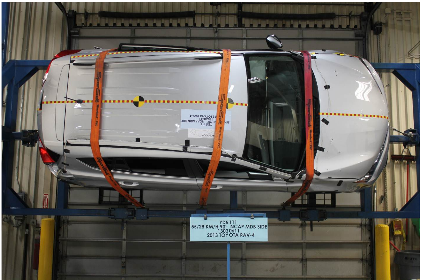
FMVSS No. 301 Static Rollover 270 Degrees
