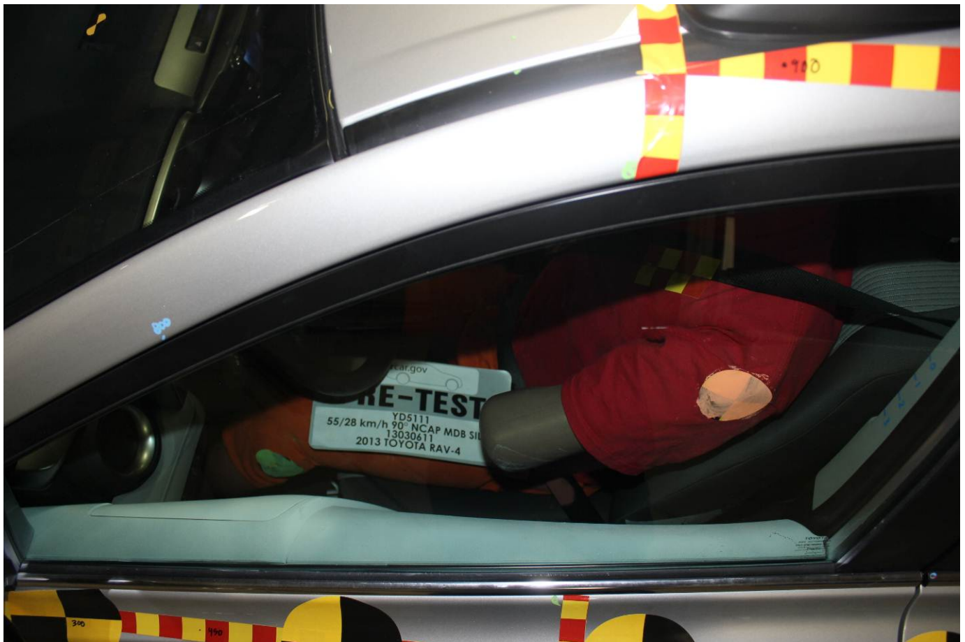
Pre-Test Driver Dummy and Door Clearance View
