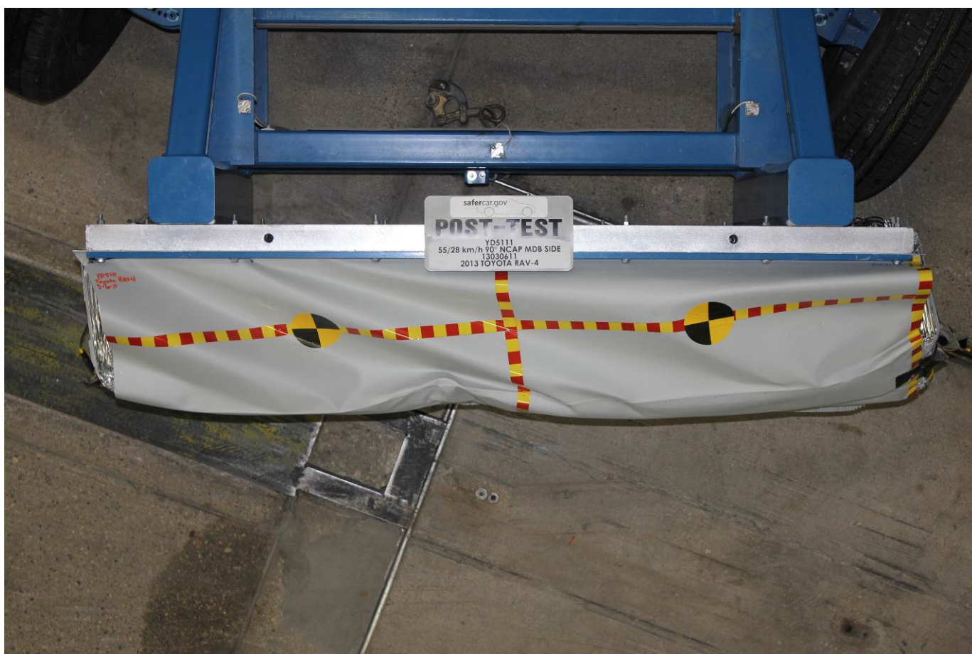
Post-Test Top View of MDB Impactor Face
