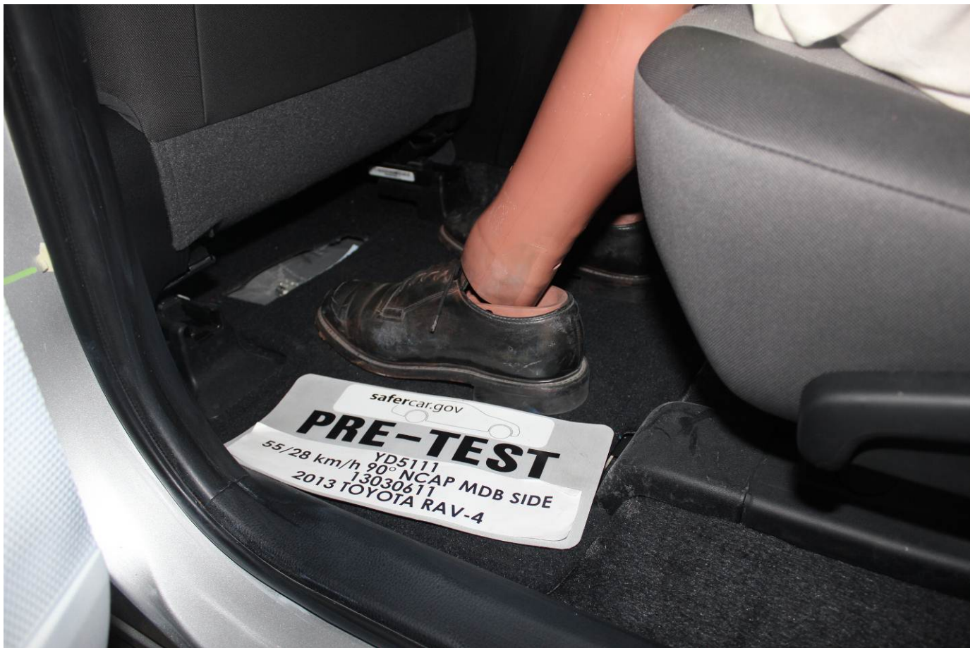
Pre-Test Placement of Rear Passenger Dummy's Feet
