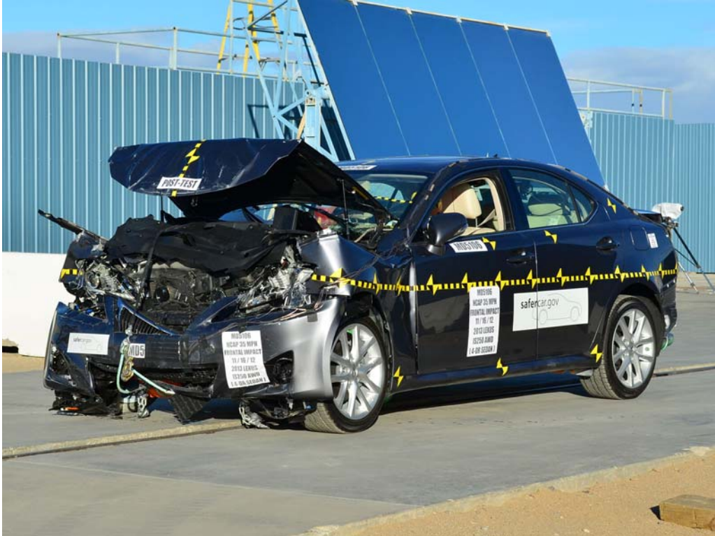
FIGURE 5. Post-Test Left Front \frac{3}{4} View of NCAP Frontal Impact Test
