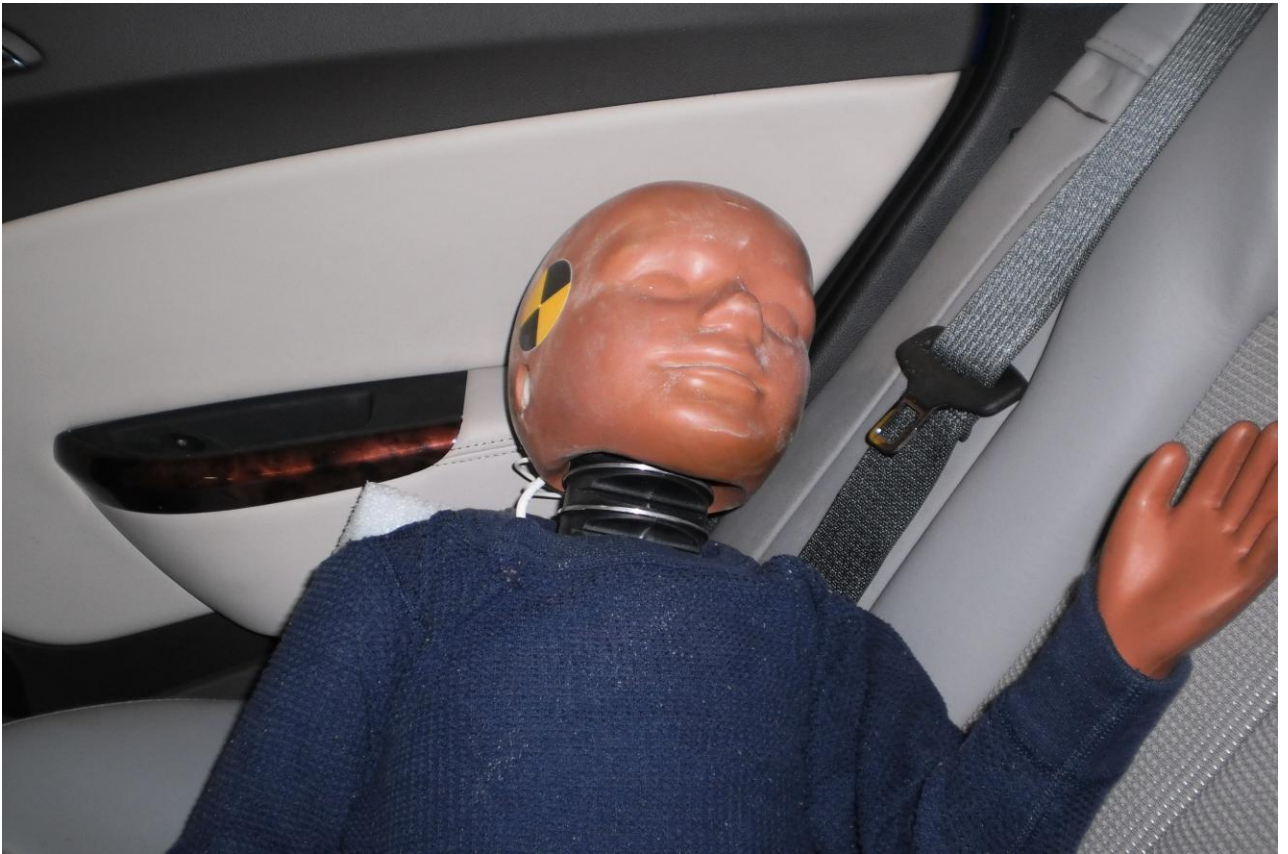
Figure A-5 Pre-Test Right Rear Dummy Position – Side View
