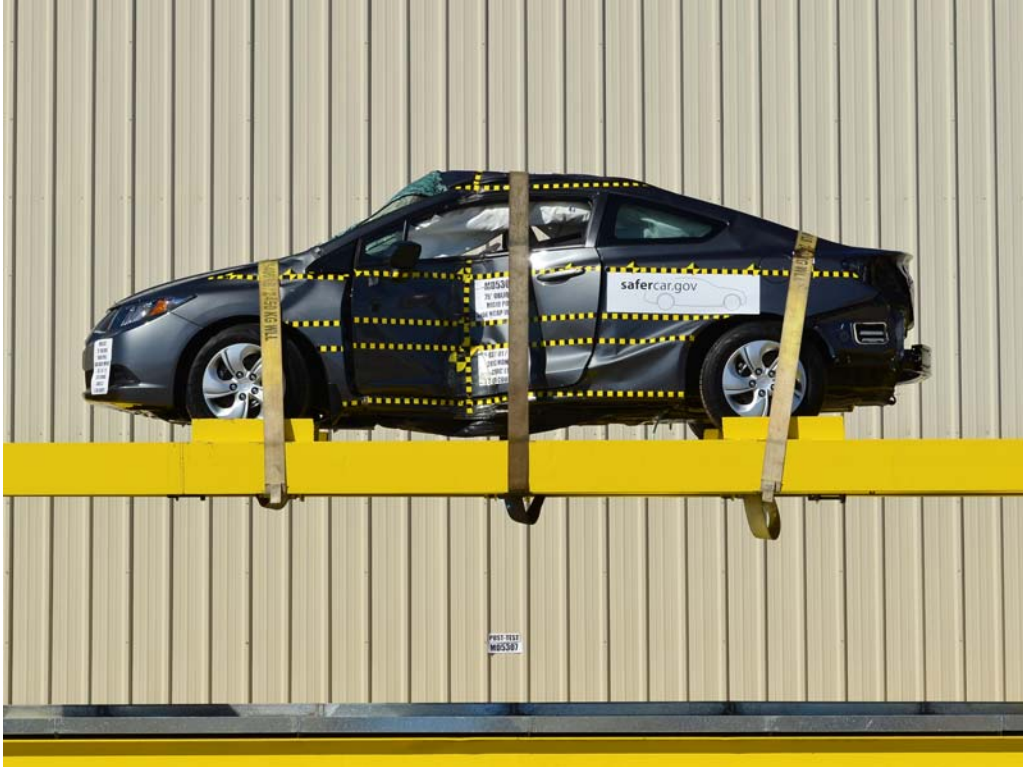
FIGURE 67. FMVSS No. 301 Static Rollover 360 Degrees
