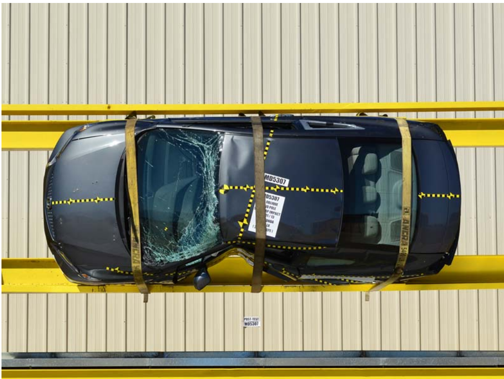
FIGURE 64. FMVSS No. 301 Static Rollover 90 Degrees
