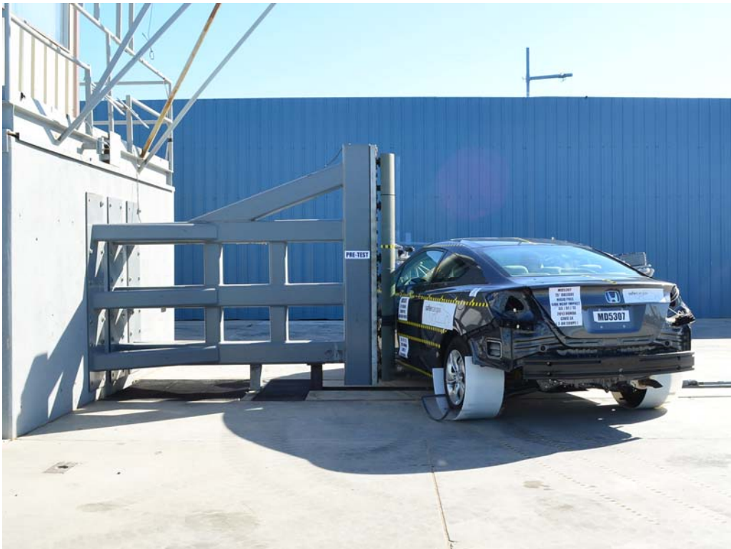
FIGURE 18. Pre-Test Right Side View of Pole Positioned Against Side of Test Vehicle
