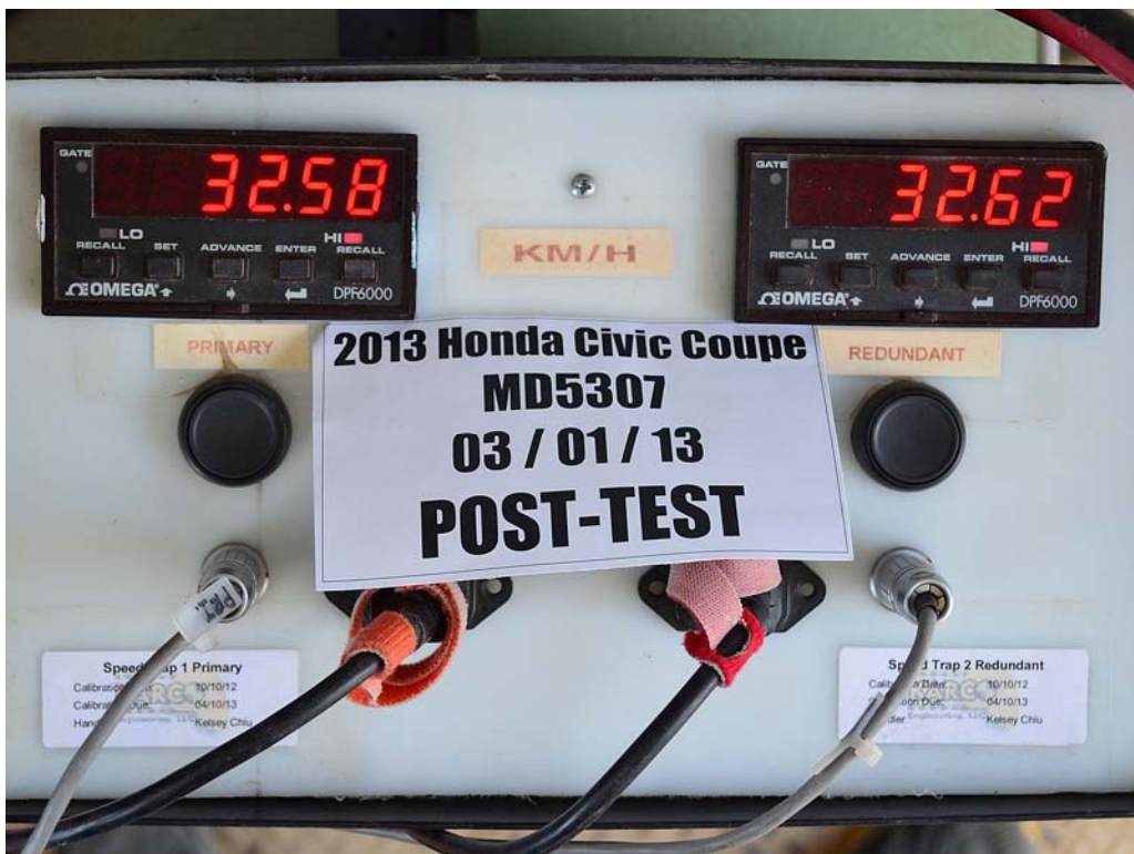
FIGURE 62. Post-Test Primary and Redundant Speed Trap Read-Out
