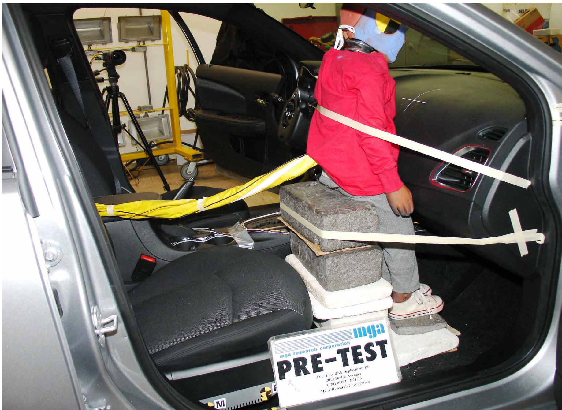
Pre-Test 3YO P1 Passenger Dummy Right Side View
