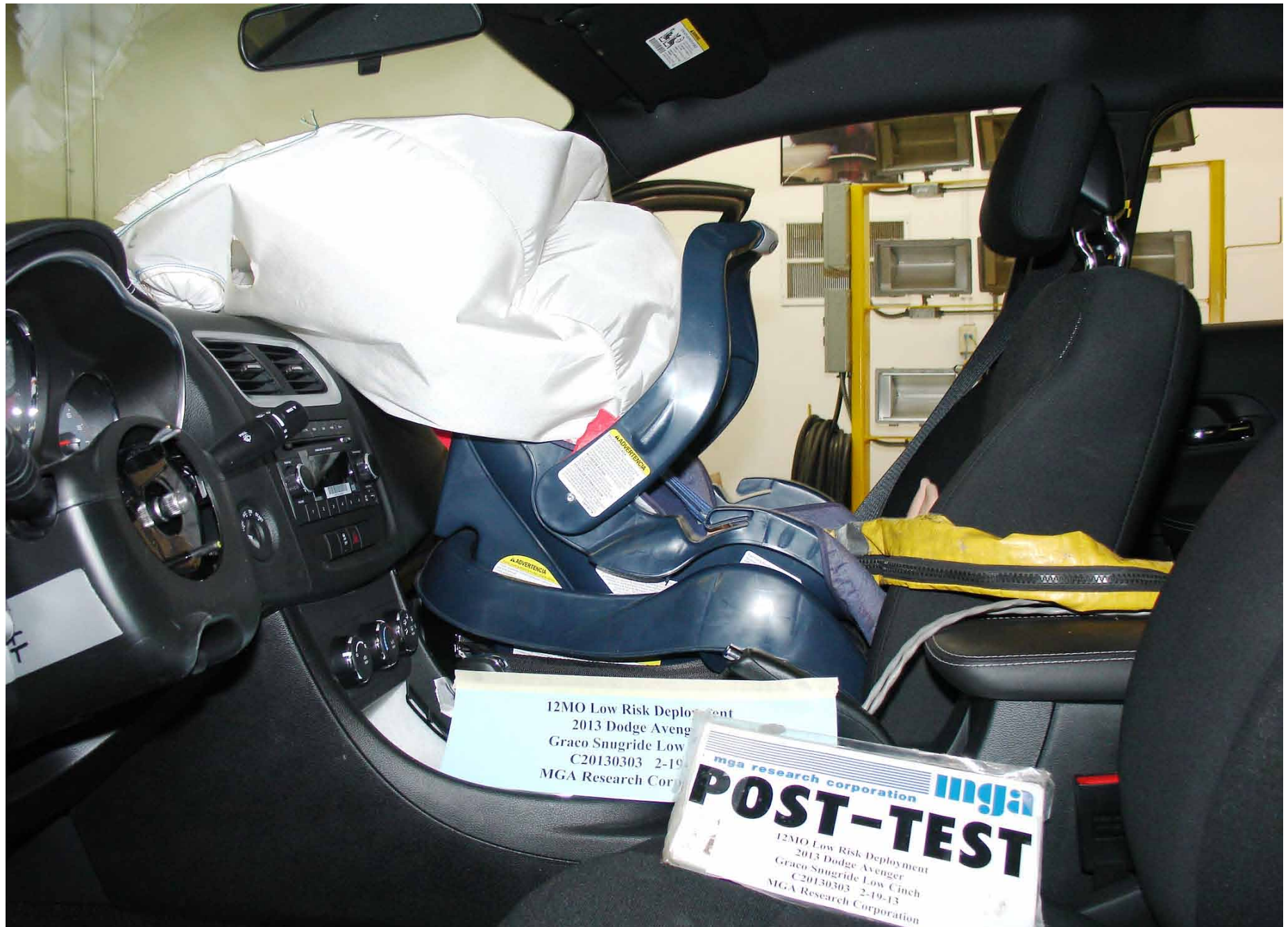
Post-Test 12 Mo Pass. Dummy Left Side View (Graco Snugride W/Base Low Cinch)
