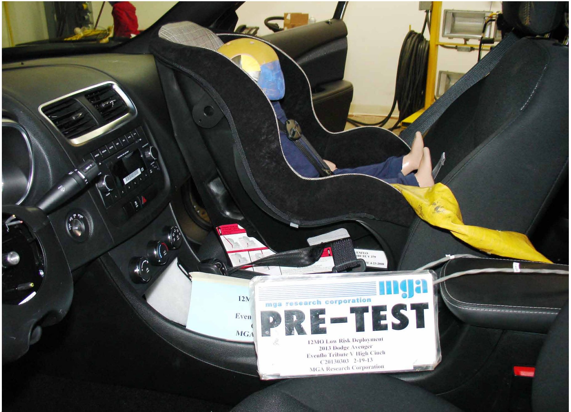
Pre-Test 12 Mo Pass. Dummy Left Side View (Evenflo Tribute High Cinch)
