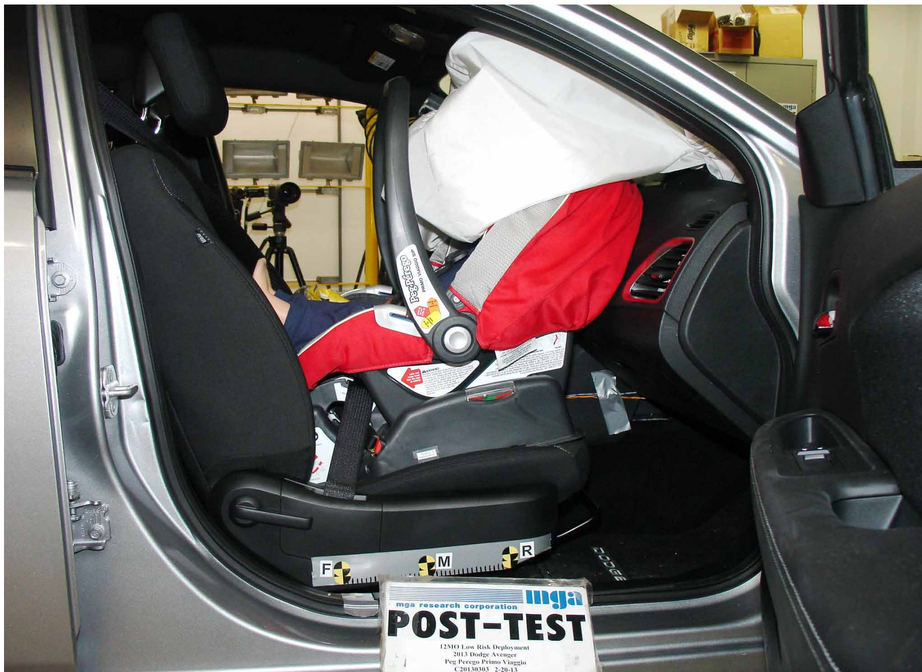
Post-Test 12 Mo Pass. Dummy Right Side View (Peg Perego Primo Viaggio W/Base Low Cinch)
