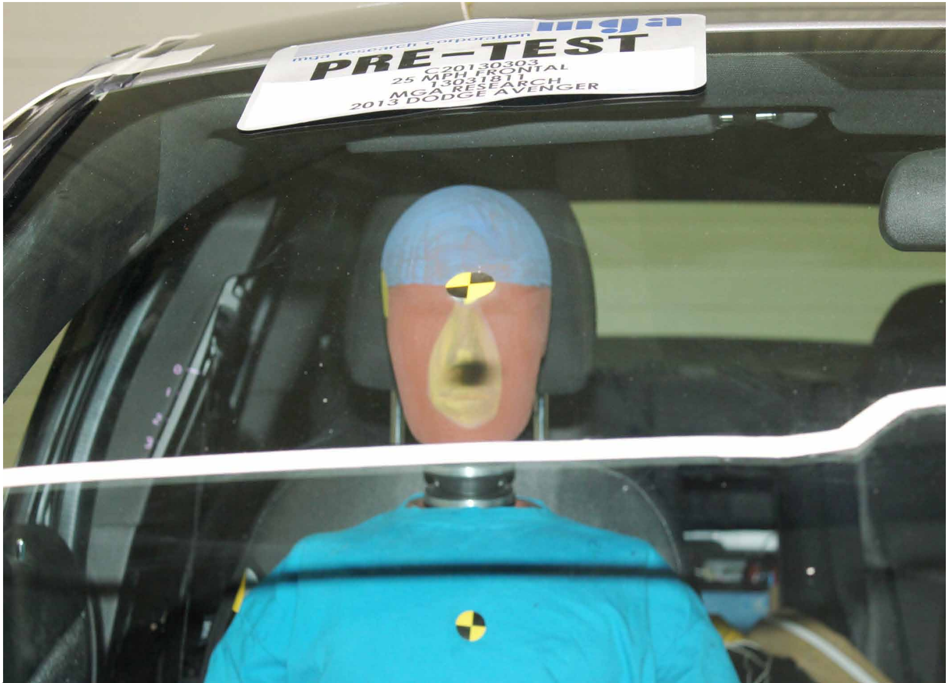
Pre-Test Passenger Dummy Front View (head position)
