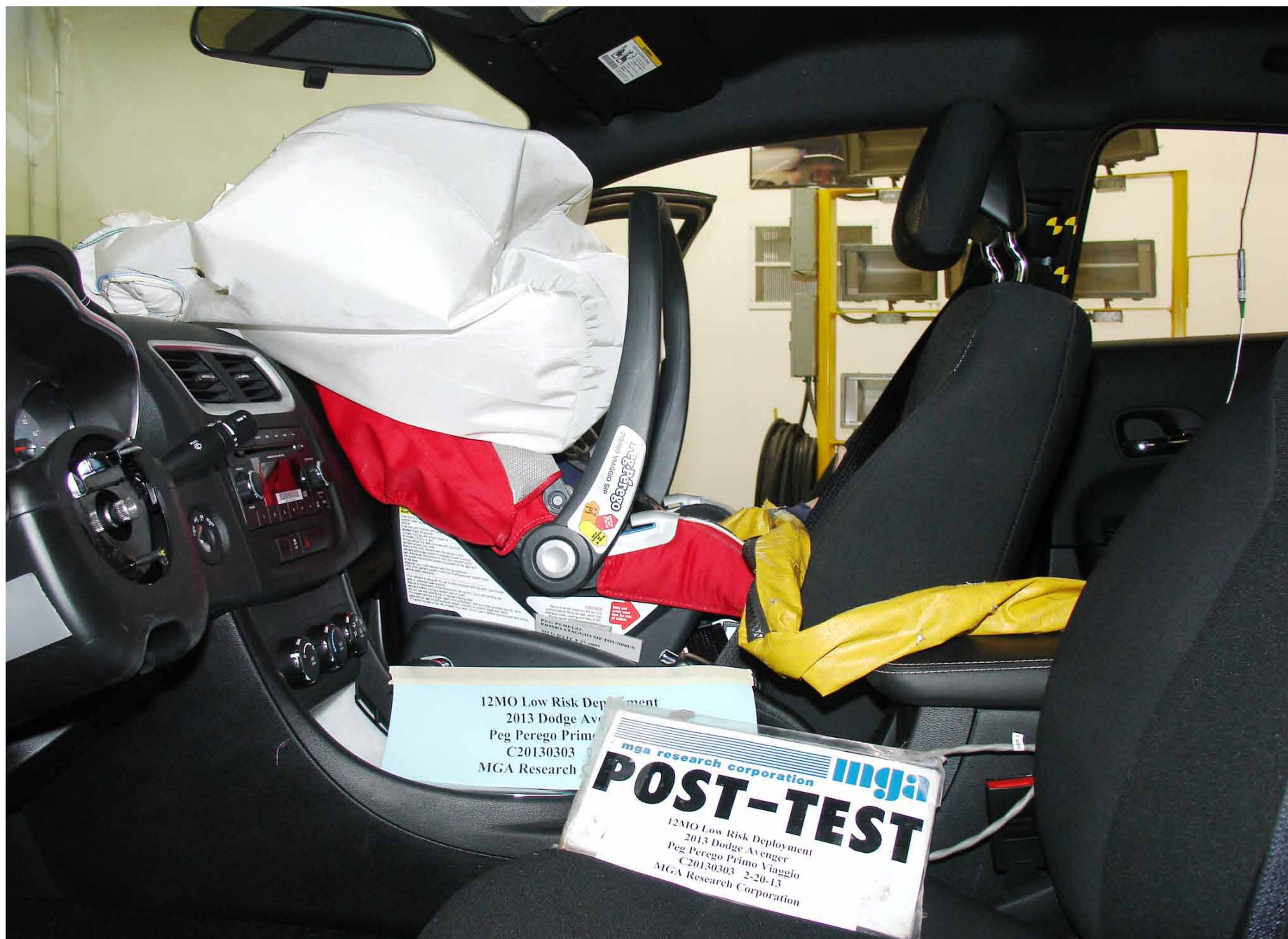
Post-Test 12 Mo Pass. Dummy Left Side View (Peg Perego Primo Viaggio W/Base Low Cinch)
