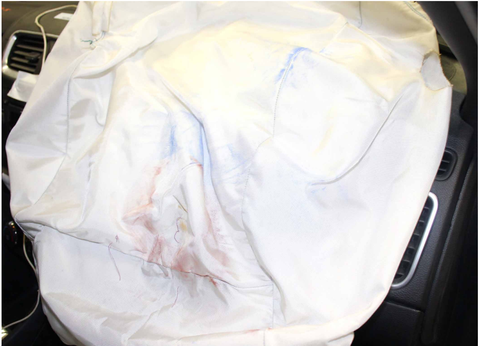
Post-Test Passenger Dummy Airbag Contact
