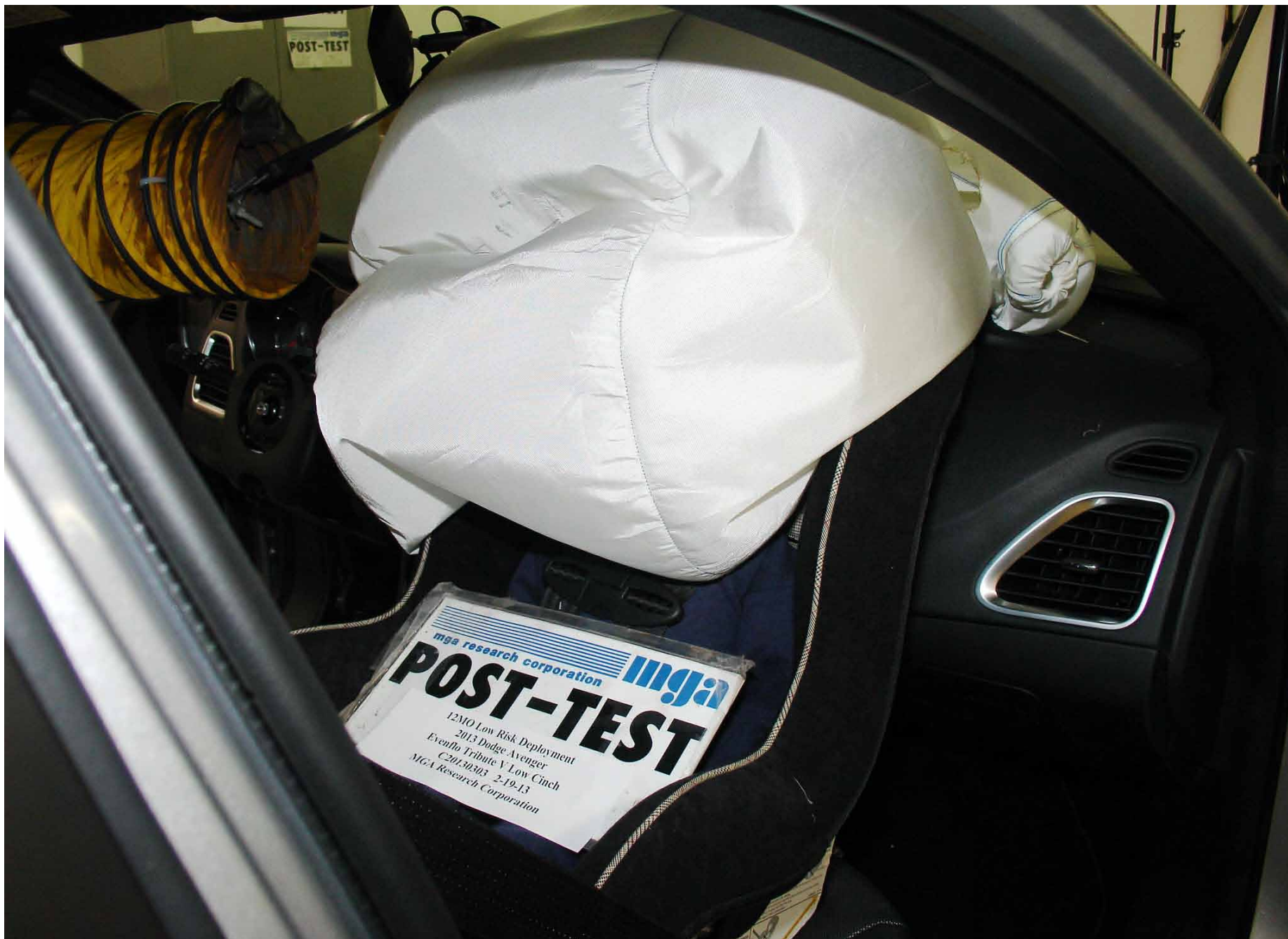
Post-Test 12 Mo Pass. Dummy Airbag Right Side View
