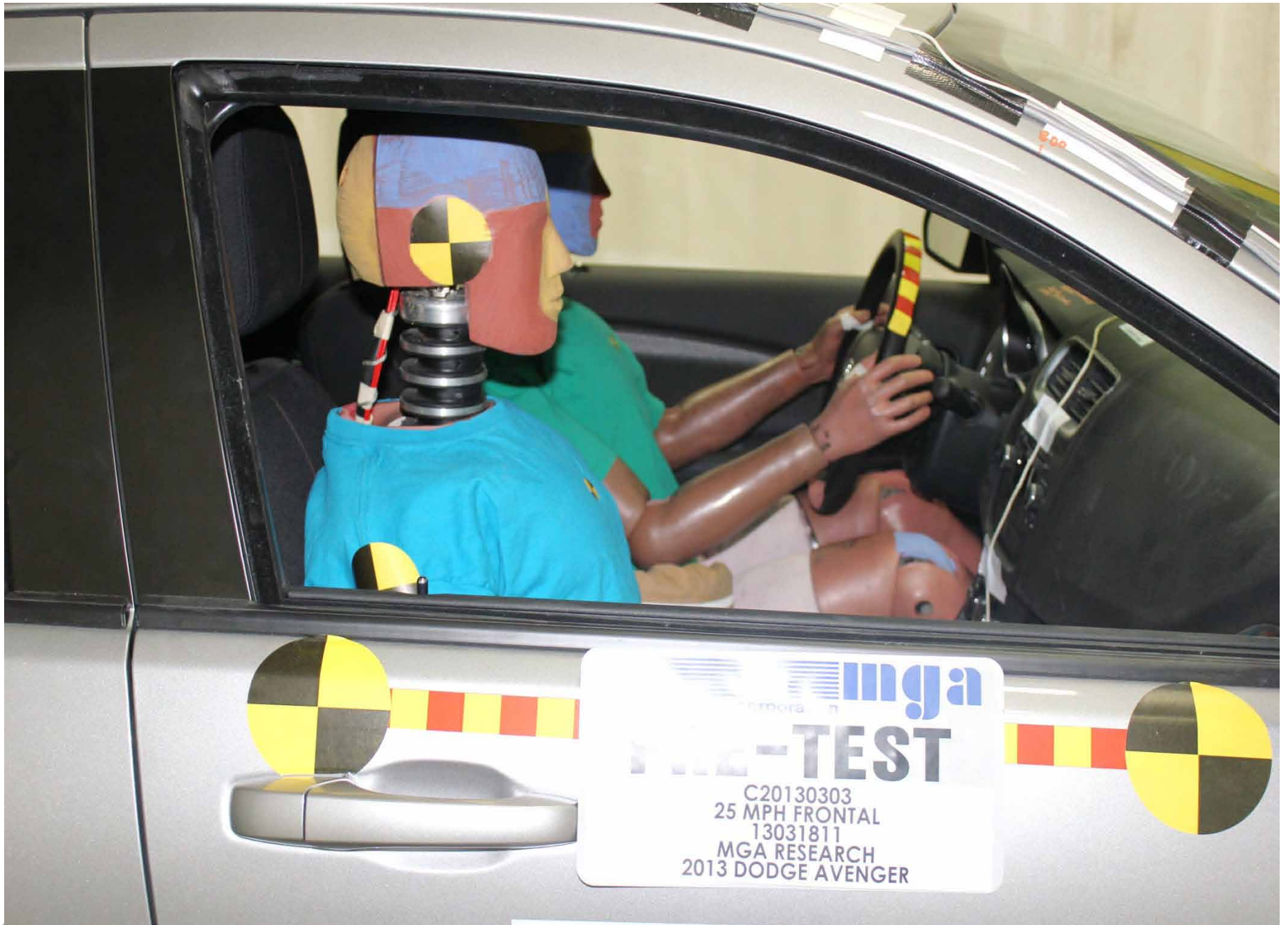
Pre-Test Passenger Dummy Position Right Side View
