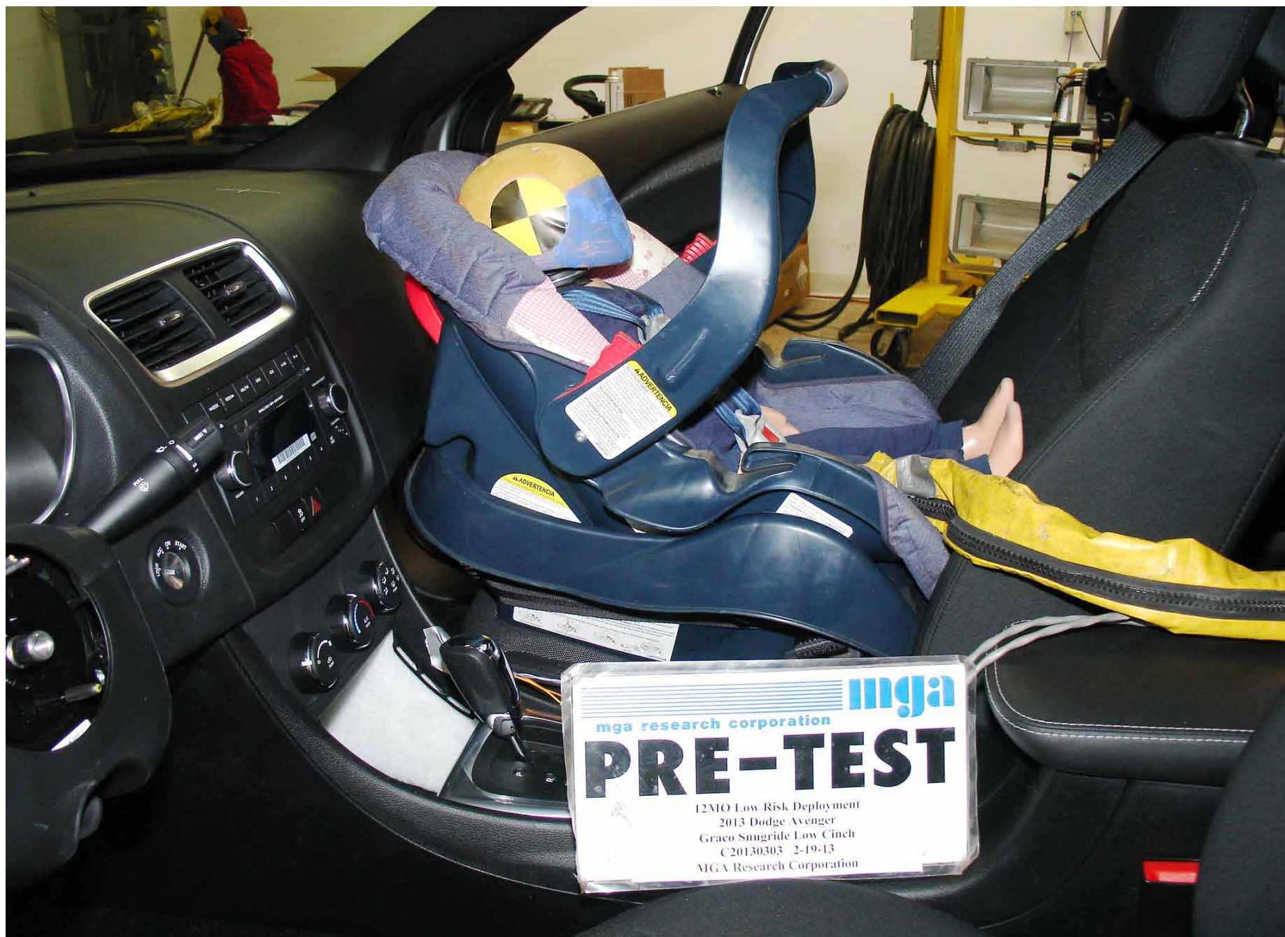
Pre-Test 12 Mo Pass. Dummy Left Side View (Graco Snugride W/Base Low Cinch)
