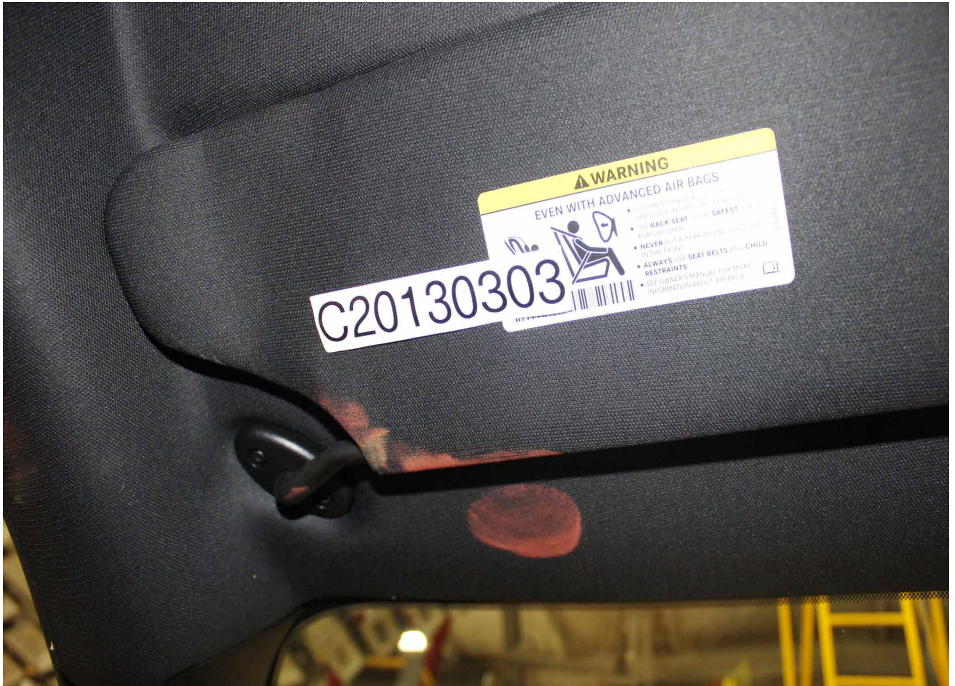
Post-Test Driver Dummy Head Contact (visor, headliner)
