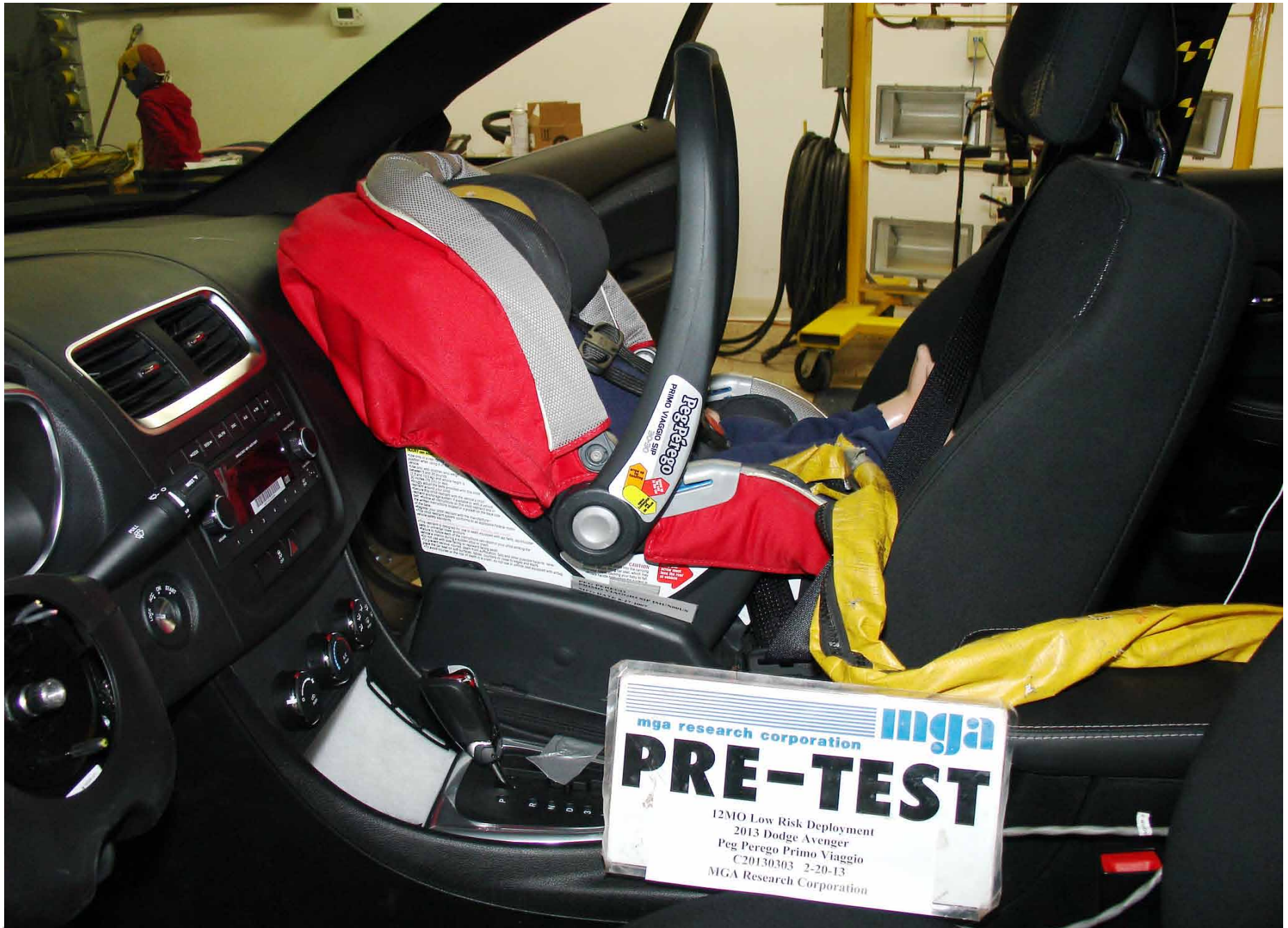
Pre-Test 12 Mo Pass. Dummy Left Side View (Peg Perego Primo Viaggio W/Base Low Cinch)
