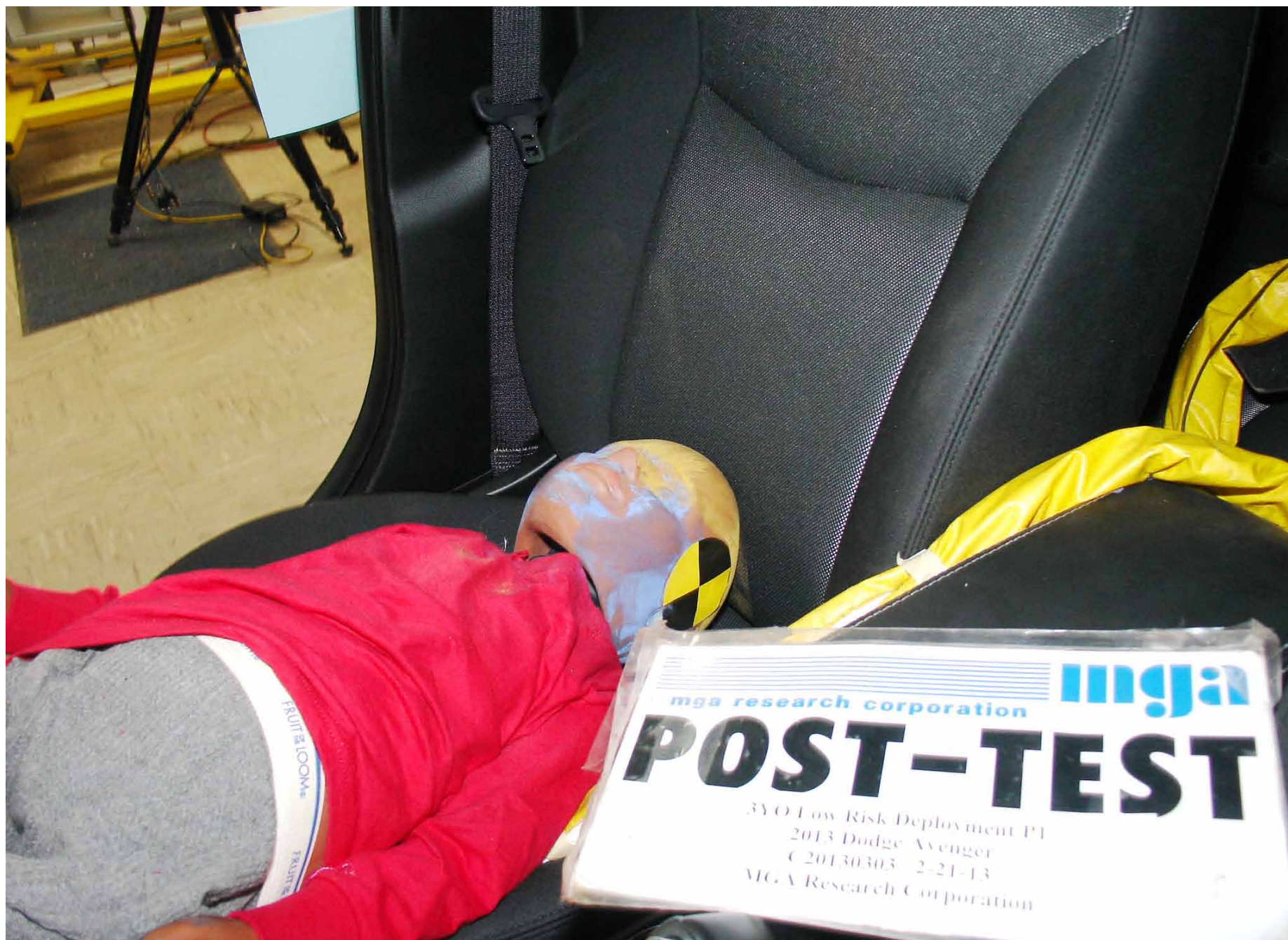
Post-Test 3YO P1 Passenger Dummy Head Contact (seat back)
