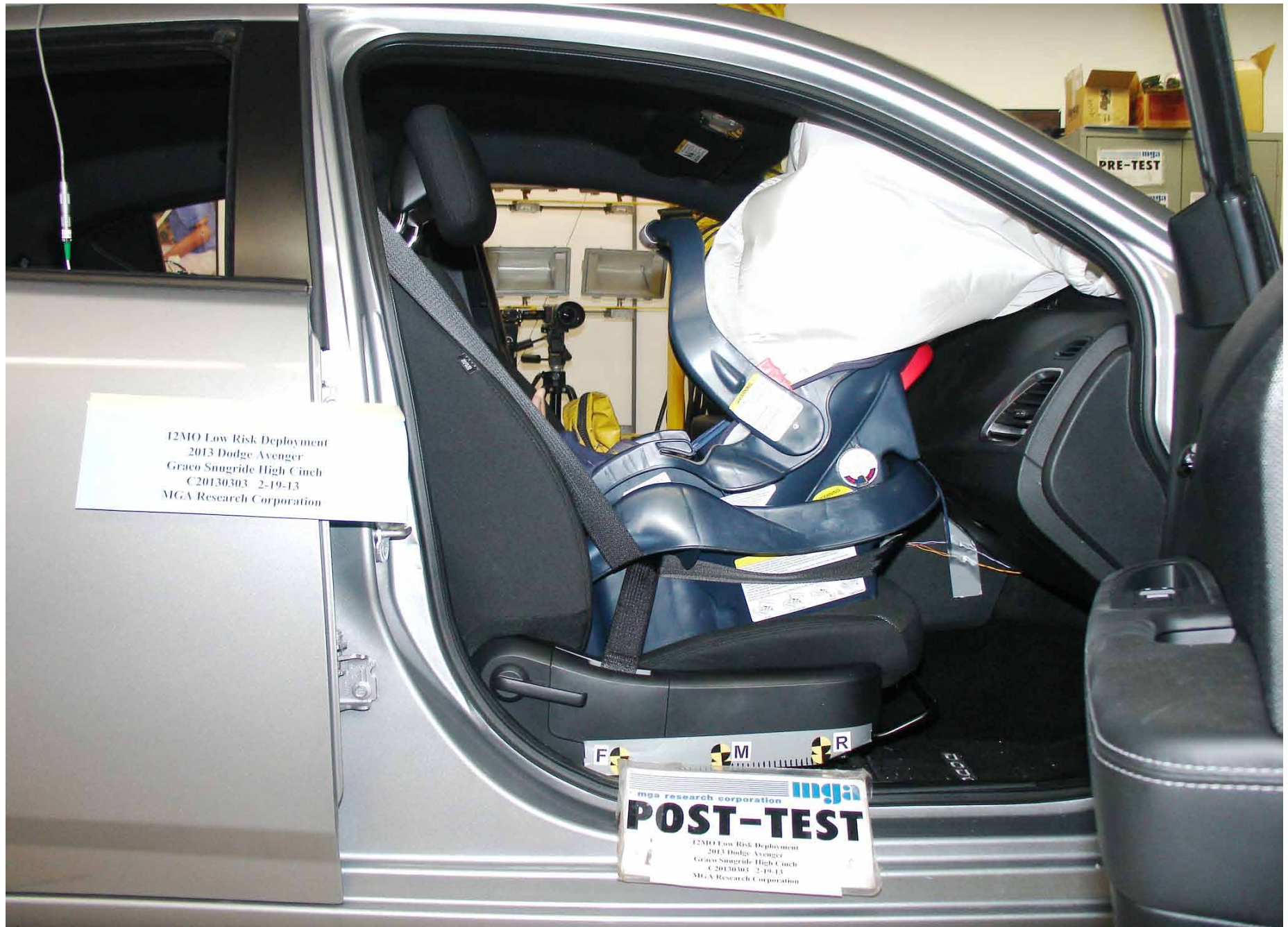
Post-Test 12 Mo Pass. Dummy Right Side View (Graco Snugride W/Base High Cinch)
