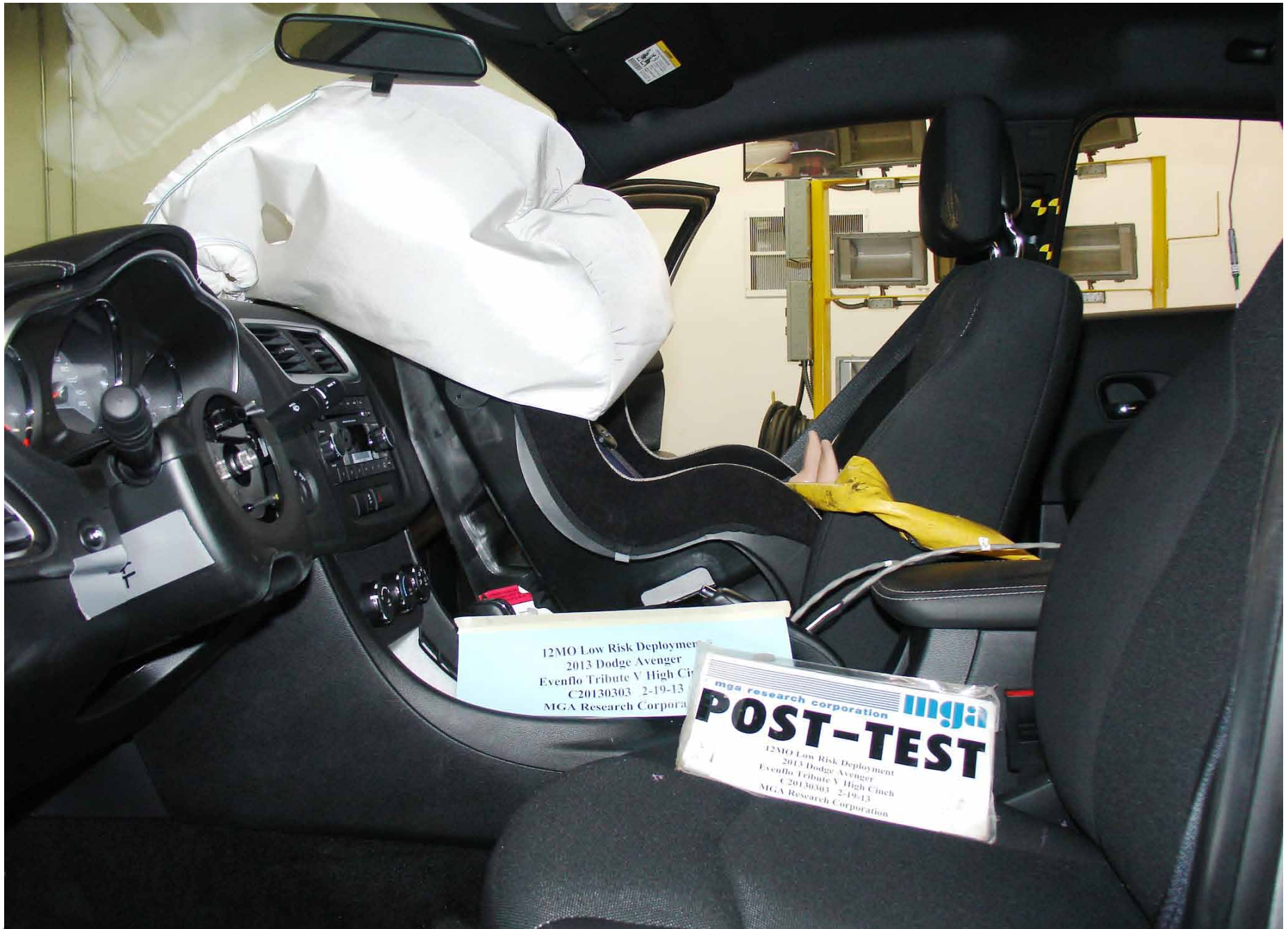
Post-Test 12 Mo Pass. Dummy Left Side View (Evenflo Tribute High Cinch)
