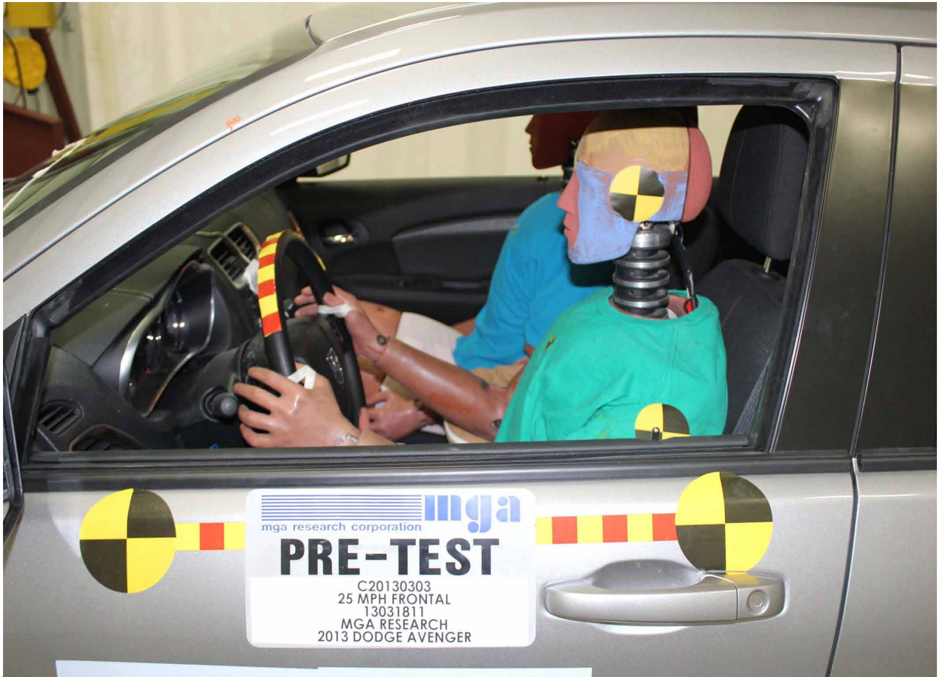
Pre-Test Driver Dummy Position Left Side View
