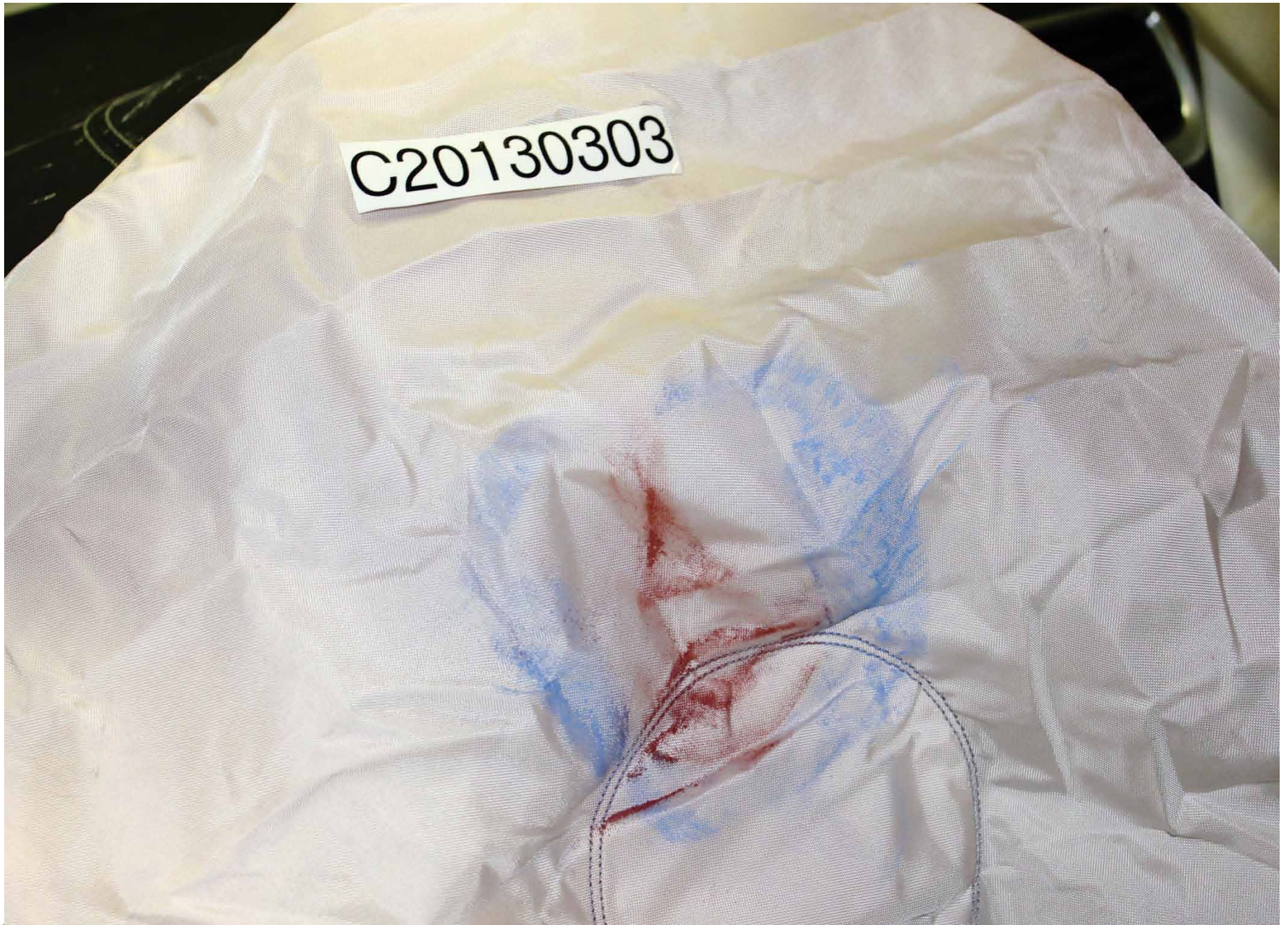
Post-Test Driver Dummy Airbag Contact
