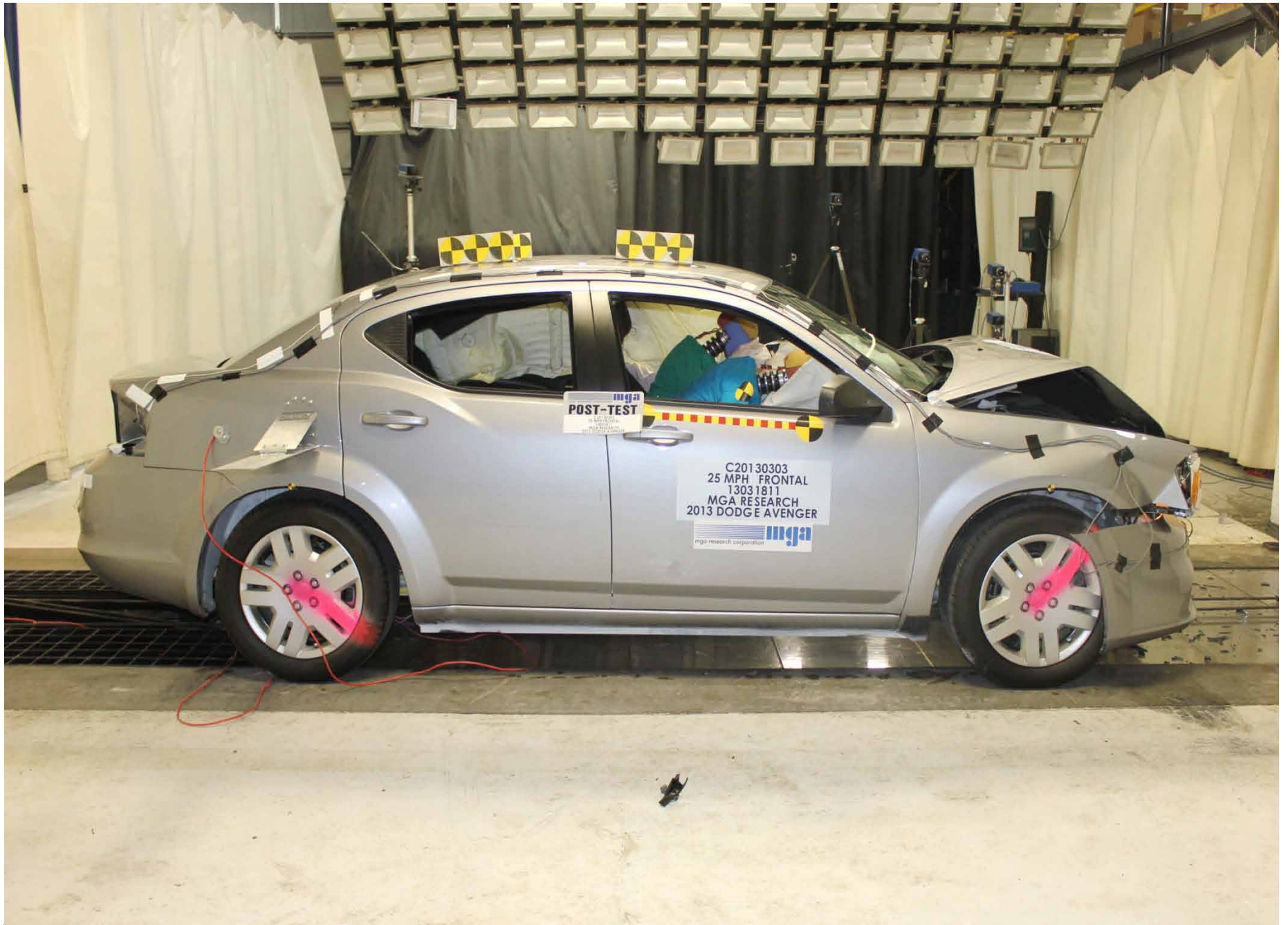
Post-Test Right Side View of Test Vehicle
