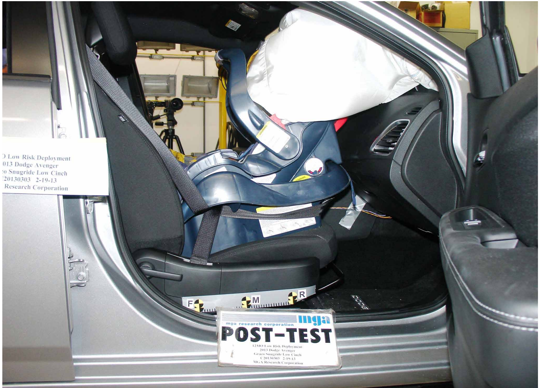
Post-Test 12 Mo Pass. Dummy Right Side View (Graco Snugride W/Base Low Cinch)
