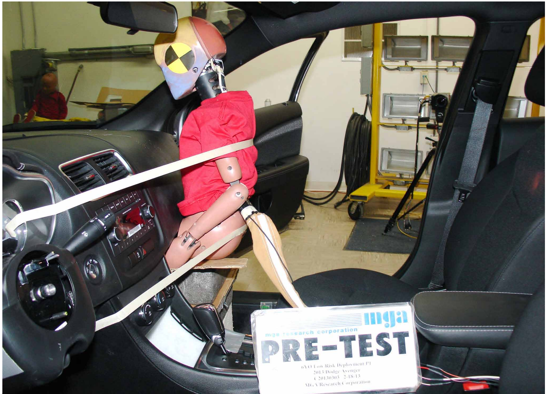
Pre-Test 6YO P1 Passenger Dummy Left Side View
