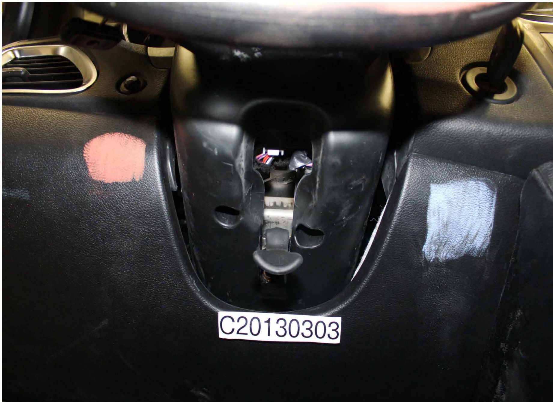
Post-Test Driver Dummy Knee Contact
