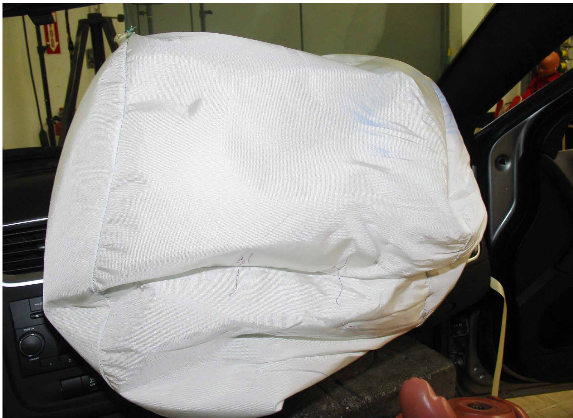
Post-Test 6YO P1 Passenger Dummy Airbag Left Side View
