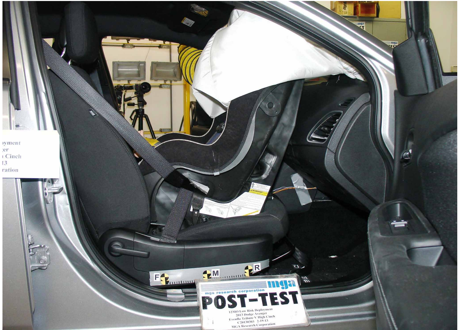
Post-Test 12 Mo Pass. Dummy Right Side View (Evenflo Tribute High Cinch)
