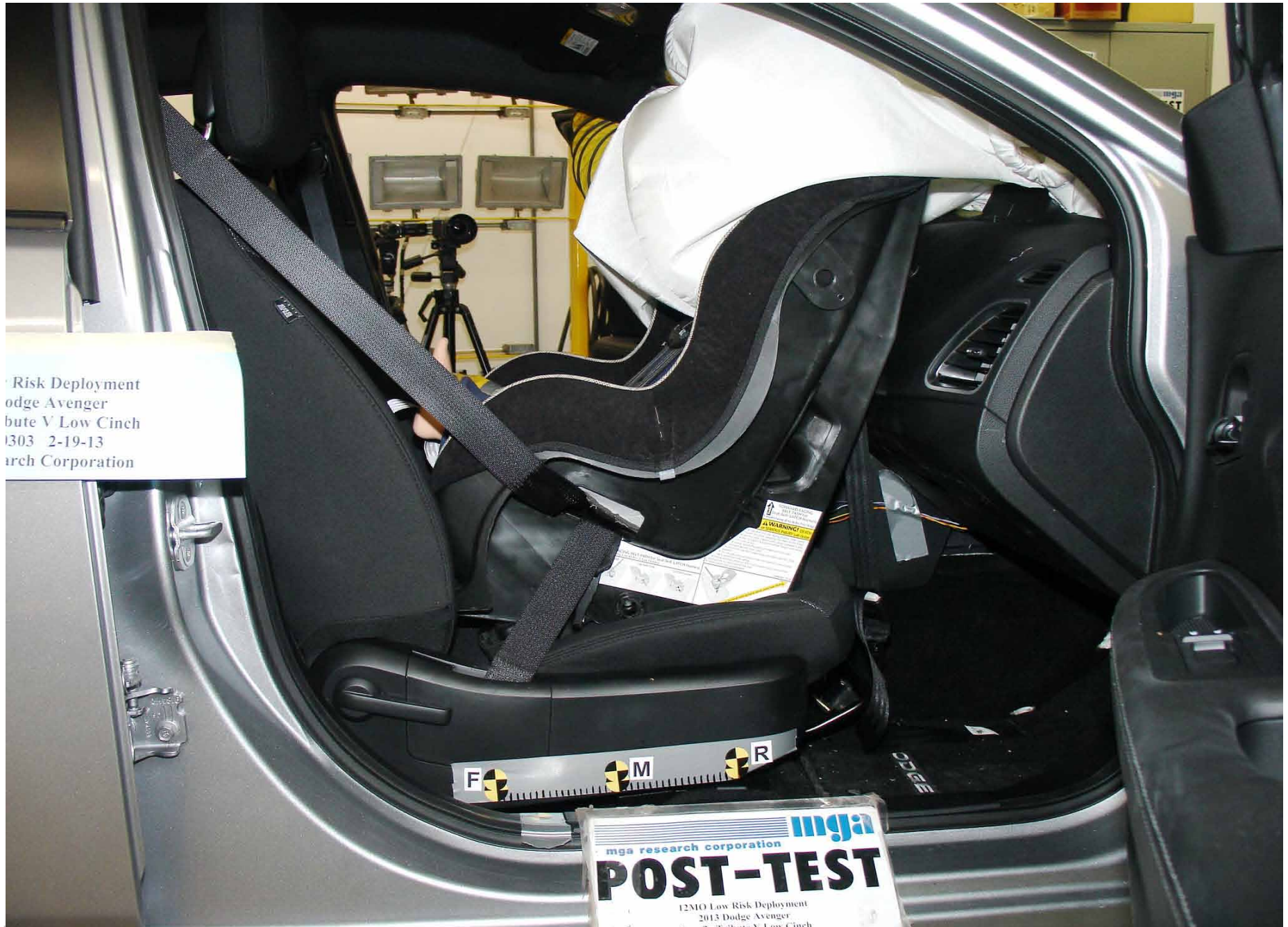
Post-Test 12 Mo Pass. Dummy Right Side View (Evenflo Tribute Low Cinch)
