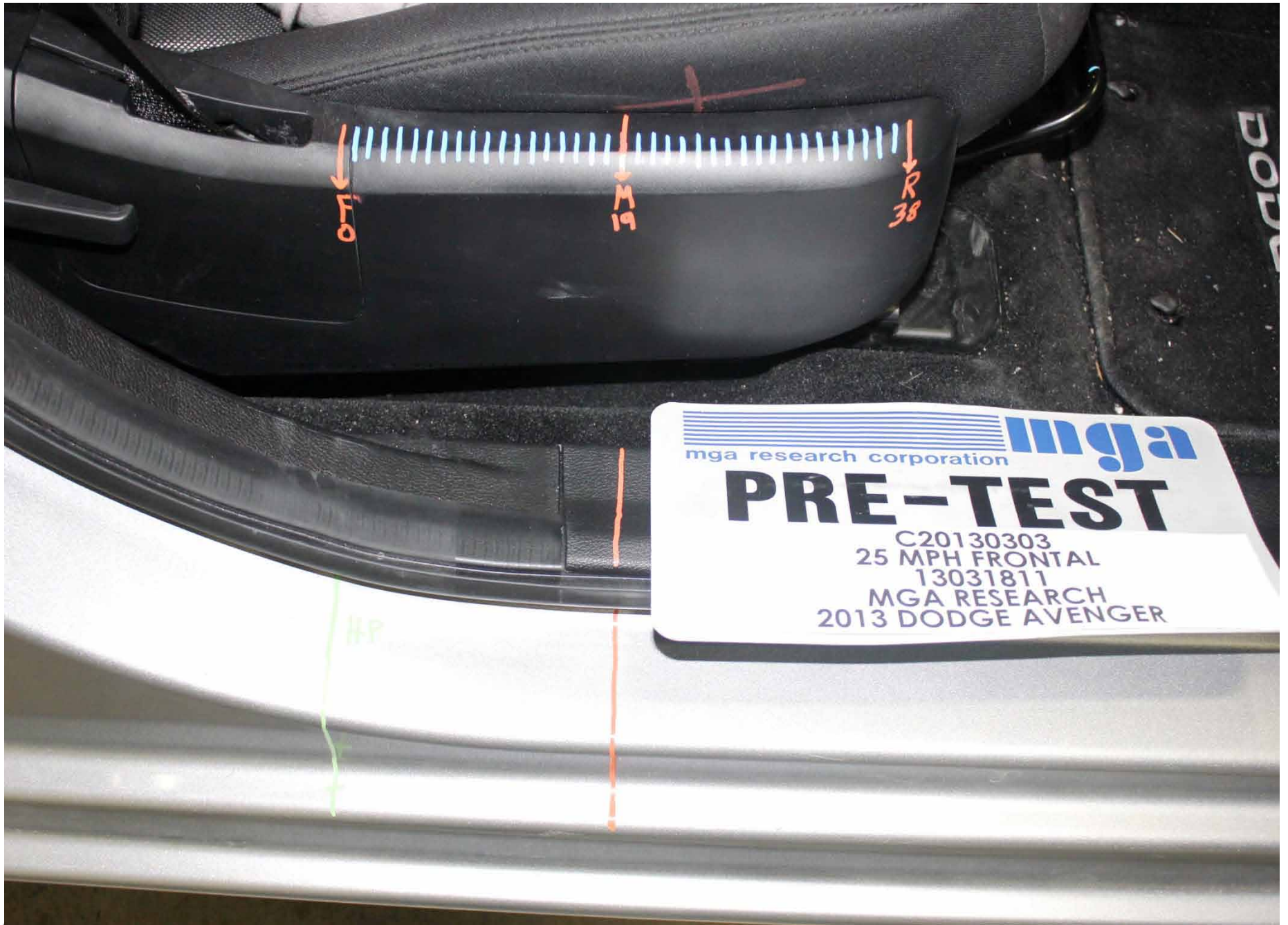
Pre-Test Passenger Dummy Seat Position
