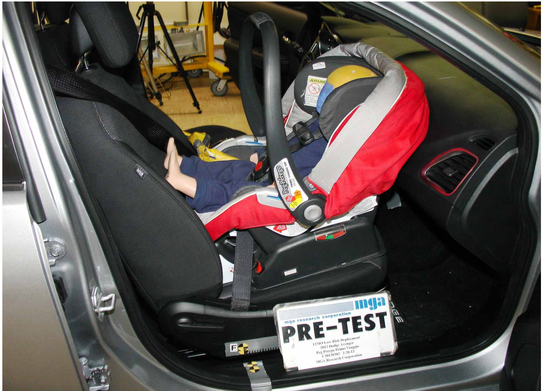
Pre-Test 12 Mo Pass. Dummy Right Side View (Peg Perego Primo Viaggio W/Base Low Cinch)
