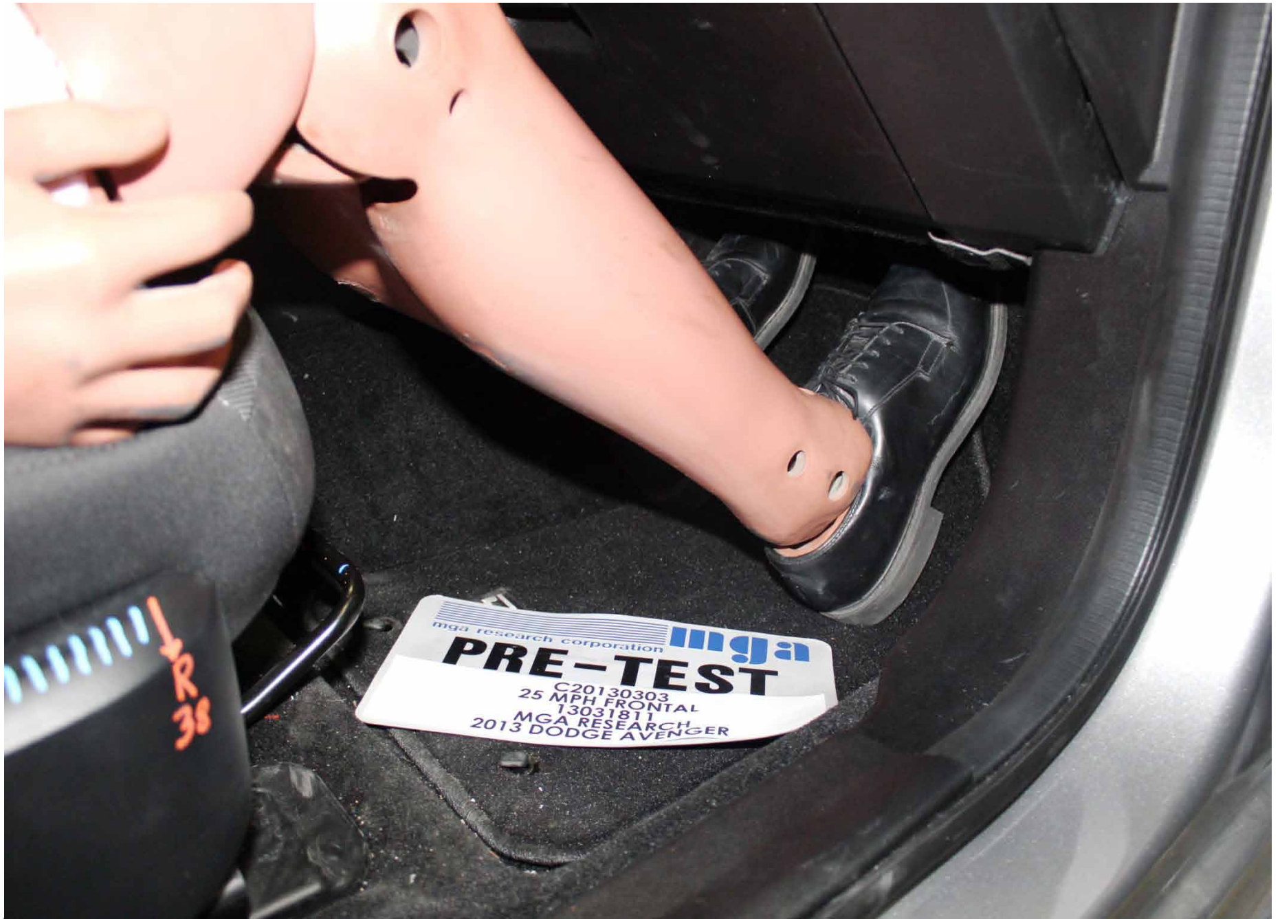
Pre-Test Passenger Dummy Feet Position
