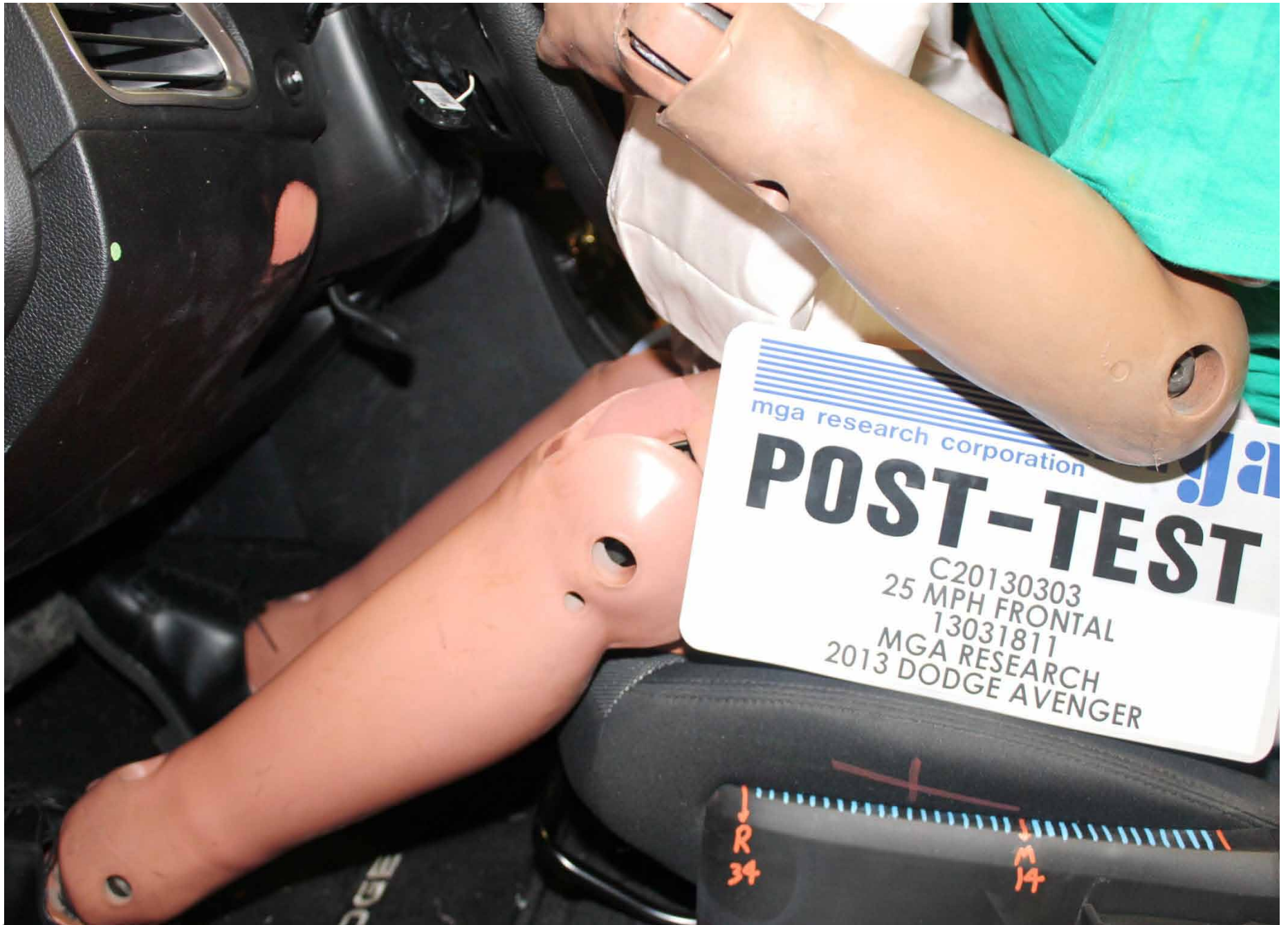
Post-Test Driver Side Knee Bolster View
