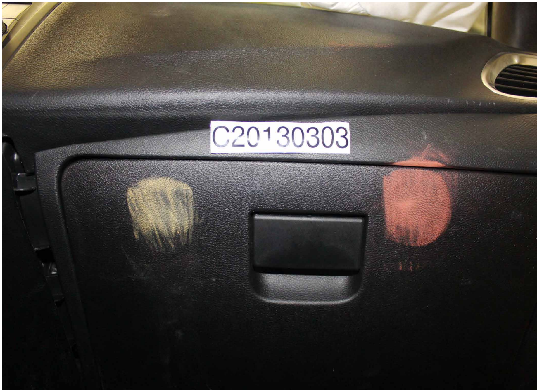
Post-Test Passenger Dummy Knee Contact
