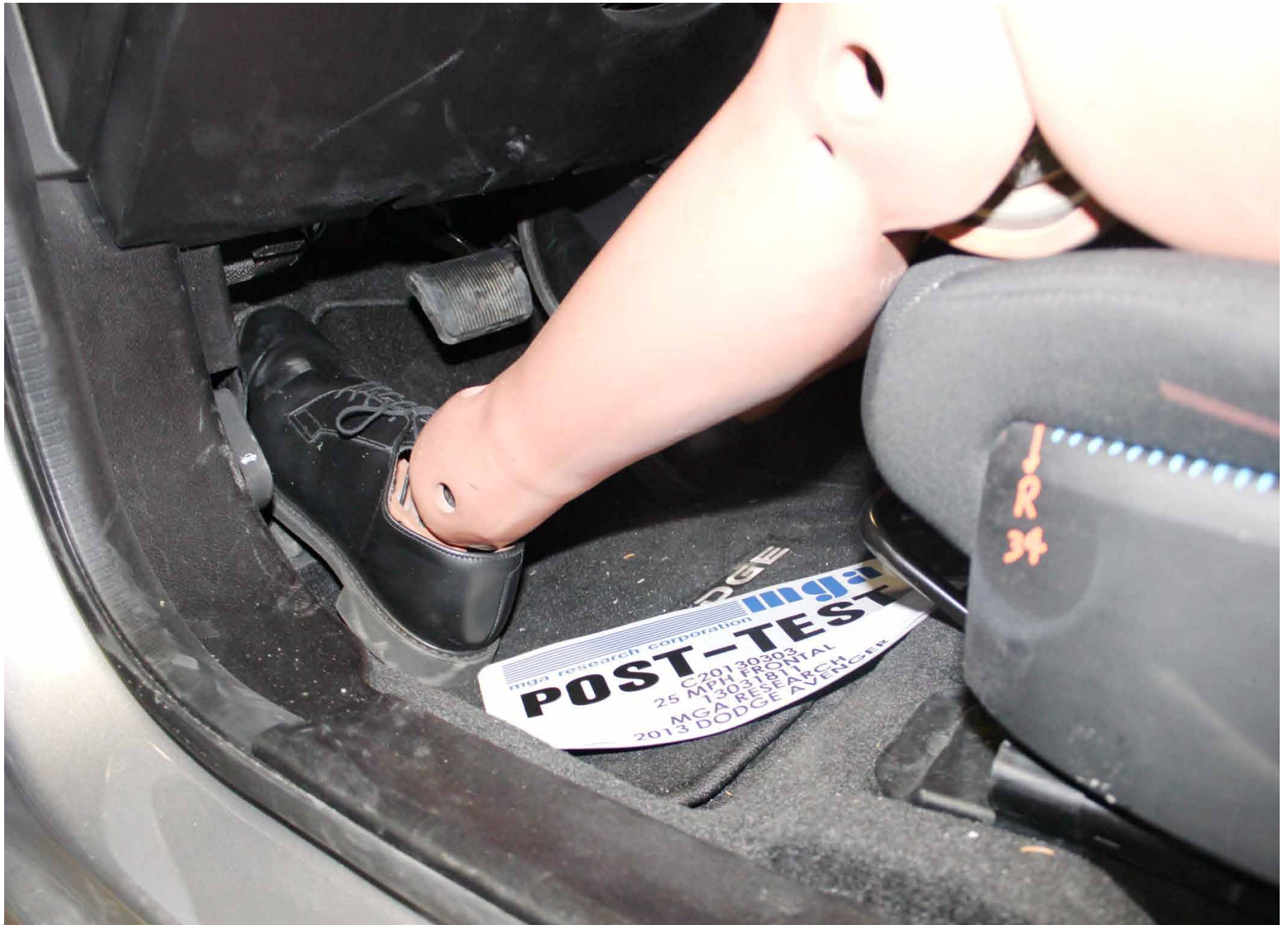
Post-Test Driver Dummy Feet Position
