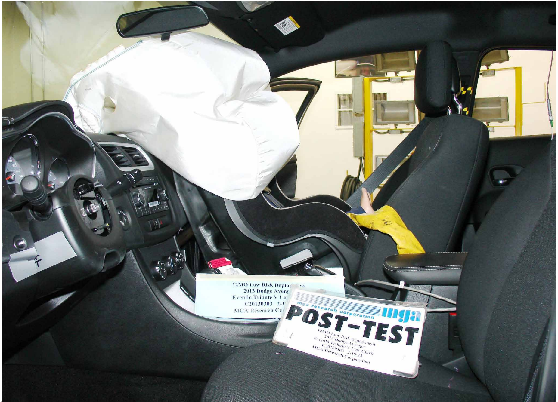
Post-Test 12 Mo Pass. Dummy Left Side View (Evenflo Tribute Low Cinch)
