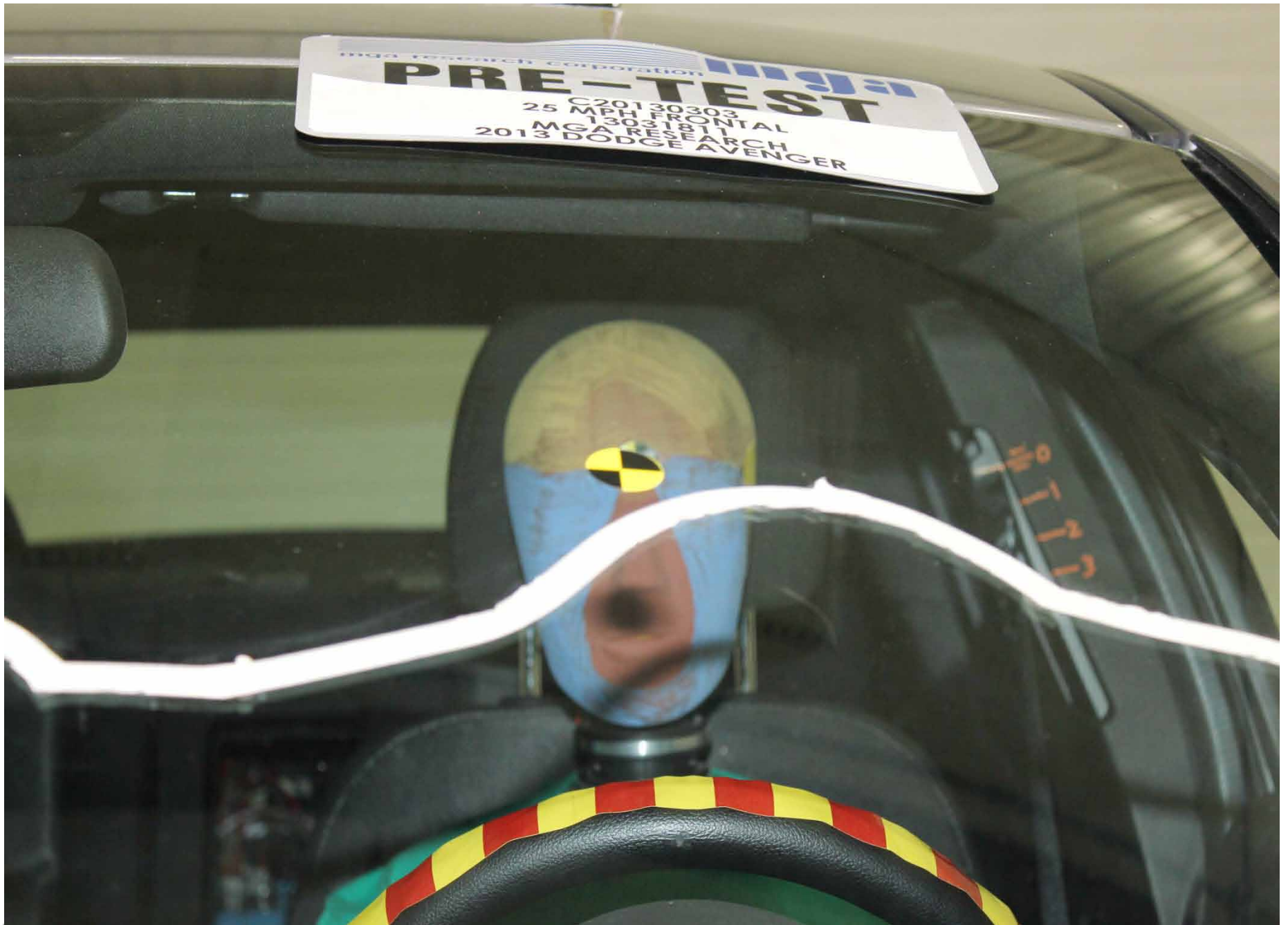
Pre-Test Driver Dummy Front View (head position)
