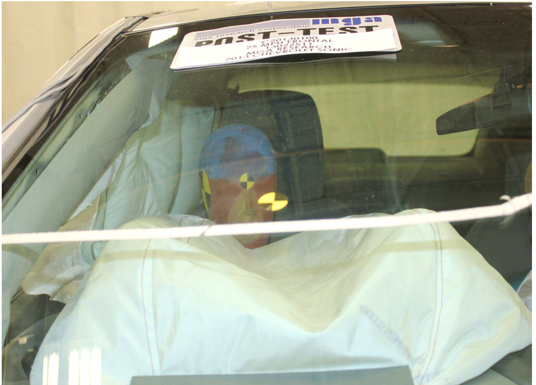
Post-Test Passenger Dummy Front View (head position)
