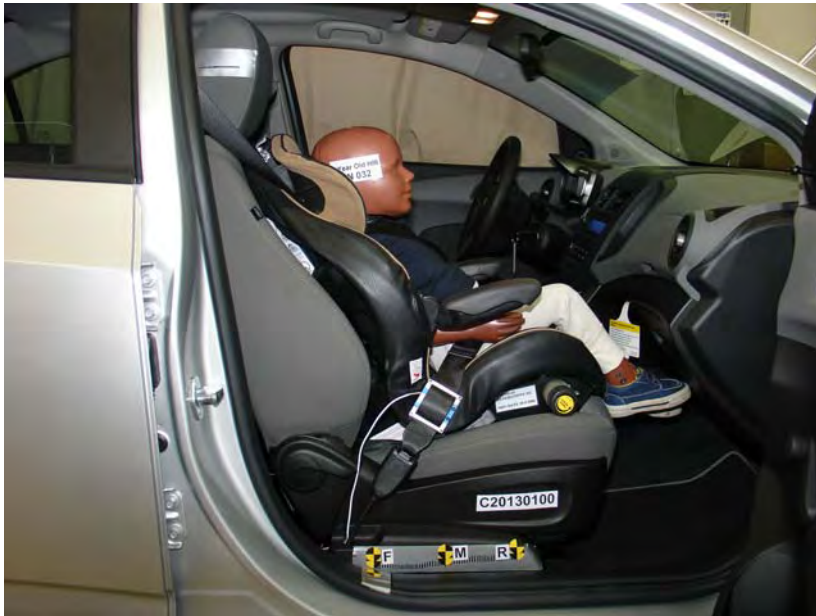
3-Year-Old Forward Facing Evenflo Generations Belted, Forward Seat Track
