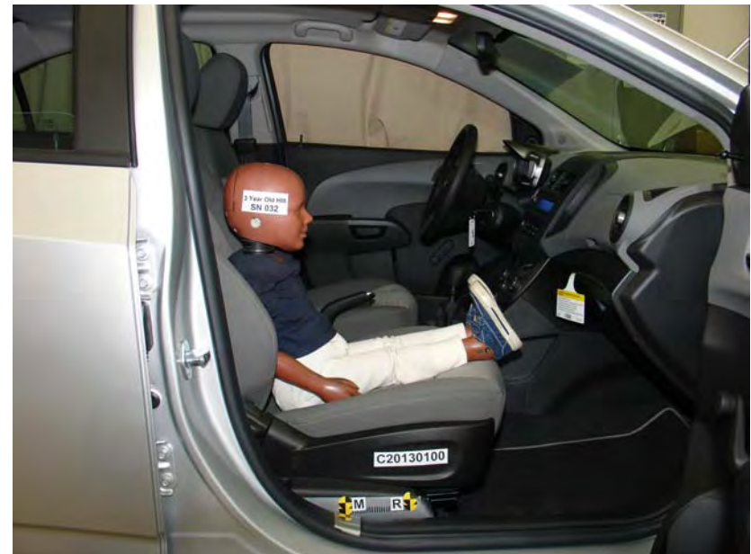
3-Year-Old Unbelted, Middle Seat Track, Position 1
