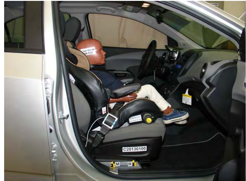
3-Year-Old Forward Facing Evenflo Generations Belted, Middle Seat Track
