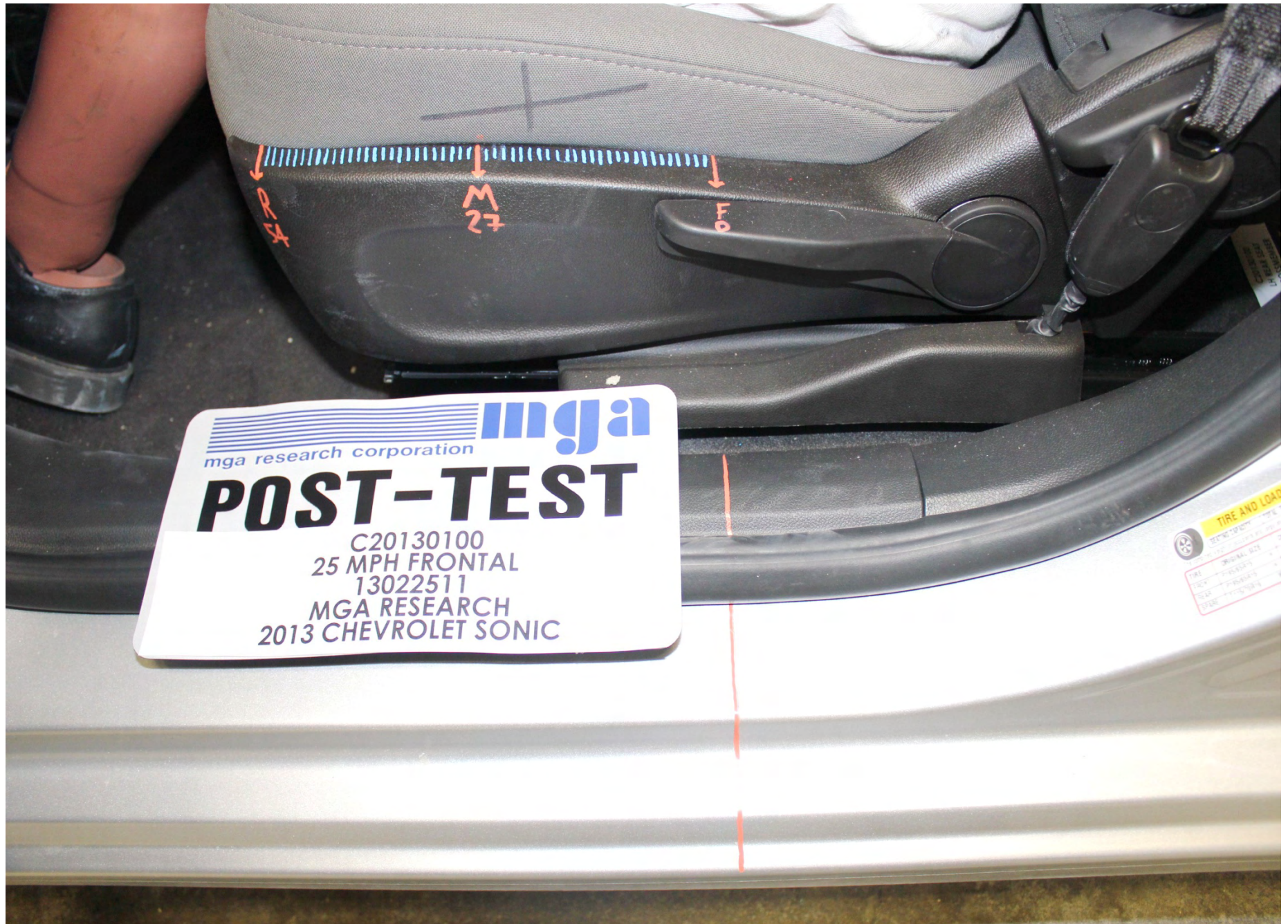
Post-Test Driver Dummy Seat Position
