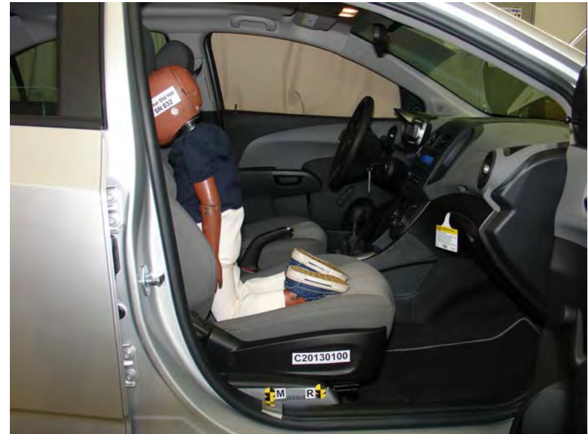
3-Year-Old Unbelted, Middle Seat Track, Position 7
