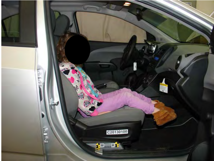
6-Year-Old Unbelted, Middle Seat Track, Position 1
