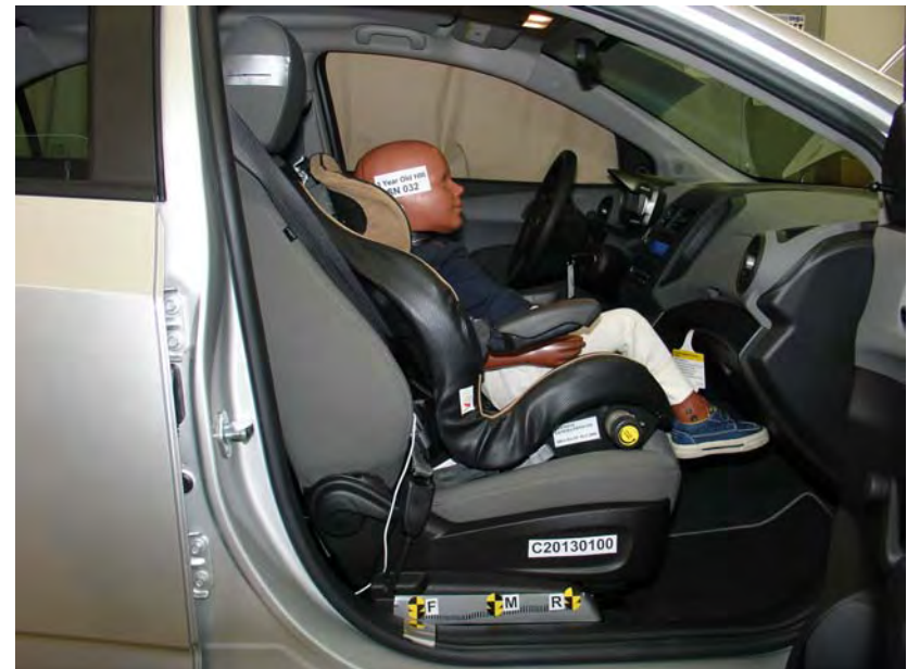
3-Year-Old Forward Facing Evenflo Generations Cinched With Harness, Forward Seat Track
