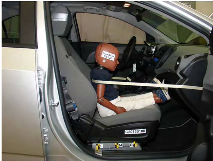
3-Year-Old Unbelted, Forward Seat Track, Position 3
