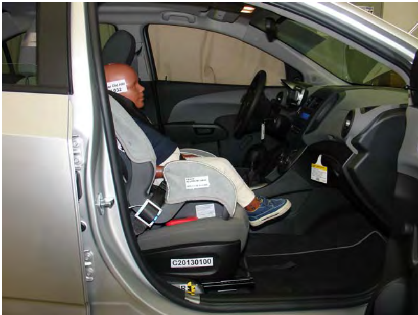
3-Year-Old Graco Platinum Cargo Belted, Rearward Seat Track
