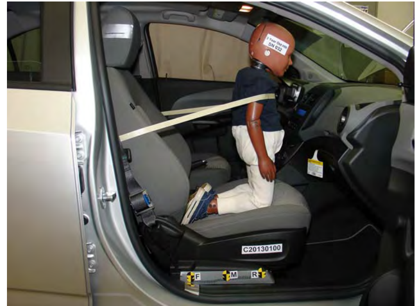
3-Year-Old Unbelted, Forward Seat Track, Position 6
