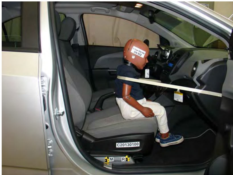
3-Year-Old Unbelted, Middle Seat Track, Position 4
