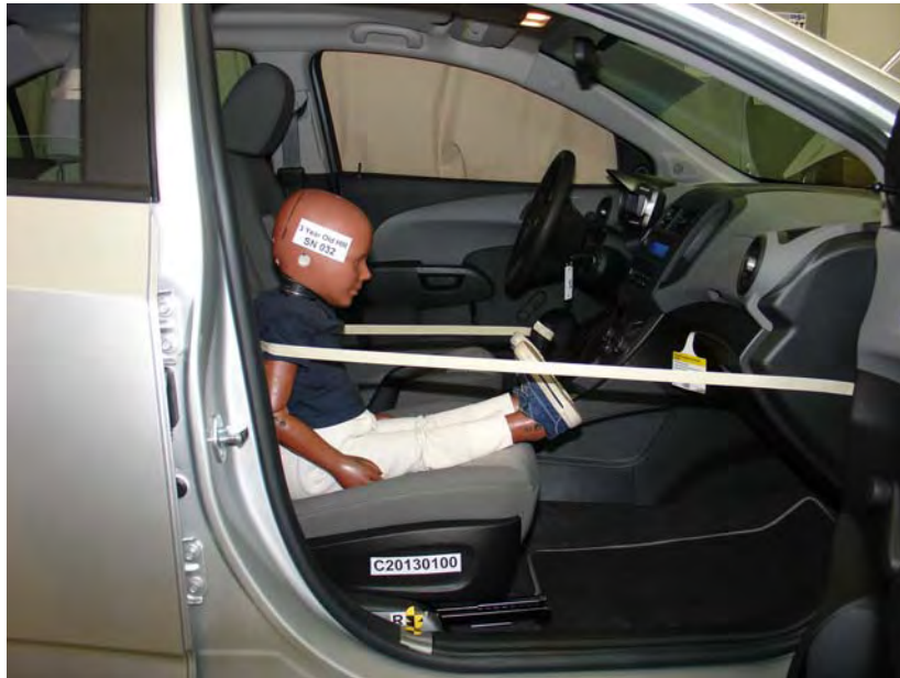
3-Year-Old Unbelted, Rearward Seat Track, Position 3
