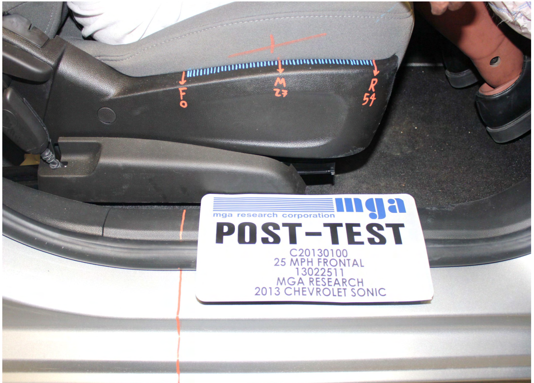
Post-Test Passenger Dummy Seat Position
