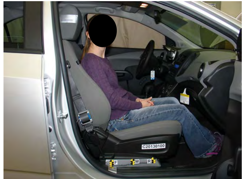
Unbelted 5th Percentile Female Representative Reactivation, Forward Seat Track
