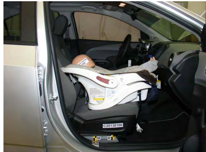
Cosco Arriva WBase, Unbelted, Forward Facing, Middle Seat Track
