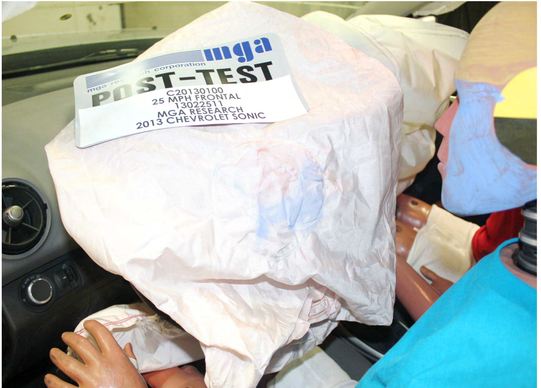
Post-Test Driver Dummy Airbag Contact
