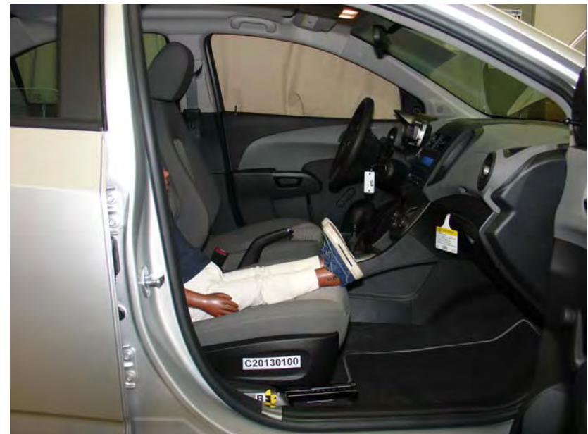
3-Year-Old Unbelted, Rearward Seat Track, Position 2
