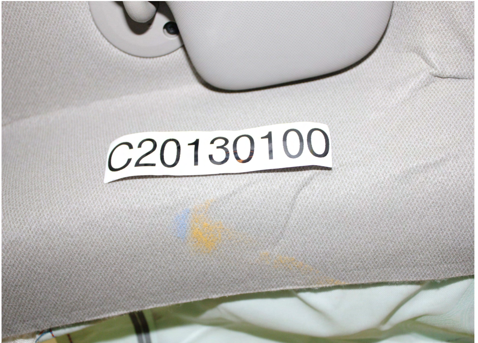
Post-Test Passenger Dummy Head Contact (headliner)
