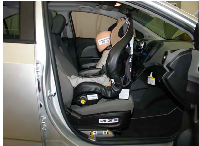
Evenflo Generations Rear Facing Unbelted, Middle Seat Track
