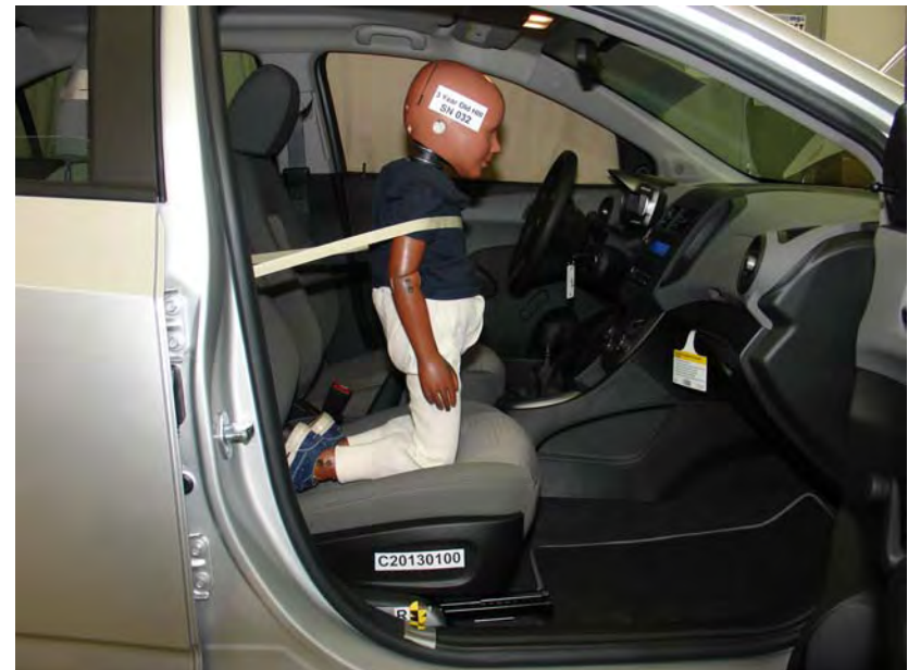
3-Year-Old Unbelted, Rearward Seat Track, Position 6
