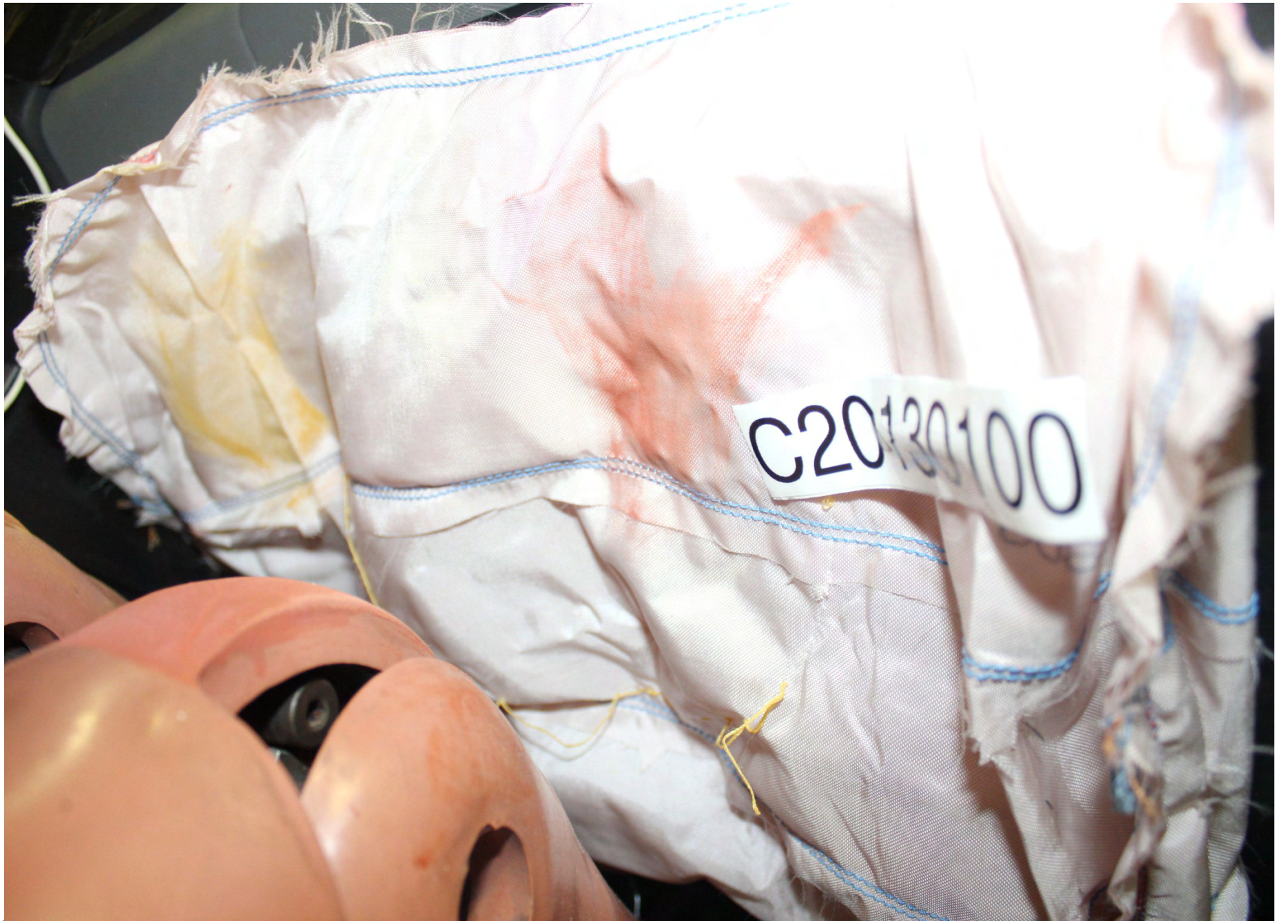
Post-Test Passenger Dummy Knee Contact (knee restraint)
