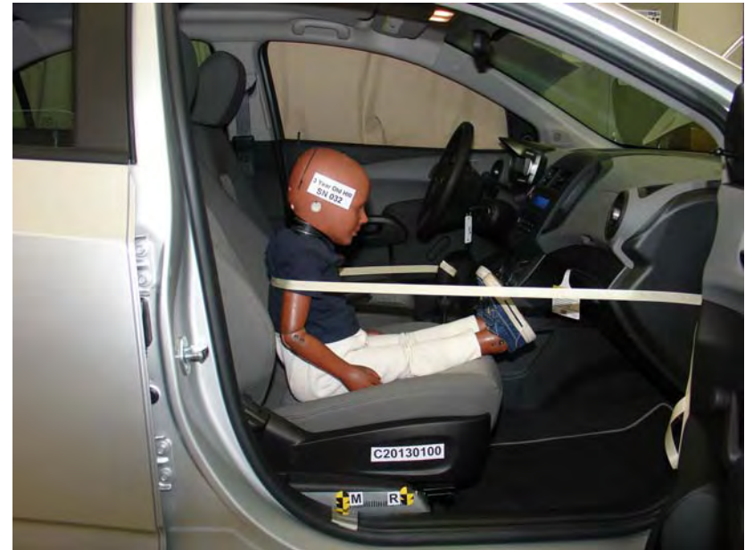
3-Year-Old Unbelted, Middle Seat Track, Position 3
