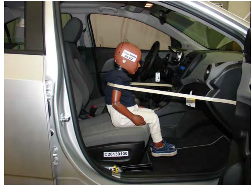
3-Year-Old Unbelted, Rearward Seat Track, Position 4
