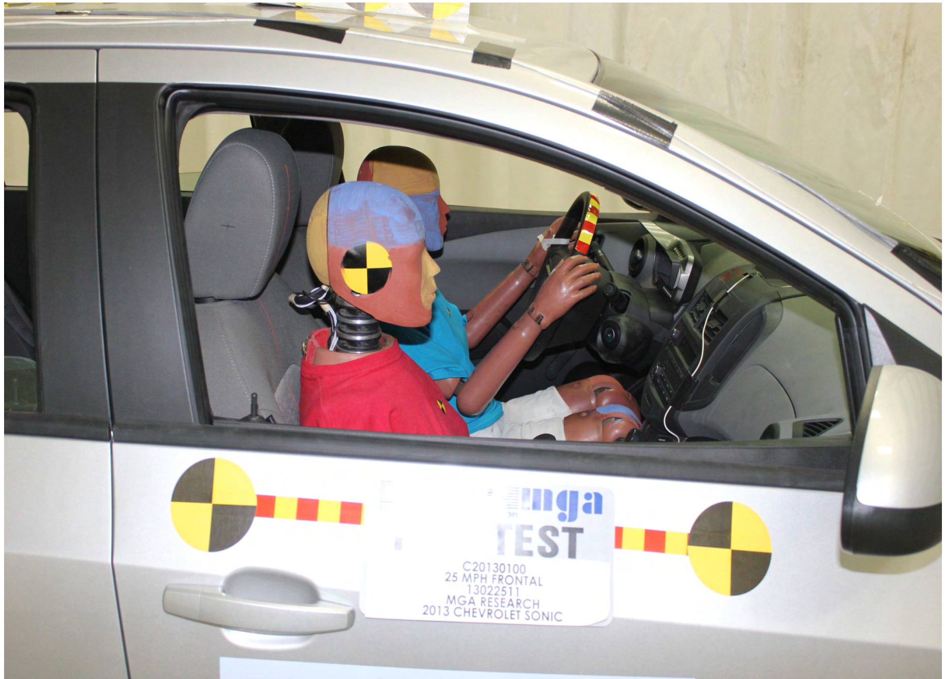
Pre-Test Passenger Dummy Position Right Side View
