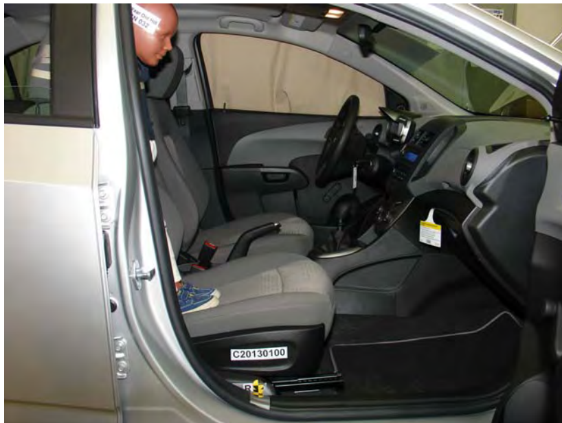
3-Year-Old Unbelted, Rearward Seat Track, Position 5
