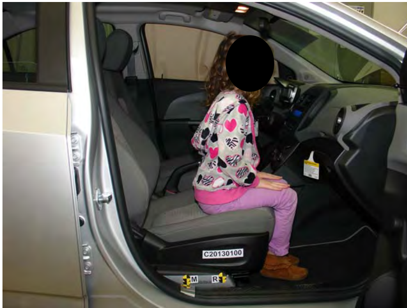
6-Year-Old Unbelted, Middle Seat Track, Position 3
