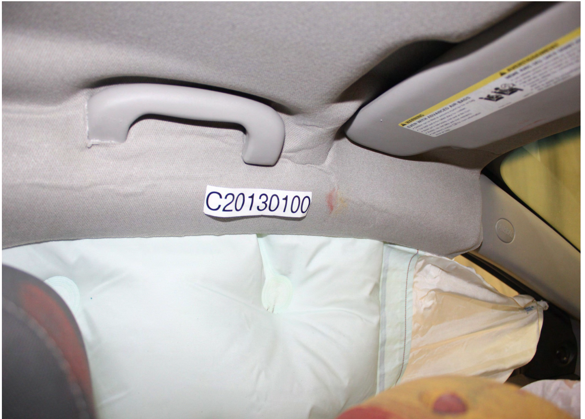
Post-Test Driver Dummy Head Contact (headliner)
