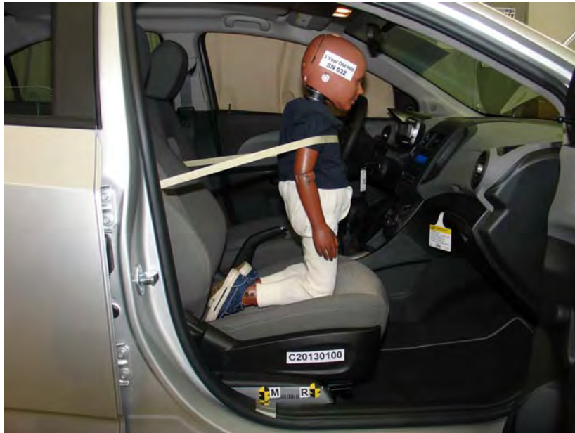
3-Year-Old Unbelted, Middle Seat Track, Position 6
