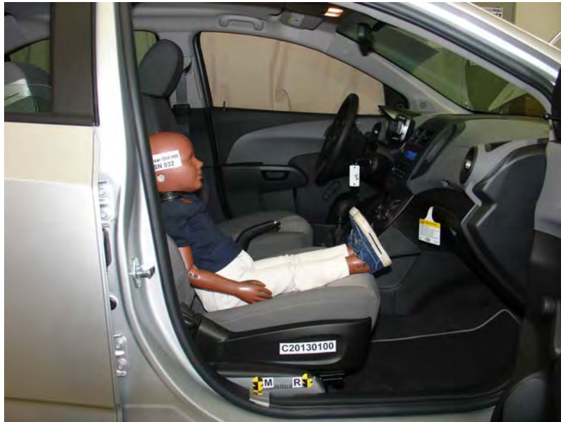
3-Year-Old Unbelted, Middle Seat Track, Position 2
