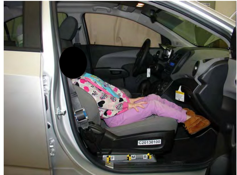
6-Year-Old Unbelted, Forward Seat Track, Position 2
