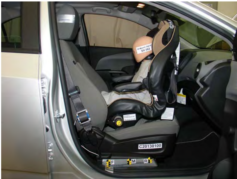
Evenflo Generations Rear Facing Unbelted, Forward Seat Track
