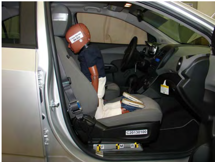
3-Year-Old Unbelted, Forward Seat Track, Position 7
