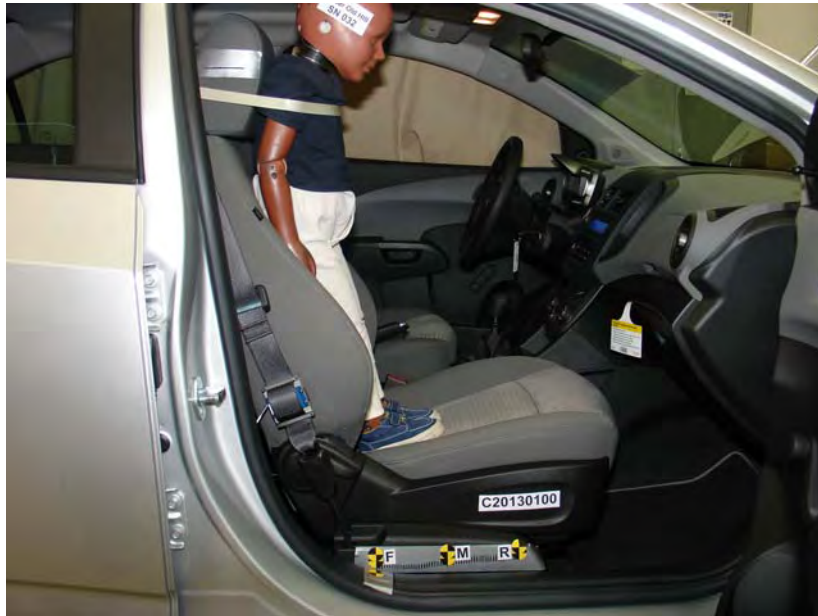
3-Year-Old Unbelted, Forward Seat Track, Position 5
