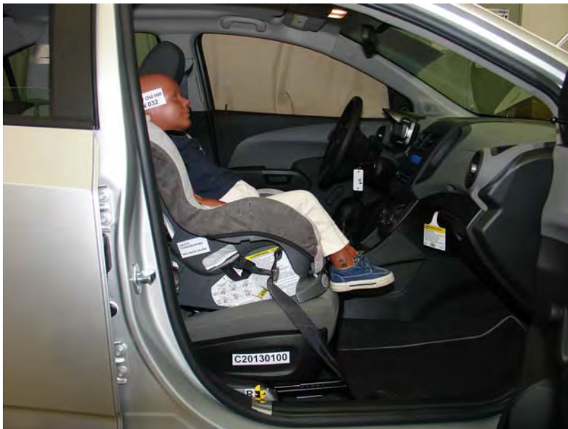
3-Year-Old Forward Facing Graco Comfortsport Belted, Rearward Seat Track
