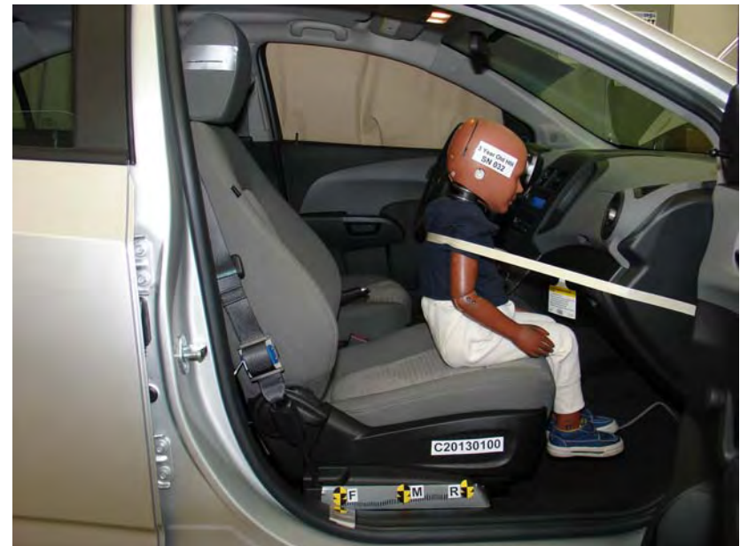
3-Year-Old Unbelted, Forward Seat Track, Position 4
