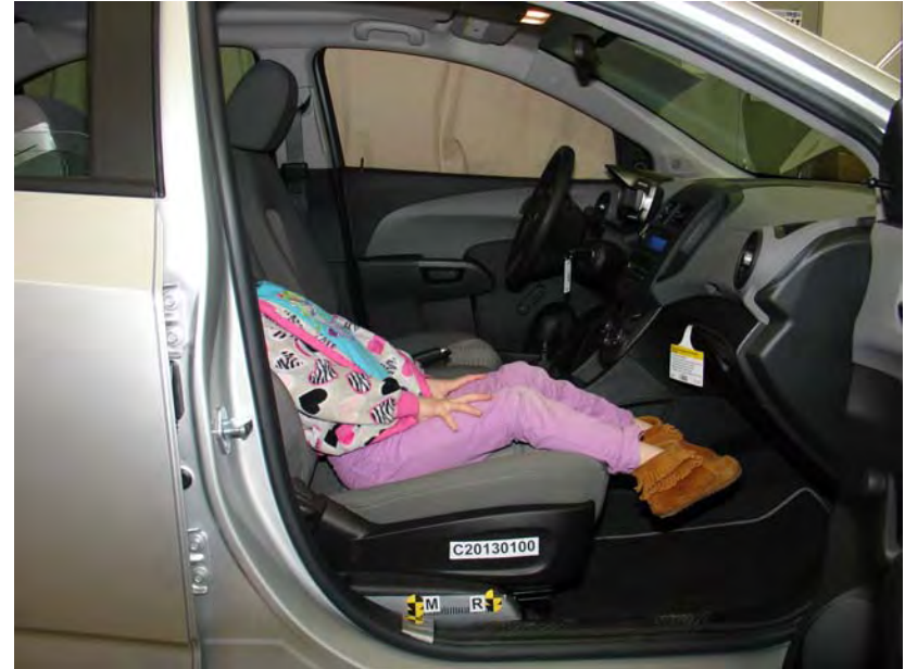
6-Year-Old Unbelted, Middle Seat Track, Position 2
