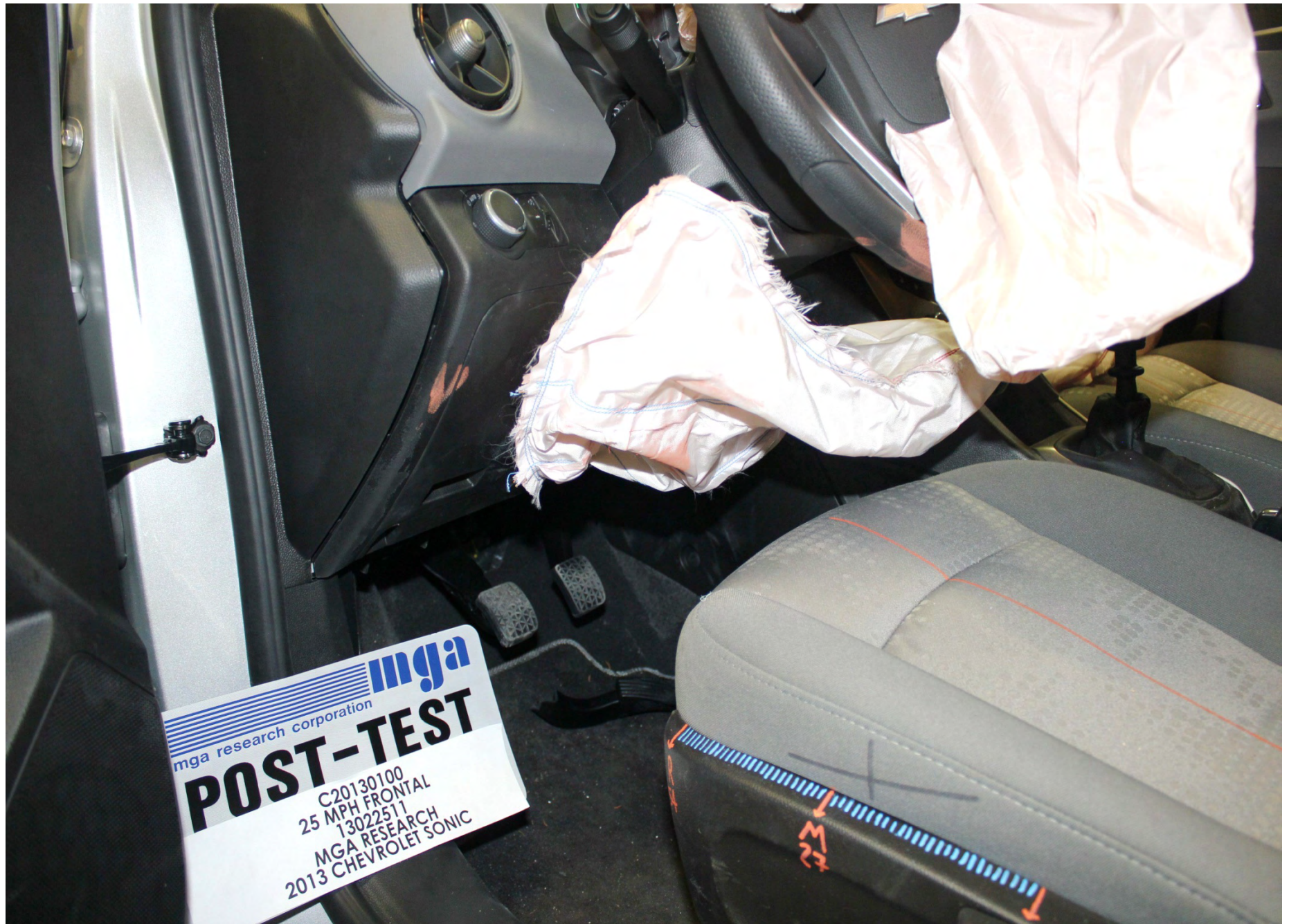
Post-Test Driver Dummy Knee Contact (knee bolster)
