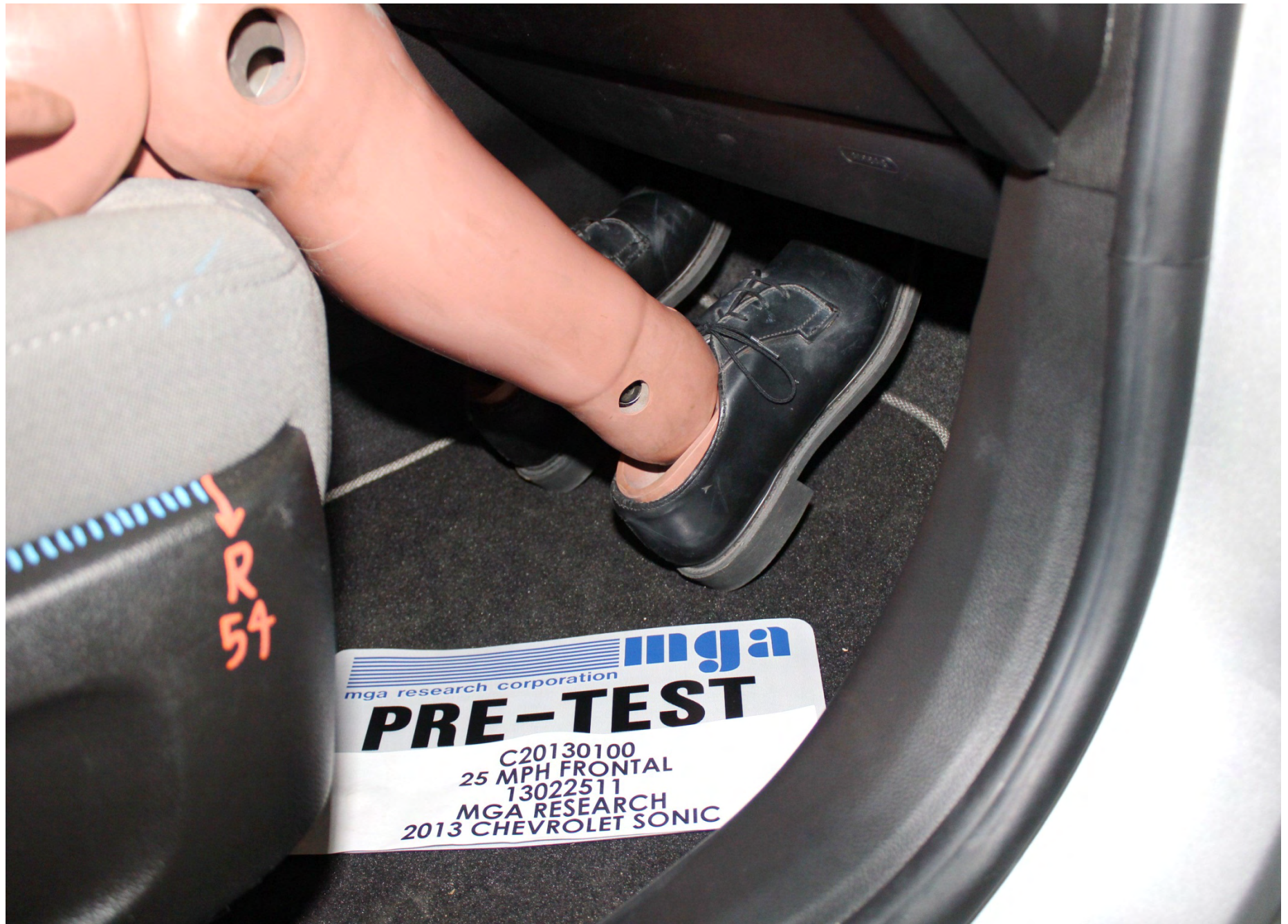
Pre-Test Passenger Dummy Feet Position
