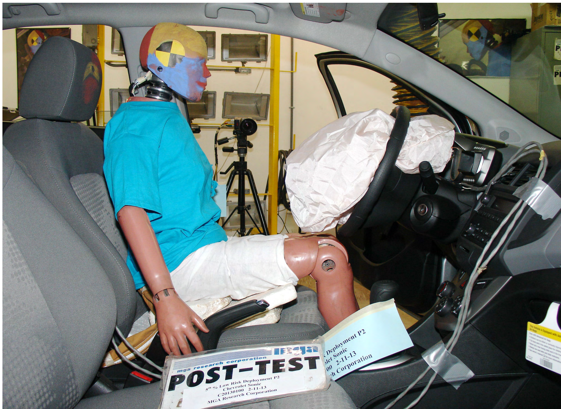
Post-Test 5th Fem. P2 Driver Dummy Right Side View
