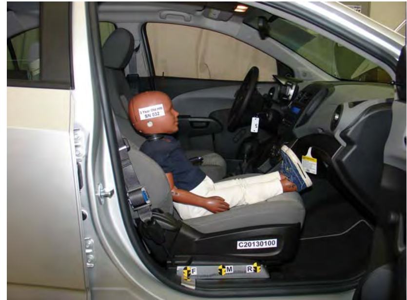
3-Year-Old Unbelted, Forward Seat Track, Position 2
