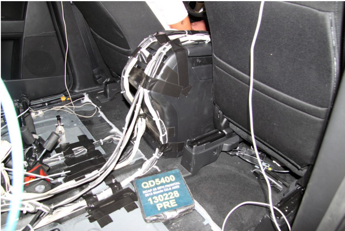
027 Pre-test Dummy Cable Routing
