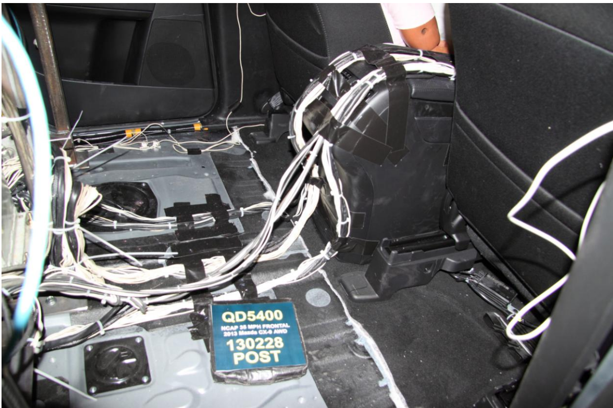
028 Post-test Dummy Cable Routing
