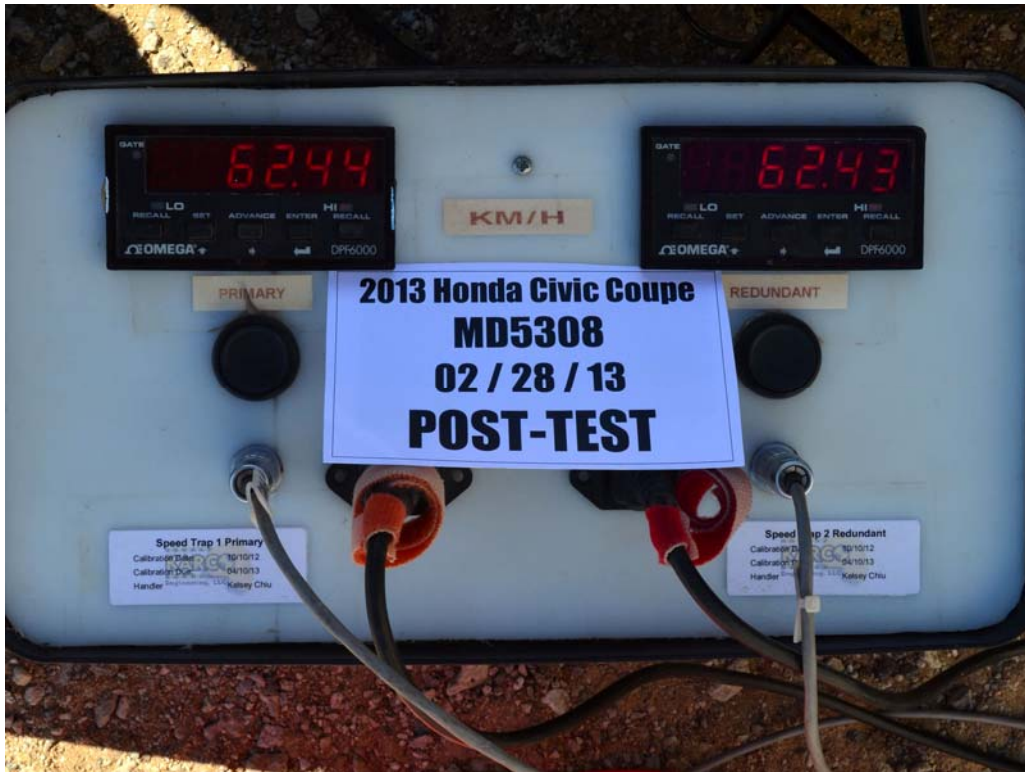
FIGURE 95. Post-Test Primary and Redundant Speed Trap Read-Out
