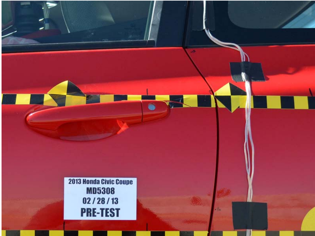
FIGURE 21. Pre-Test Left Front Door Latch Close-Up
