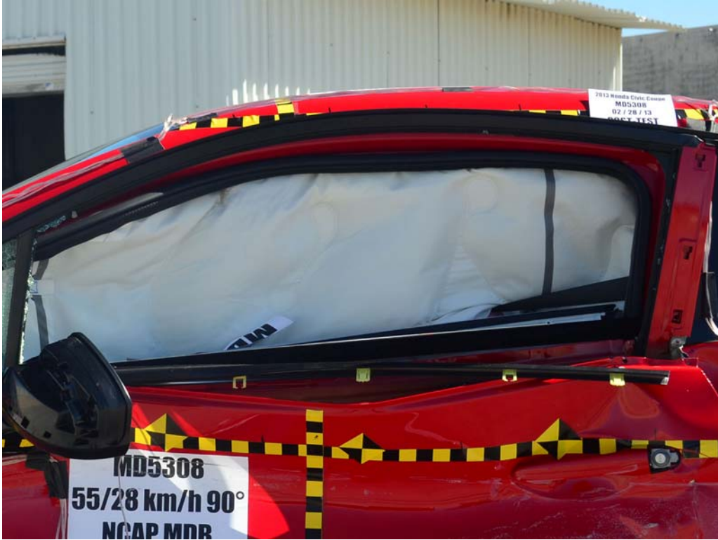
FIGURE 29. Post-Test Left Side View of Driver Dummy Shoulder and Door Top View
