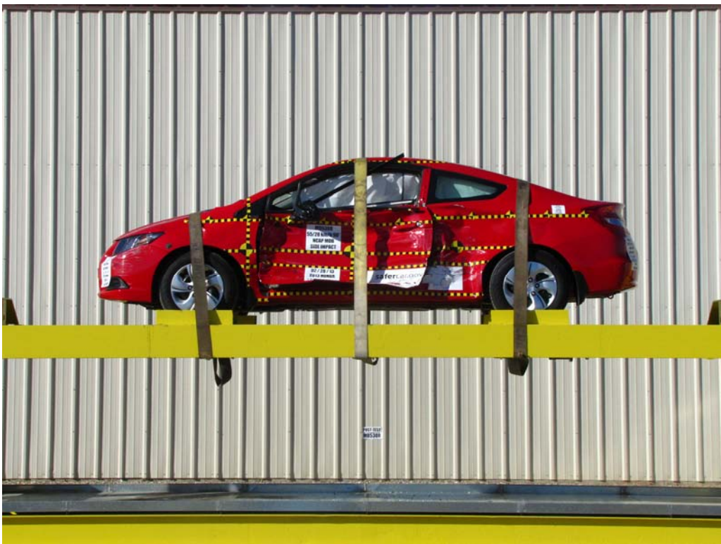
FIGURE 100. FMVSS No. 301 Static Rollover 360 Degrees
