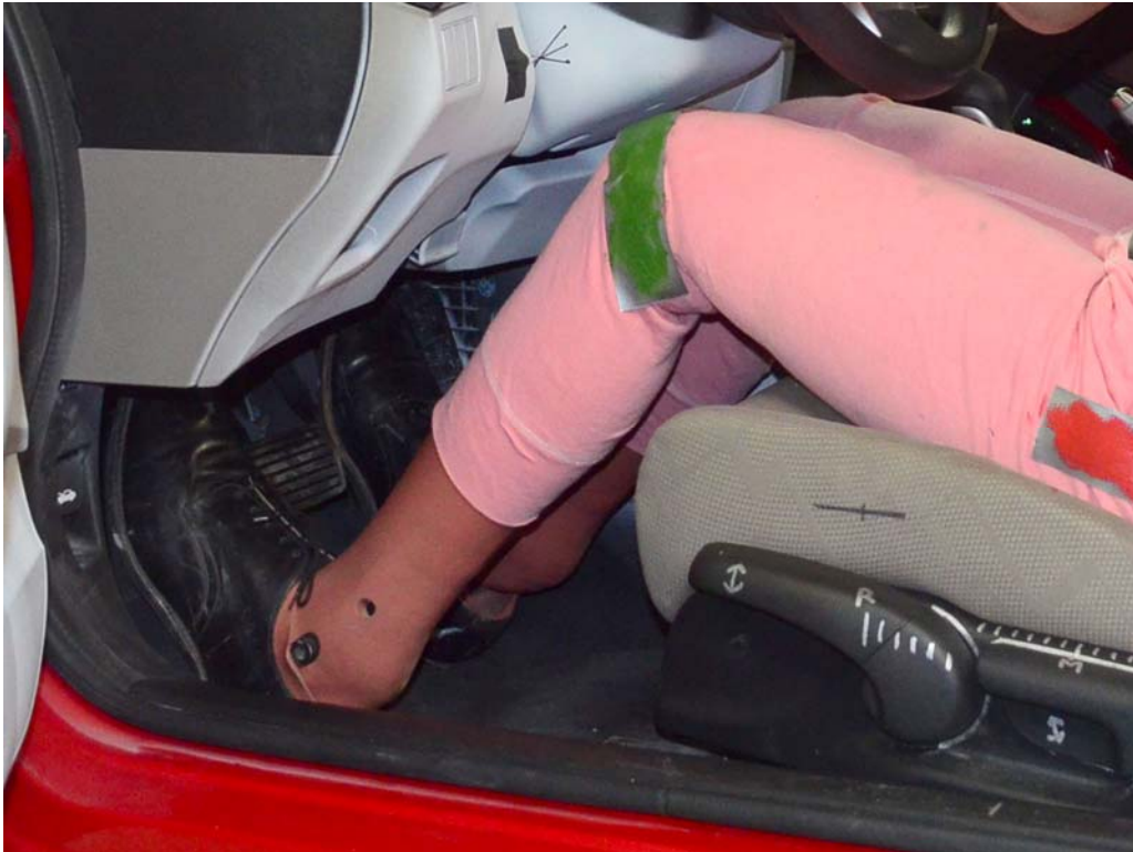
FIGURE 34. Pre-Test Placement of Driver Dummy's Feet
