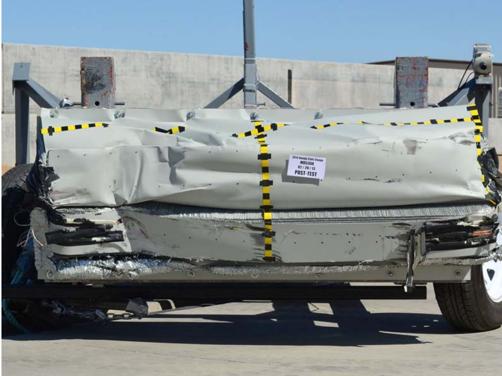
FIGURE 85. Post-Test Front View of MDB Impactor Face
