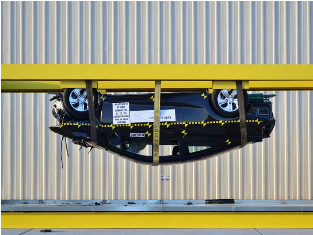
FIGURE 72. Vehicle at 180° on Static Rollover Device
