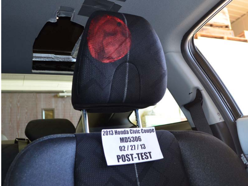
FIGURE 47. Post-Test Driver Dummy Contact with Headrest
