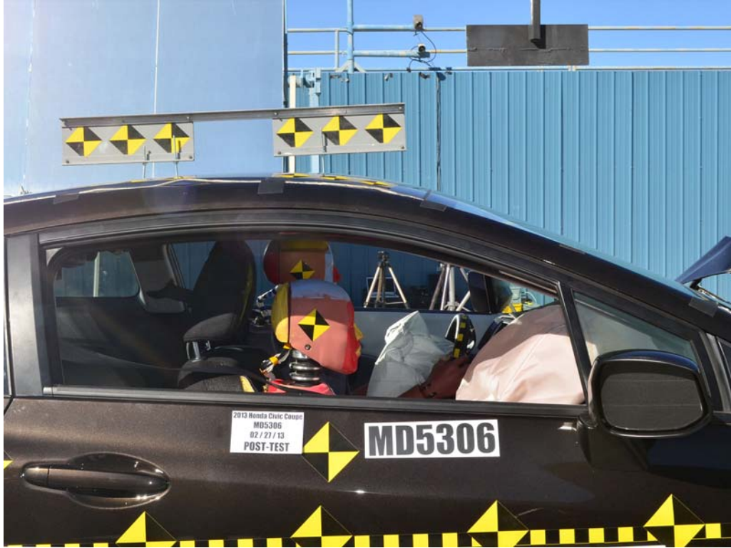
FIGURE 53. Post-Test Passenger Dummy Window View
