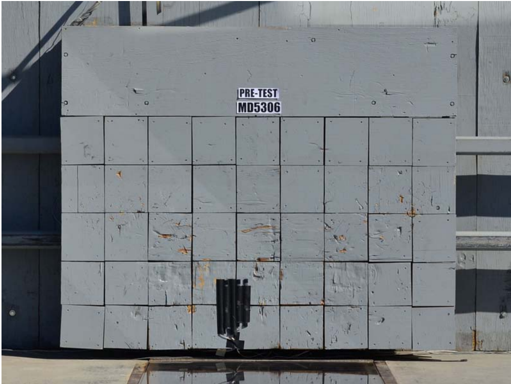
FIGURE 2. Load Cell Wall
