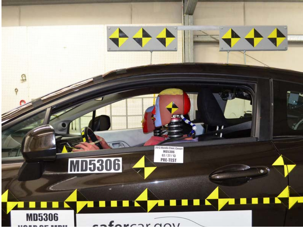
FIGURE 31. Pre-Test Driver Dummy Window View
