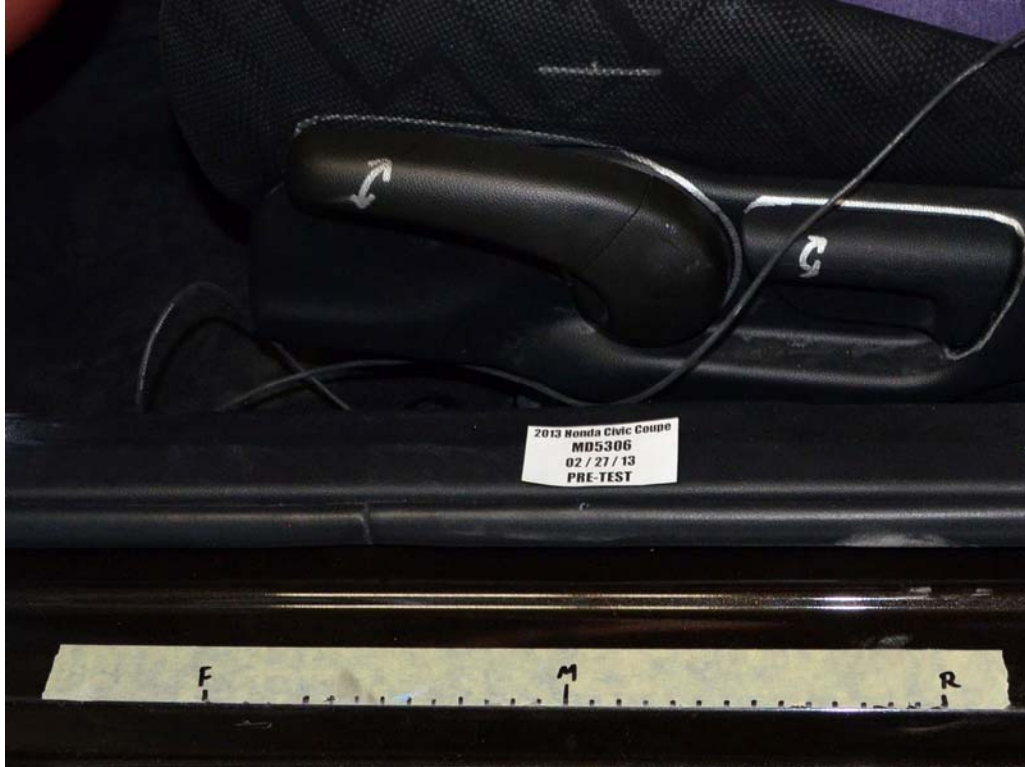
FIGURE 35. Pre-Test Driver's Seat Fore-Aft Markings
