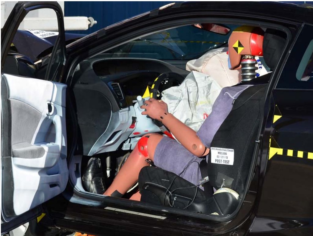
FIGURE 34. Post-Test Driver Dummy and Vehicle Interior View
