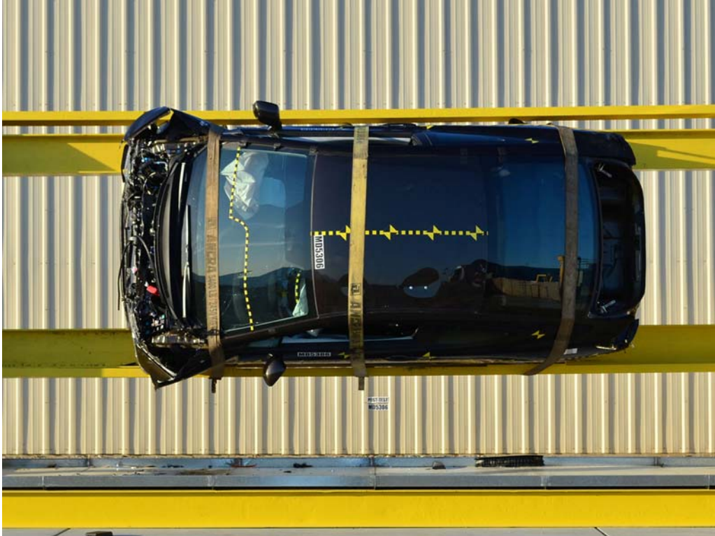
FIGURE 71. Vehicle at 90° on Static Rollover Device
