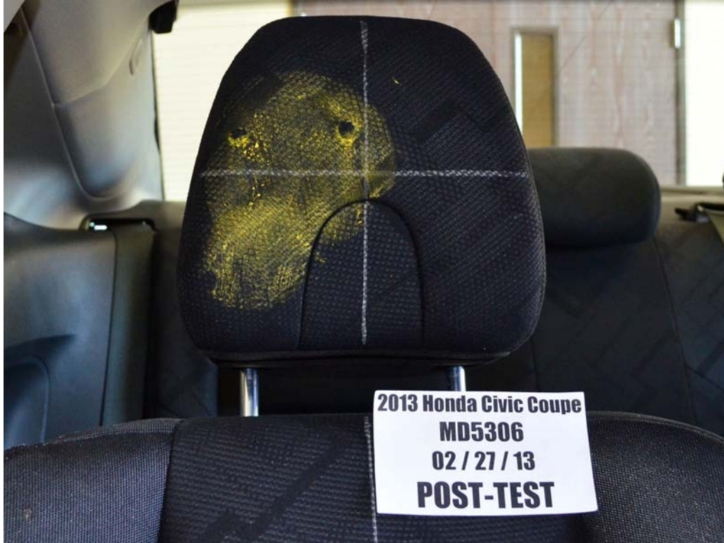
FIGURE 66a. Post-Test Passenger Dummy Contact with Headrest
