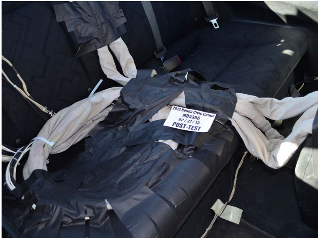
FIGURE 28. Post-Test Dummy Cable Routing
