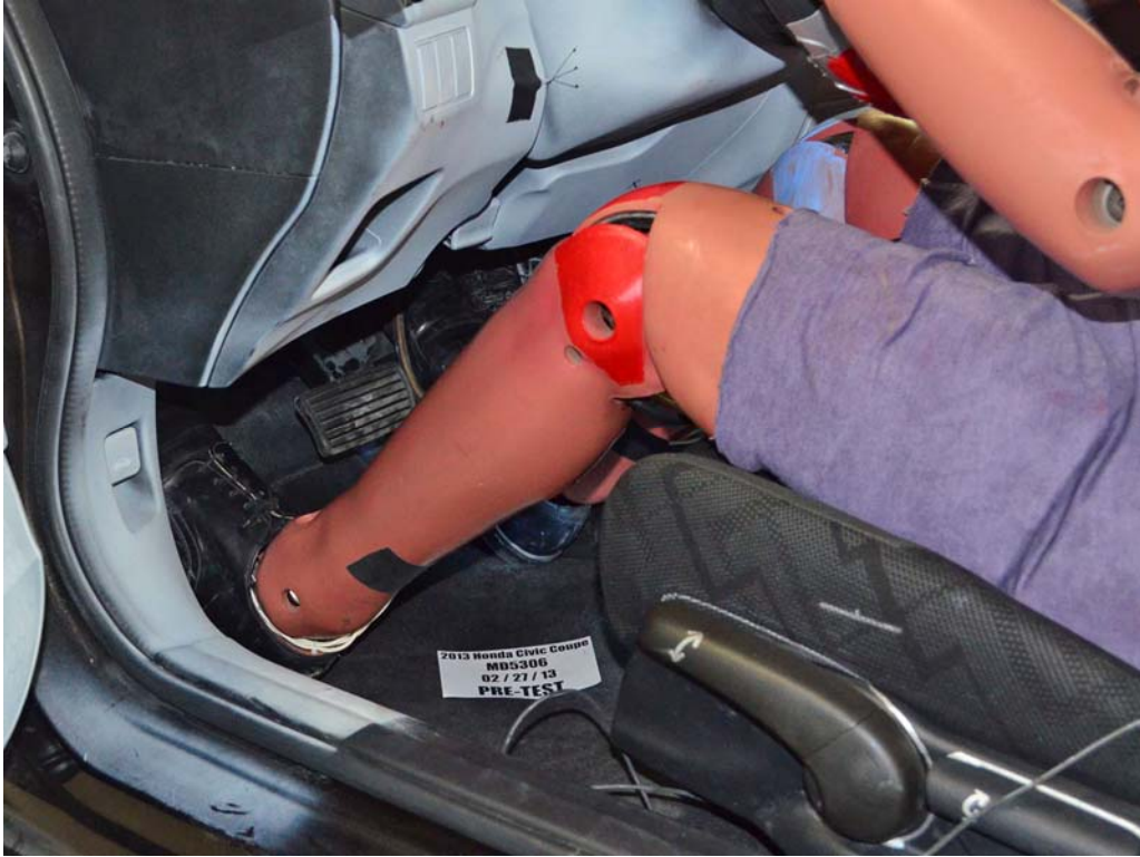
FIGURE 39. Pre-Test Driver Dummy Feet
