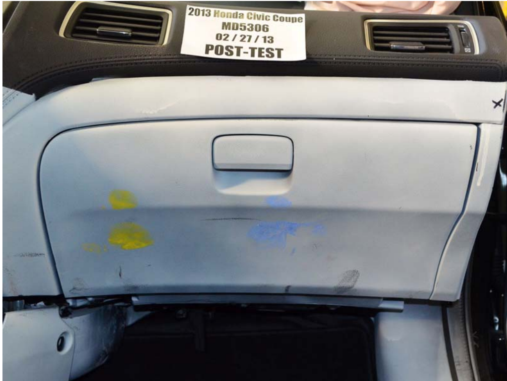
FIGURE 63. Post-Test Passenger's Side Knee Bolster
