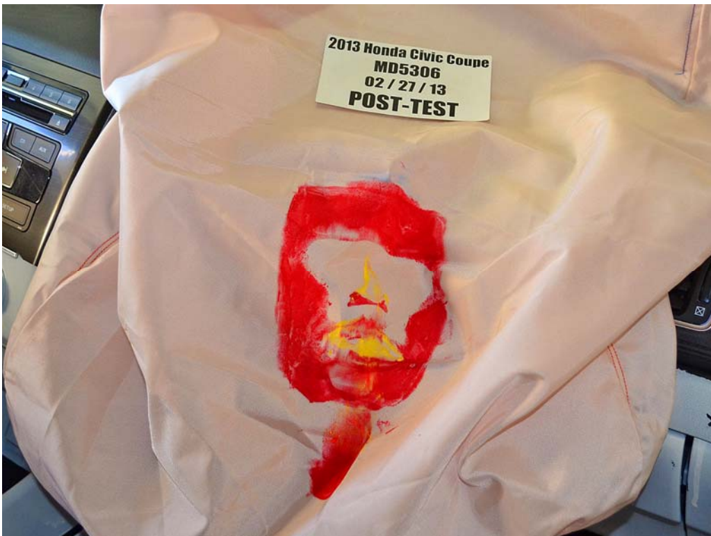
FIGURE 66. Post-Test Passenger Dummy Contact with Airbag
