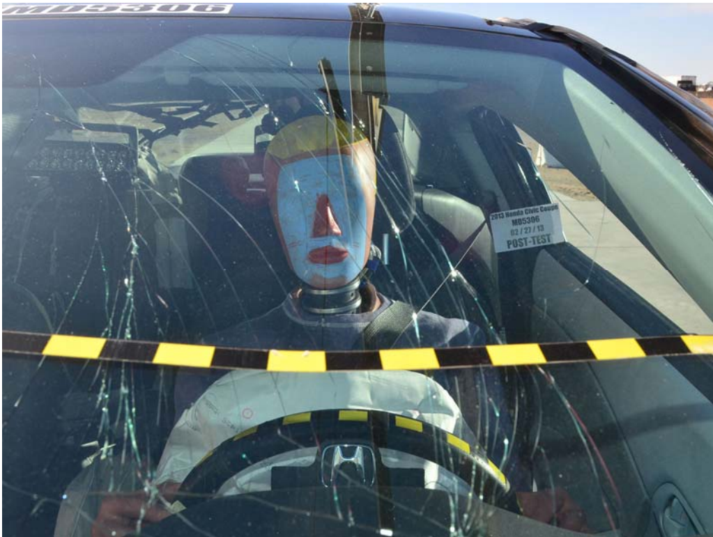
FIGURE 30. Post-Test Driver Dummy Front View
