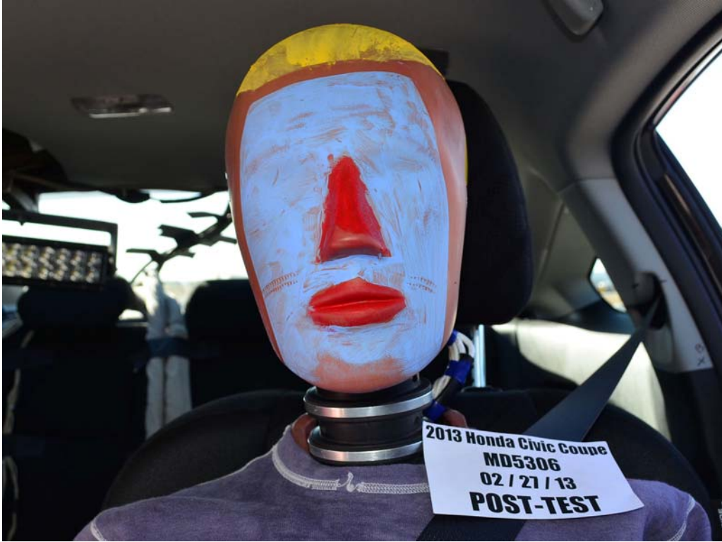
FIGURE 45. Post-Test Driver Dummy Face
