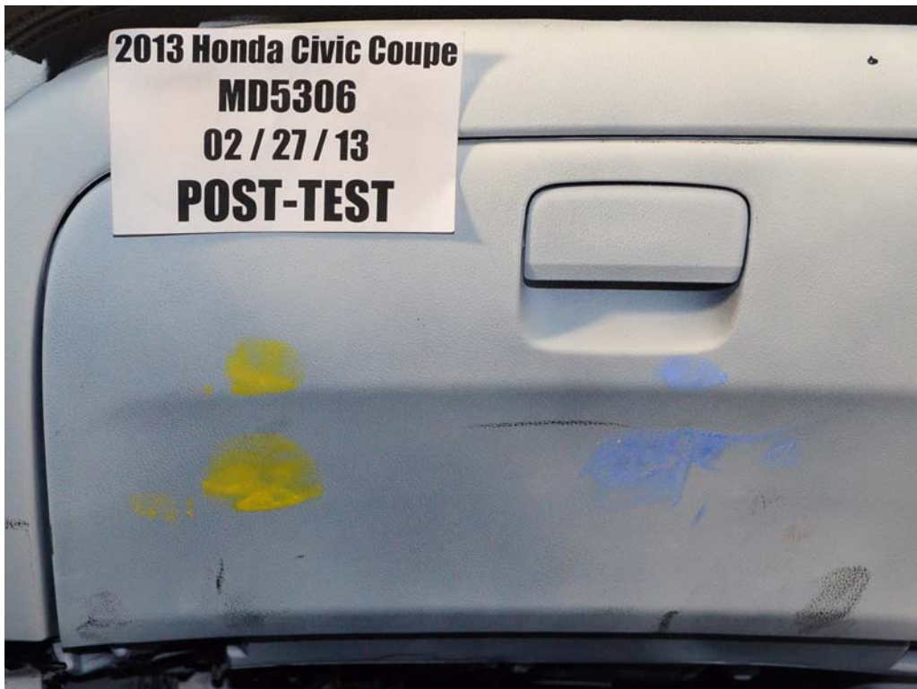
FIGURE 66b. Post-Test Passenger Dummy Contact with Glovebox
