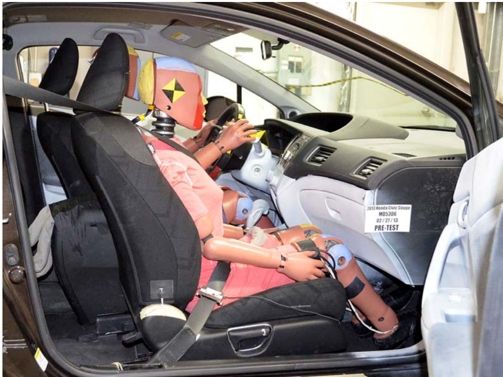
FIGURE 54. Pre-Test Passenger Dummy and Vehicle Interior View
