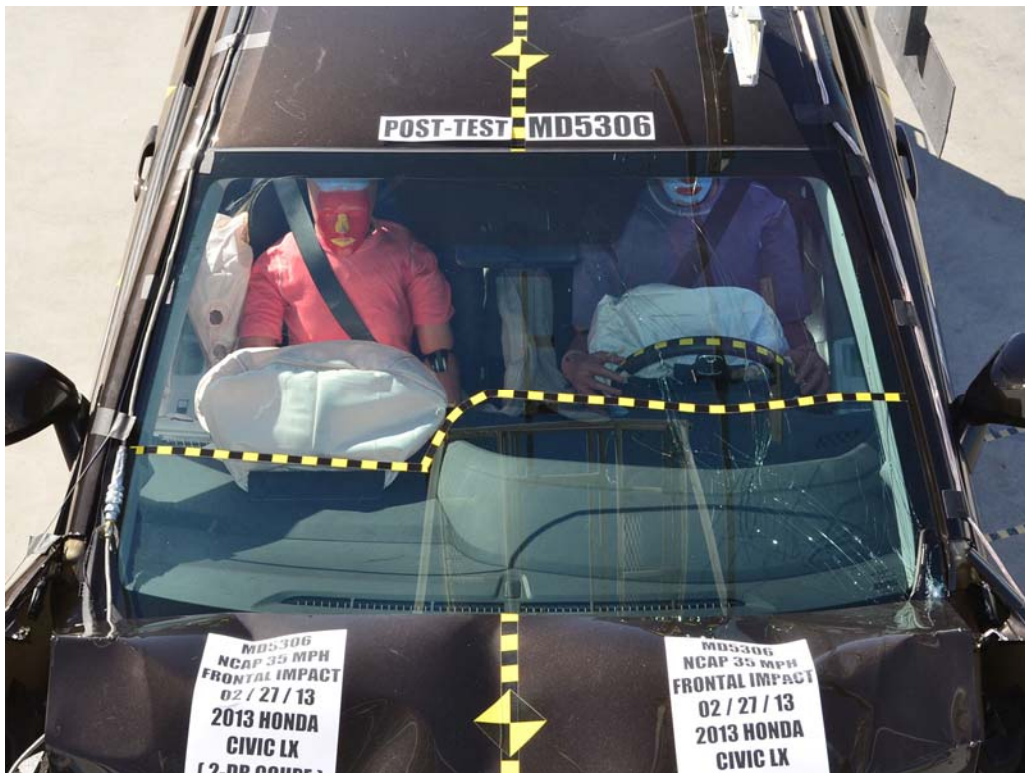
FIGURE 18. Post-Test Windshield View
