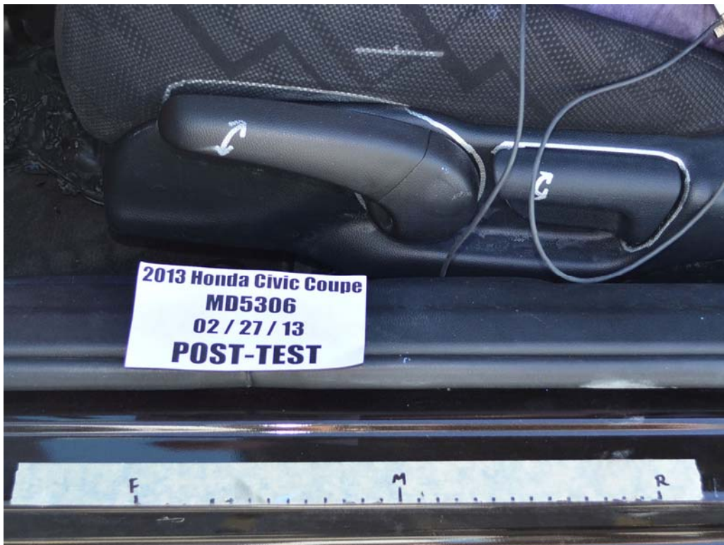
FIGURE 36. Post-Test Driver's Seat Fore-Aft Markings
