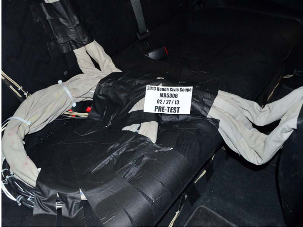
FIGURE 27. Pre-Test Dummy Cable Routing
