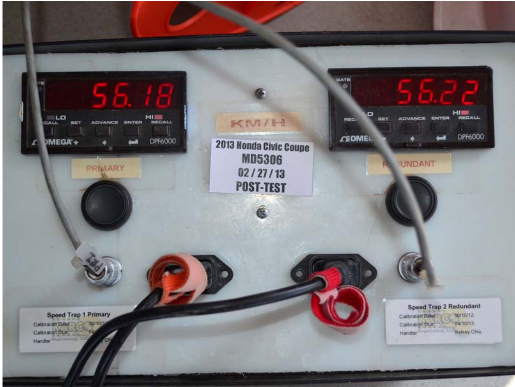
FIGURE 69. Post-Test Speed Trap Read-Out
