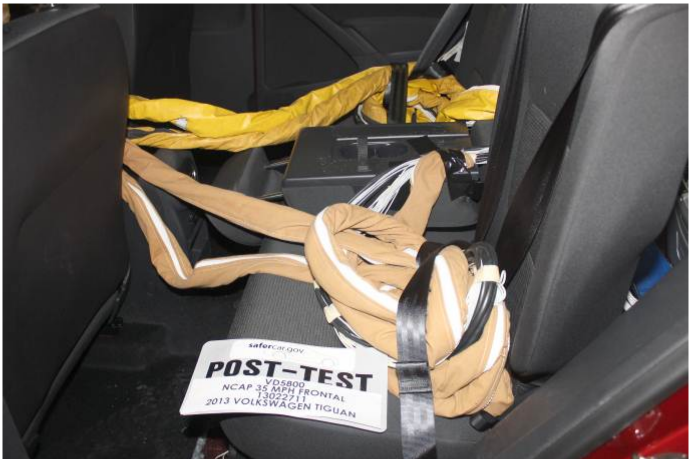
Post-Test Dummy Cable Routing
