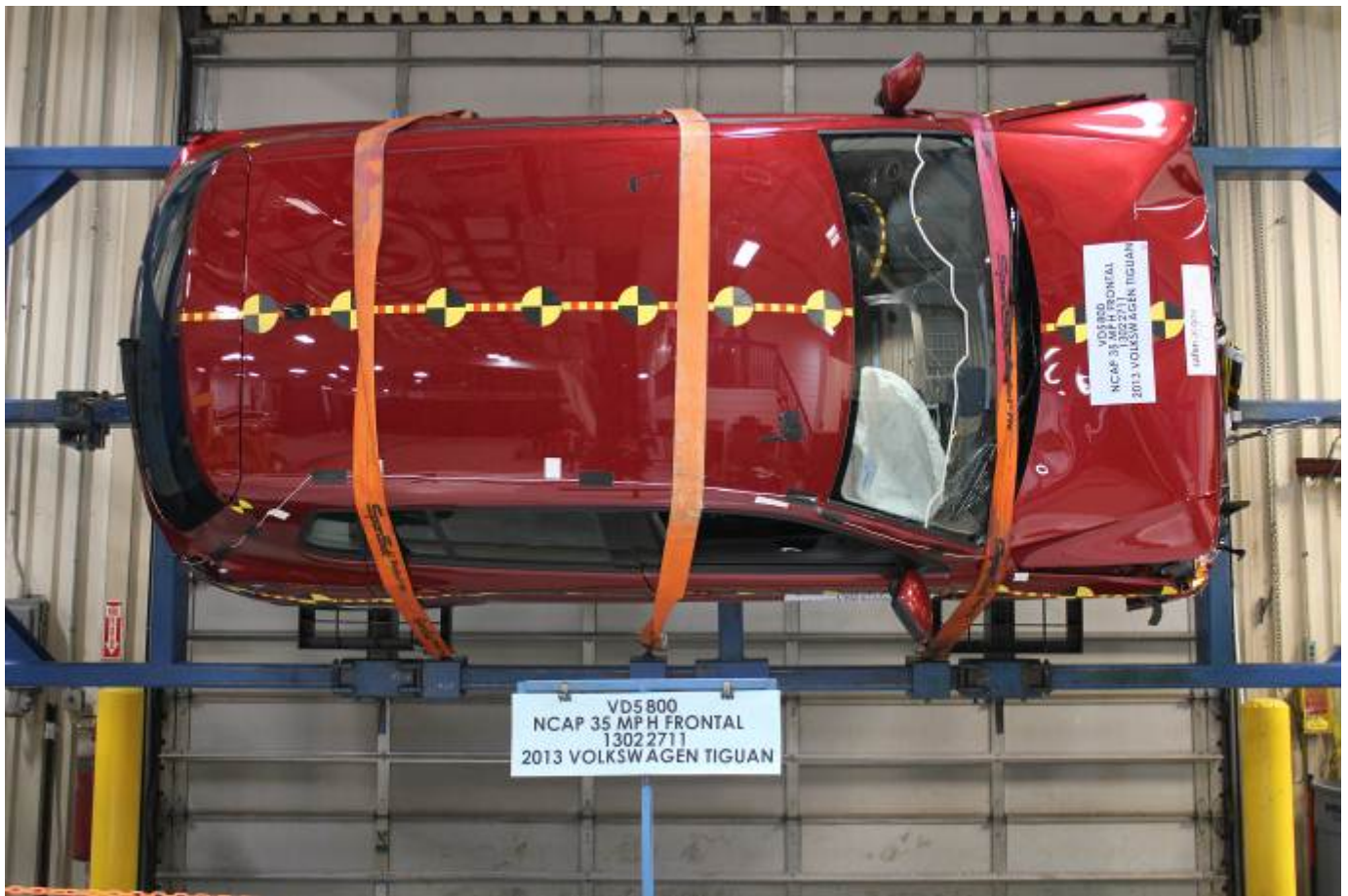
Vehicle at 90° on Static Rollover Device
