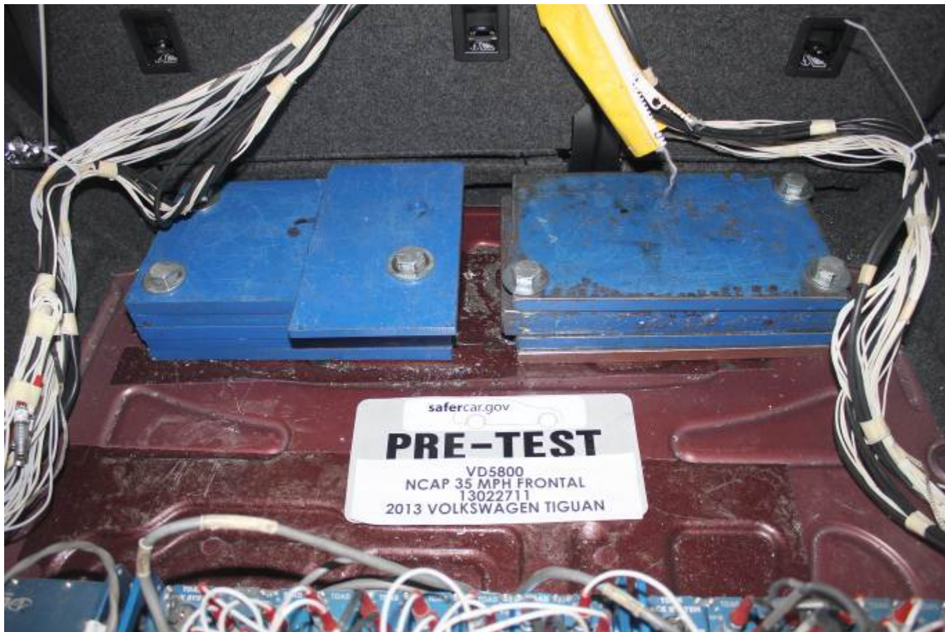
Ballast Installed in Vehicle
