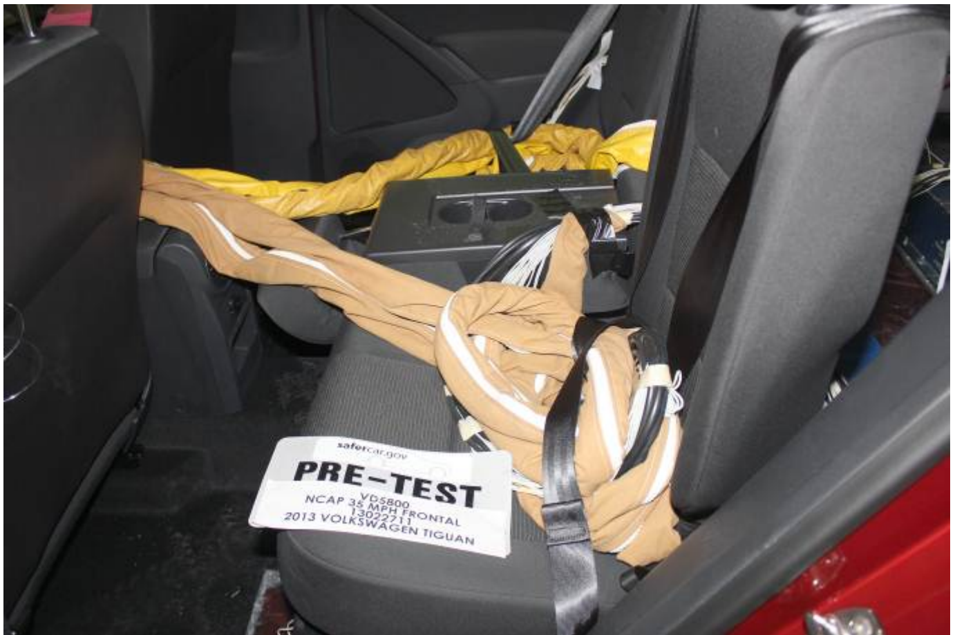
Pre-Test Dummy Cable Routing
