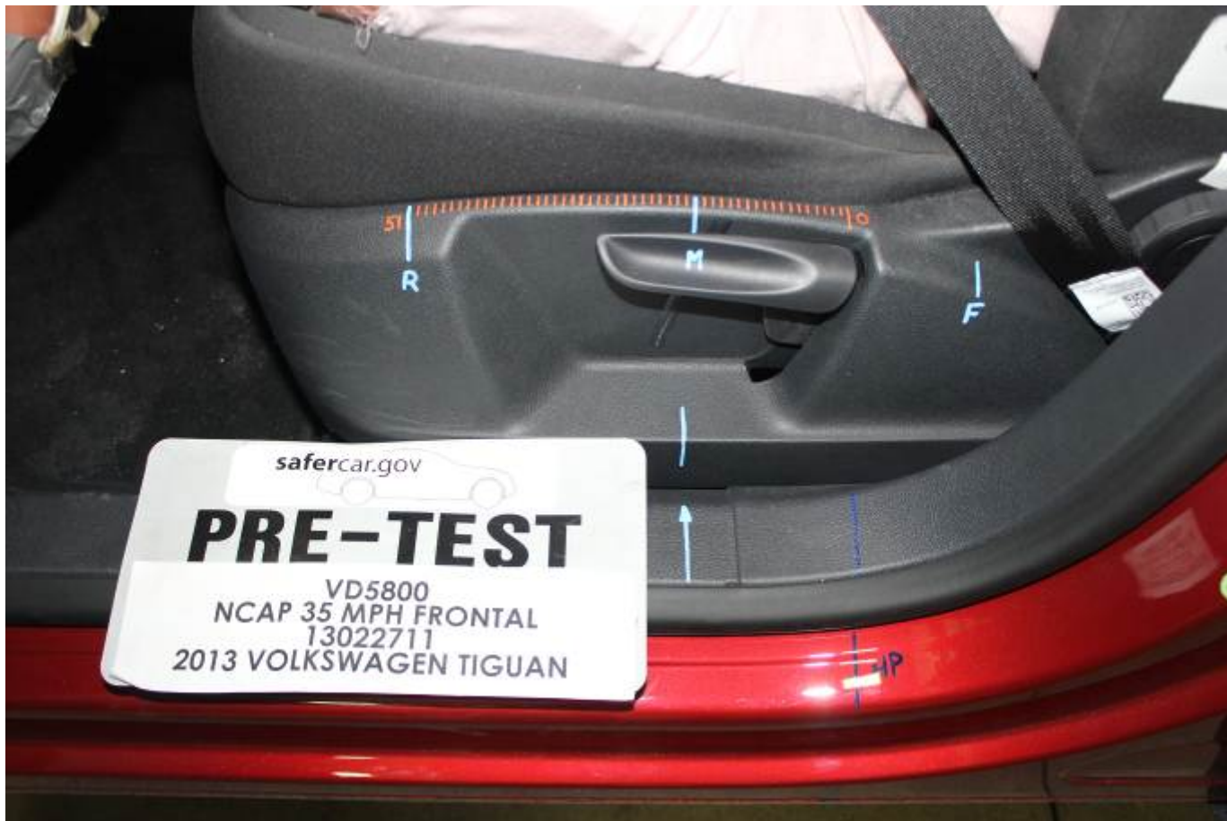
Pre-Test Driver's Seat Fore-Aft Markings
