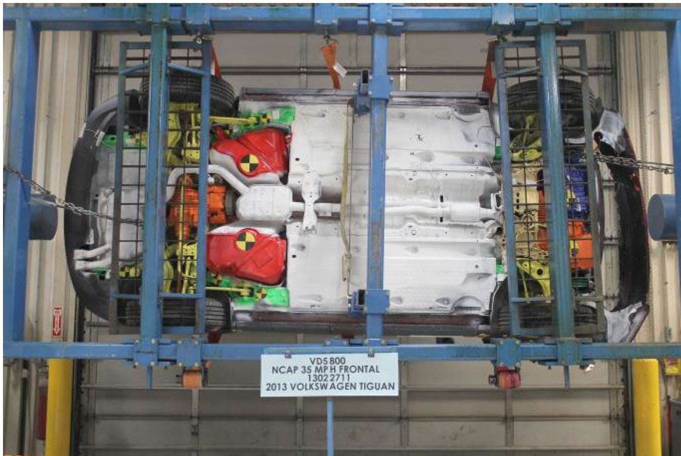
Vehicle at 270° on Static Rollover Device
