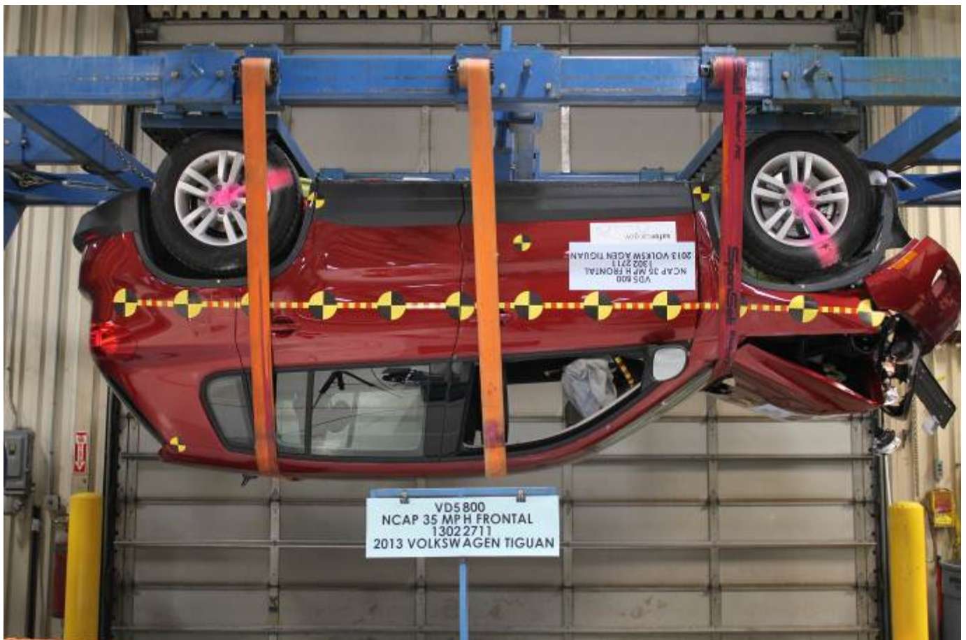
Vehicle at 180° on Static Rollover Device
