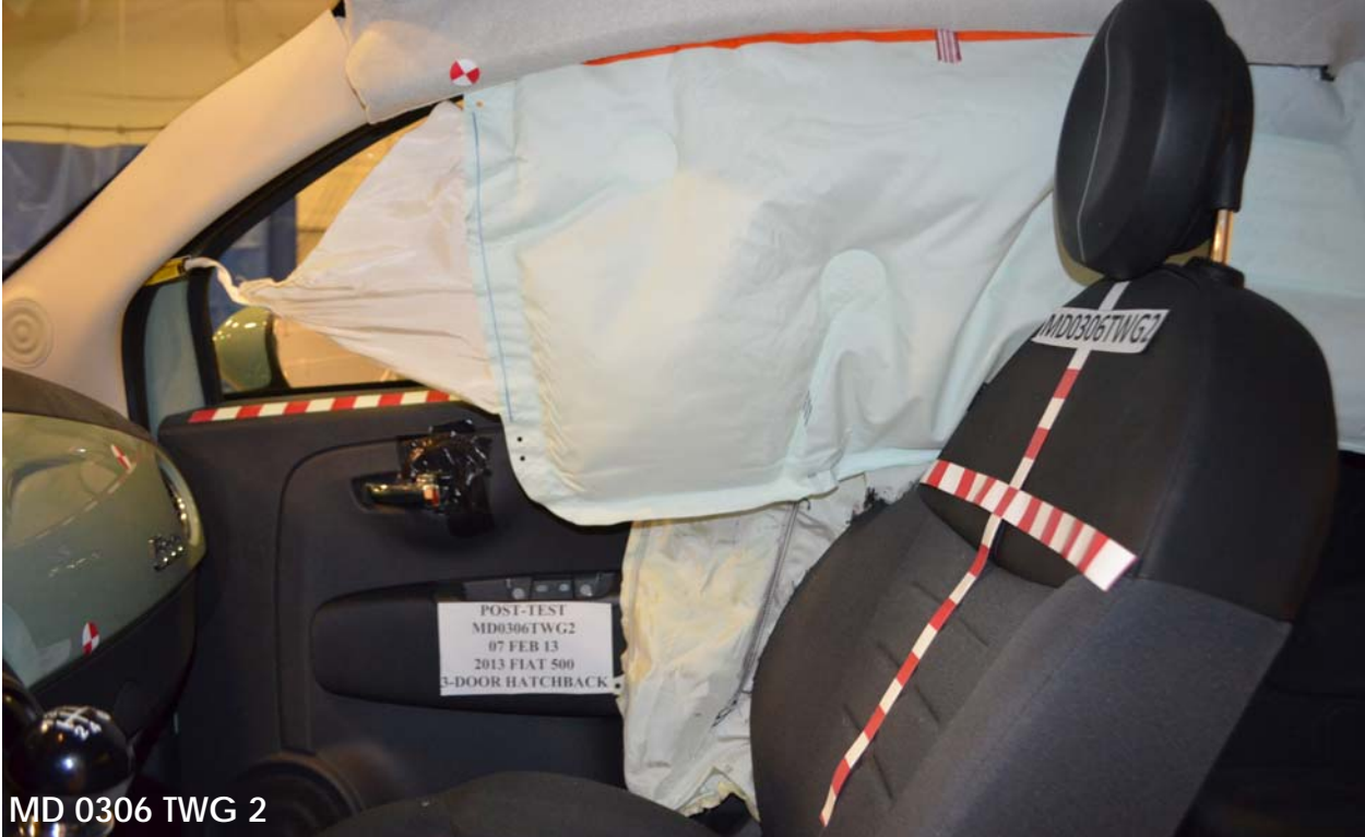
Figure A-11: Post-Test Left Side View of Side Airbag
