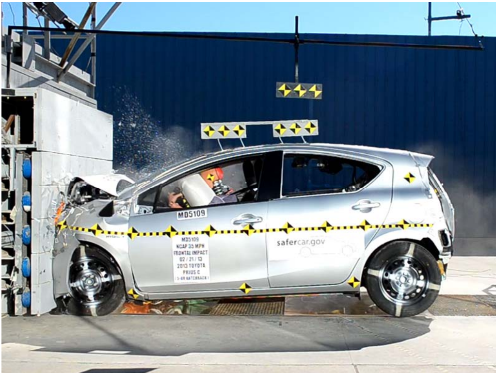
FIGURE 75. 2013 Toyota Prius C Frontal Impact Event
