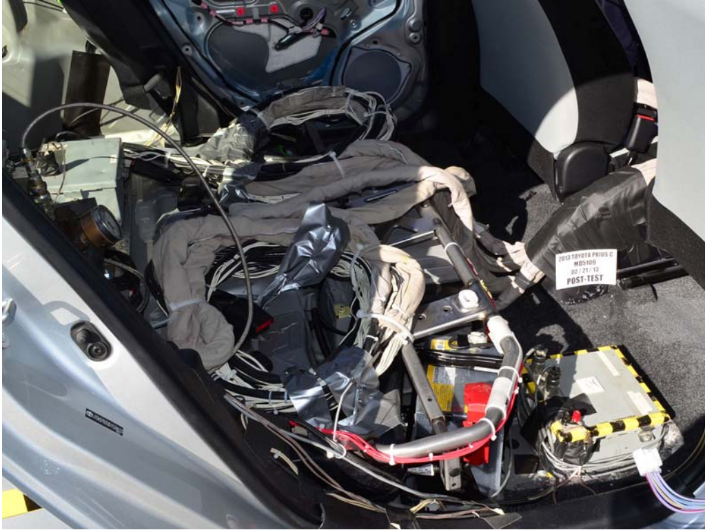
FIGURE 28. Post-Test Dummy Cable Routing
