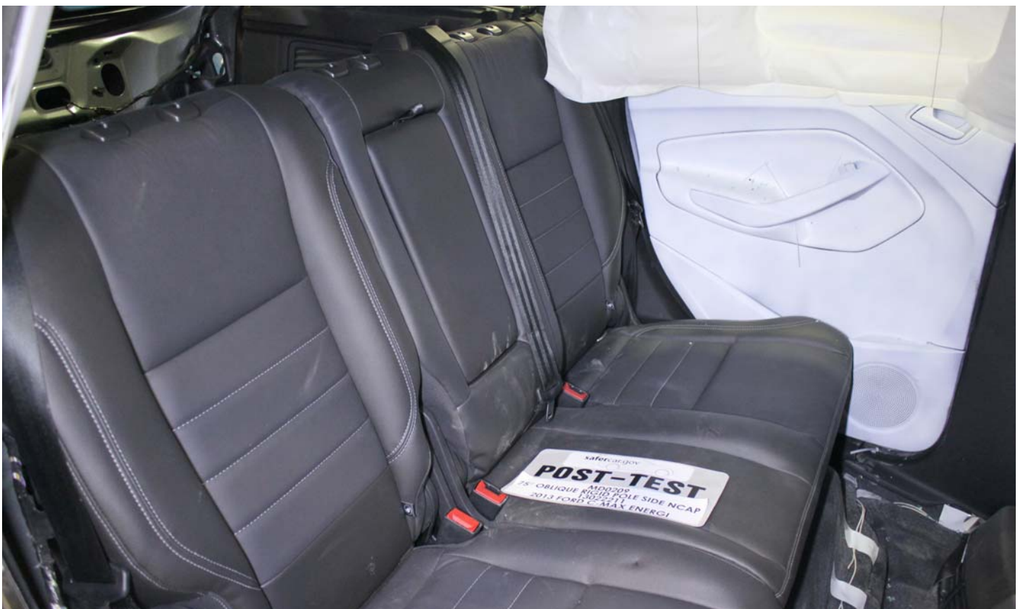
No. 033 Post-Impact View of the Vehicle Passenger Compartment Adjacent to Propulsion Battery
