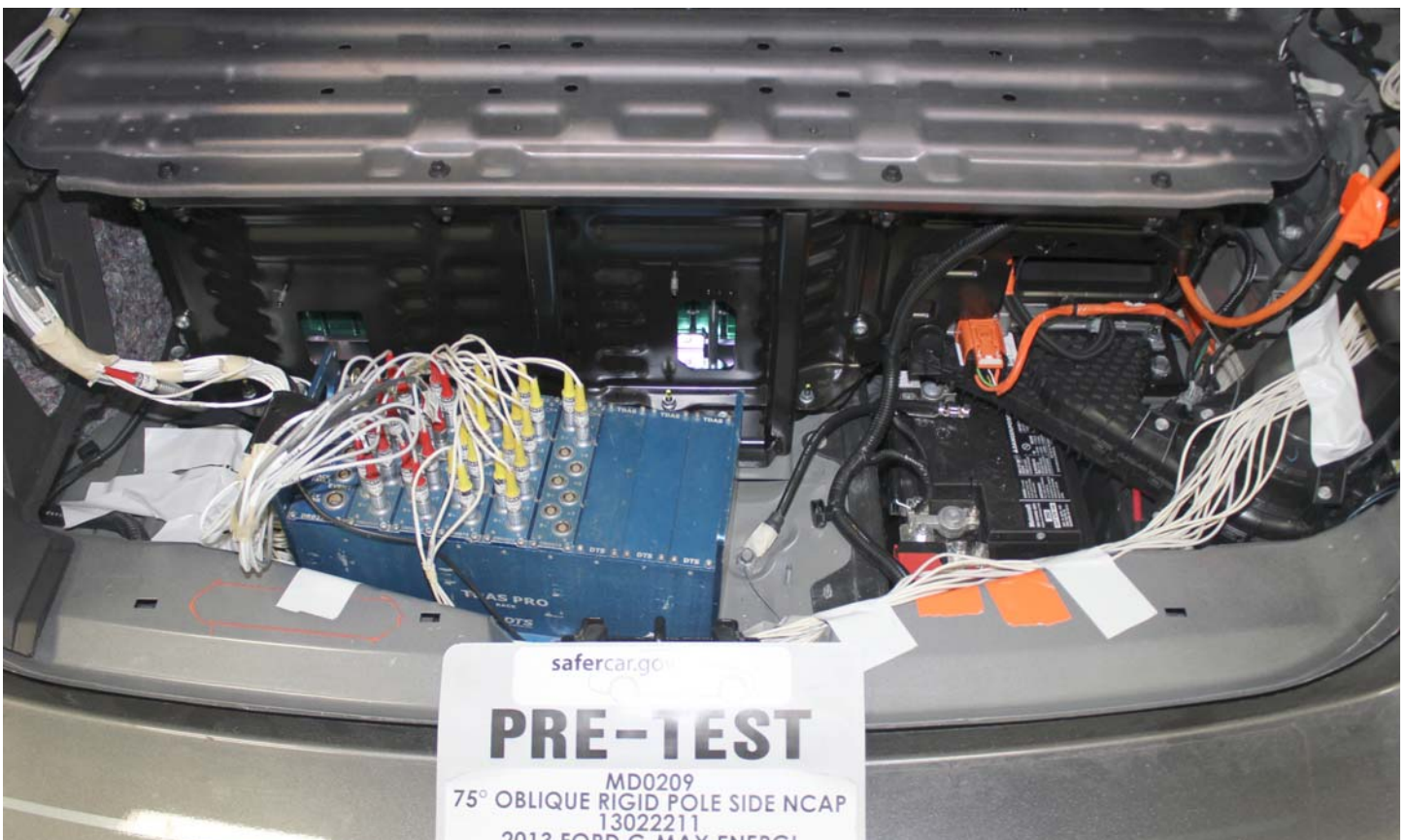
No. 019 Pre-Impact View Propulsion Battery Venting System(s)
