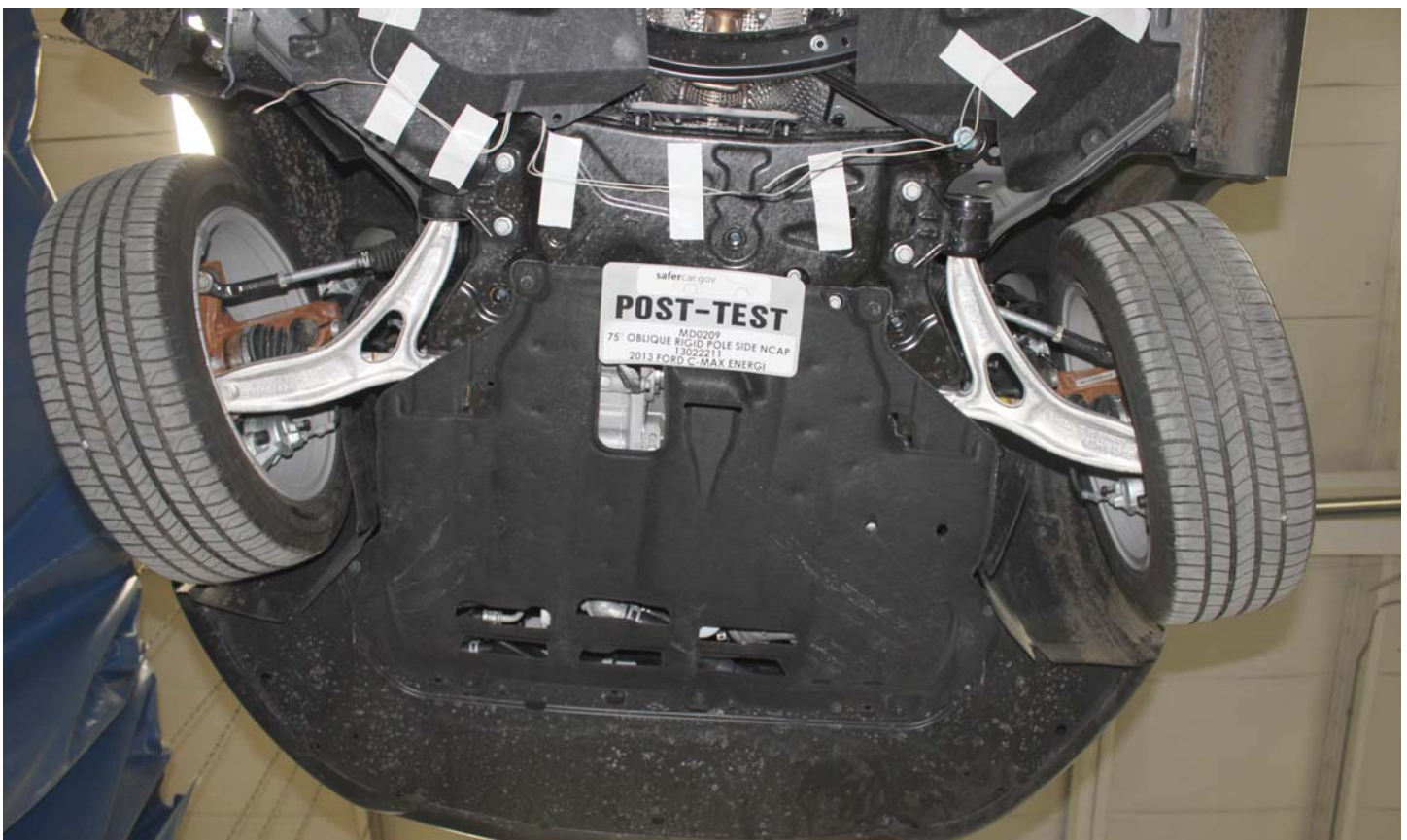
No. 017a Post-Impact View of Electric Propulsion Drive
