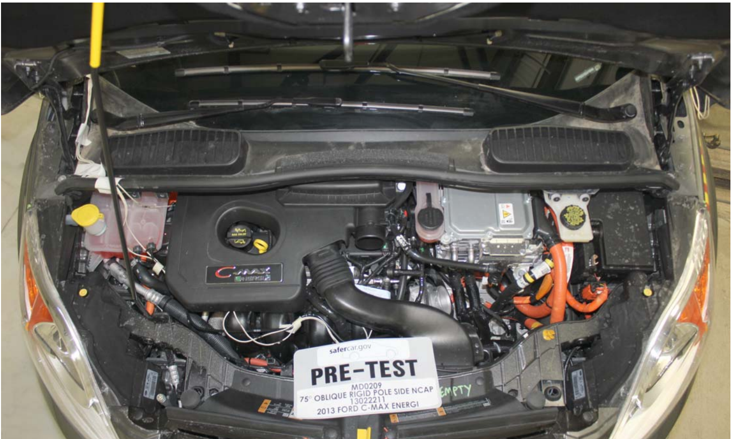
No. 016 Pre-Impact View of Electric Propulsion Drive
