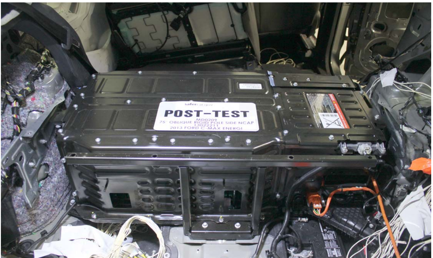
No. 011 Post-Impact Rear View of Propulsion Battery
