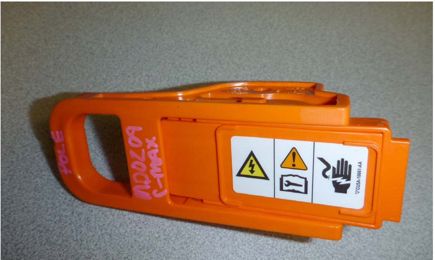
No. 008 Manual High Voltage Service Disconnect Removed
