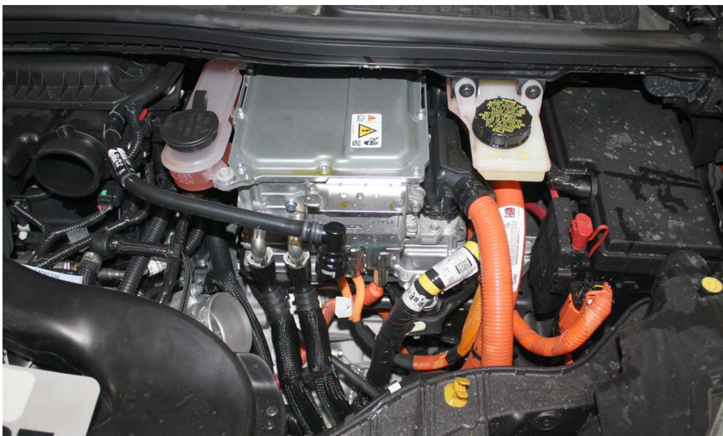
No. 002 Power Inverter Warning Label
