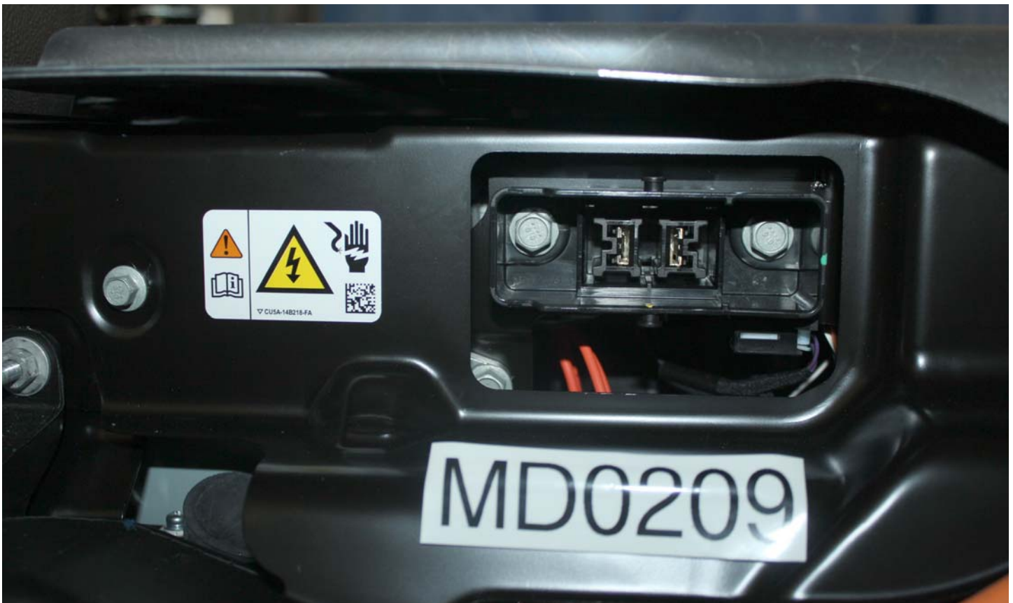
No. 007 Manual High Voltage Service Disconnect Removed
