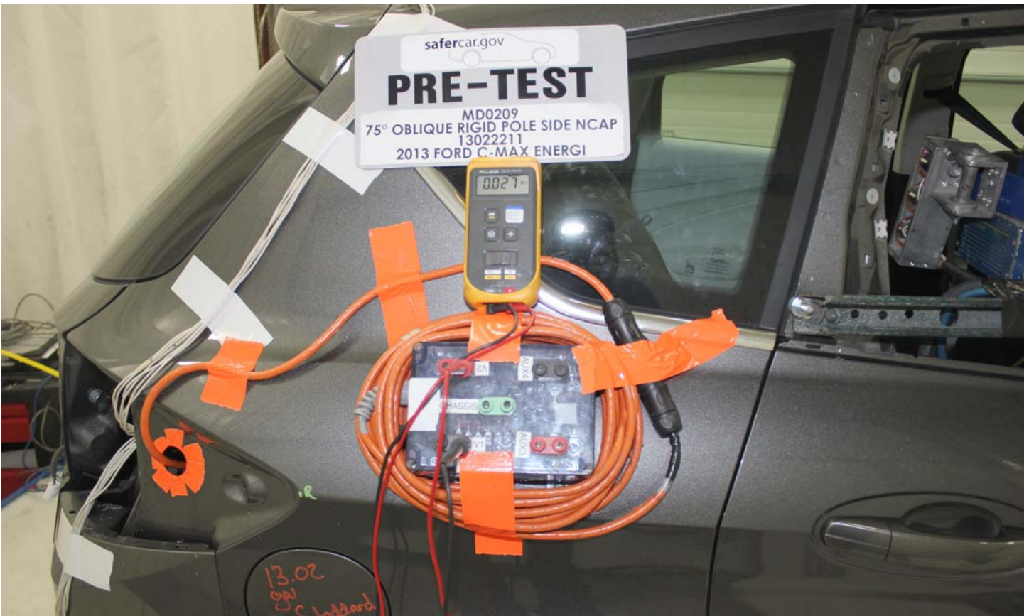
No. 024 Pre-Impact View of Installed Impact Interface Port
