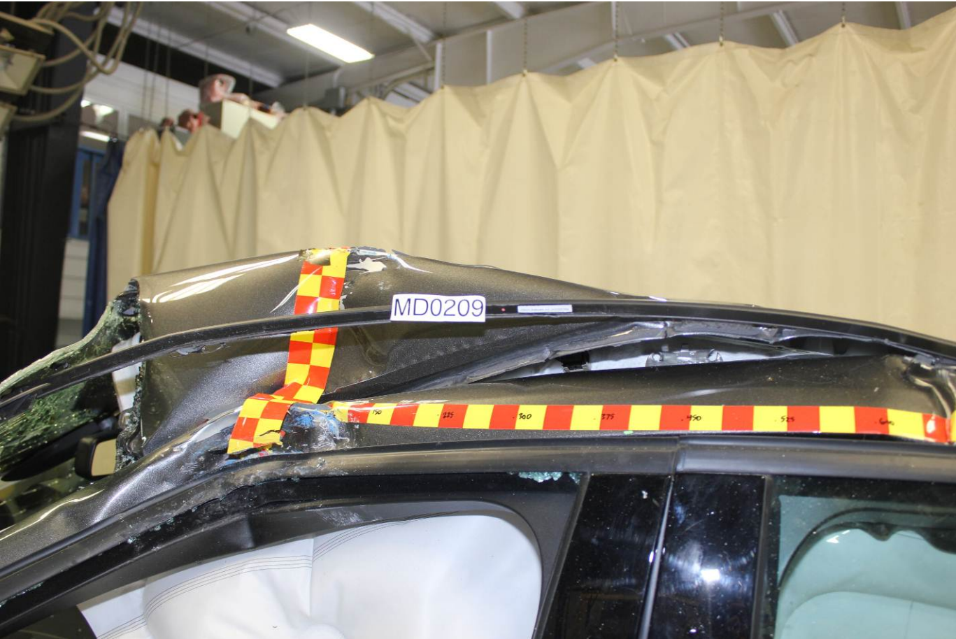
Post-Test Roof and Windshield Separations
