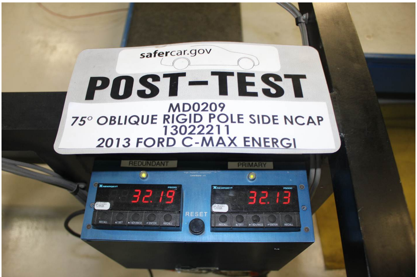
Post-Test Primary and Redundant Speed Trap Read-Out
