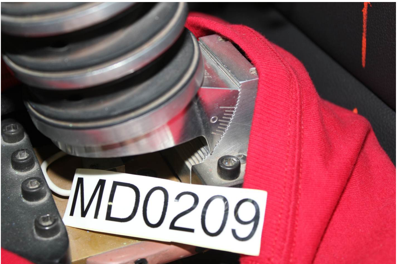
Pre-Test Left Side View of Dummy's Neck Showing Position of Adjustable Neck Bracket
