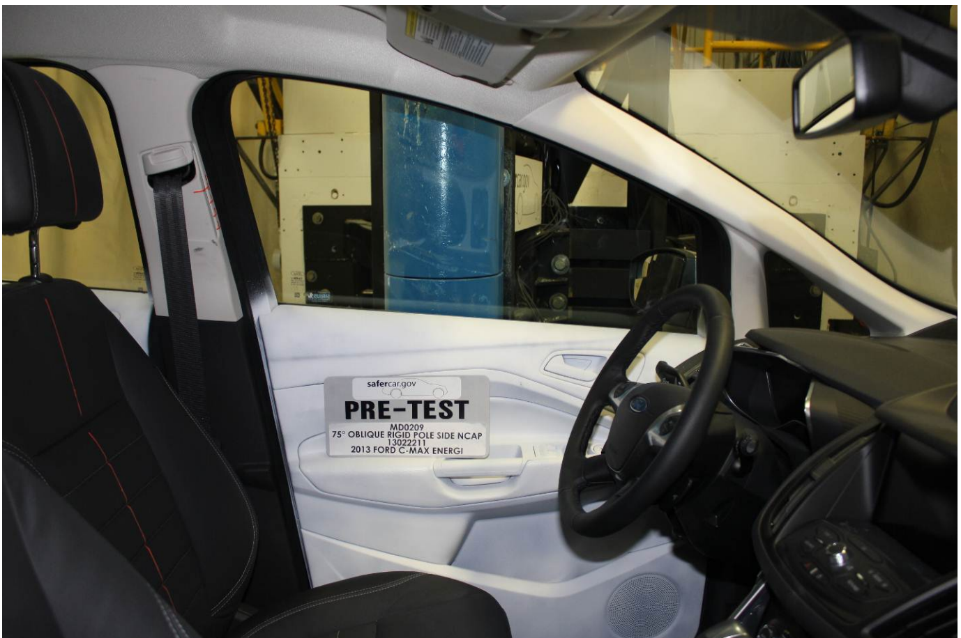
Pre-Test Inner Door Panel View
