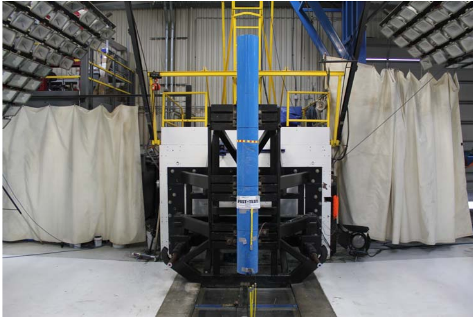
254 mm Diameter Rigid Pole
