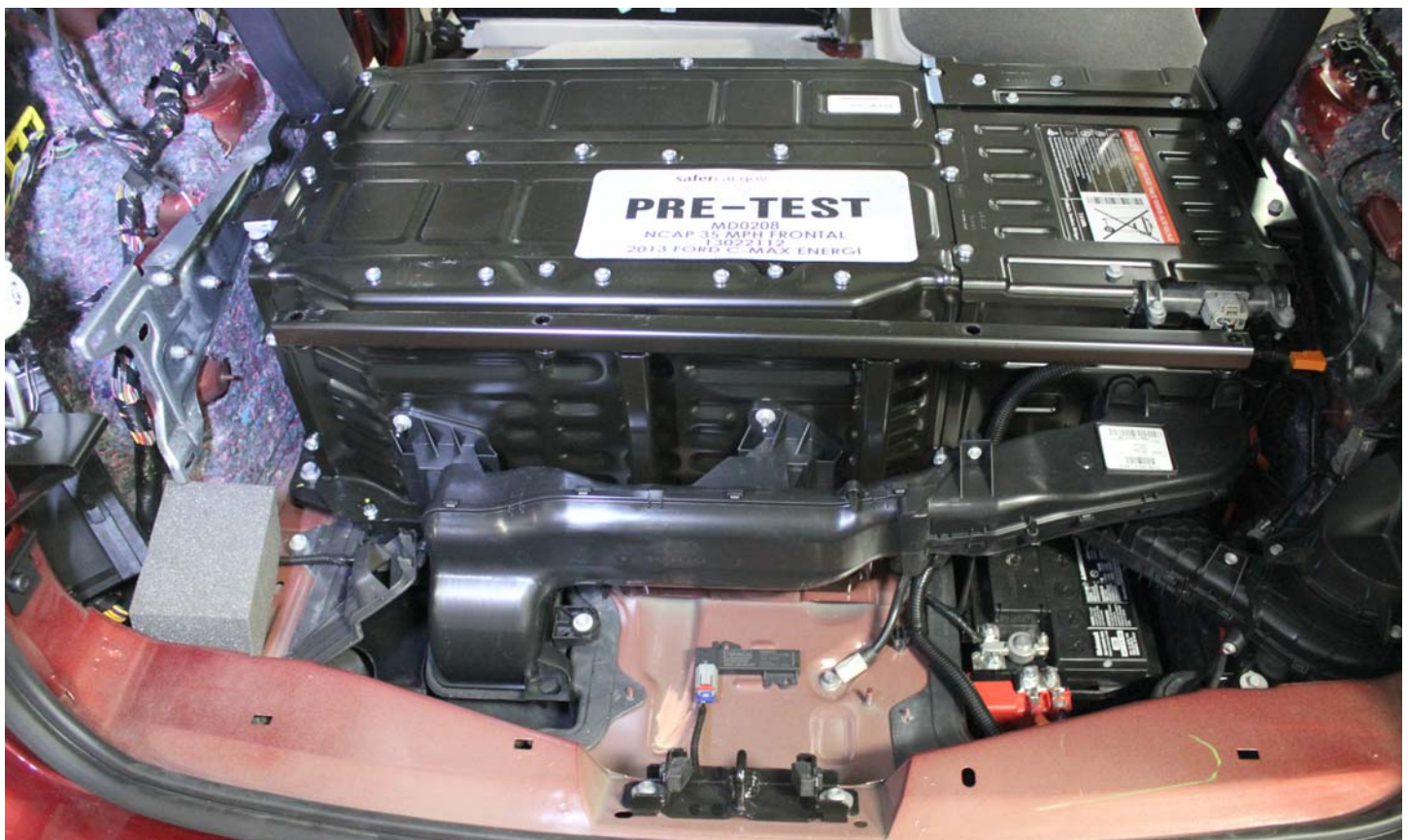
No. 019 Pre-Impact View Propulsion Battery Venting System(s)
