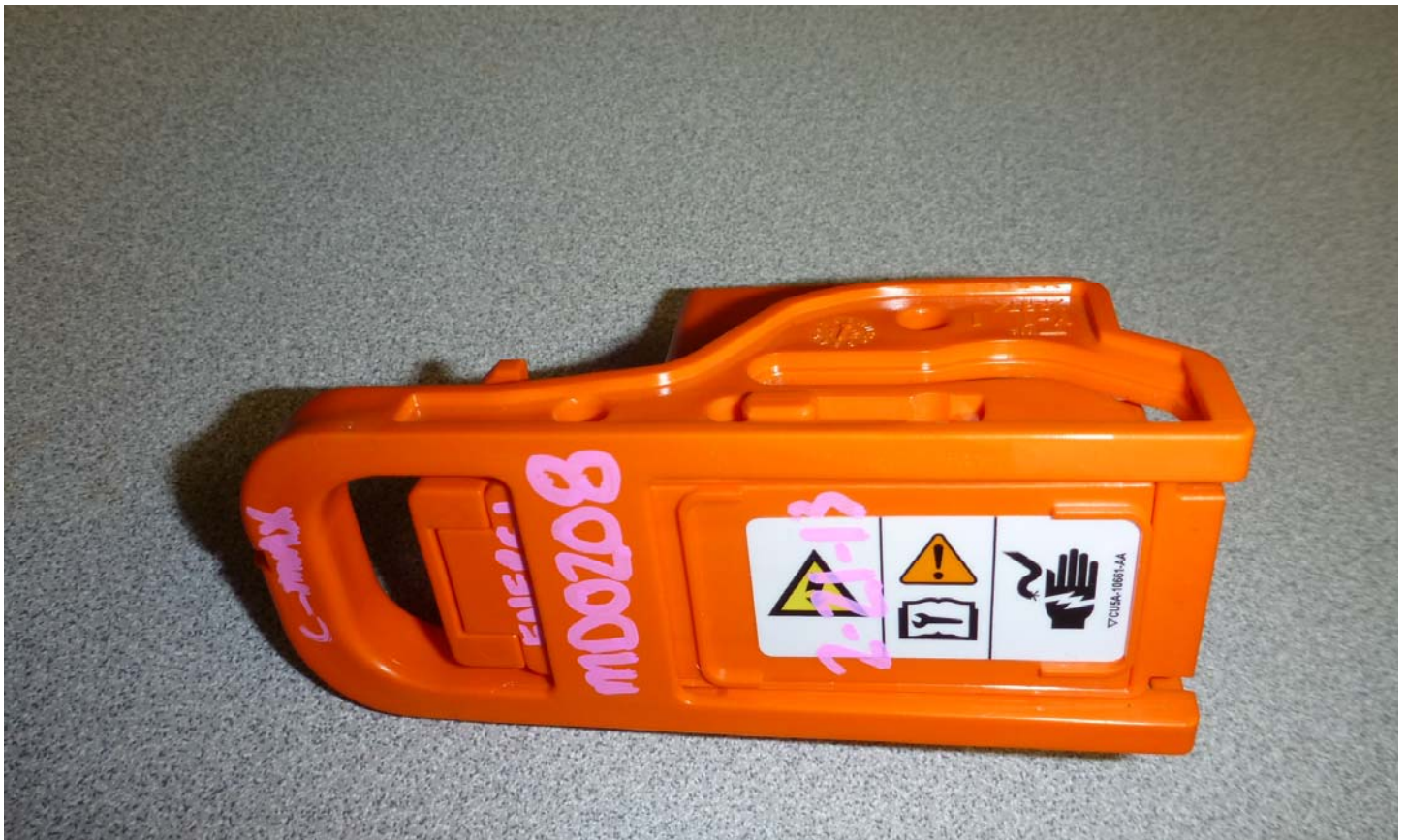
No. 008 Manual High Voltage Service Disconnect Removed
