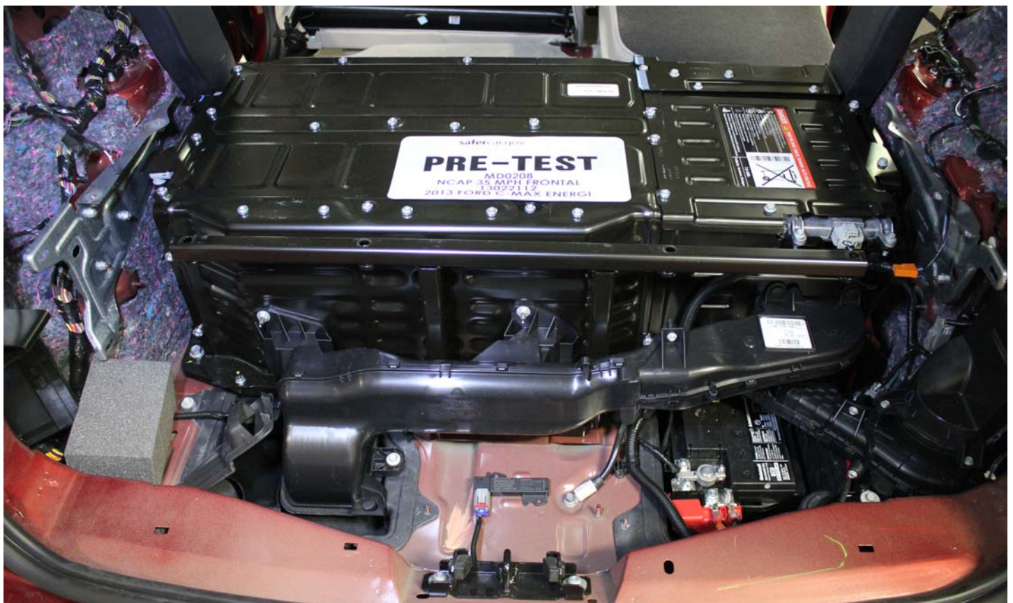
No. 009 Pre-Impact View of Propulsion Battery
