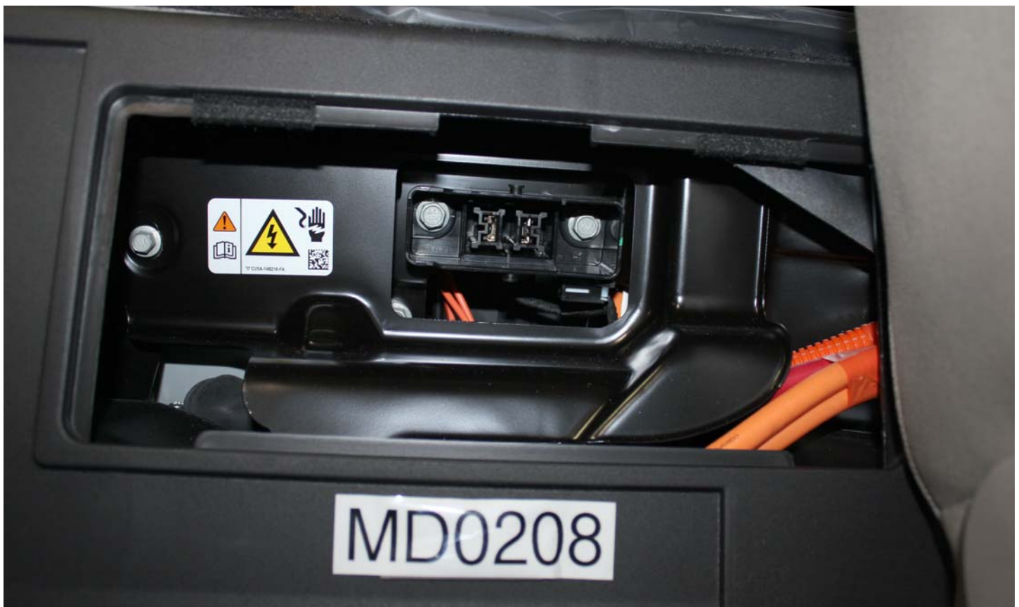
No. 007 Manual High Voltage Service Disconnect Removed
