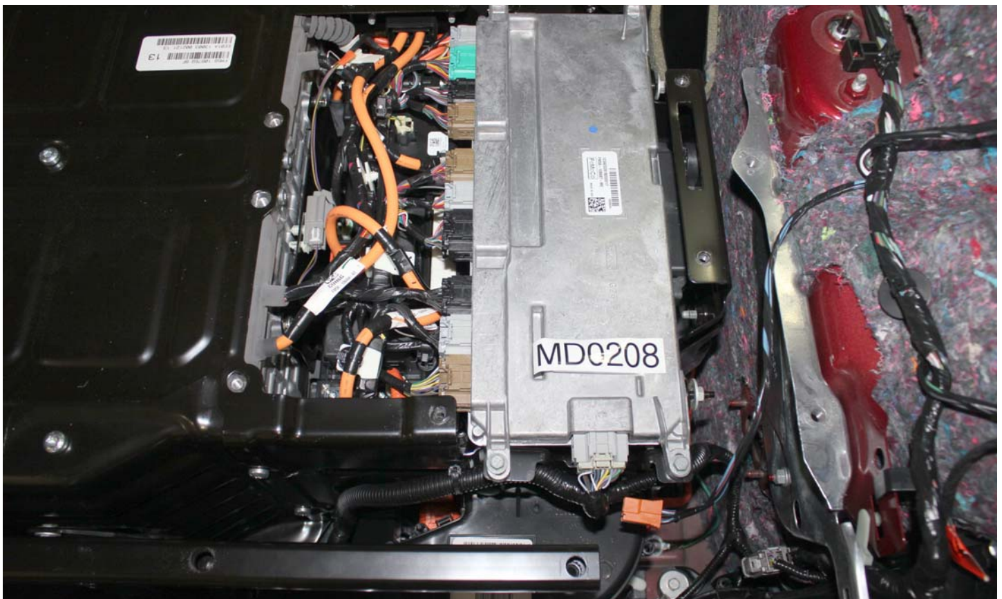
No. 018 Pre-Impact View of High Voltage Interconnect(s)
