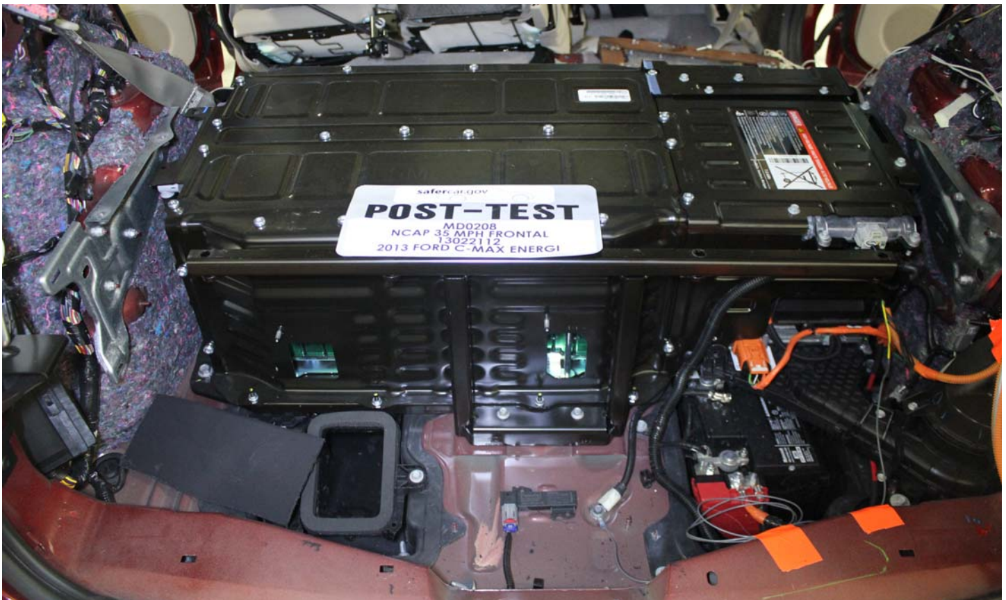
No. 011 Post-Impact Rear View of Propulsion Battery
