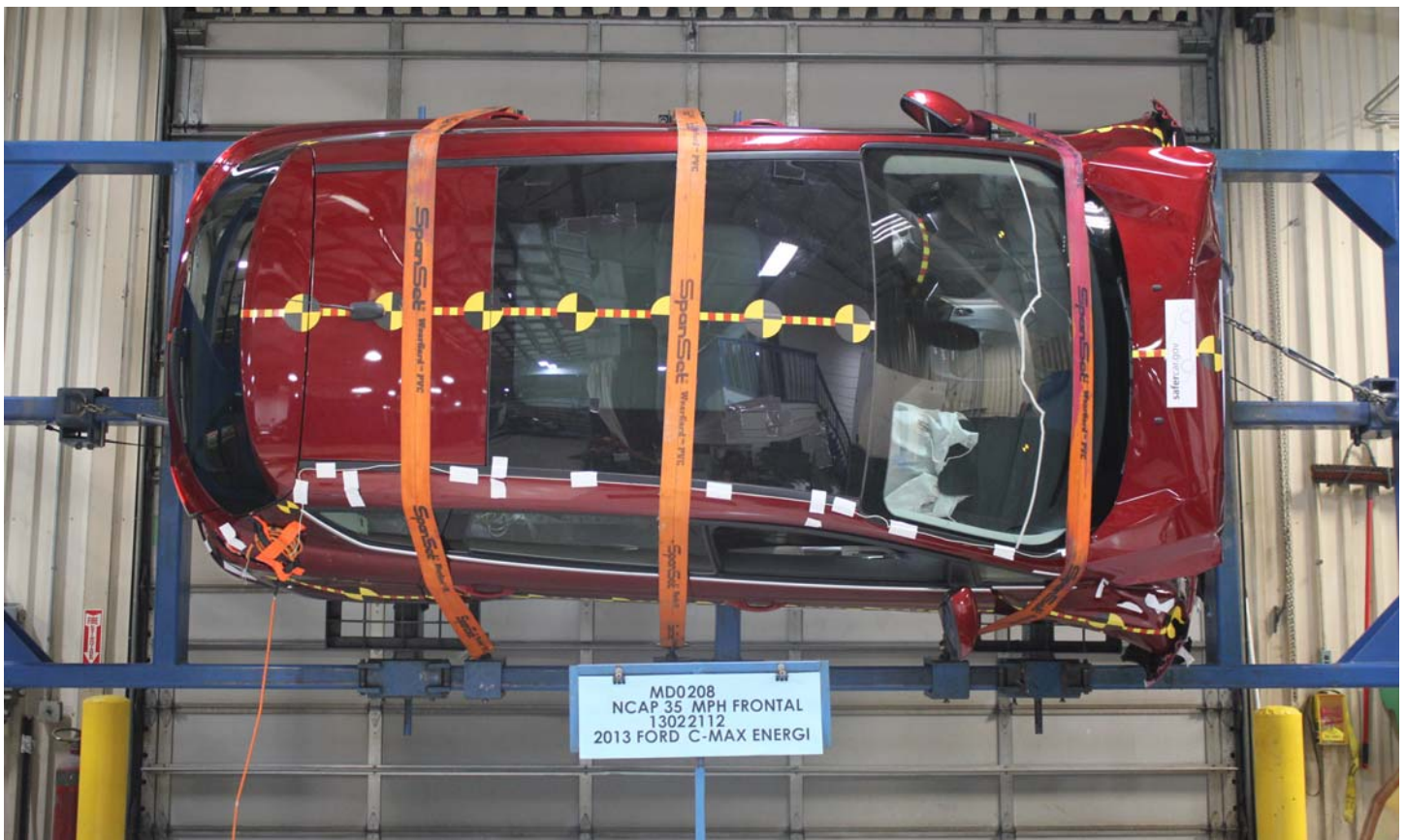
No. 028 FMVSS No. 305 Static Rollover at 90°
