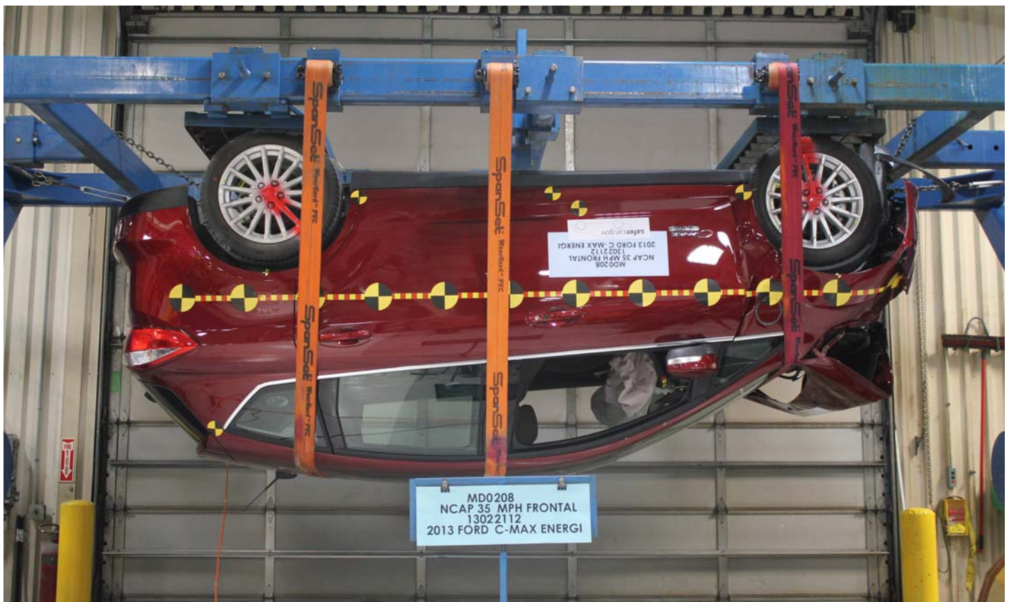
No. 029 FMVSS No. 305 Static Rollover at 180°
