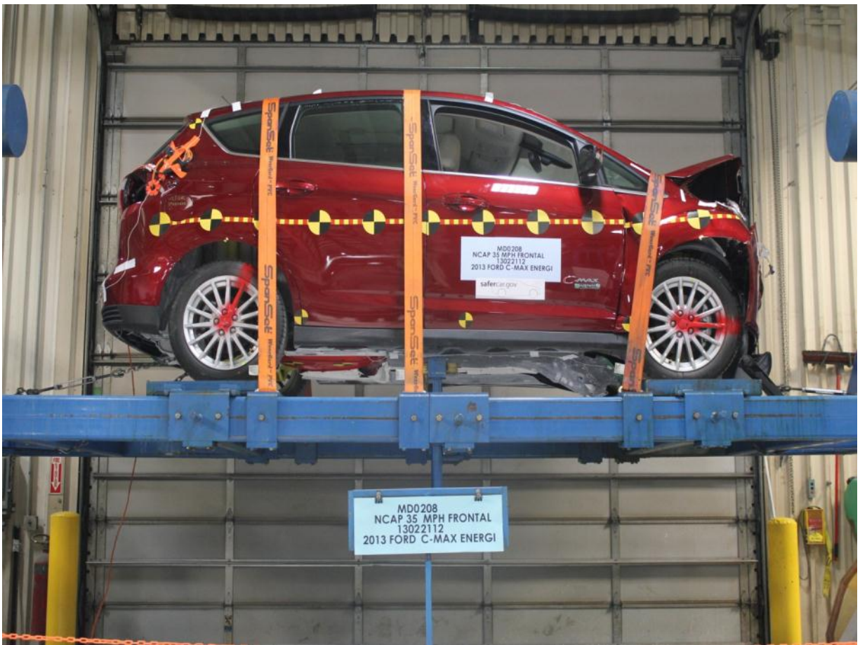
Vehicle at 360° on Static Rollover Device
