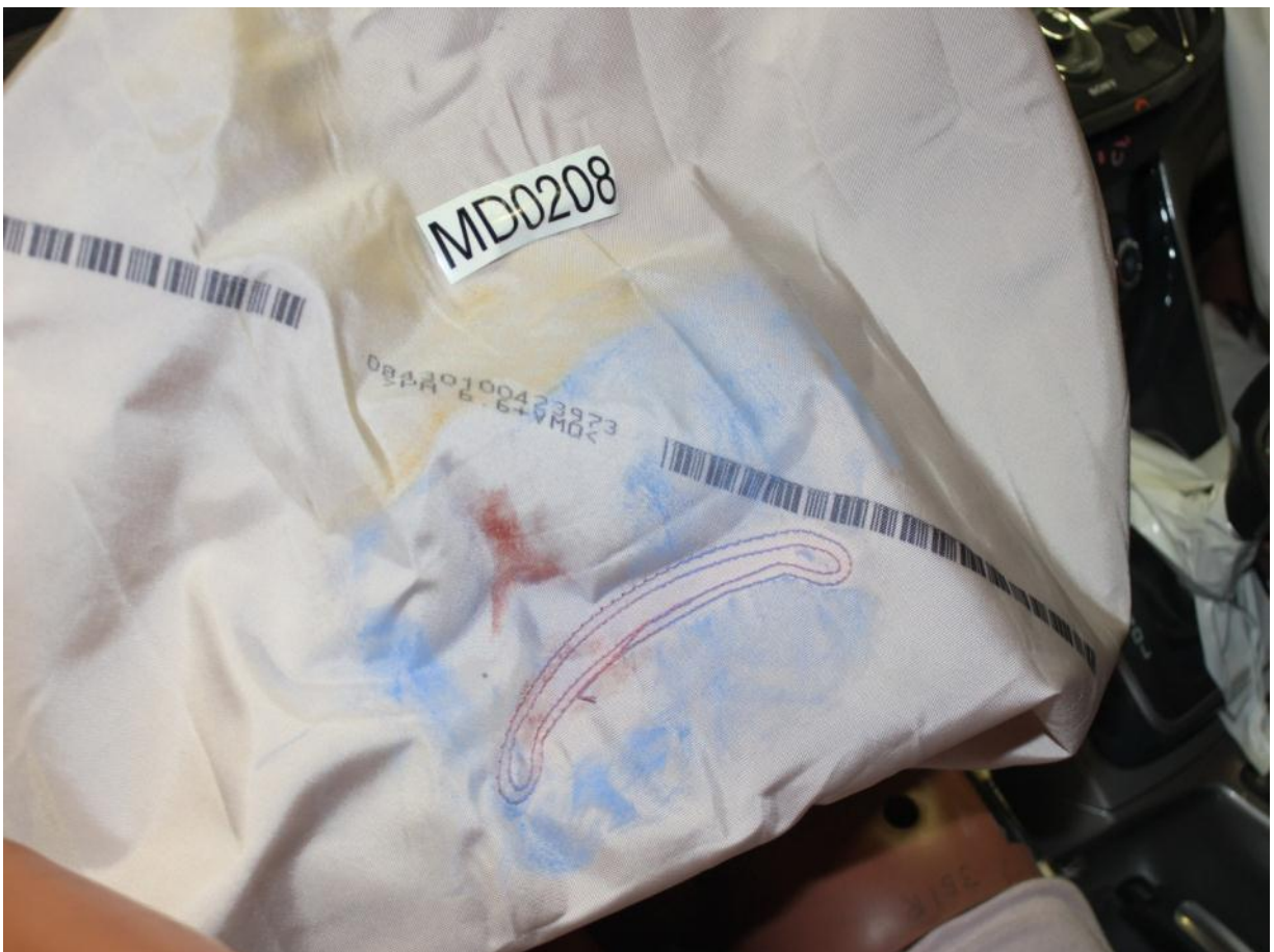
Post-Test Driver Dummy Contact with Airbag
