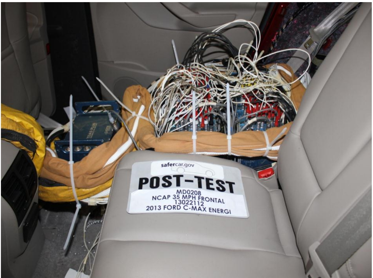
Post-Test Dummy Cable Routing
