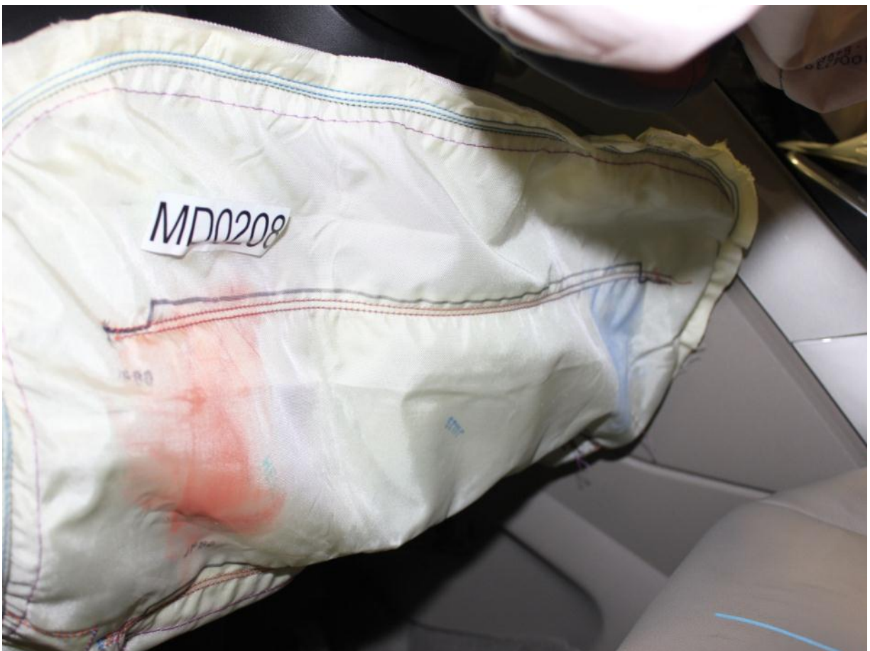
Post-Test Driver Dummy Contact with Knee Airbag
