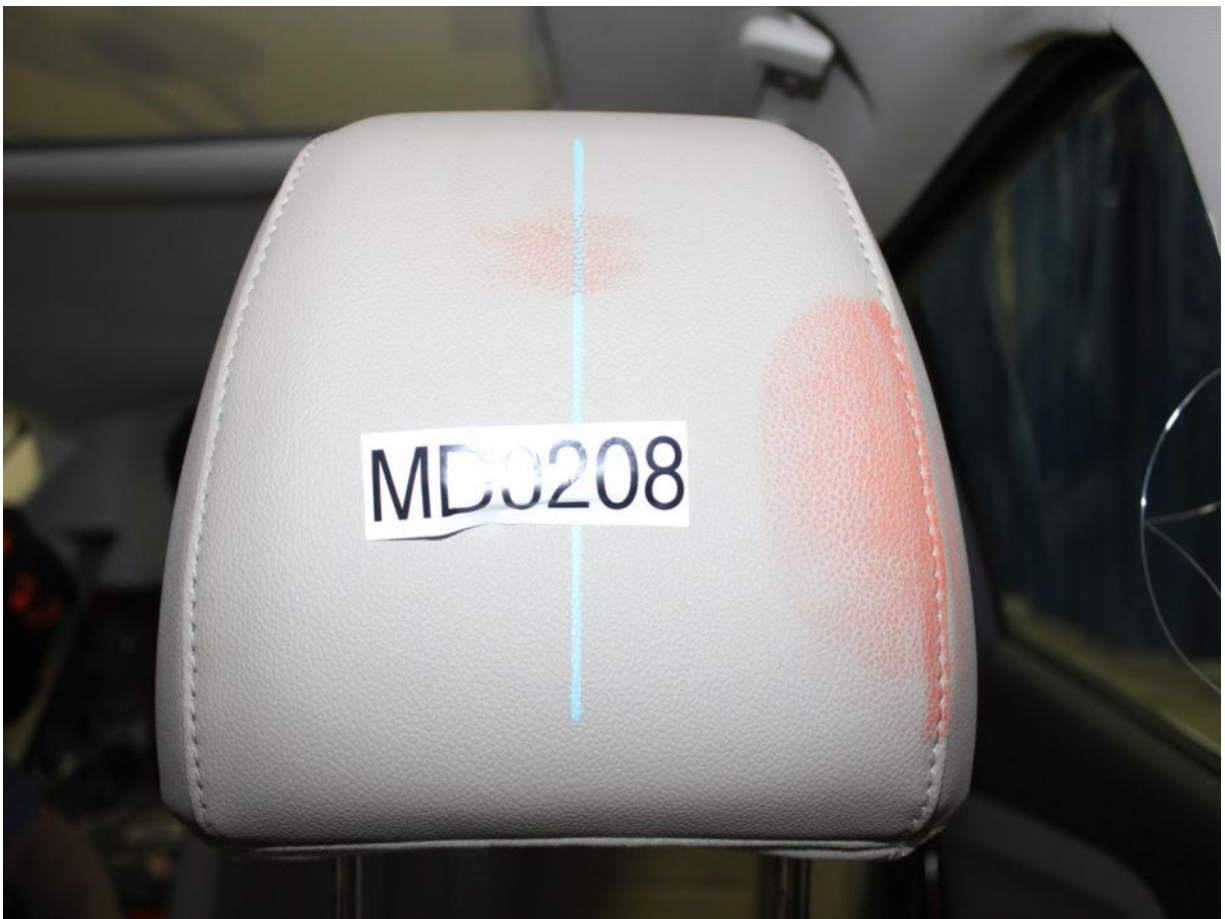
Post-Test Driver Dummy Contact with Headrest
