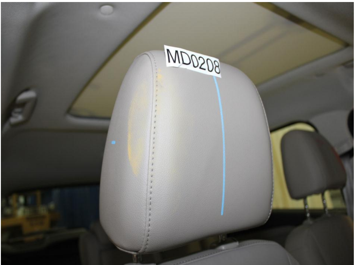
Post-Test Passenger Dummy Contact with Headrest
