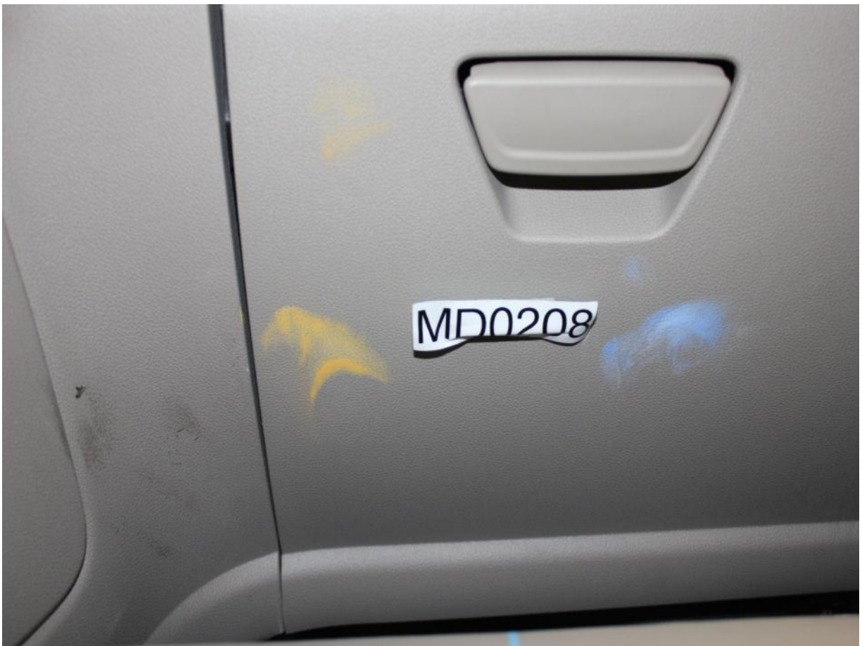
Post-Test Passenger Dummy Contact with Glove Box
