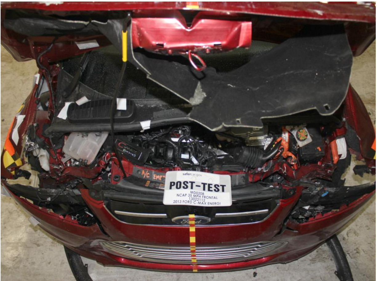
Post-Test Engine Compartment View
