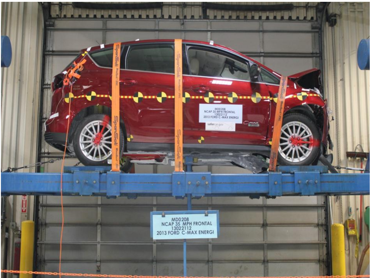
Vehicle at 0° on Static Rollover Device
