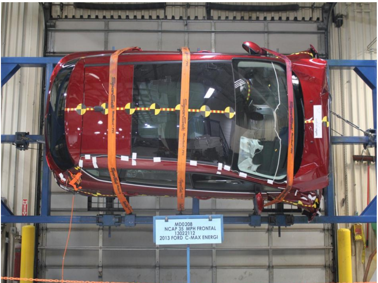
Vehicle at 90° on Static Rollover Device
