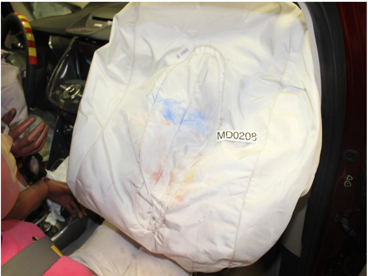
Post-Test Passenger Dummy Contact with Airbag
