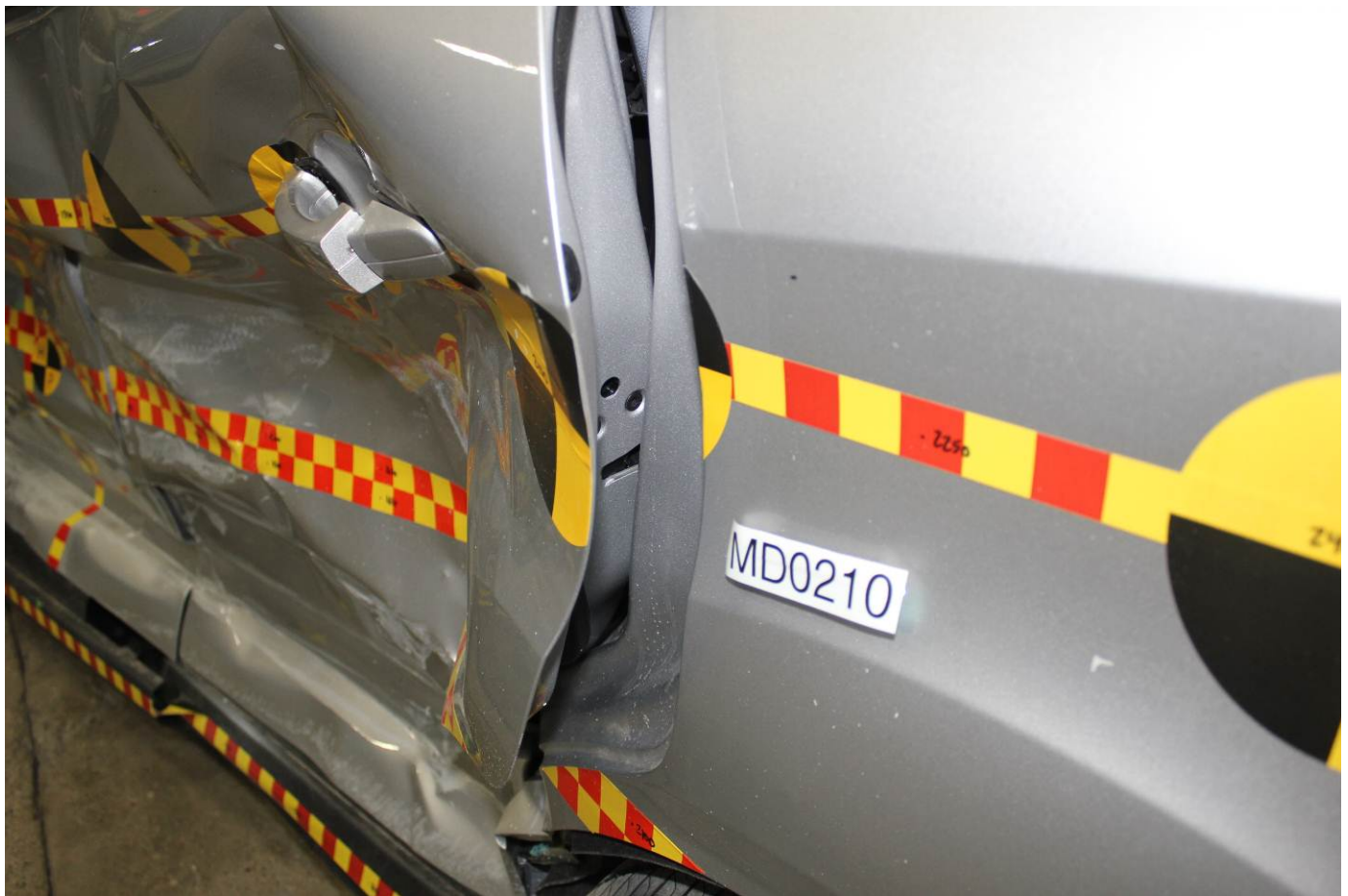
Post-Test Left Rear Door Disengaged
