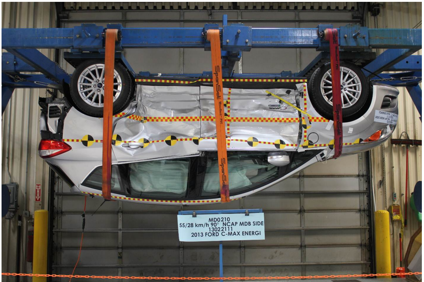
FMVSS No. 301 Static Rollover 180 Degrees
