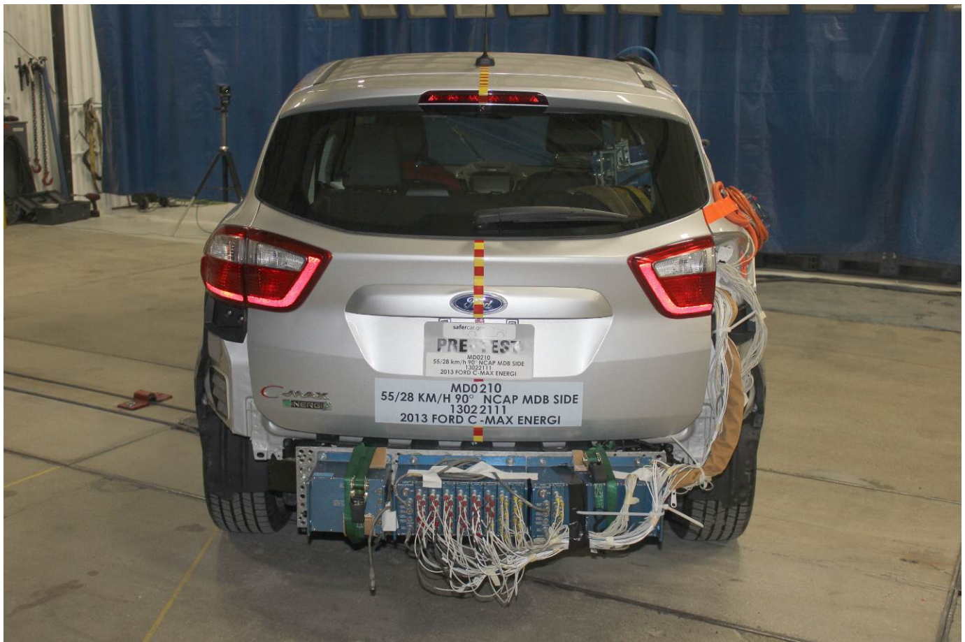
Pre-Test Rear View of Test Vehicle
