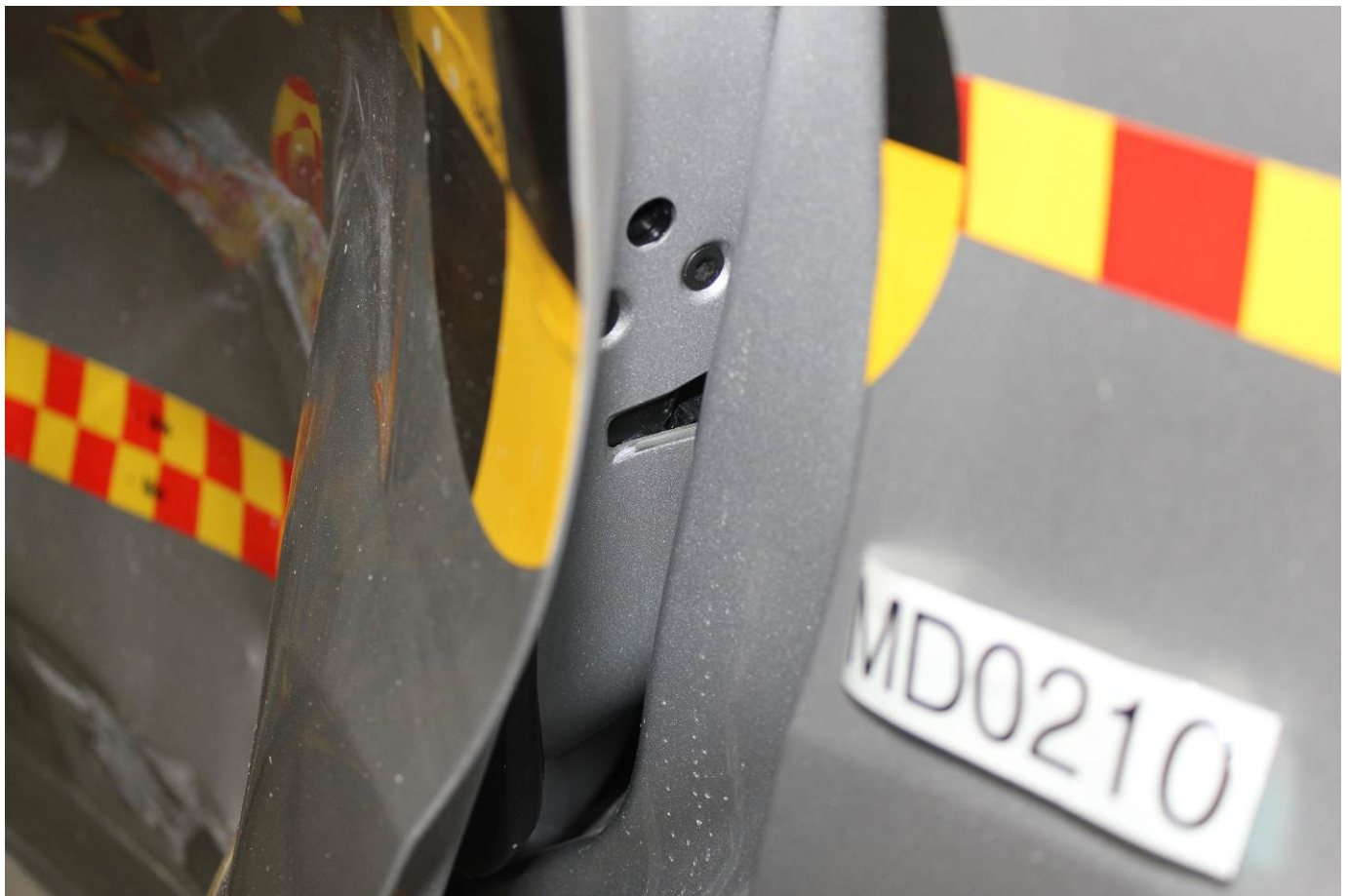
Post-Test Left Rear Door Disengaged
