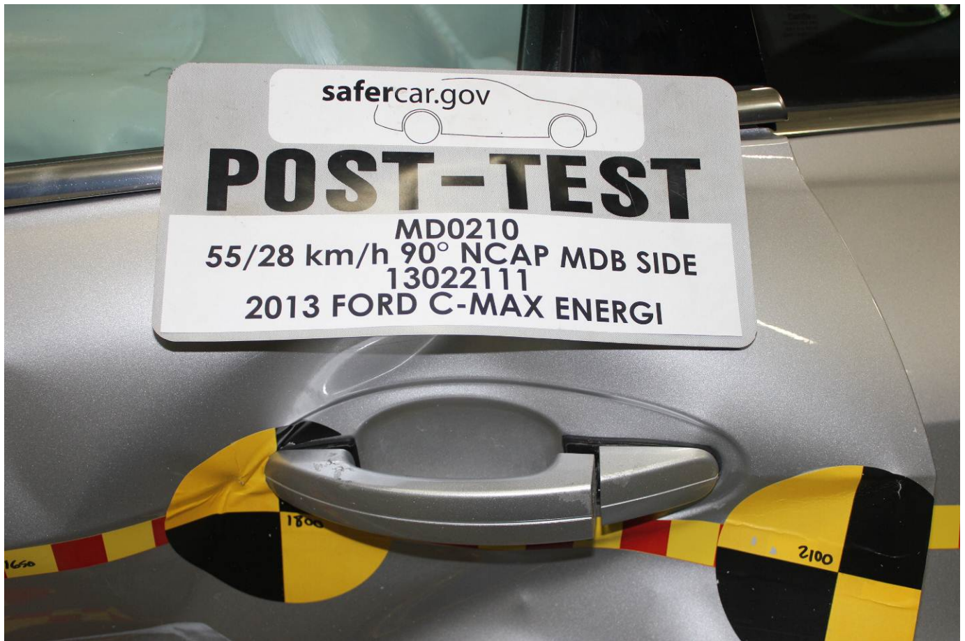
Post-Test Left Rear Door Latch Close-Up
