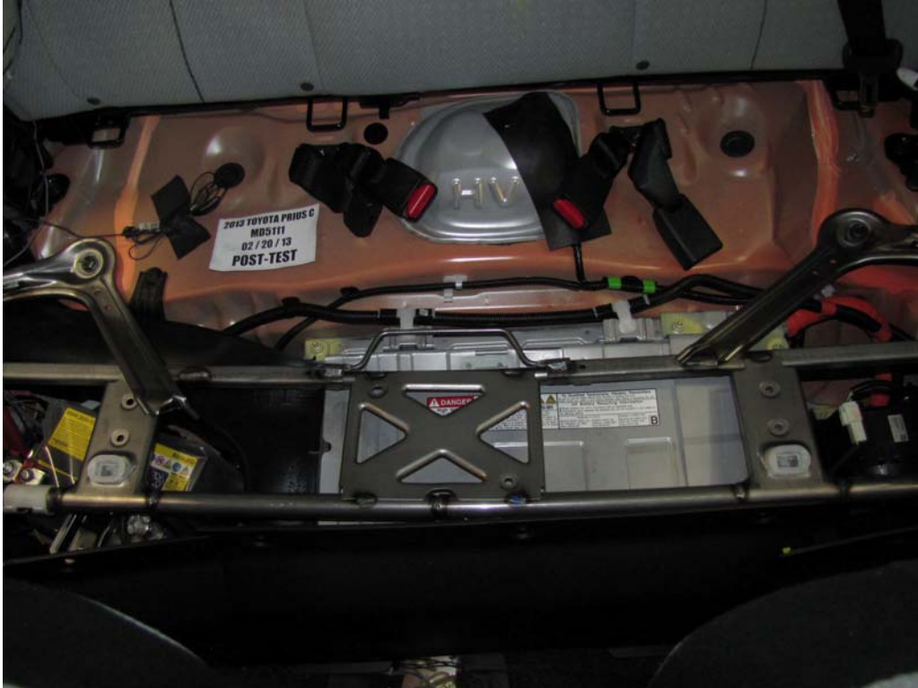
FIGURE 34. Post-Impact View of Vehicle Passenger Compartment of The Vehicle Adjacent to Propulsion Battery
