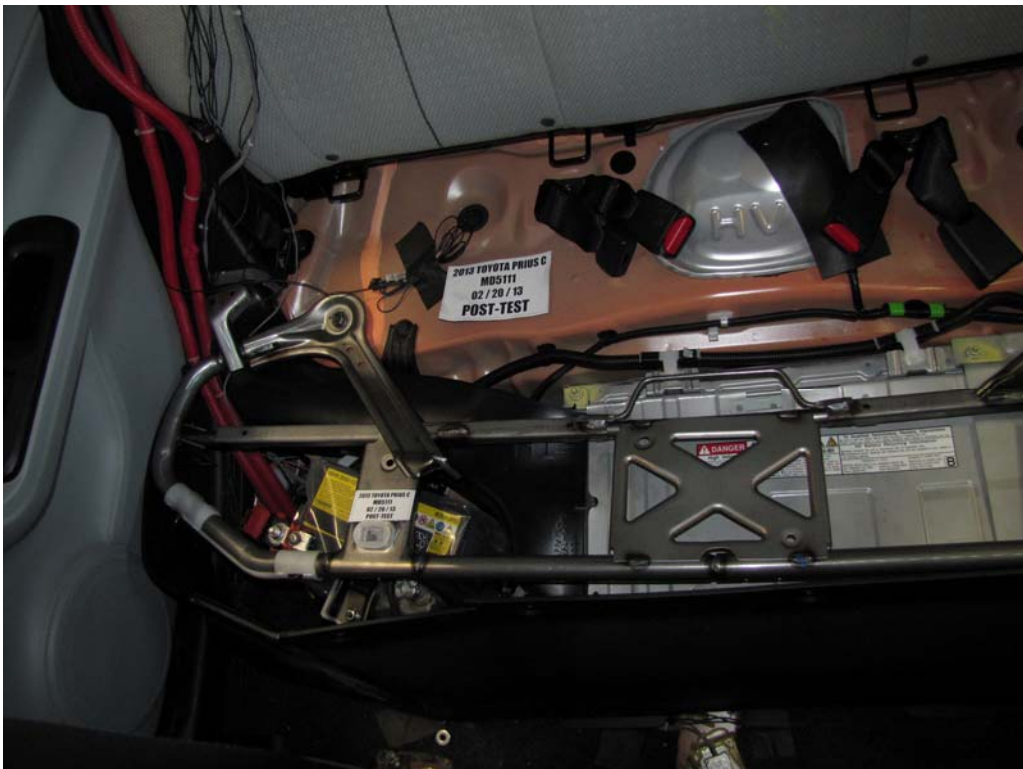
FIGURE 34a. Post-Impact View of Vehicle Passenger Compartment of The Vehicle Adjacent to Propulsion Battery
