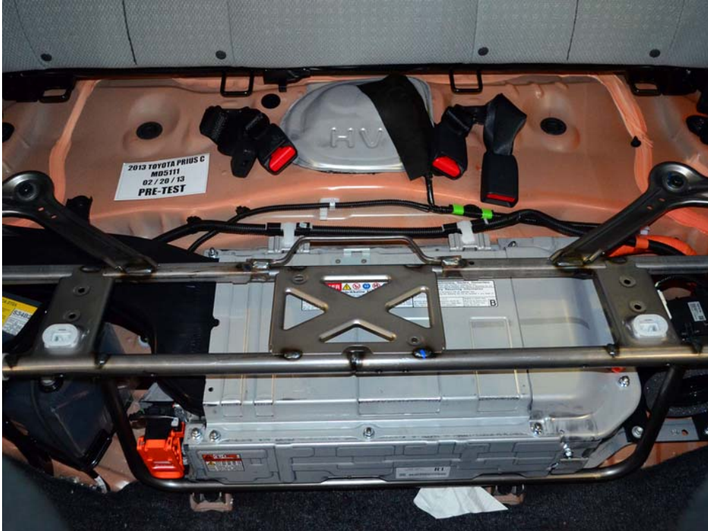
FIGURE 33. Pre-Impact View of Vehicle Passenger Compartment of The Vehicle Adjacent to Propulsion Battery
