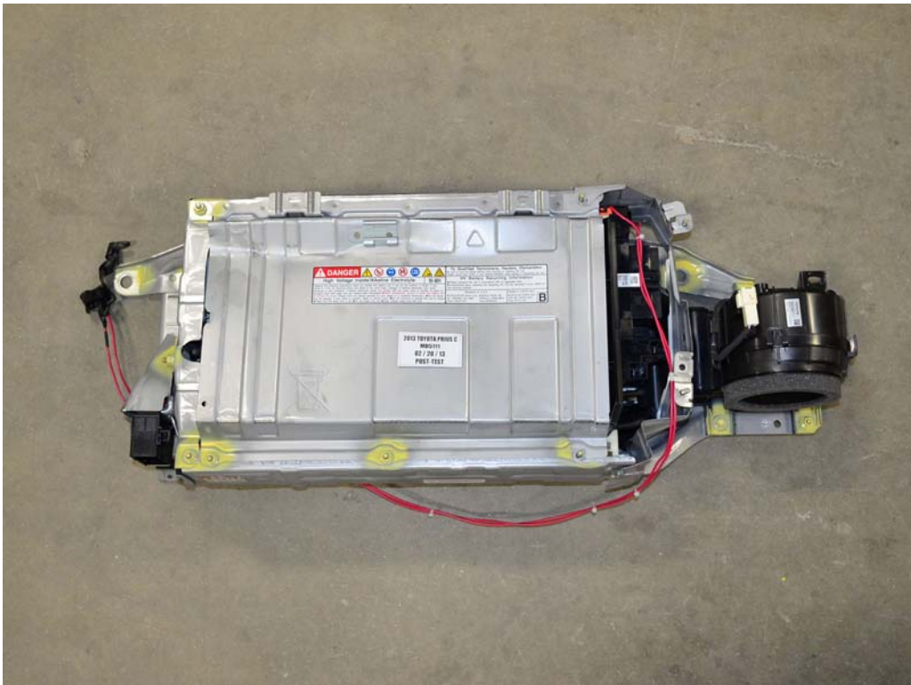
FIGURE 13. Post-Impact View of Battery Box or Container Which Holds Individual Battery Modules
