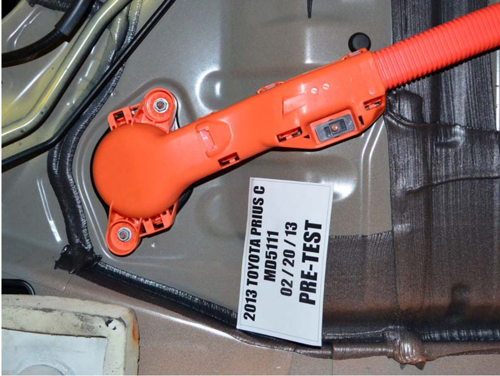
FIGURE 18a. Pre-Impact View of High Voltage Interconnect
