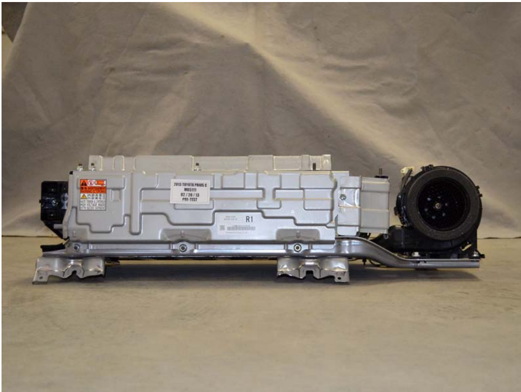
FIGURE 12a. Pre-Impact View of Battery Box or Container Which Holds Individual Battery Modules
