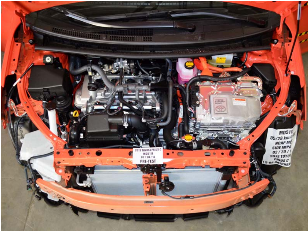
FIGURE 16. Pre-Impact View of Electric Propulsion Drive
