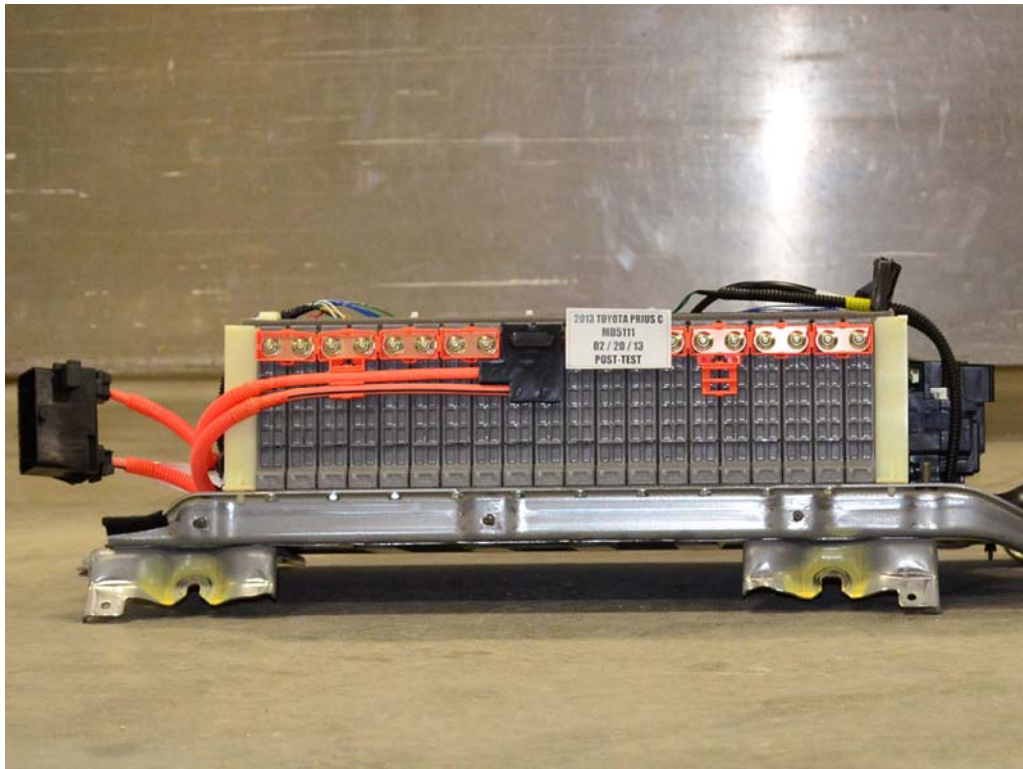
FIGURE 15. Post-Impact View of Propulsion Battery Modules
