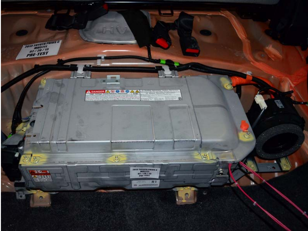
FIGURE 10. Post-Impact Front View of Propulsion Battery
