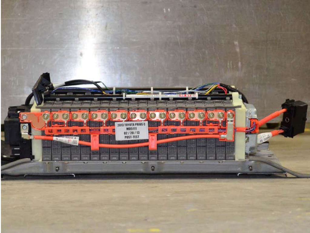
FIGURE 15a. Post-Impact View of Propulsion Battery Modules
