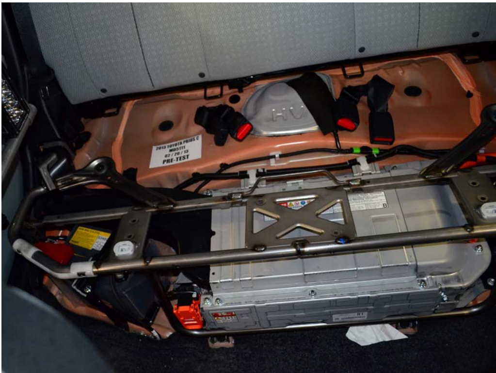
FIGURE 33a. Pre-Impact View of Vehicle Passenger Compartment of The Vehicle Adjacent to Propulsion Battery
