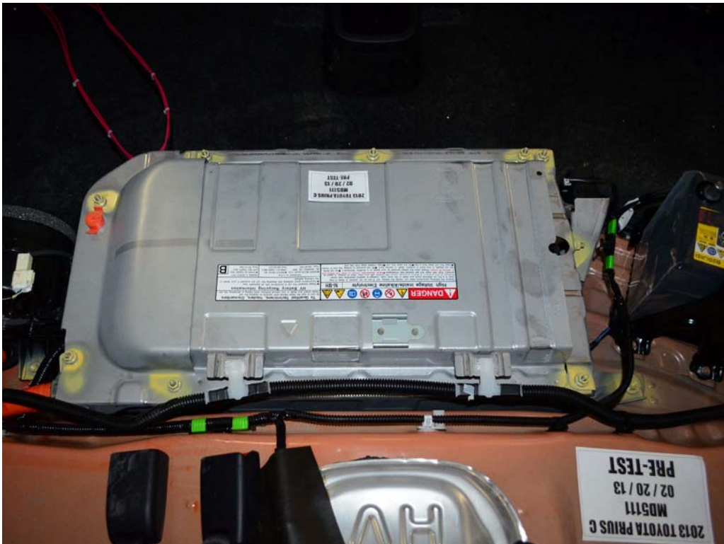
FIGURE 11. Post-Impact Rear View of Propulsion Battery
