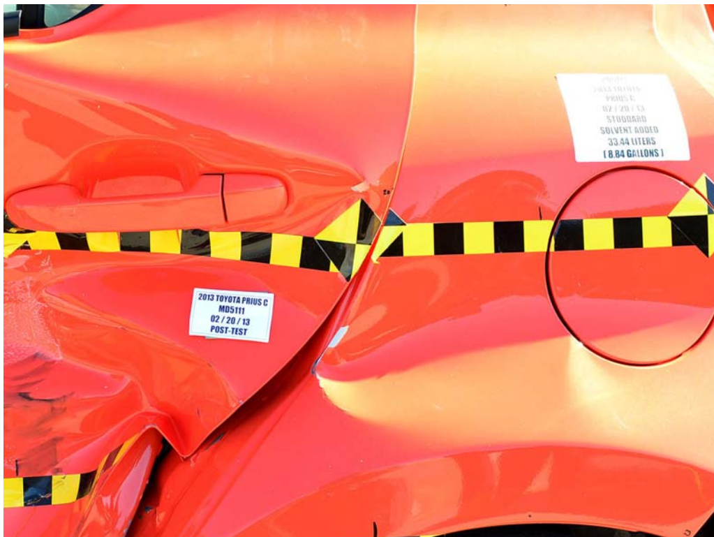
FIGURE 24. Post-Test Left Rear Door Latch Close-Up
