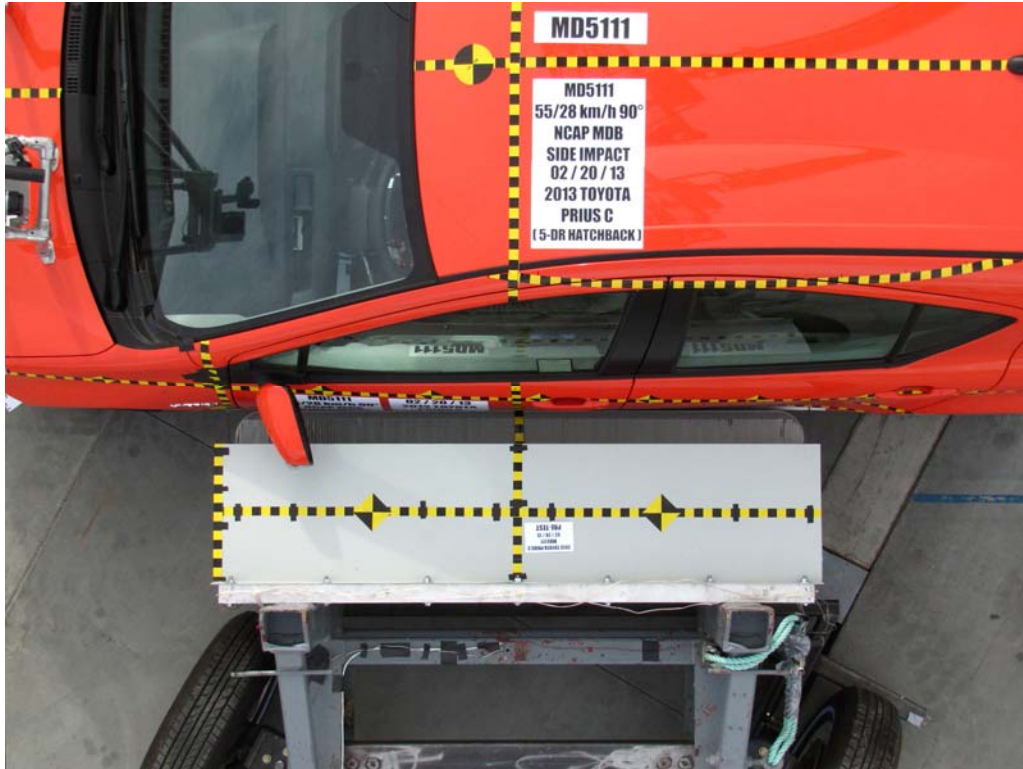
FIGURE 15. Pre-Test Overhead View of Test Area
