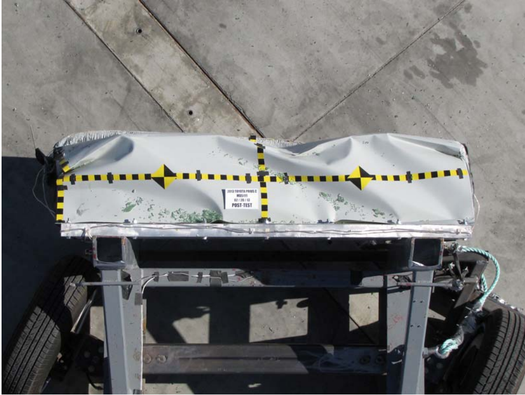
FIGURE 87. Post-Test Top View of MDB Impactor Face
