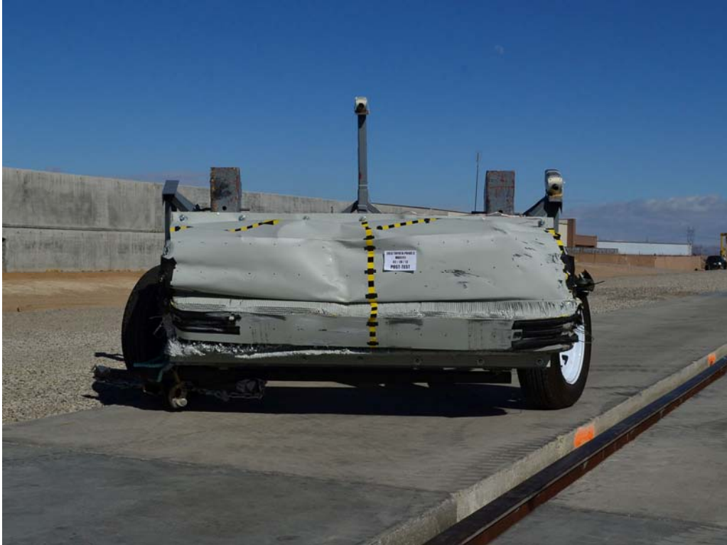
FIGURE 85. Post-Test Front View of MDB Impactor Face
