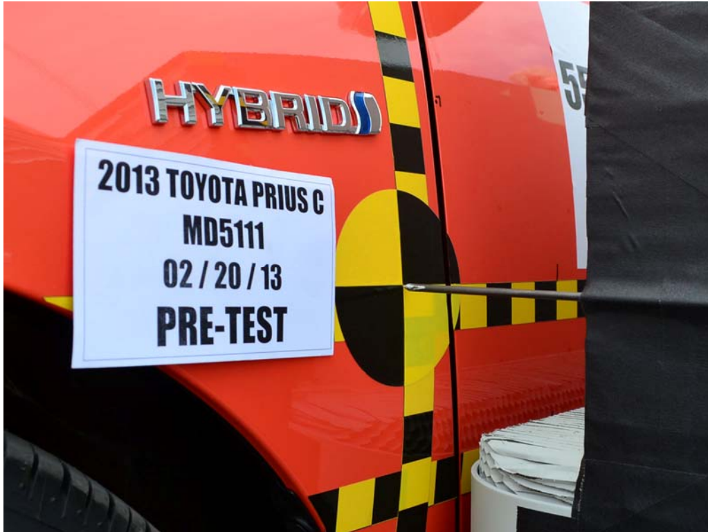
FIGURE 19. Pre-Test Close-Up View of Impact Point Target
