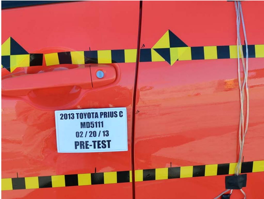
FIGURE 21. Pre-Test Left Front Door Latch Close-Up
