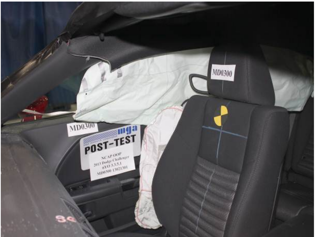
Post-Test Curtain Airbag Left 3/4 Front View
