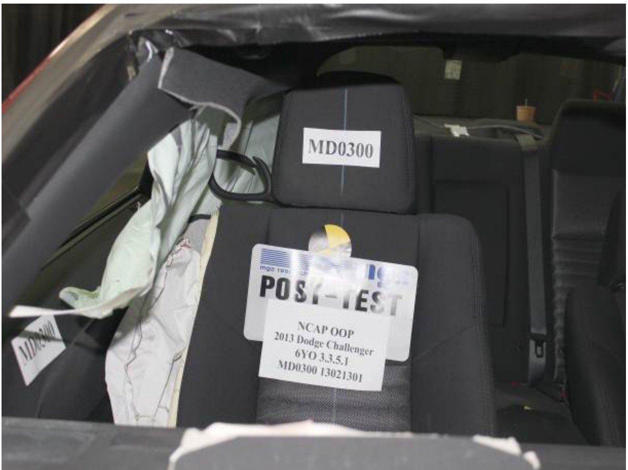
Post-Test Curtain Airbag Front View
