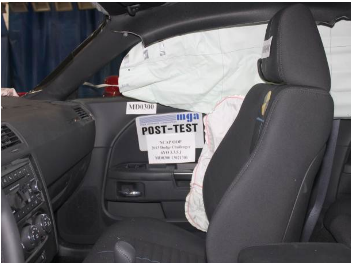
Post-Test Curtain Airbag Left Side View
