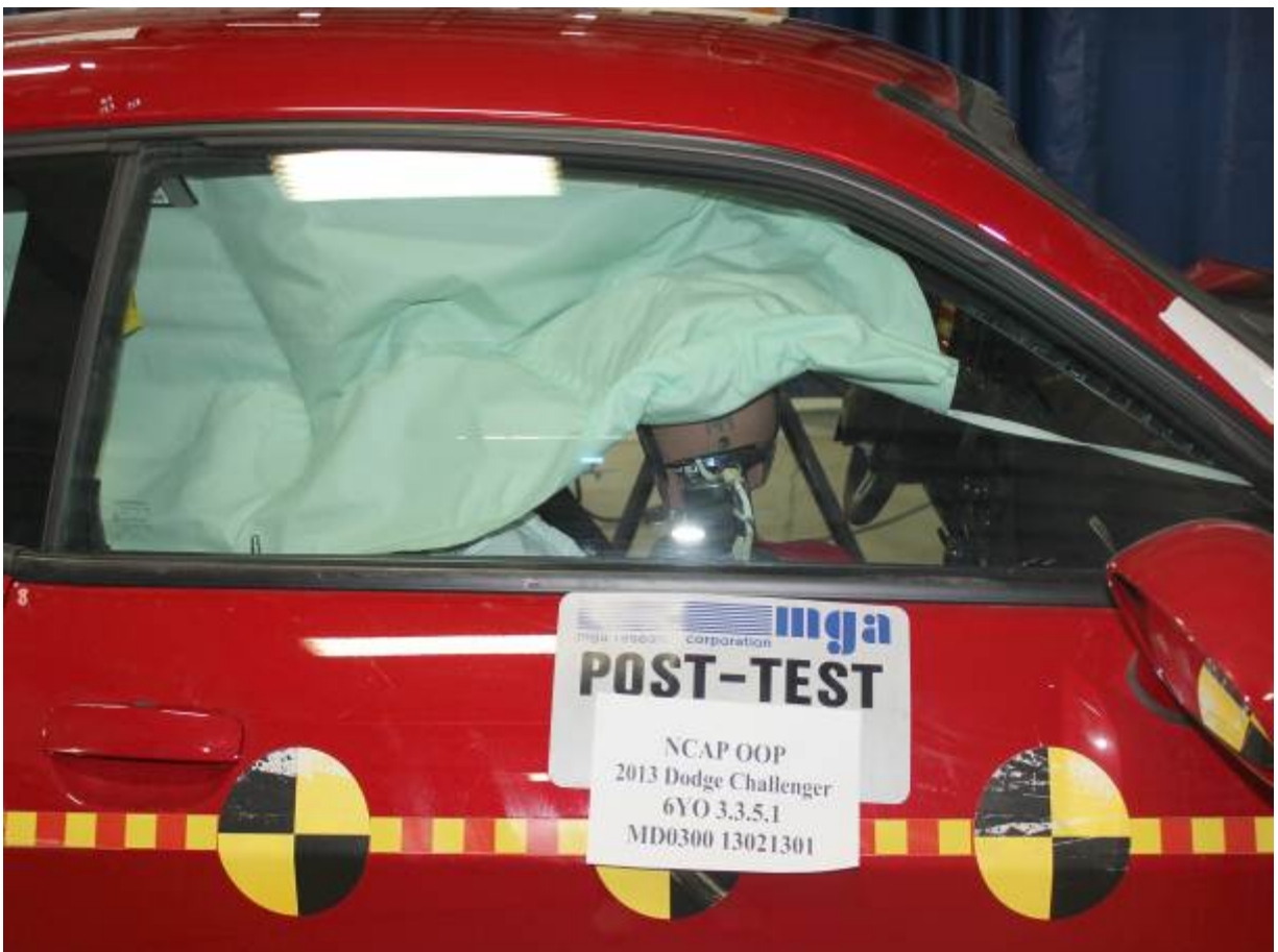
Post-Test 6-Year-Old Child Dummy Right Side View
