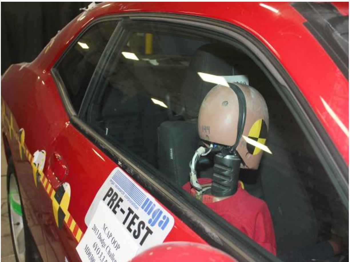
Pre-Test 6-Year-Old Child Dummy Right ¾ Front View
