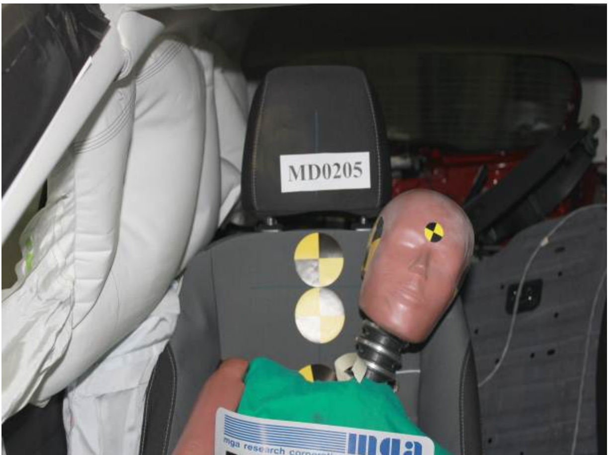
Post-Test SID-IIs Dummy Front Closeup View
