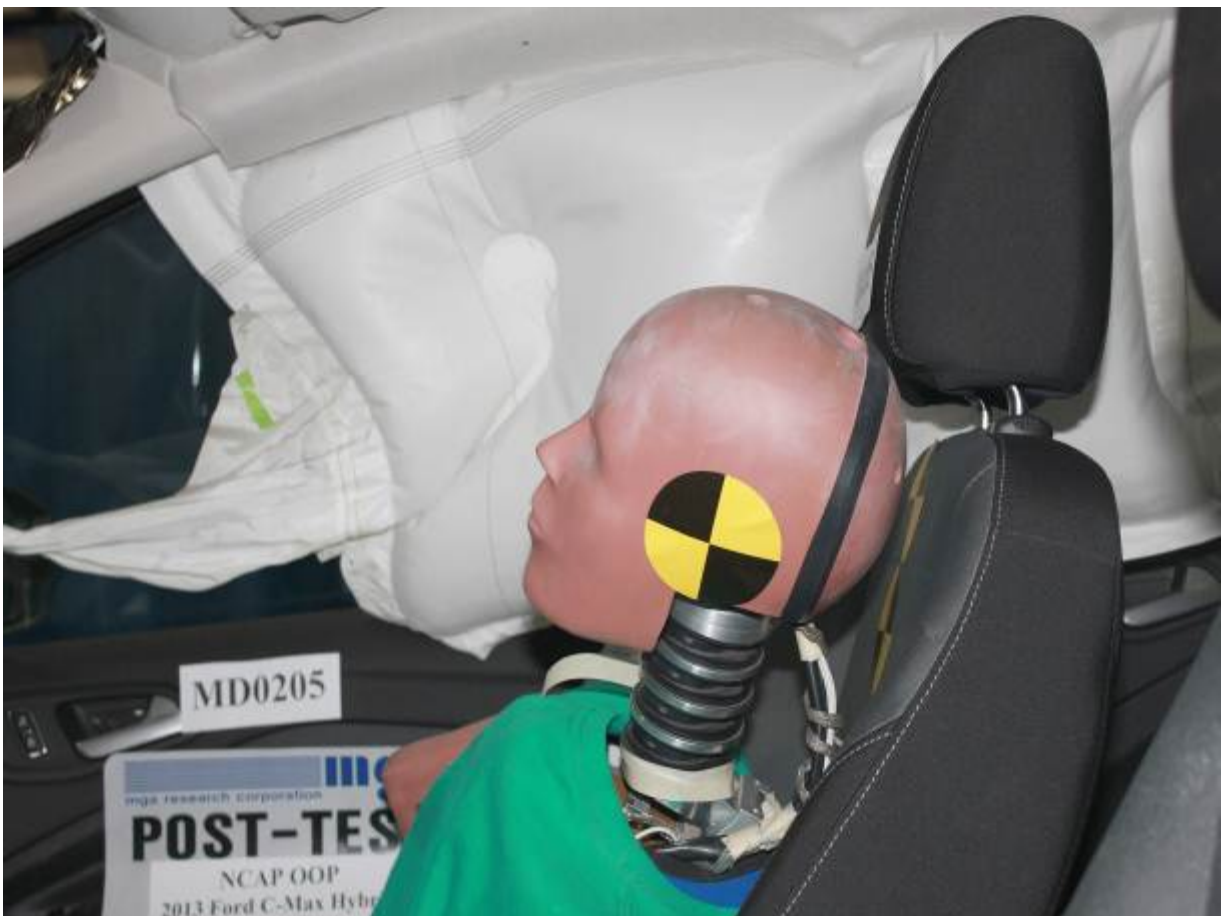
Post-Test SID-IIs Dummy Left Side Closeup View
