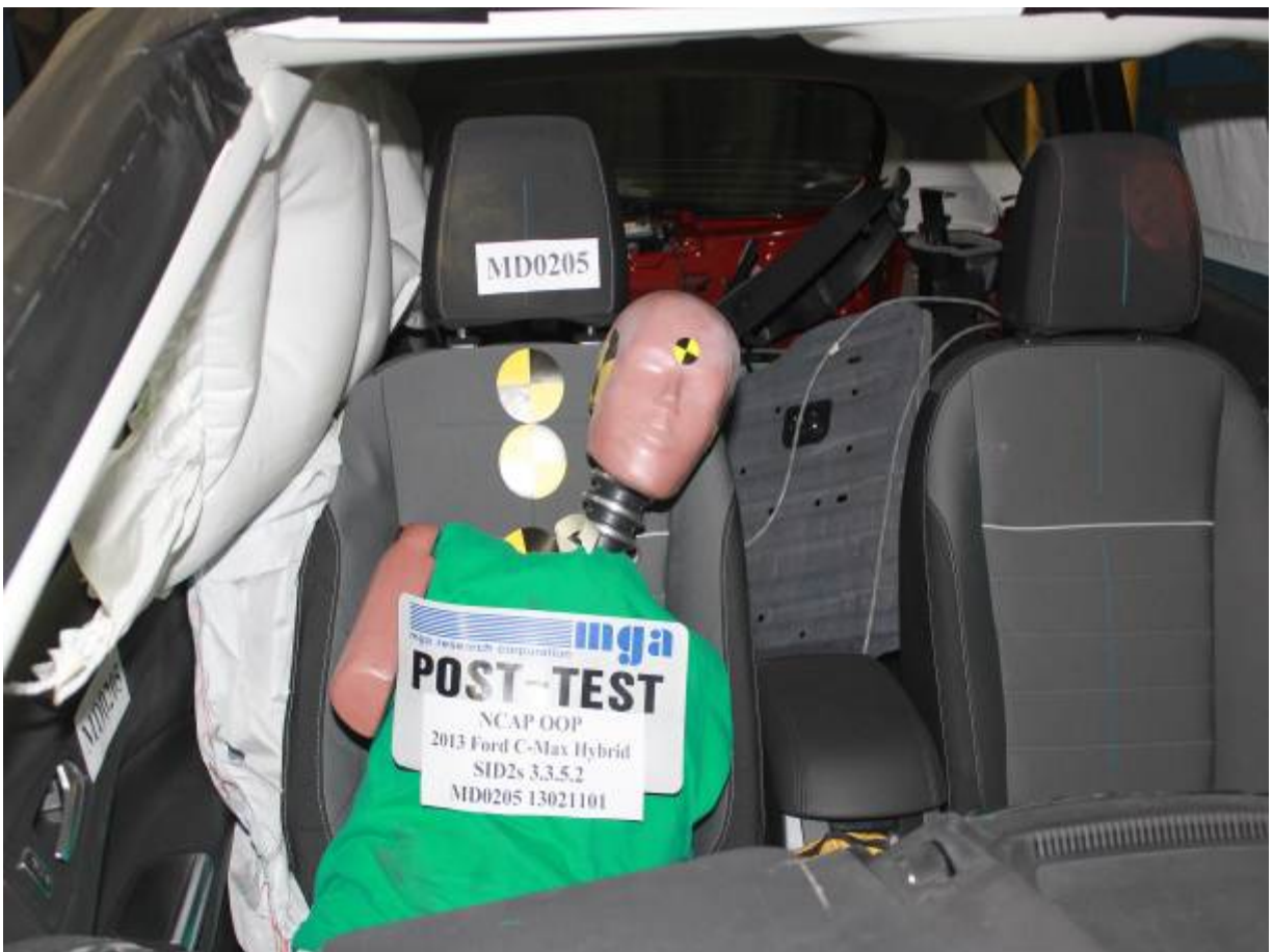
Post-Test SID-IIs Dummy Front View
