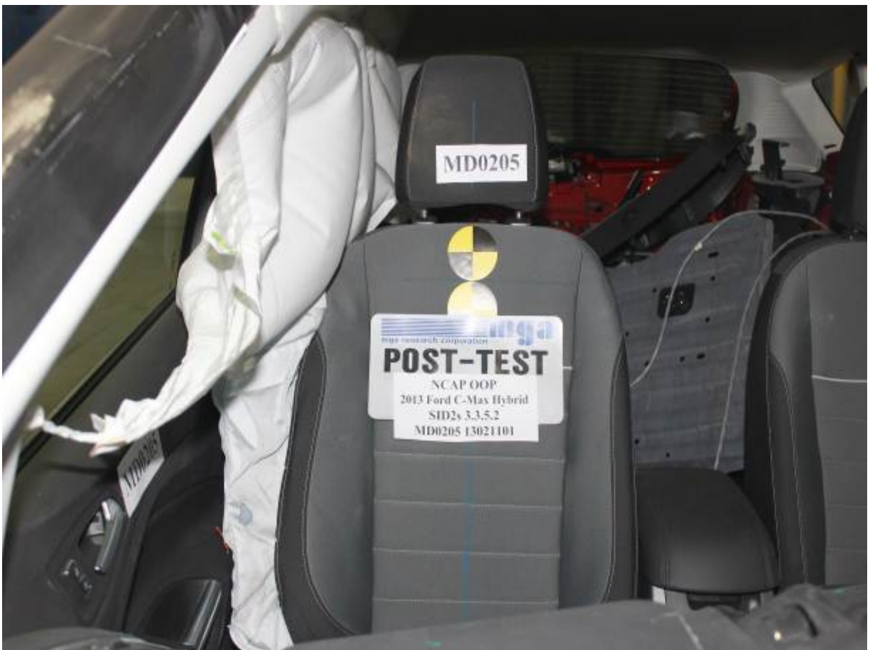
Post-Test Curtain Airbag Front View
