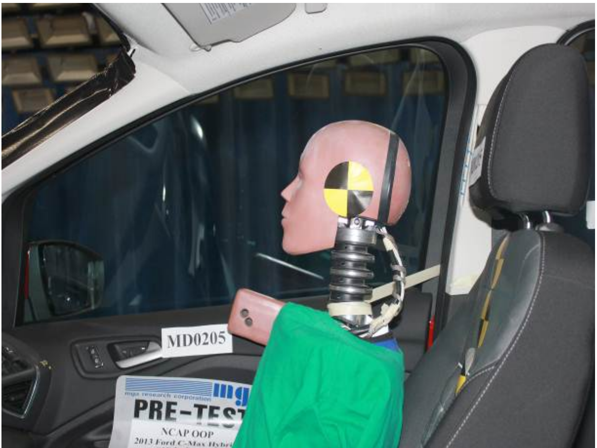
Pre-Test SID-IIs Dummy Left Side Closeup View
