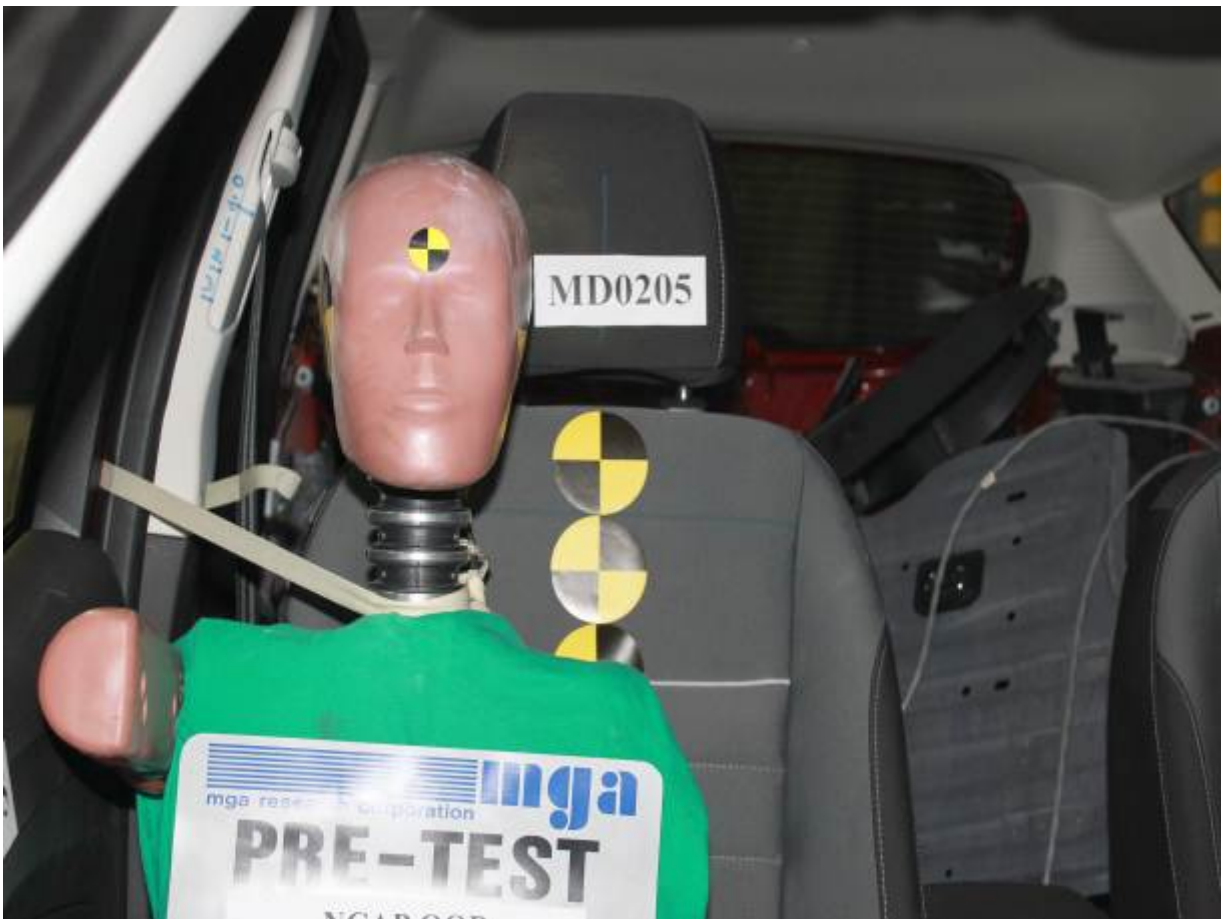
Pre-Test SID-IIs Dummy Front Closeup View
