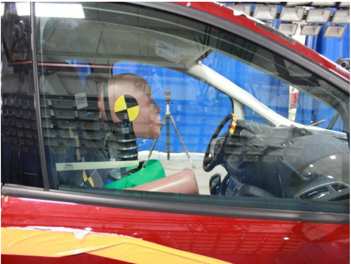
Pre-Test SID-II's Dummy Right Side View
