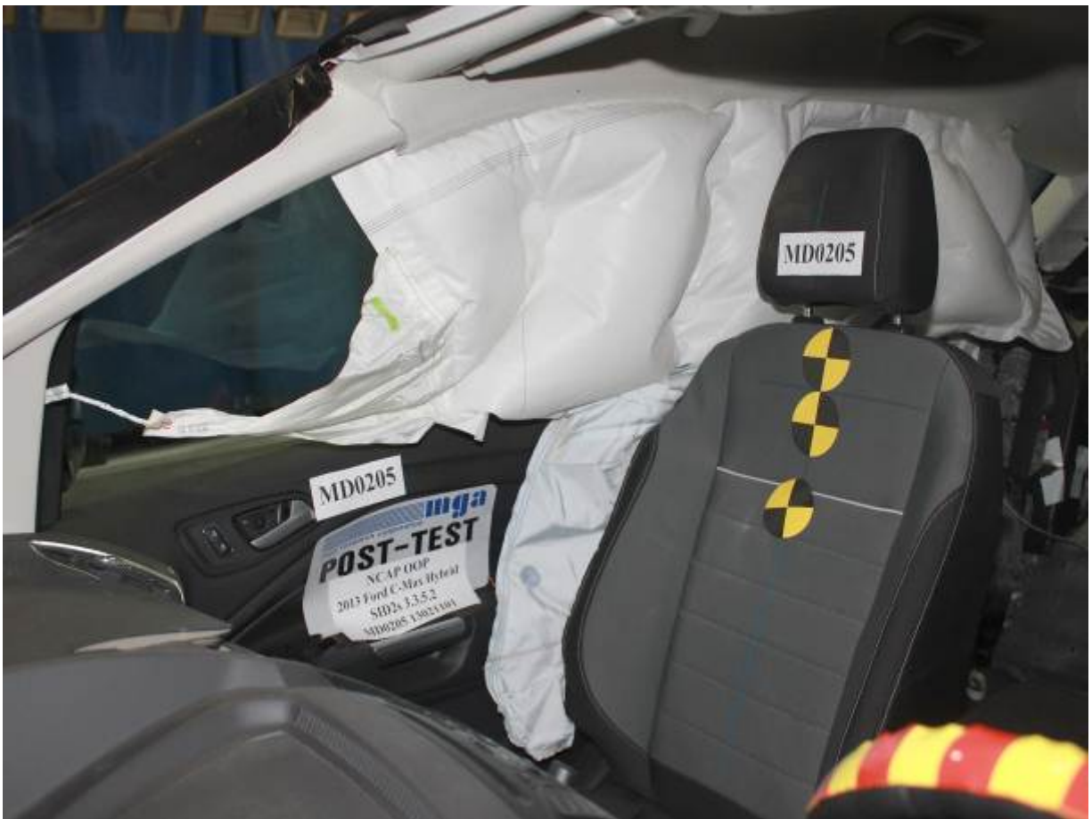
Post-Test Curtain Airbag Left 3/4 Front View
