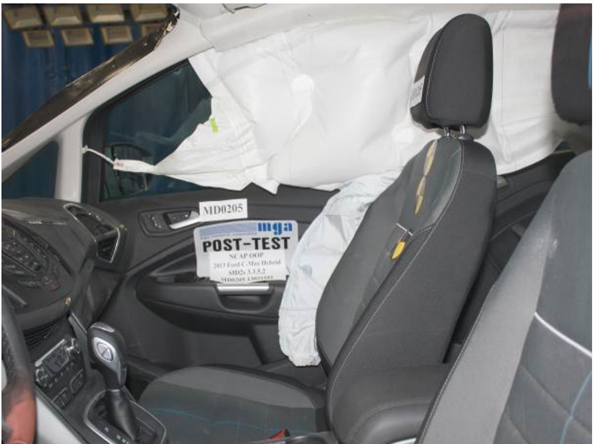
Post-Test Curtain Airbag Left View
