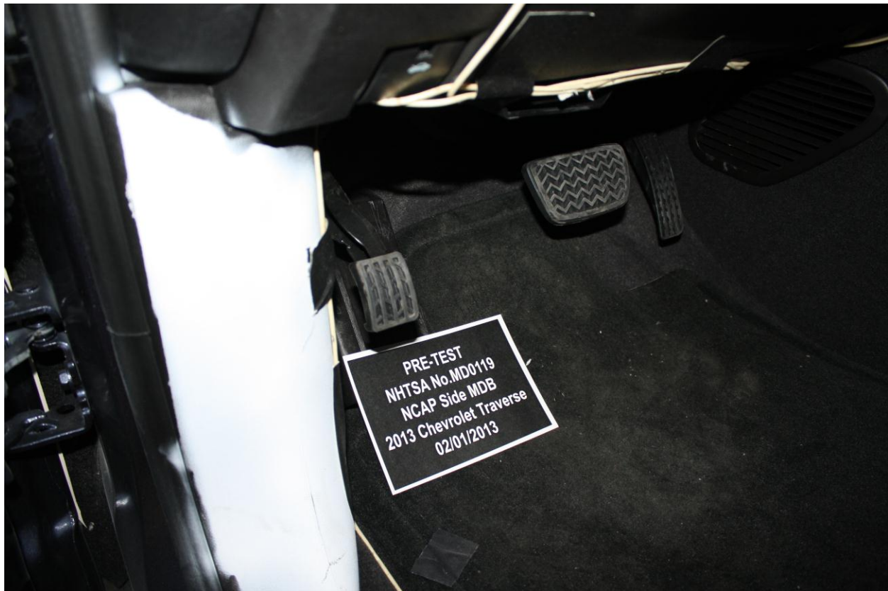
Figure A-37: View of Disengaged Parking Brake
